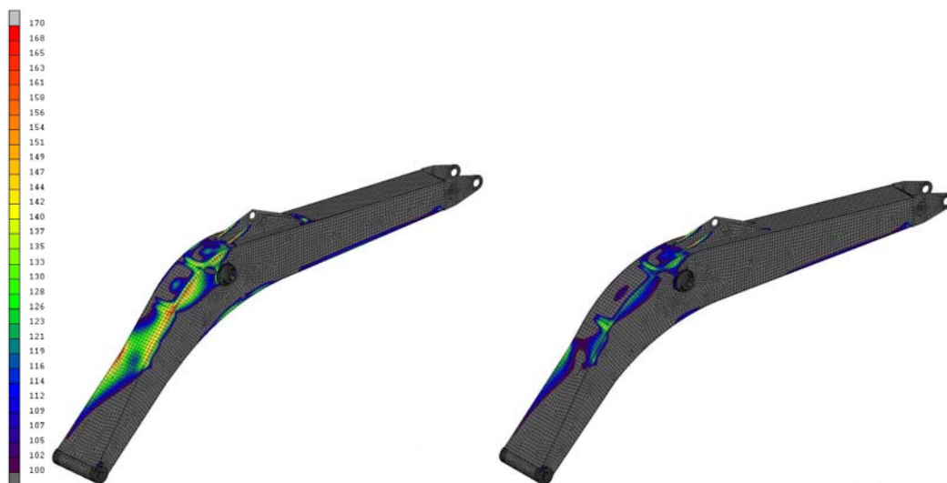
Figure 6.7: von Mises stress maps for initial (left) and 90 th (right) booms_B
