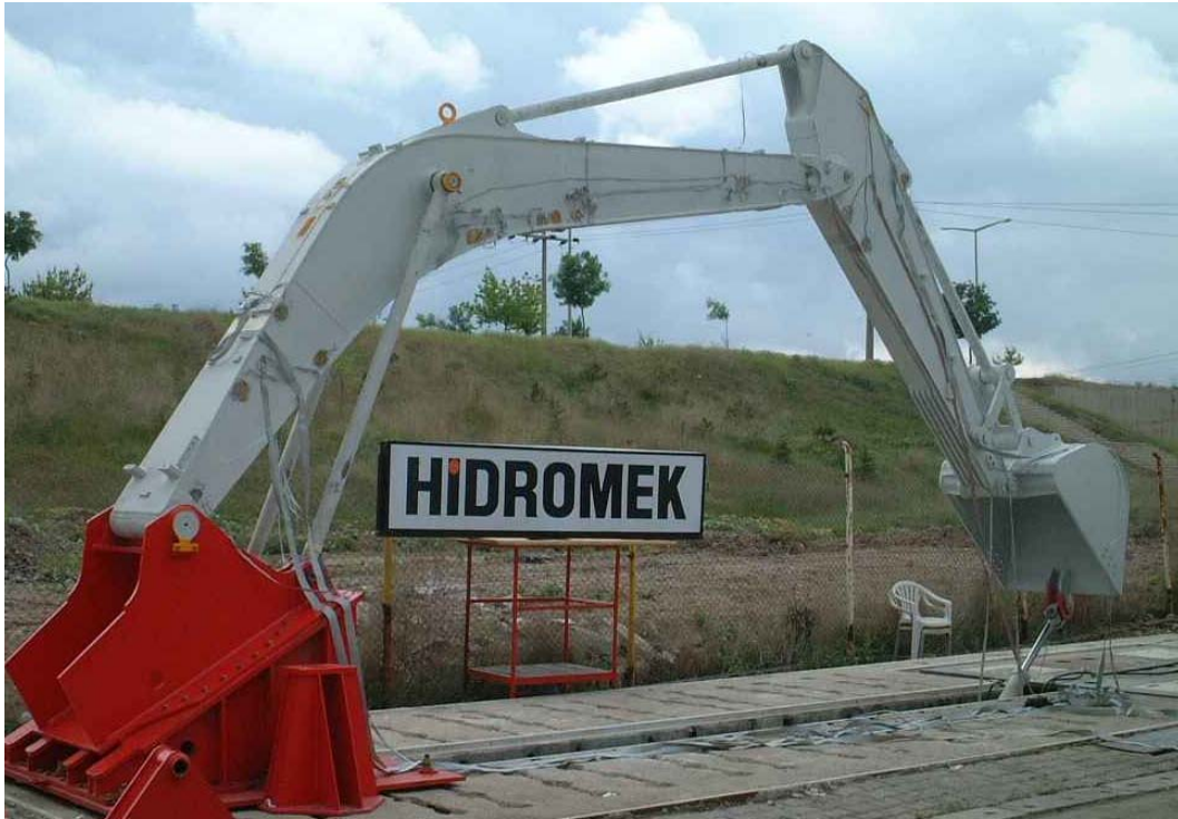
Figure 4.10: Test setup of the boom [15]
