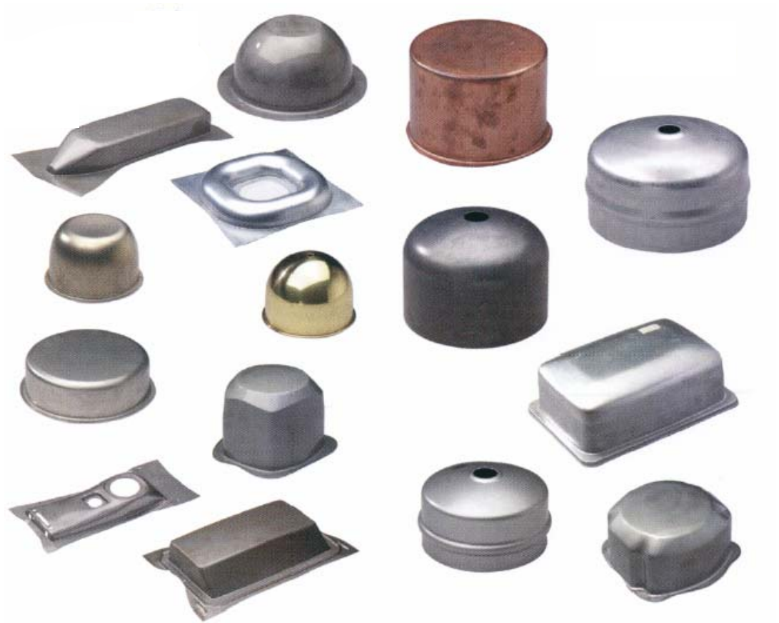
Figure 2.2 Examples to conventional deep drawing workpieces
