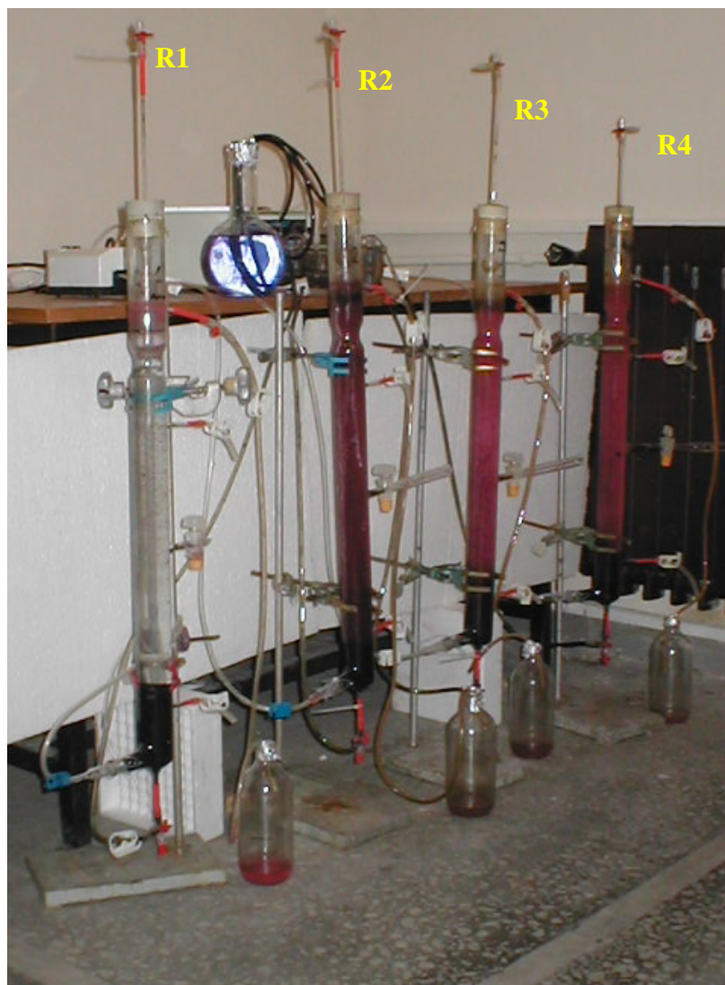
Figure 4.13. The set-up of the USB reactors conducted for study 3.
