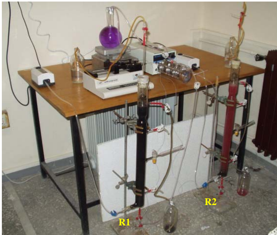
Figure 4.8. Two USB reactors operated in the temperature-controlled room.
