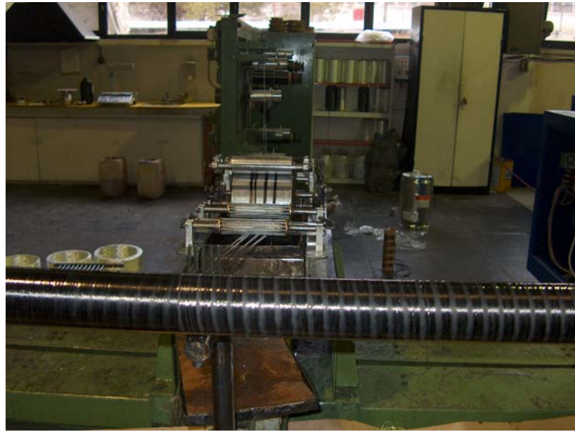
Figure 3.5 Three axial computer controlled Bolenz&Scafer filament winding machine.
