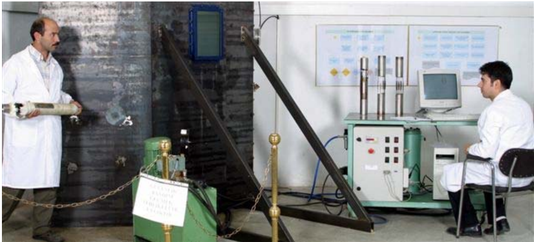
Figure 3.2 Internal pressure test system.
