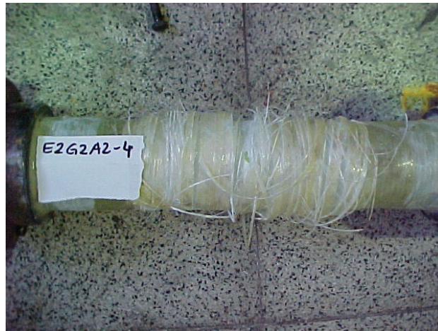
Figure 5.22. Failed glass fiber reinforced tube of [\pm 45^\circ]_2 [90^\circ]_1 winding configuration.
