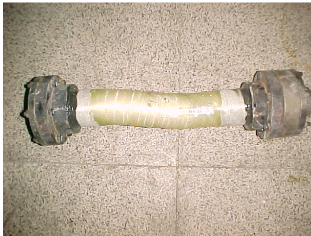
Figure 5.25. Failed glass fiber reinforced tube of [\pm 65^\circ]_3 [90^\circ]_1 winding configuration.
