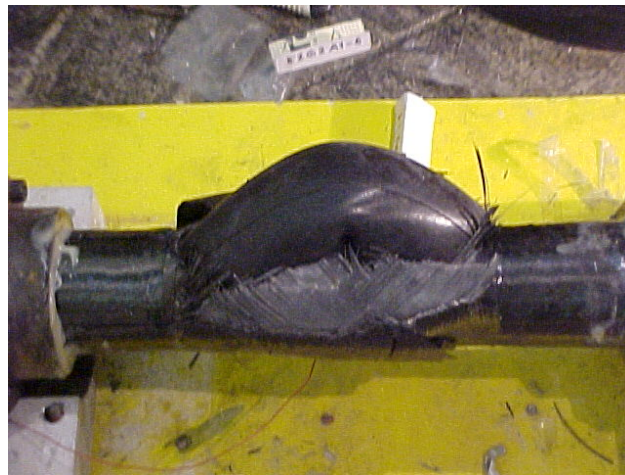
Figure 5.21. Failed carbon fiber reinforced tube of [\pm 45^\circ]_3 [90^\circ]_1 winding configuration.
