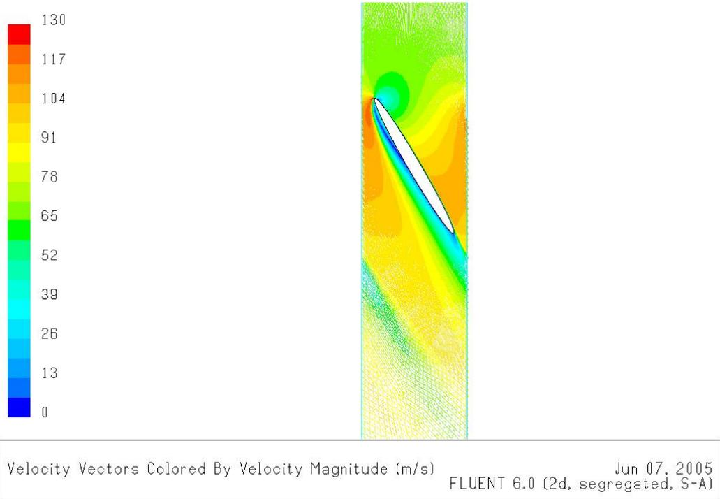
**Figure 2.14:** Velocity vectors of the overall field ( $\sigma = 1.5$ ,  $i=30^\circ$ ,  $V=70$  m/s)
