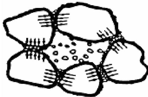
**Figure 2.1.** Structure of Collapsible Soils (Loaded Structure before Inundation)
