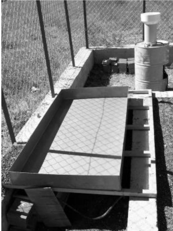
Figure 2.12 Installed snowmelt lysimeter at Güzelyayla station
