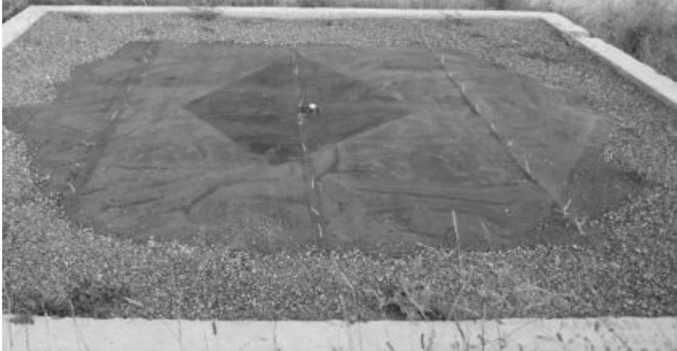
Figure 2.10 Installed snow pillow at Güzelyayla station
