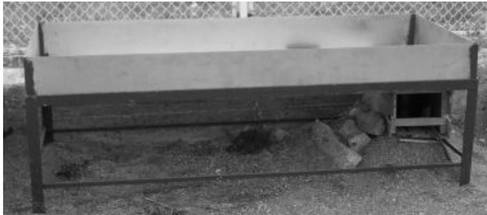
Figure 2.15 Snowmelt lysimeter installed at Ovacık station
