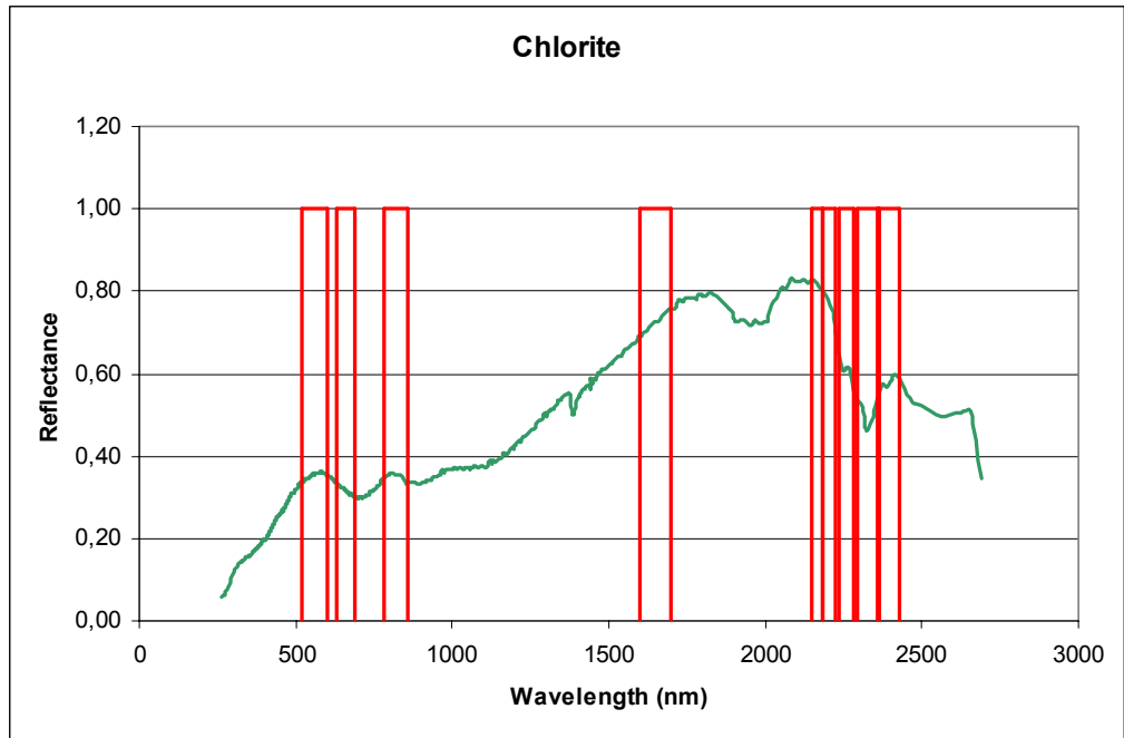
Figure 5.10. USGS spectral reflectance curve of chlorite.
