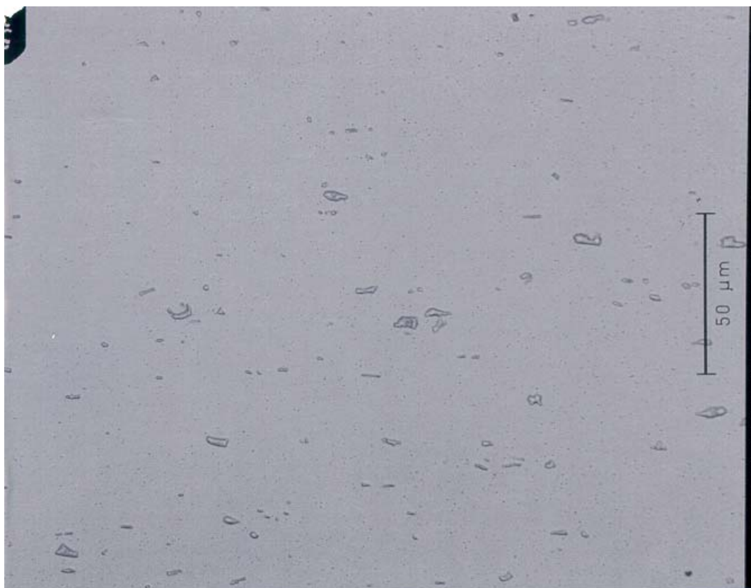
Figure C.1: Longitudinal section at the t/2 location for 6111-T4 sample 786052 in the etched condition (Graff-Sergeant) showing constituent and dispersoid particle distributions (500X)
