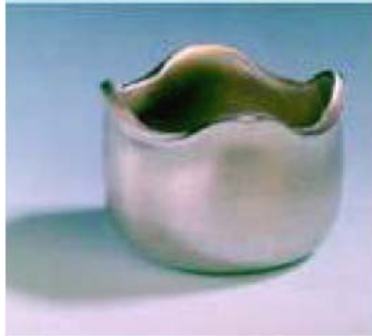
Figure 2.3: Earing in a deep drawn cup (Tekkaya, 2003)
