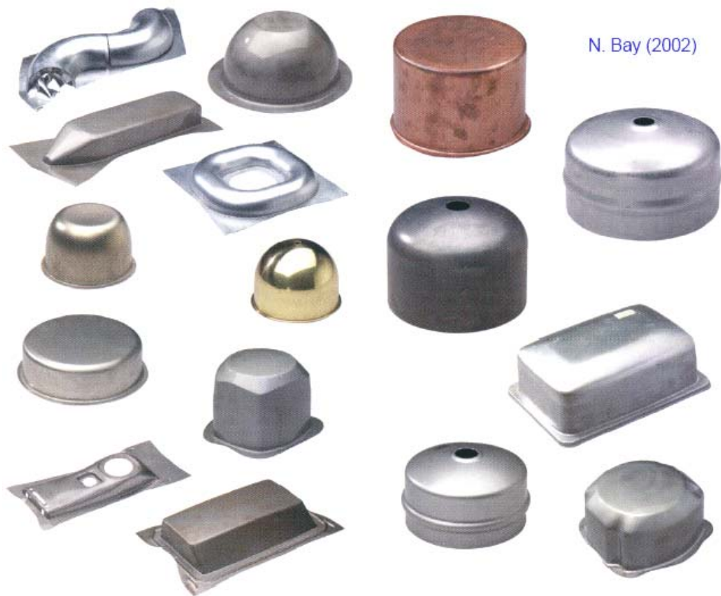
Figure 3.2: Examples of deep drawing (Tekkaya, 2002)
