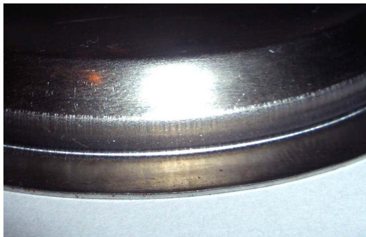
Figure 6.5: Ironing marks at the side of the workpiece
