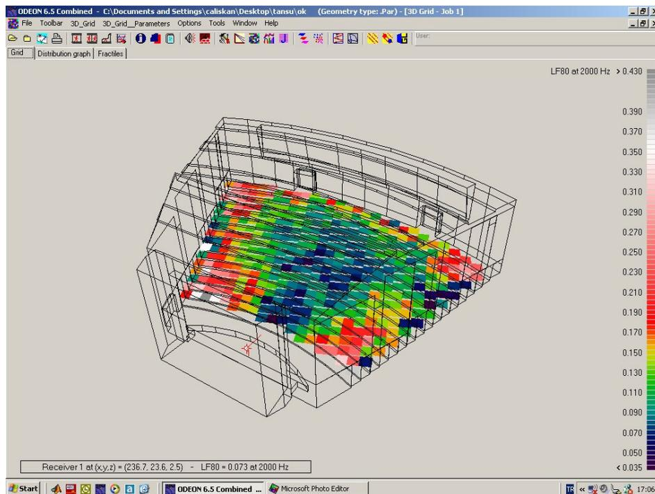
**Figure 74:** Lateral Fraction (LF80) at 2000Hz in auditorium mode.
