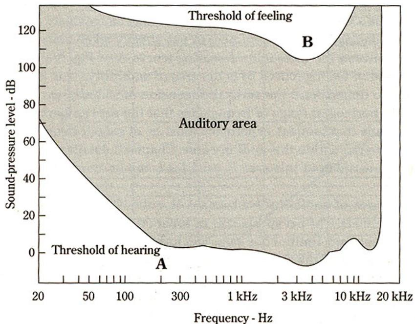
**Figure 11:**“The auditory area of the human ear is bounded by two threshold curves, (A) the threshold of hearing delineating the lowest level sounds the ear can detect, and (B) the threshold of feeling at the upper extreme. All of our auditory experiences occur within this area.” (Everest, 2001)
