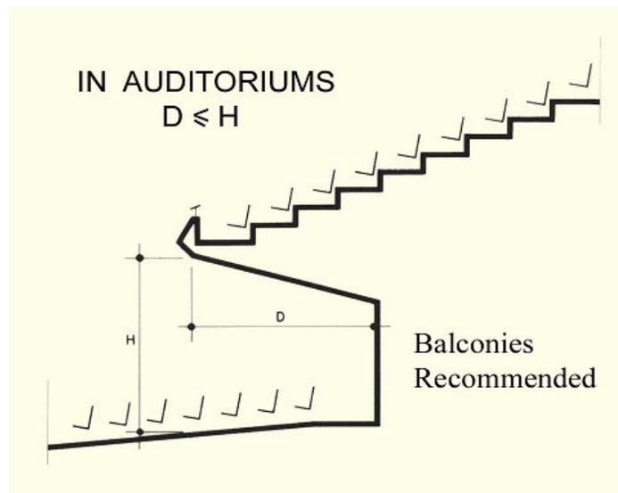
**Figure 15:** Balconies or overhangs recommended in the design stage of a hall to prevent sound shadows (Doelle, 1972).
