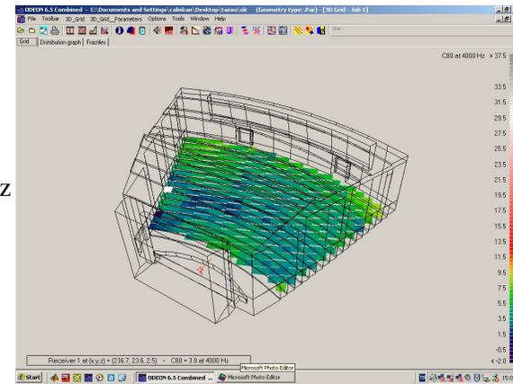
Fig C4: Clarity Index (C80) of NCCA in concert mode at 125Hz, 500Hz, 1000Hz and 4000 Hz.
