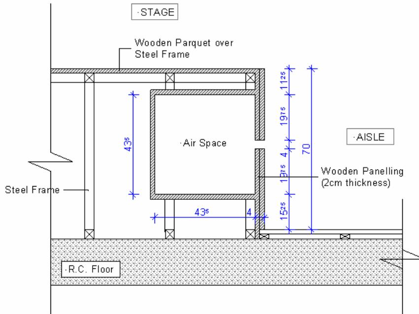
**Figure 98:** Detailed section of the volume resonator constructed on the surface of the stage front.
