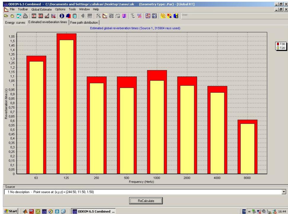
**Figure 57:** Global reverberation times in auditorium mode.(Fully occupied)
