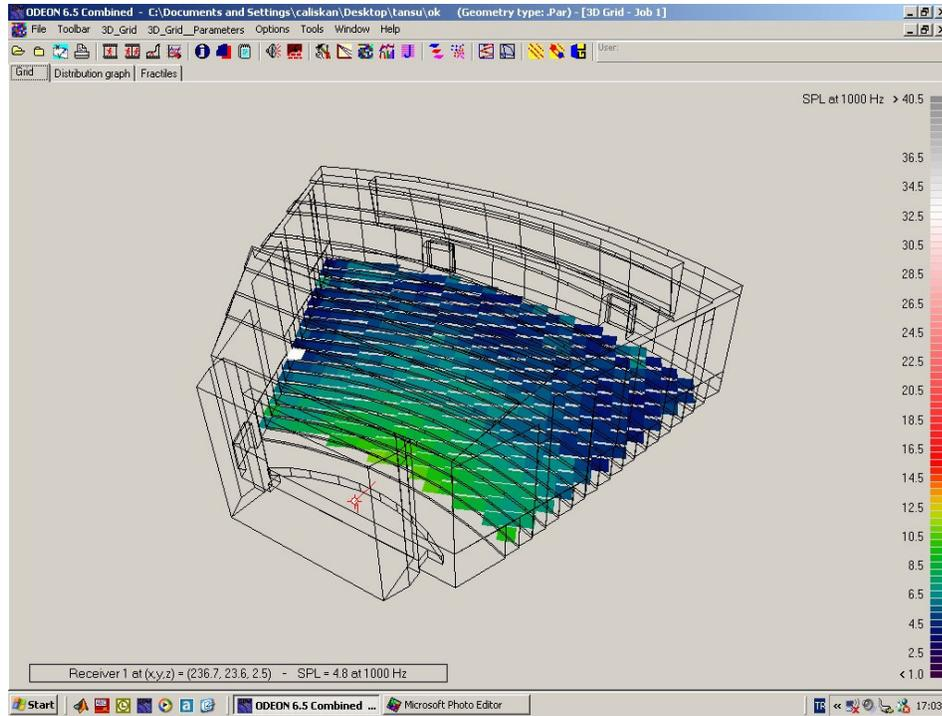
**Figure 60:** Sound Pressure Levels (SPL) at 1000Hz in auditorium mode.(Fully occupied)
