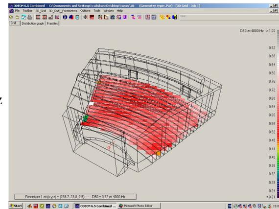
**Fig C5:** Definition Index (D50) of NCCA in concert mode at 125Hz, 500Hz, 1000Hz and 4000 Hz.
