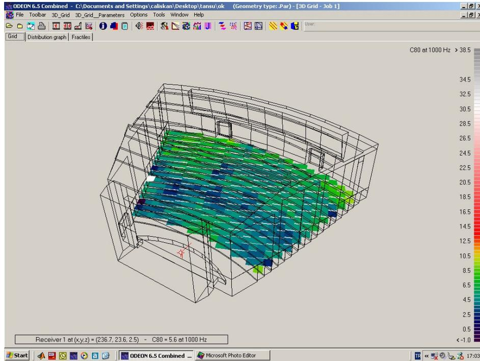
**Figure 67:** Clarity index at 1000Hz in auditorium mode.(Fully occupied)
