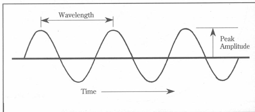
**Figure 9:** Wavelength is the distance a wave travels in the time it takes to complete one cycle. (Everest, 2000)
