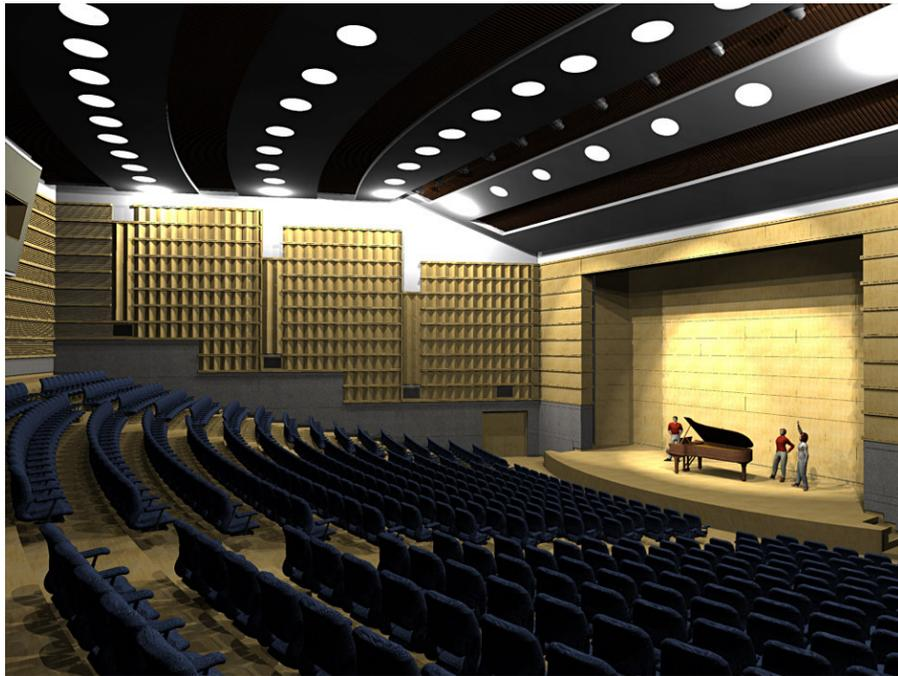
**Figure 41:** Interior perspective render of wooden panels are folded on highly absorptive material for the concert mode. (By Ilhan S. Kural)
