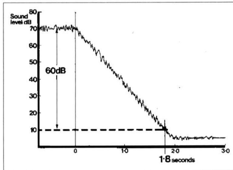
**Figure 27:** Reverberation time definition with sample decay.
