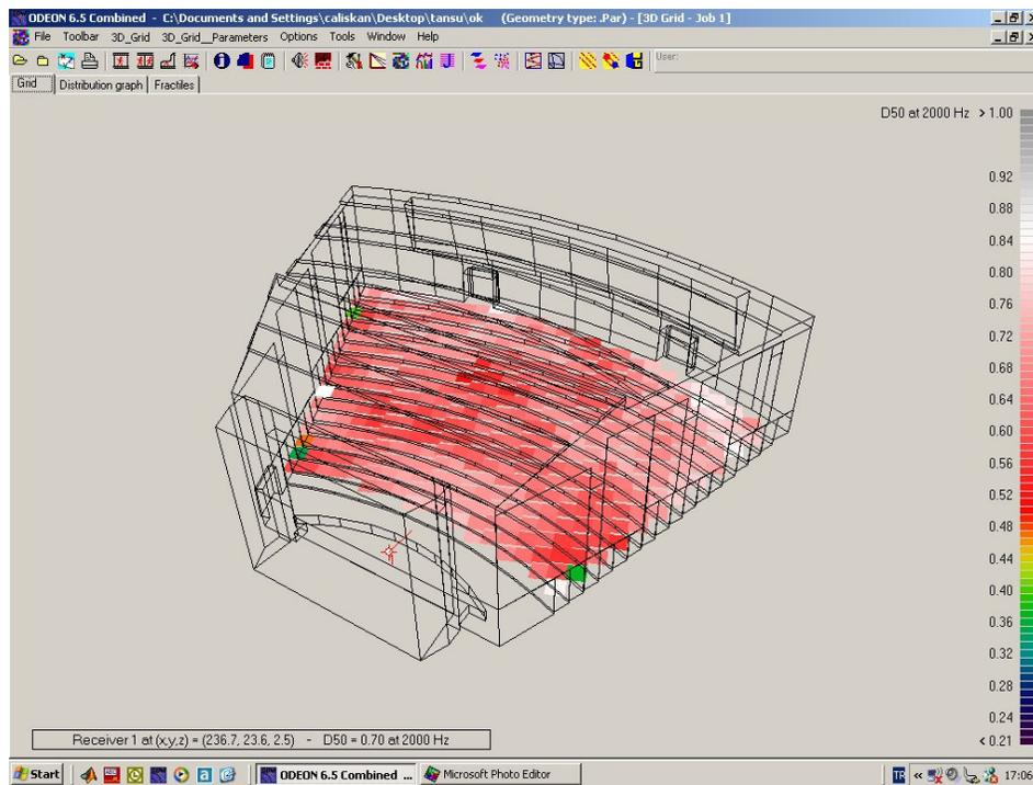
**Figure 71:** Definition index at 2000Hz in auditorium mode.(Fully occupied)
