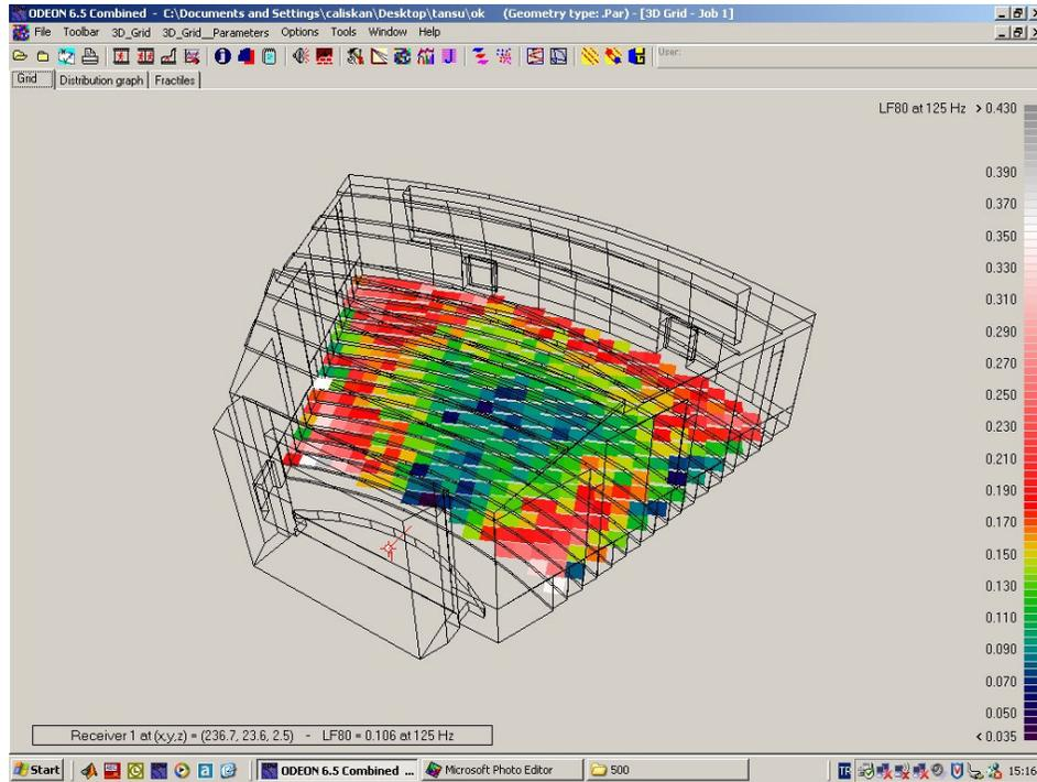
**Figure 93:** Lateral Fraction (LF80) at 125Hz in concert mode.
