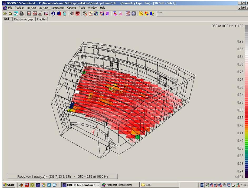
**Figure 91:** Definition index at 1000Hz in concert mode.(Fully occupied)
