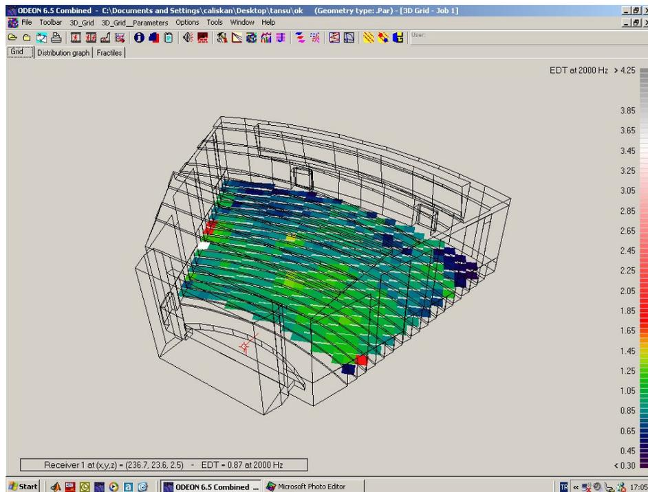
**Figure 65:** Early Decay Time (EDT) at 2000Hz in auditorium mode.
