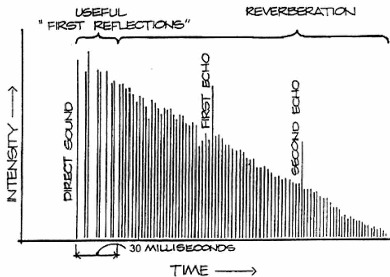
**Figure 25:** The intensity graph of direct sound and reflections with respect to time (Irwine & Richards, 1998).
