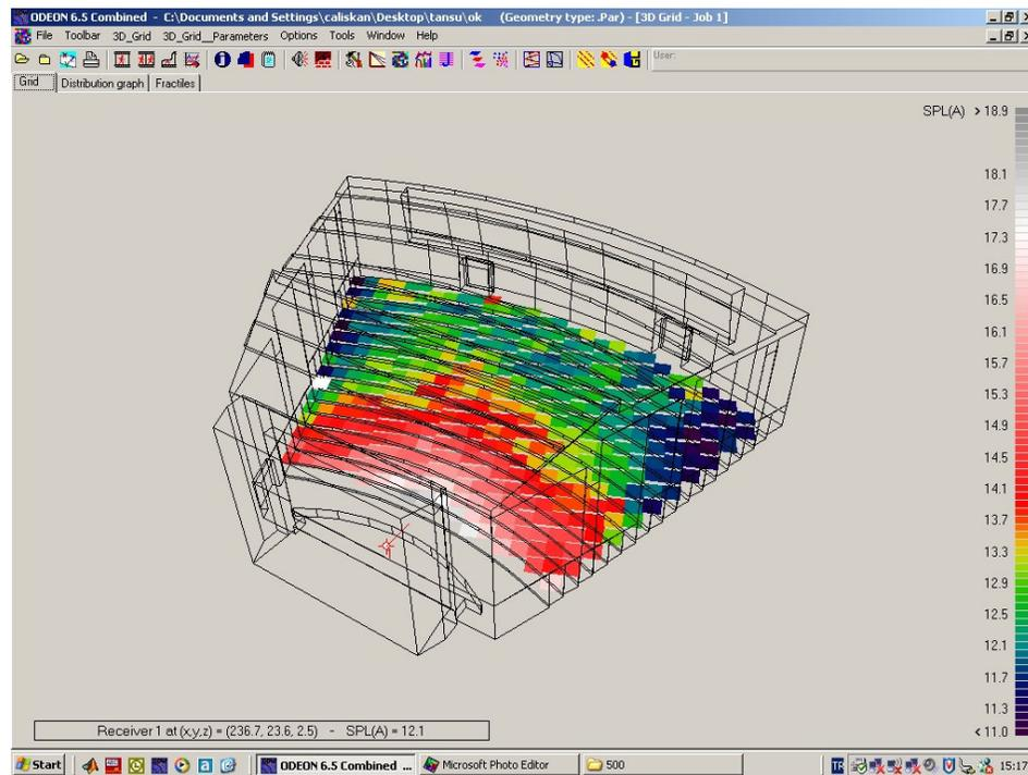
**Figure 83:** Sound Pressure Level (SPL(A)) (A-weighted) in concert mode.(Fully occupied)
