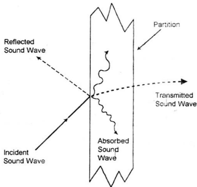
**Figure 18:** Reflection of a sound wave to interaction with a partition
