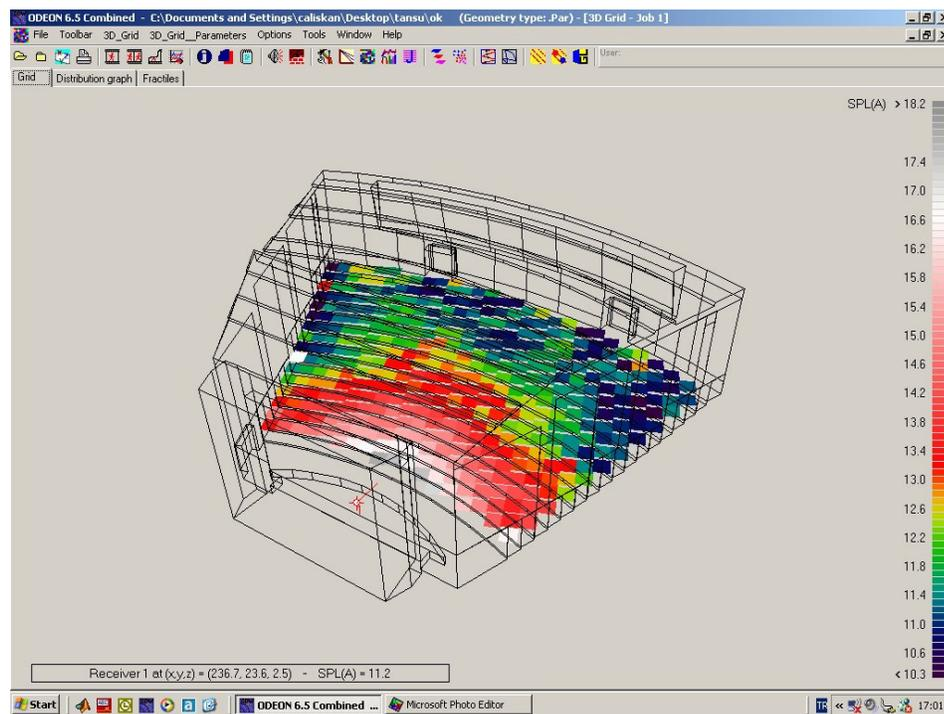
**Figure 62:** Sound Pressure Level (SPL(A)) (A-weighted) in auditorium mode.(Fully occupied)
