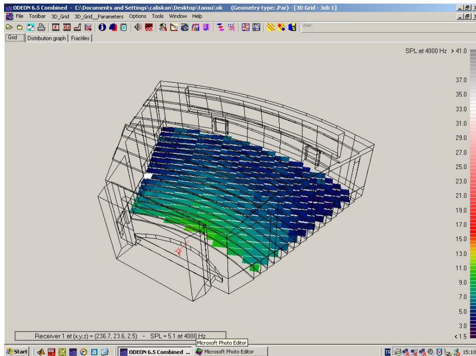
**Figure 82:** Sound Pressure Levels (SPL) at 4000Hz in concert mode.(Fully occupied)
