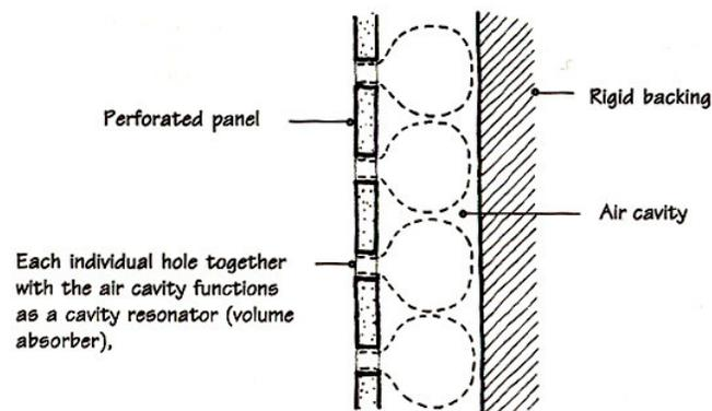
**Figure 19:** A perforated panel as an absorber (Everest, 2000).
