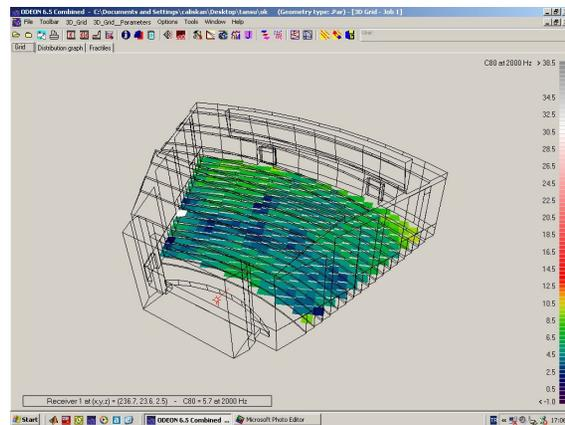
**Fig B4:** Clarity Index (C80) of NCCA in auditorium mode at 125Hz, 500Hz, 1000Hz and 2000 Hz.
