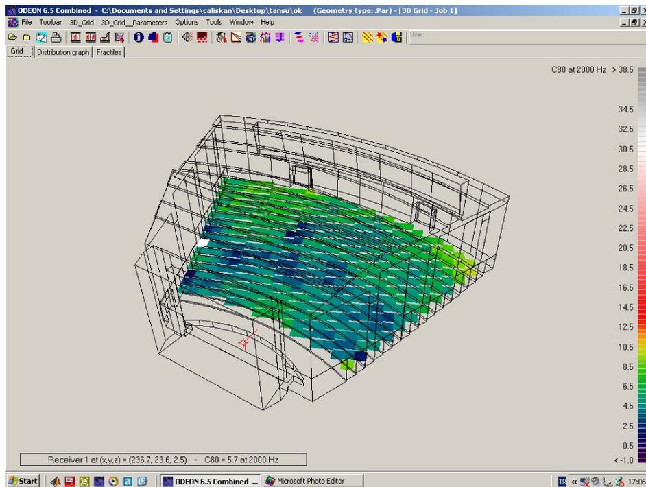
**Figure 68:** Clarity index at 2000Hz in auditorium mode.(Fully occupied)
