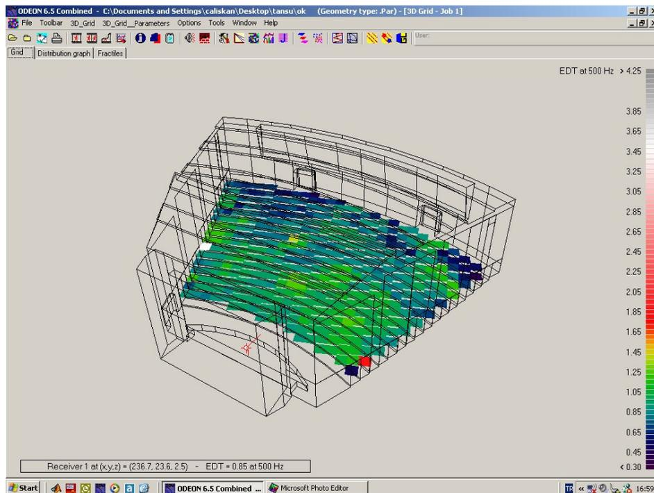
**Figure 63:** Early Decay Time (EDT) at 500Hz in auditorium mode.
