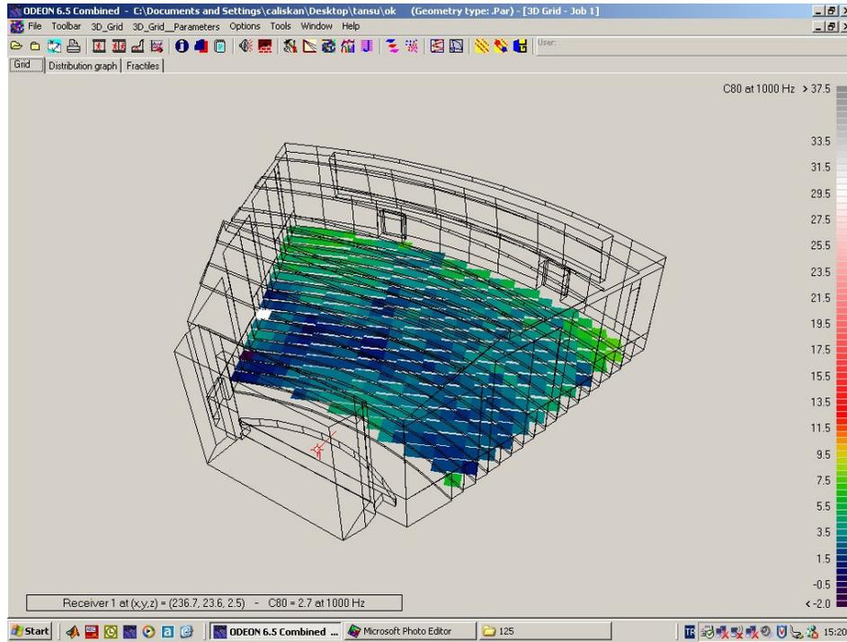
**Figure 88:** Clarity index at 1000Hz in concert mode.(Fully occupied)
