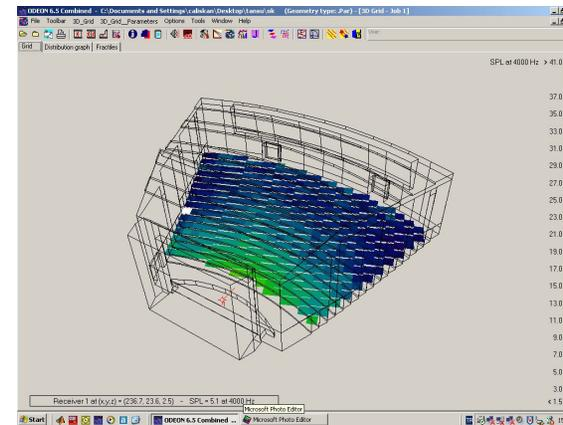
**Fig C1:** Sound Pressure Levels (SPL) of NCCA in concert mode at 125Hz, 500Hz, 1000Hz and 4000 Hz.
