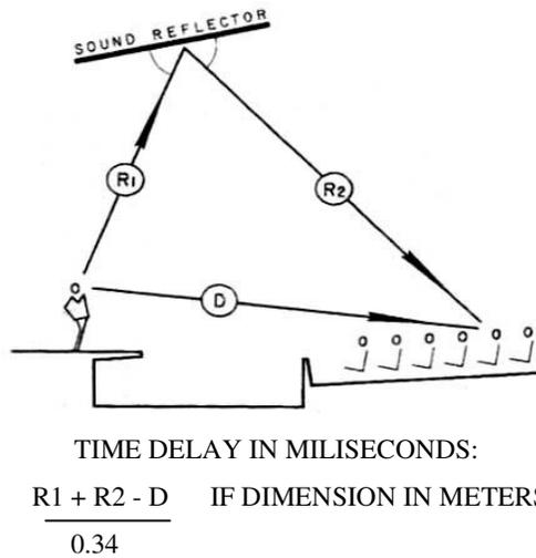
**Figure 26:** Reflected sound beneficially reinforces the direct sound if the time delay between them is relatively short, that is, a maximum of 30 ms (Doelle 1972).
