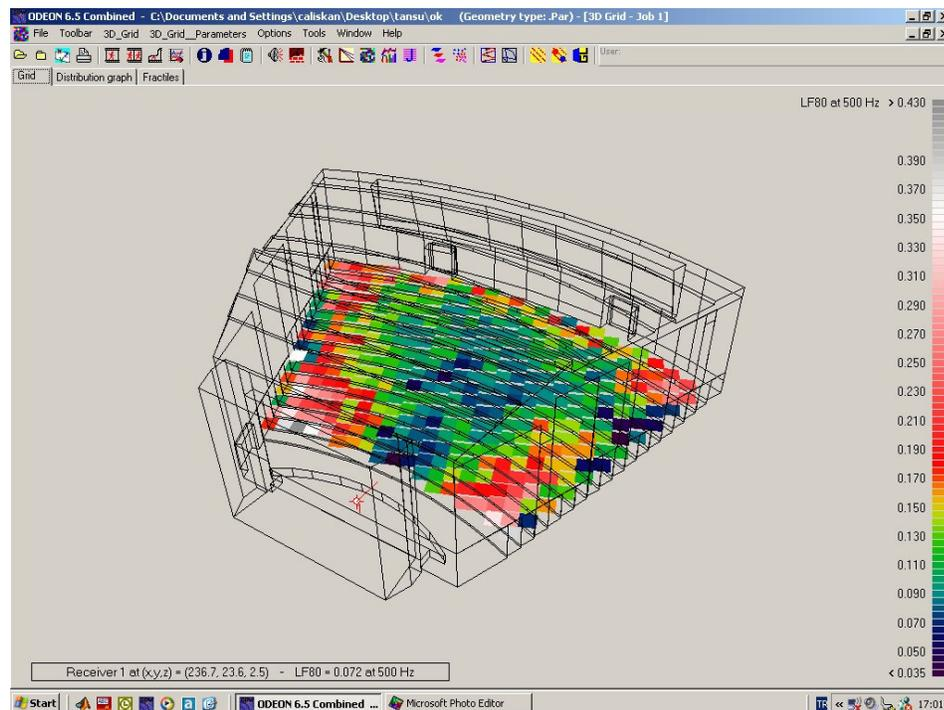
**Figure 72:** Lateral Fraction (LF80) at 500Hz in auditorium mode.
