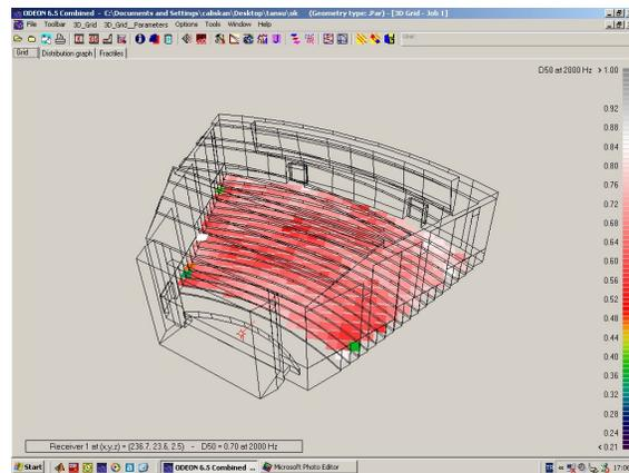
**Fig B5:** Definition Index (D50) of NCCA in auditorium mode at 125Hz, 500Hz, 1000Hz and 2000 Hz.
