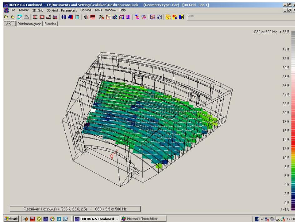
**Figure 66:** Clarity index at 500Hz in auditorium mode.(Fully occupied)
