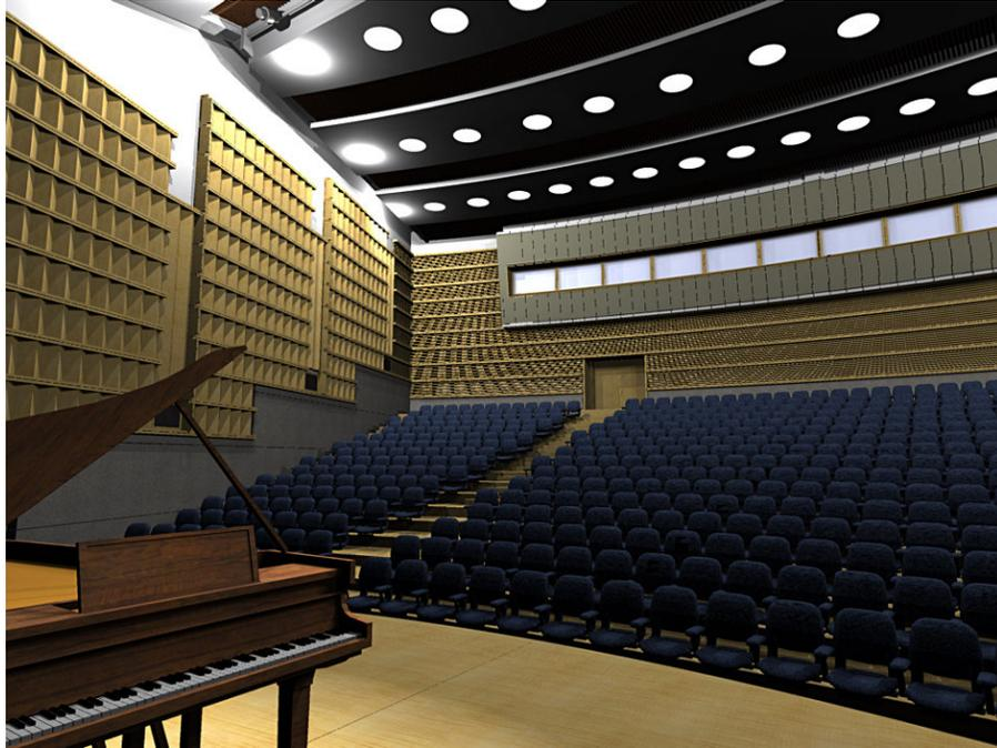
**Figure 40:** Interior render of wooden panels are folded on highly absorptive material for the concert mode. (By Ilhan S. Kural)
