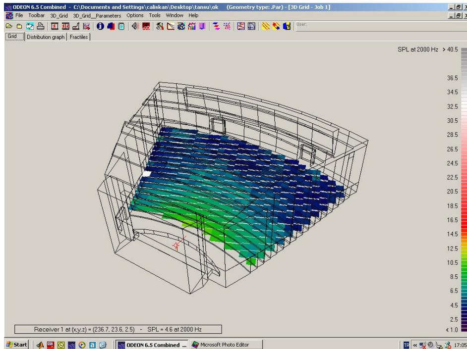
**Figure 61:** Sound Pressure Levels (SPL) at 2000Hz in auditorium mode.(Fully occupied)
