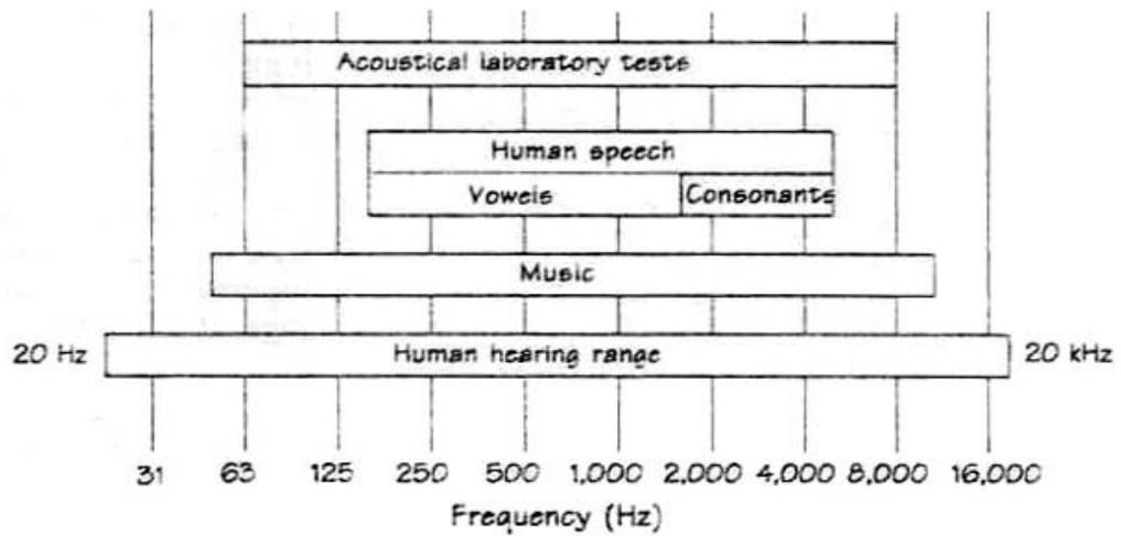
**Figure 10:** Octave bands and frequency ranges of acoustical laboratory tests, human speech, and music (Mehta, Johnson & Rocafort 1999).
