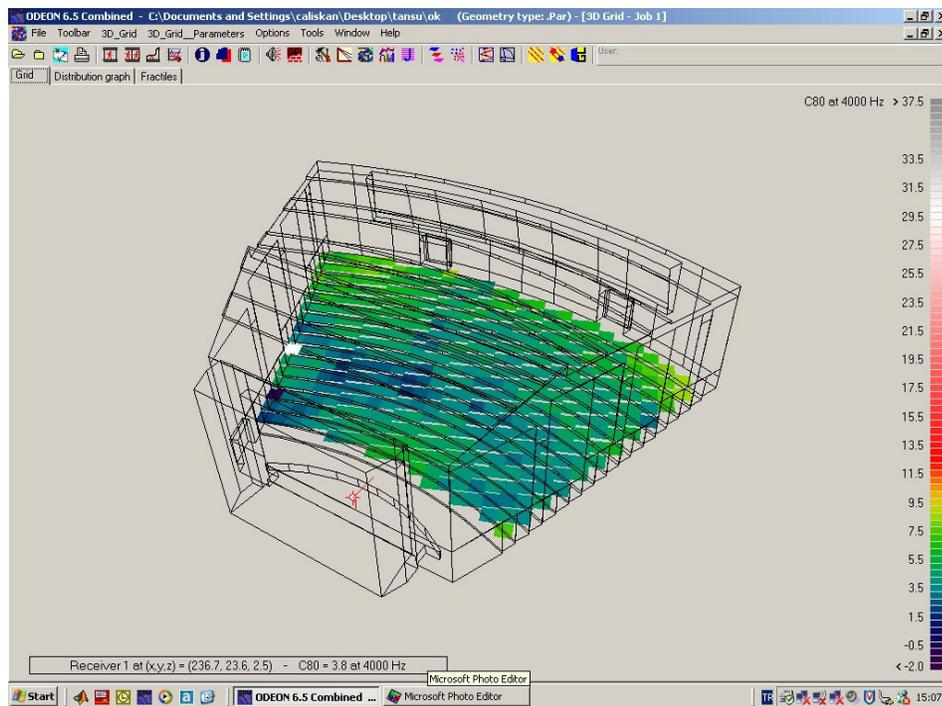
**Figure 89:** Clarity index at 4000Hz in concert mode.(Fully occupied)
