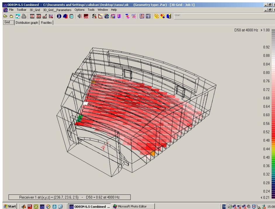
**Figure 92:** Definition index at 4000Hz in concert mode.(Fully occupied)
