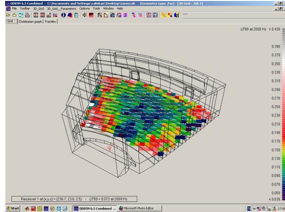
**Fig B6:** Lateral Fraction (LF80) of NCCA in auditorium mode at 125Hz, 500Hz, 1000Hz and 2000 Hz.
