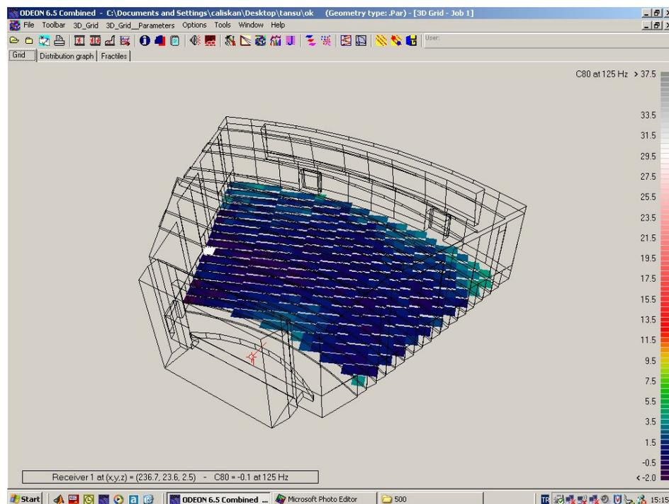
**Figure 87:** Clarity index at 125Hz in concert mode.(Fully occupied)
