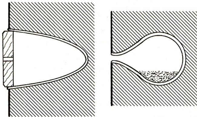
**Figure 20:** Pots embedded inside of those walls in Sweden and Denmark served as Helmholtz resonators (Everest, 2001).
