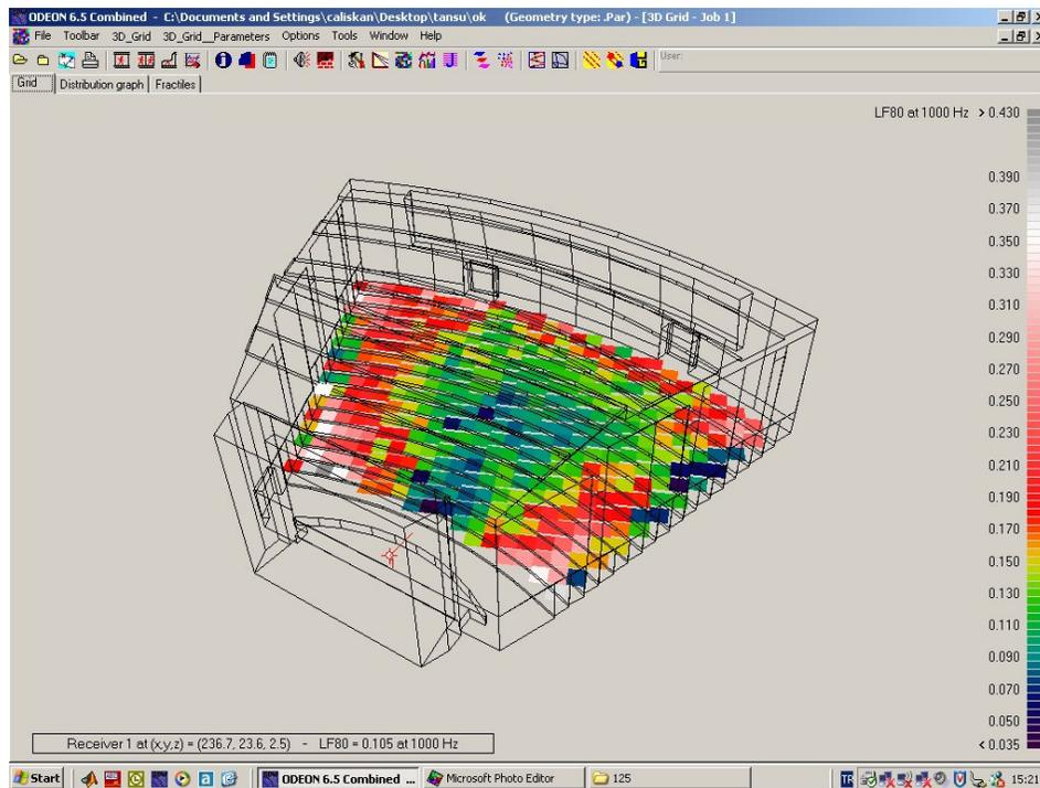
**Figure 94:** Lateral Fraction (LF80) at 1000Hz in concert mode.
