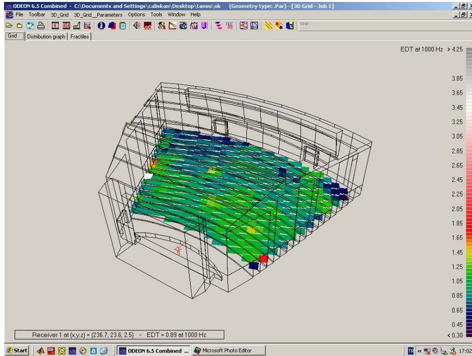
**Figure 64:** Early Decay Time (EDT) at 1000Hz in auditorium mode.
