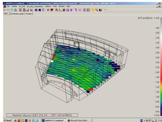
**Fig B3:** Early Decay Time (EDT) of NCCA in auditorium mode at 125Hz, 500Hz, 1000Hz and 2000 Hz.
