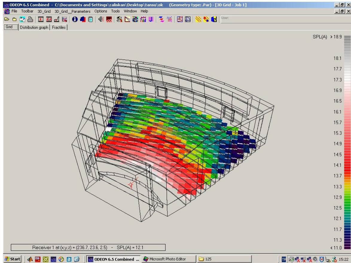
**Fig C2:** A-Weighted Sound Pressure Level (SPLA) of NCCA in concert mode.
