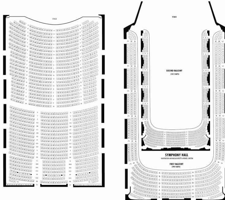
**Figure 3:** Seating plan of Boston Symphony Hall (1900); as a classical rectangular hall, first floor plan (left), second floor plan (right)[37]
