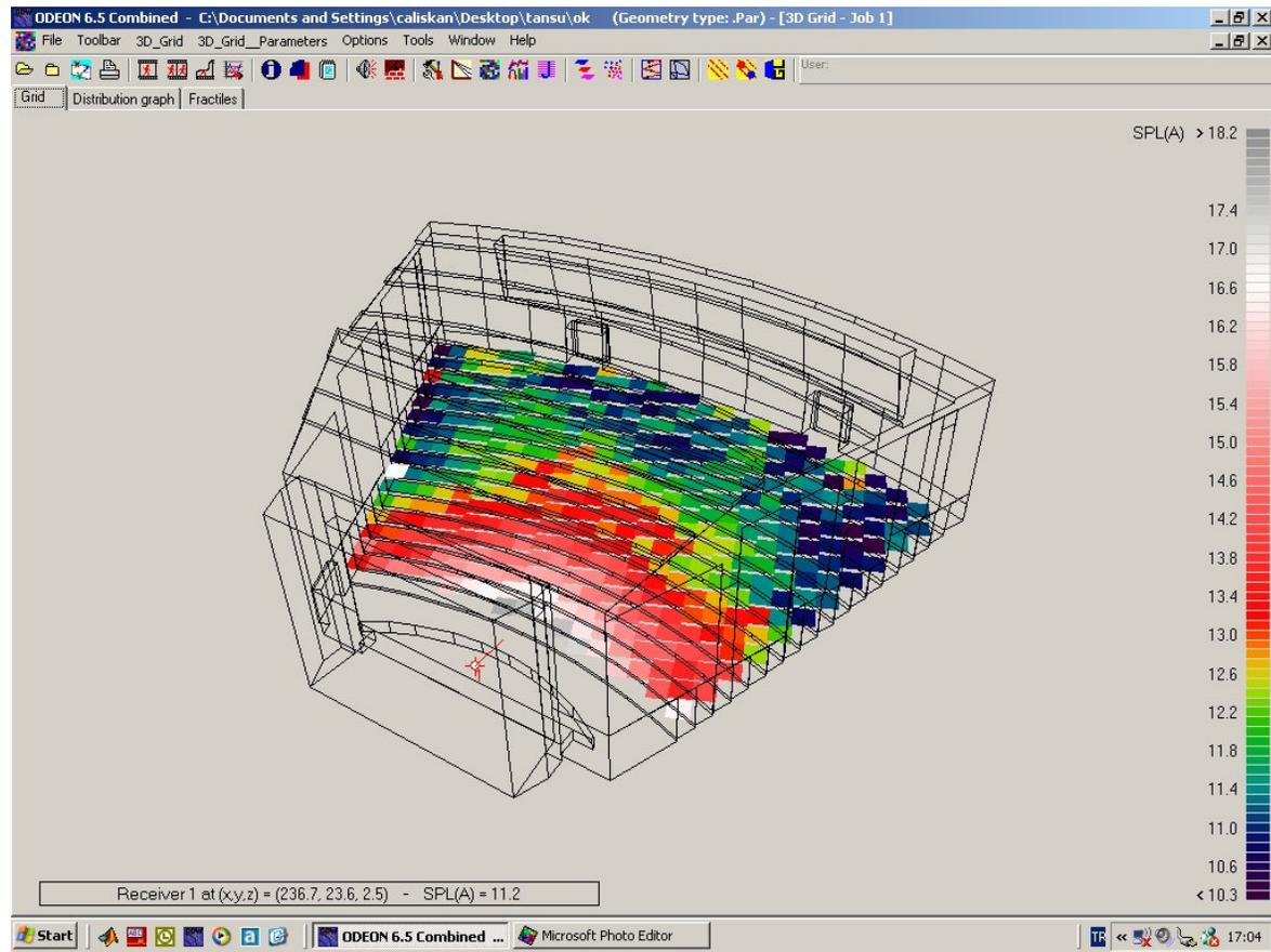
**Fig B2:** A-Weighted Sound Pressure Level (SPLA) of NCCA in auditorium mode.
