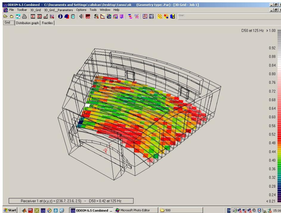
**Figure 90:** Definition index at 125Hz in concert mode.(Fully occupied)
