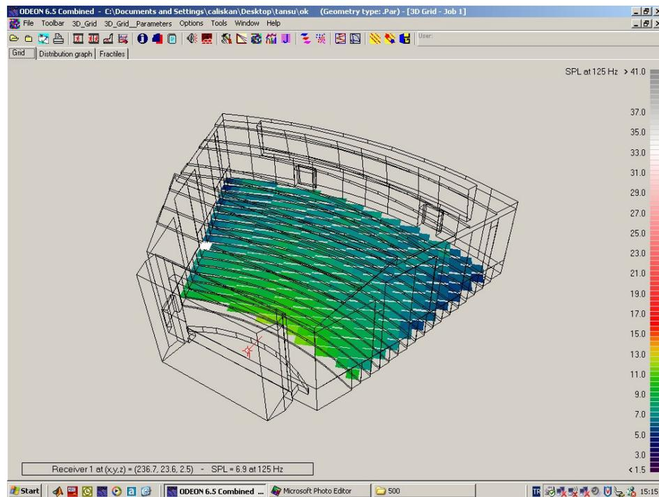
**Figure 80:** Sound Pressure Levels (SPL) at 125Hz in concert mode.(Fully occupied)
