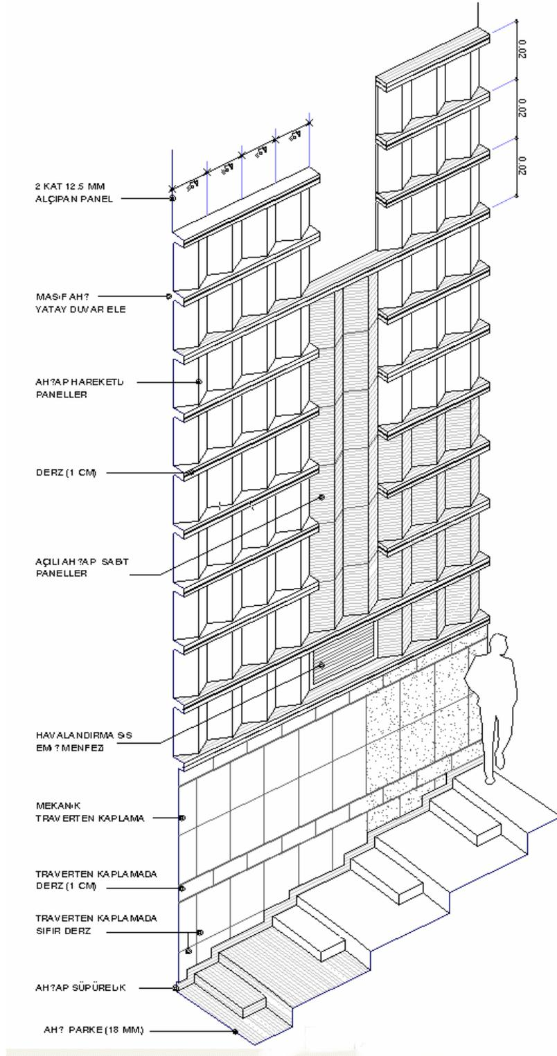
**Figure 39:** Wooden panels are folded on highly absorptive material for the concert mode. (Design by Ilhan S. Kural, drawn by Oya Caymaz)
