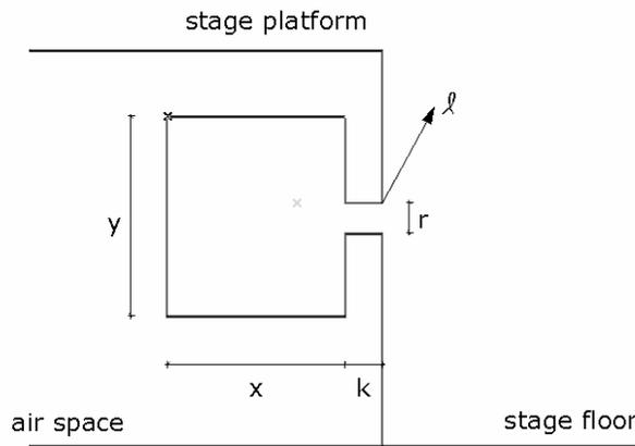
**Figure 97:** Section of the volume resonator constructed on the surface of the stage front.
