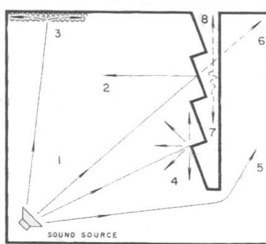
**Figure 17:** Behavior of sound in an enclosed space.(1) Incident or direct sound; (2) reflected sound; (3) sound absorbed by surface treatment; (4) diffused or dispersed sound; (5) diffracted or bent sound; (6) transmitted sound; (7) sound dissipated within the structure; (8) sound conducted by the structure (Doelle1972).
