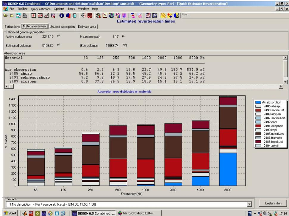
Figure 52: Material absorption areas in auditorium mode.(Fully occupied)
