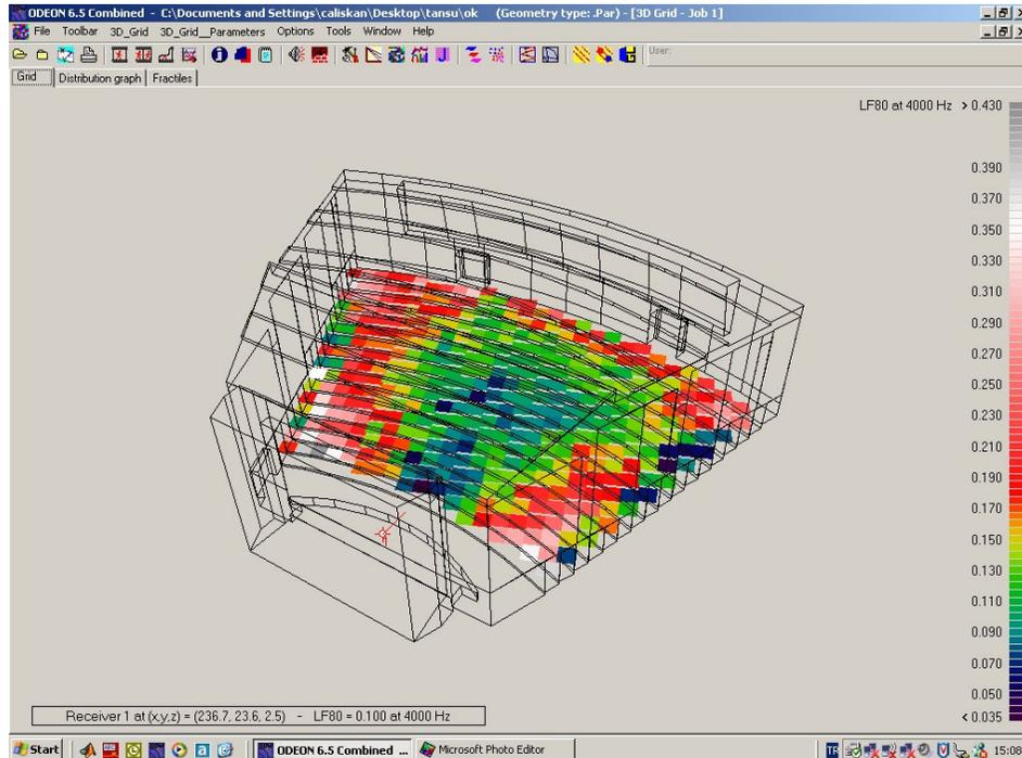
**Figure 95:** Lateral Fraction (LF80) at 4000Hz in concert mode.
