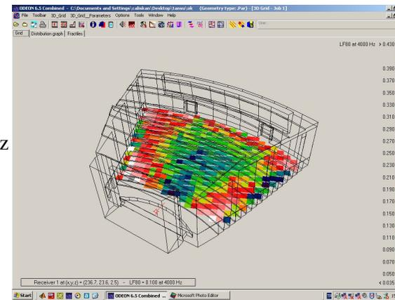
**Fig C6:** Lateral Fraction (LF80) of NCCA in concert mode at 125Hz, 500Hz, 1000Hz and 4000 Hz.
