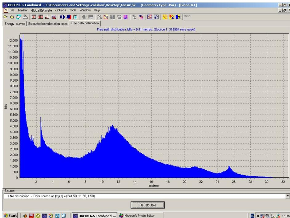
**Figure 58:** Free path distribution in auditorium mode.(Fully occupied)
