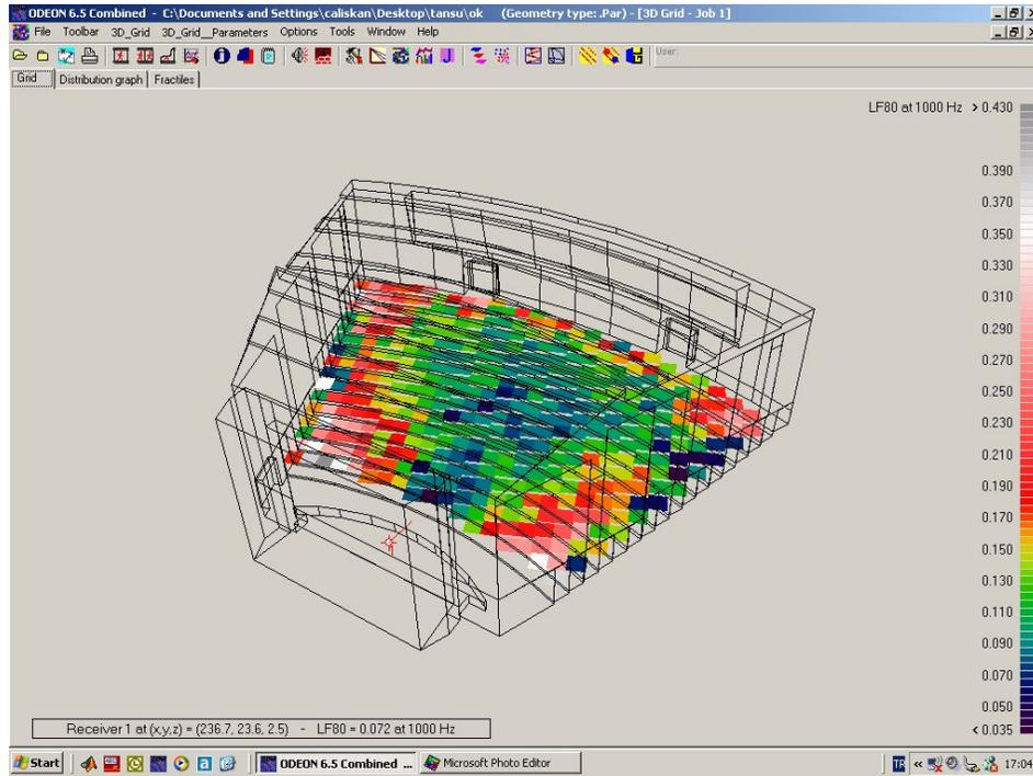
**Figure 73:** Lateral Fraction (LF80) at 1000Hz in auditorium mode.
