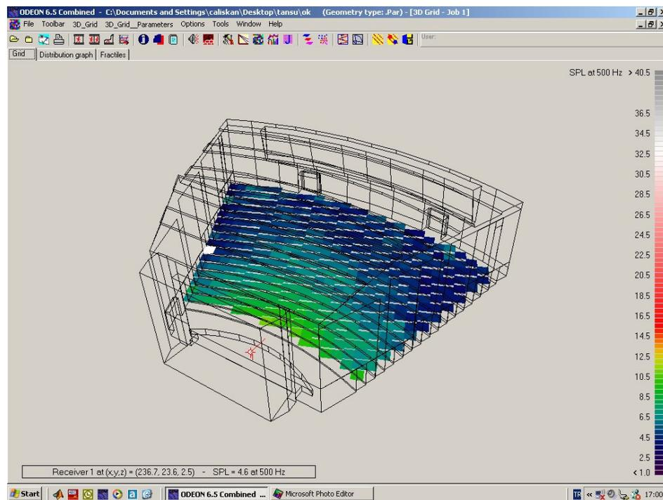
**Figure 59:** Sound Pressure Levels (SPL) at 500Hz in auditoriummode.
