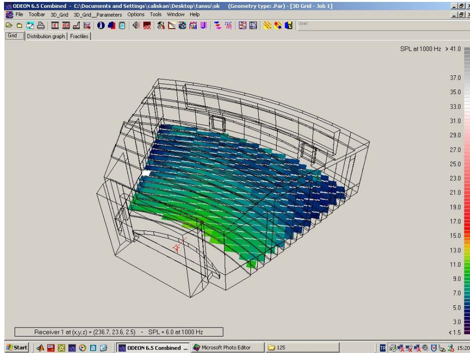
**Figure 81:** Sound Pressure Levels (SPL) at 1000Hz in concert mode.(Fully occupied)
