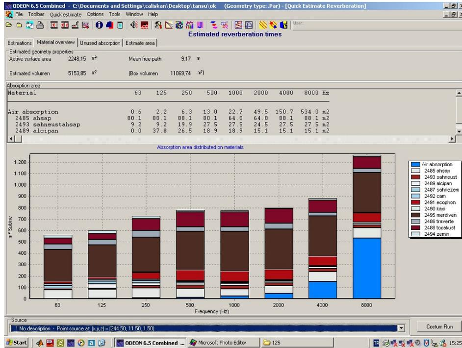
Figure 76: Material absorption areas in concert mode.(Fully occupied)
