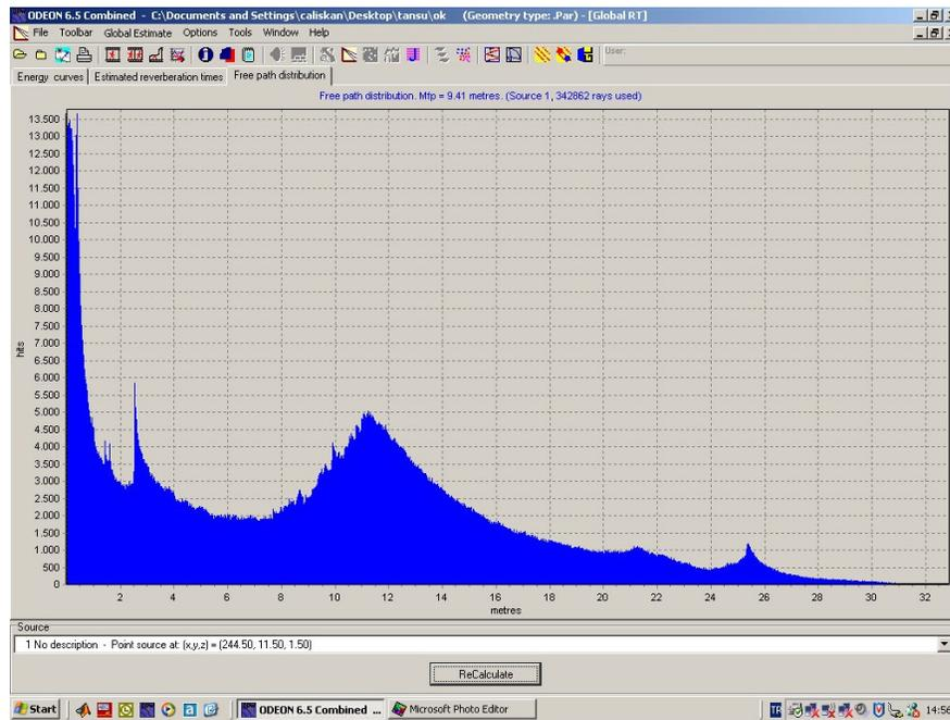
**Figure 79:** Free path distribution in concert mode.(Fully occupied)
