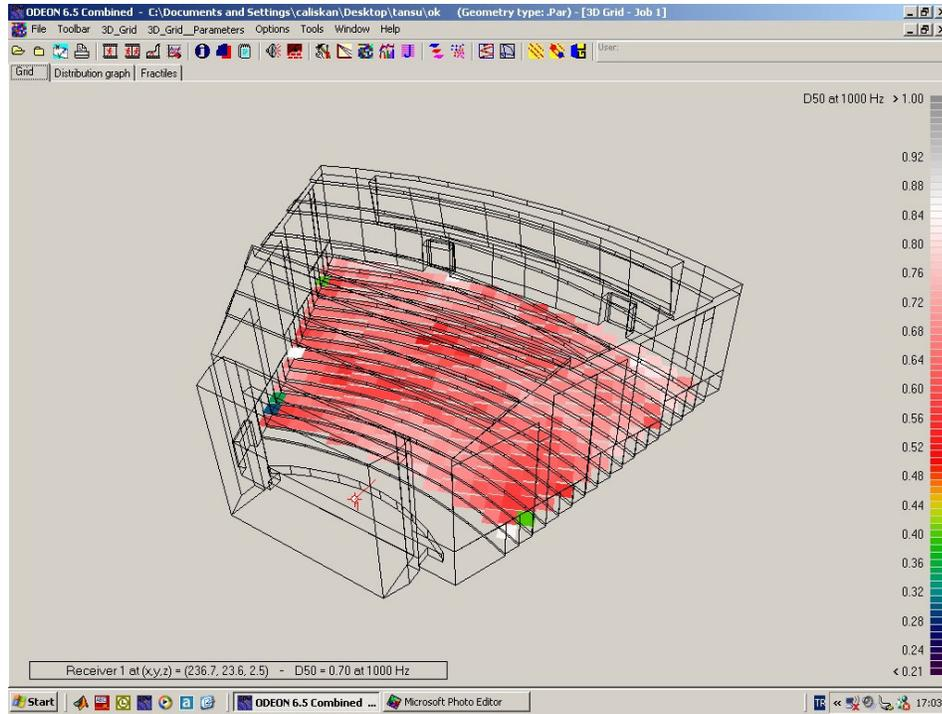
**Figure 70:** Definition index at 1000Hz in auditorium mode.(Fully occupied)
