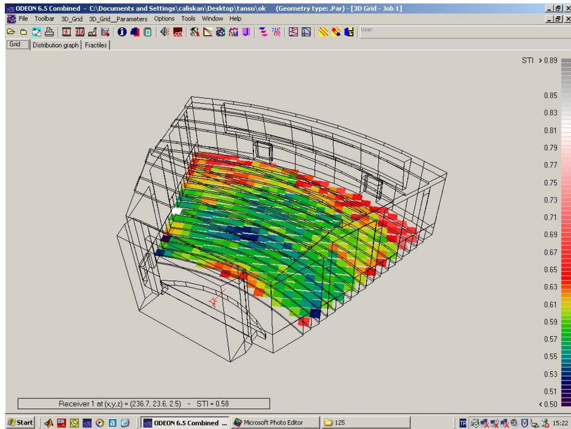
**Fig C7:** Sound Transmission Index (STI) of NCCA in concert mode at 125Hz, 500Hz, 1000Hz and 4000 Hz.
