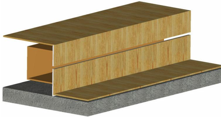
**Figure 99:** Perspective view of the volume resonator constructed on the surface of the stage front.
