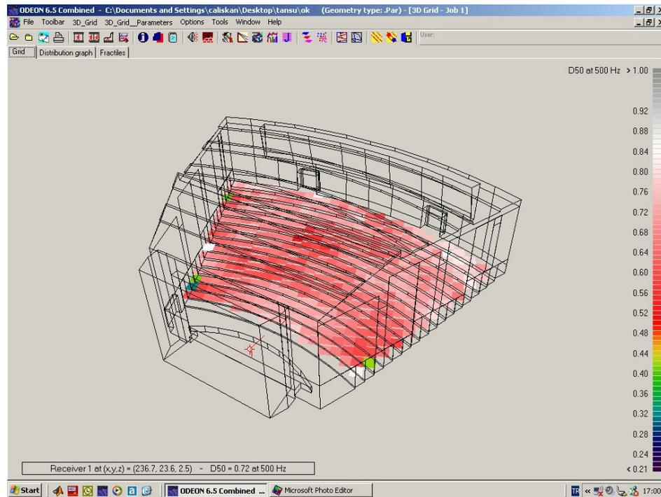
**Figure 69:** Definition index at 500Hz in auditorium mode.(Fully occupied)
