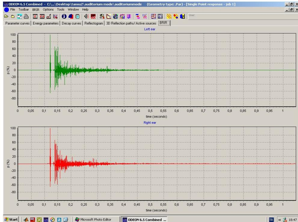
**Figure 55:** Binaural Impulse Response of the receiver at 20m.
