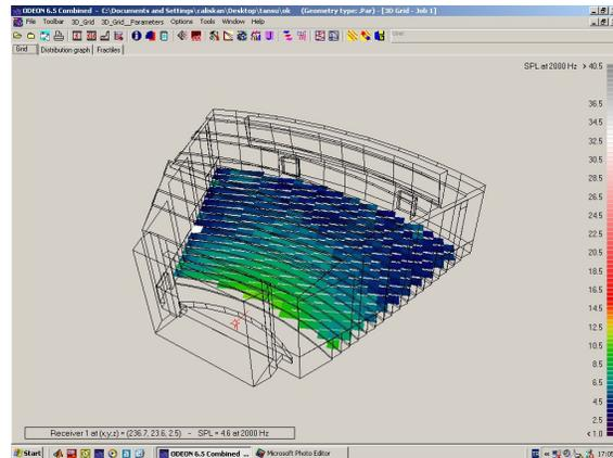
**Fig B1:** Sound Pressure Levels (SPL) of NCCA in auditorium mode at 125Hz, 500Hz, 1000Hz and 2000 Hz.
