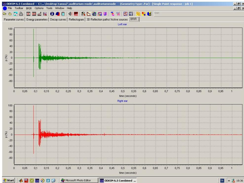
**Figure 54:** Binaural Impulse Response of the receiver at 13m.
