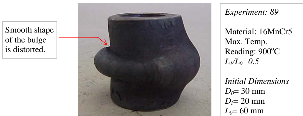
Figure 5.18 The walls above and below the heated portion may interfere into the bulge area. Smoothness of the bulge shape is distorted.
