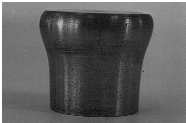
Figure 2.5 Part is heated locally by induction and formed by upsetting [10].
