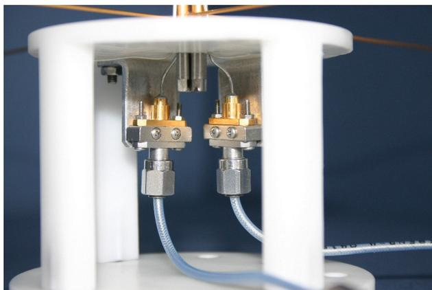
**Figure 6.20** Connectors at the bottom of the antenna
