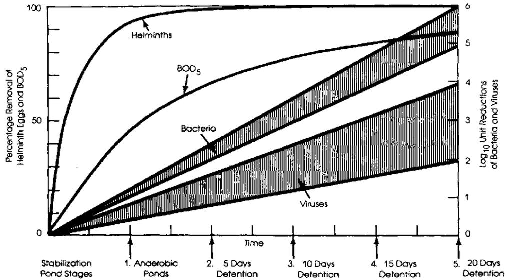
**Figure 1 Generalized removal curves for BOD, helminth eggs, excreted bacteria, and viruses in waste stabilization ponds at temperatures above 20°C, [16]**
