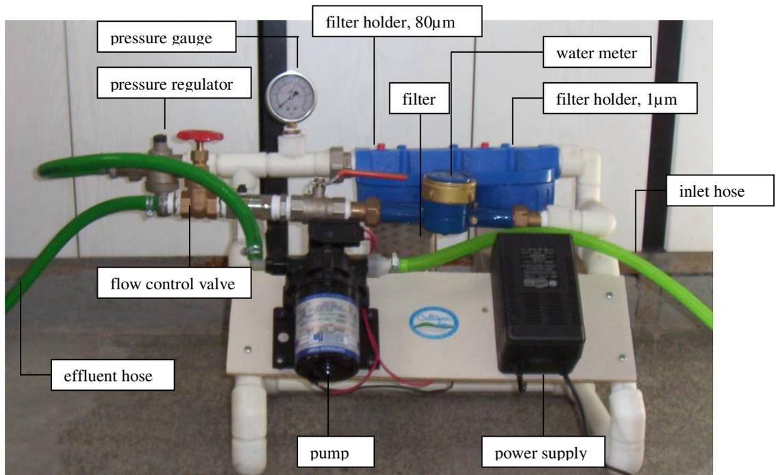
**Figure 4 Apparatus assembled for the concentration of helminth eggs and cysts.**
