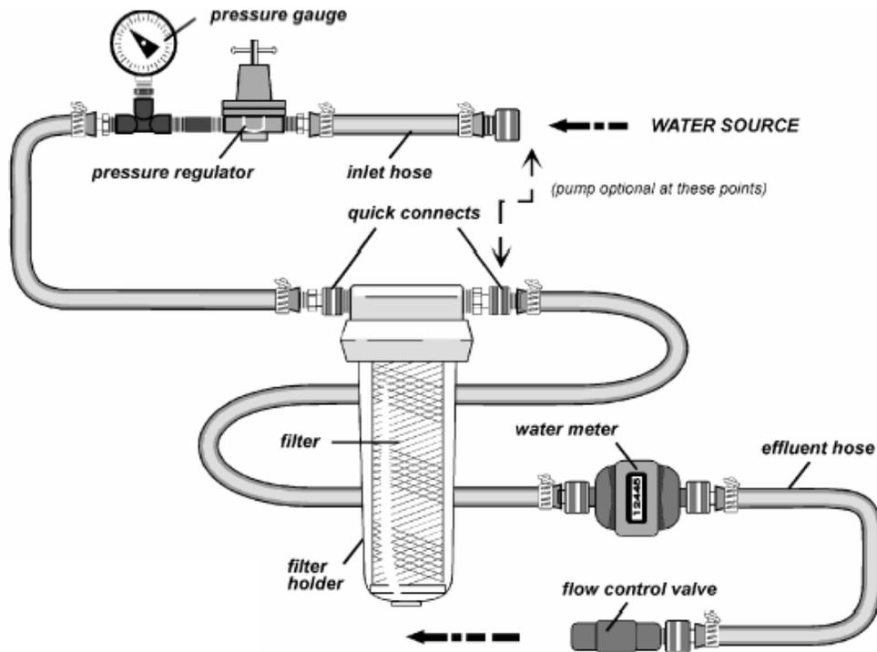
**Figure 3 Apparatus designed for the concentration of parasite eggs and cysts suggested by EPA, [38]**
