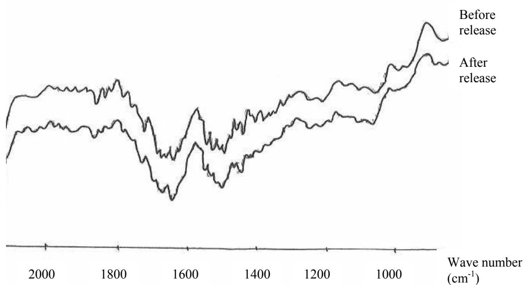
b) IR Spectra of PHBV before and after-release rods (1:1 P:V, prepared by cold paste method).
