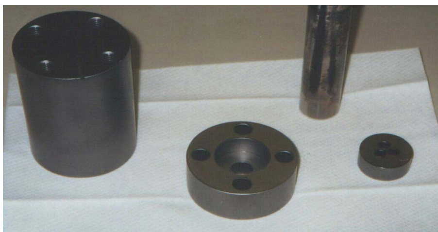
Figure 2.4 Sections of Metal Die Used in Hot Extrusion
