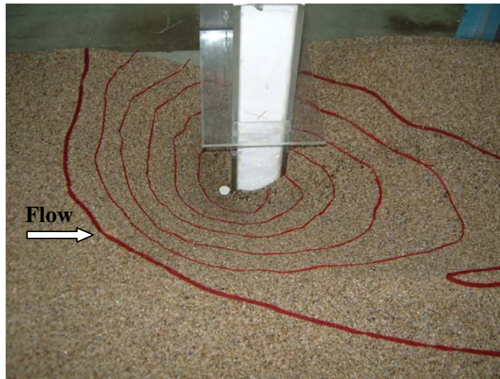
Figure 4.2. A general view of the scour hole when a collar is used (R69, L_a=25 cm, B_c=5 cm, Z_c=+2.5 cm)
