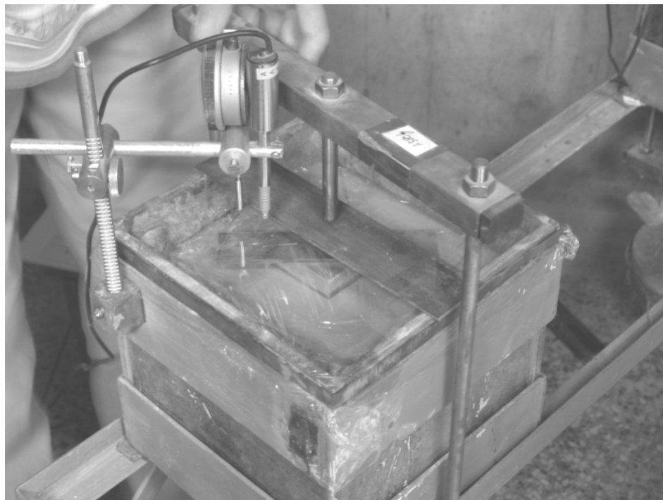
Figure 3.34 Placement of the Load Hanger on the Steel Support (Load is not Applied on the Footing Yet)
