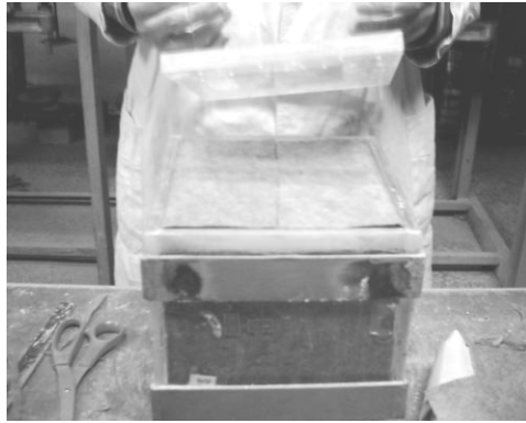
Figure 3.15 Placement of the Plexiglas Cover
