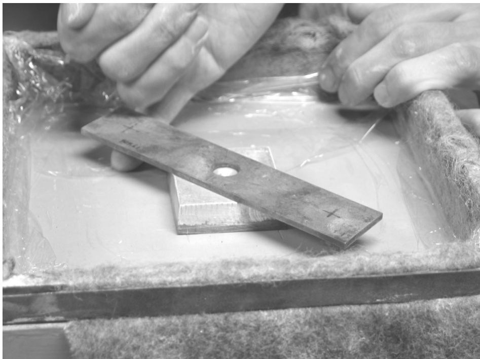
Figure 3.28 Placement of Nylon Sheet around the Footing
