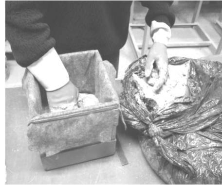
Figure 3.12 Placement of Prepared Soil Manually
