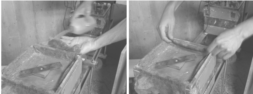
Figure 3.30 Wetting and Rolling of Remaining Portions of Geotextile
