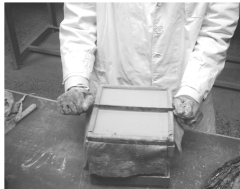
Figure 3.14 Surface Finishing with the Aid of a Special Straightedge
