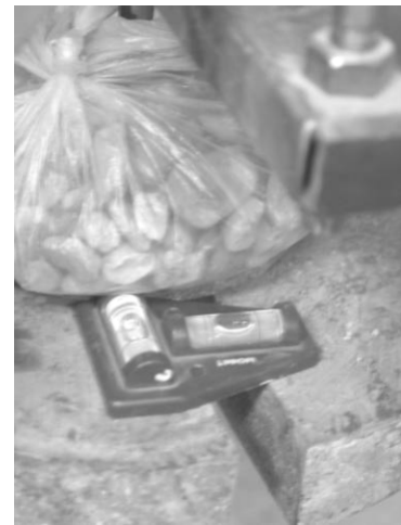
Figure 3.36 a) Levelling of the Load Hanger b) Close View
