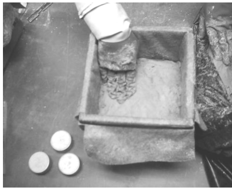
Figure 3.13 Representative Samples Taken for Water Content Determination
