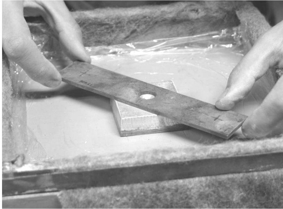
Figure 3.5 Placement of 50x50x15 mm Model Footing with a Rigid Steel Platform Fixed on Top on the Soil Surface Freely Before Testing
