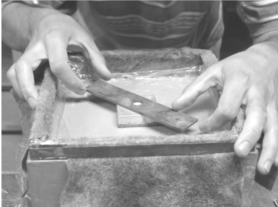
Figure 3.27 Placement of the Footing in Guidance of the Traces Left by Spatula
