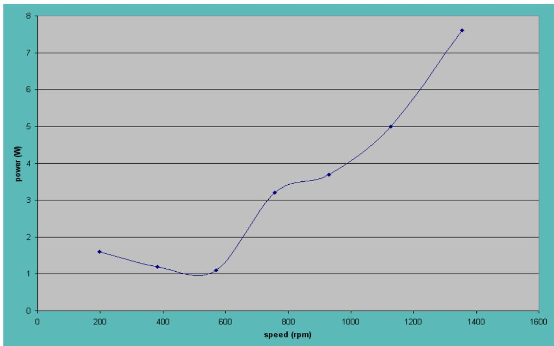
Fig.E.1 Rotational loss curve of 1.1 kW induction motor
