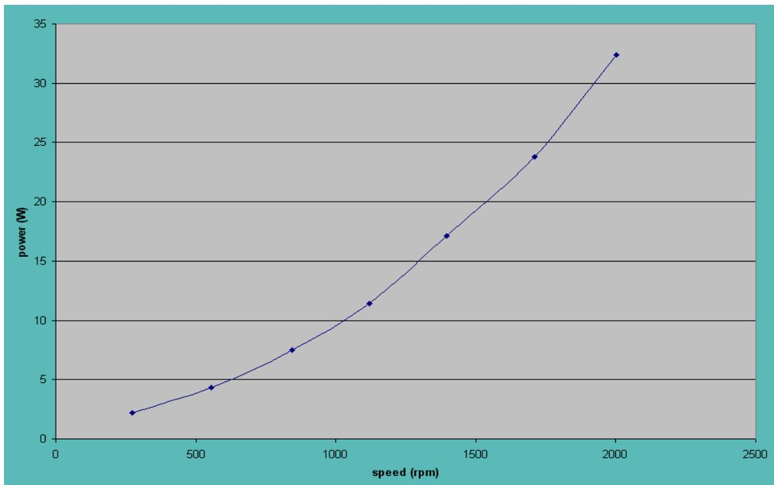
Fig.E.2 Rotational loss curve of 2.2 kW induction motor
