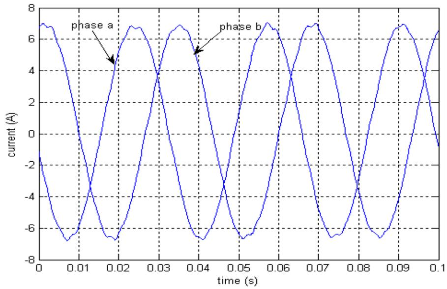
Fig.4.22 Measured stator currents at 30 Hz
