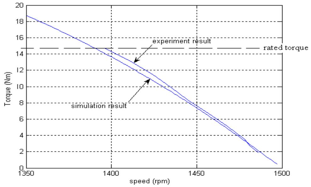
Figure.4.31 Linear portion of torque-speed curves for experiment result and simulation of 2.2 kW motor
