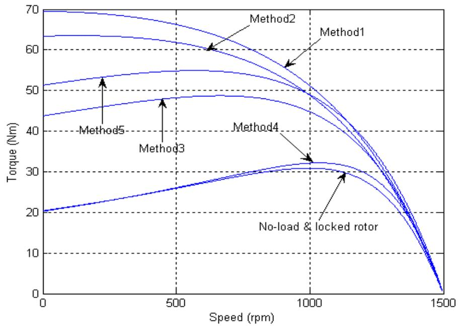
Fig.2.10 Torque-speed curves for 2.2kW induction motor
