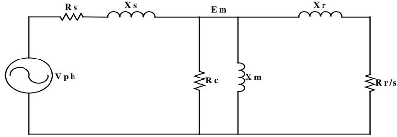
Figure.3.1: Exact steady-state model of induction machine
