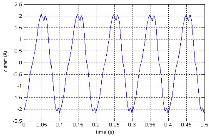
Figure.4.13 Stator phase current obtained from Trace program at 10Hz
