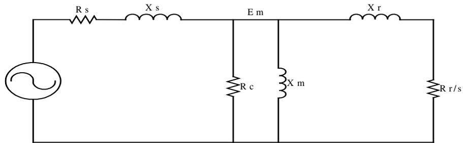
Fig.2.4 Equivalent circuit of induction machine
