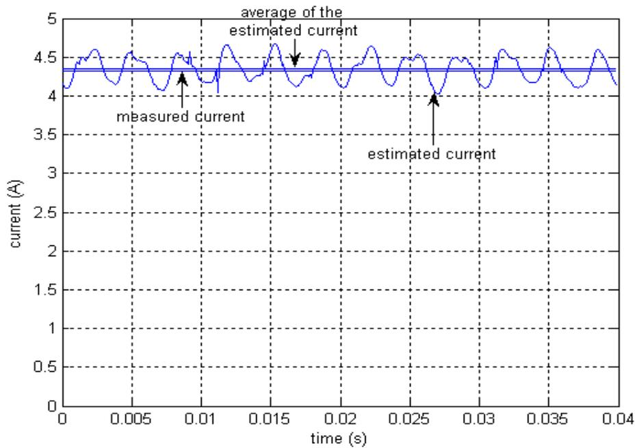
Fig.4.24 Measured and estimated rms value of stator current when motor is driven from the mains (f=50Hz)
