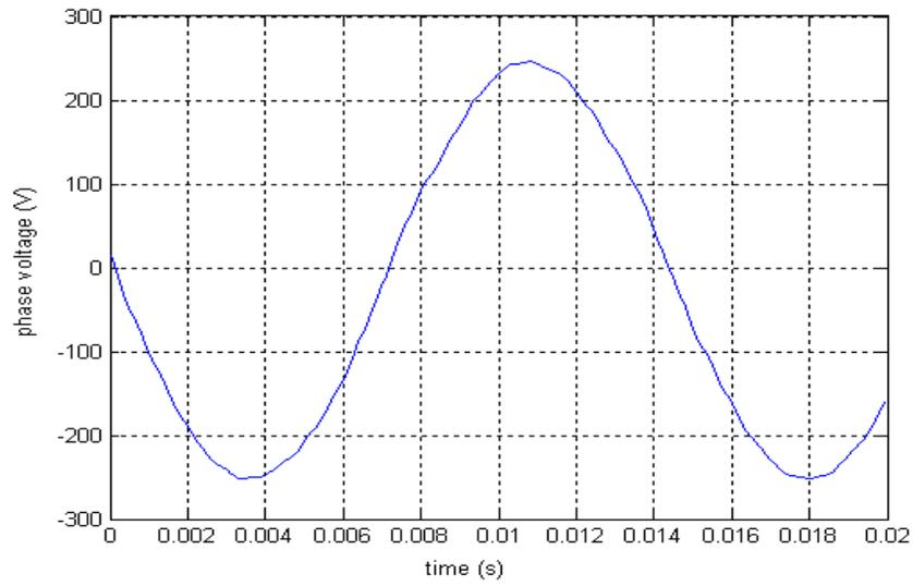
Fig.4.11 Stator phase voltage obtained from Trace program at 70Hz
