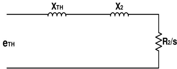
Fig.3.4. Thevenin theorem applied form of the equivalent circuit
