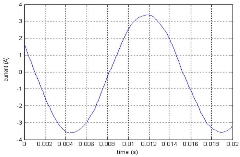
Figure.4.19 Stator phase current obtained from Trace program at 70Hz
