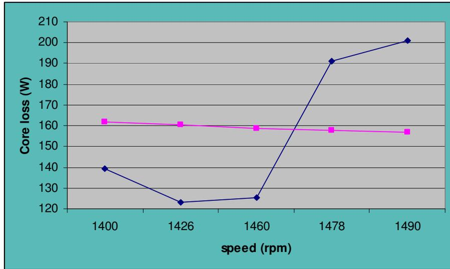
Fig.4.21 Calculated and measured core loss for mains (50Hz) driven motor
