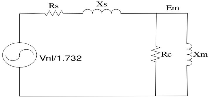
Fig.B.1 Induction motor model in no-load test
