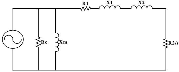
Figure.3.2. Approximate model of induction machine
