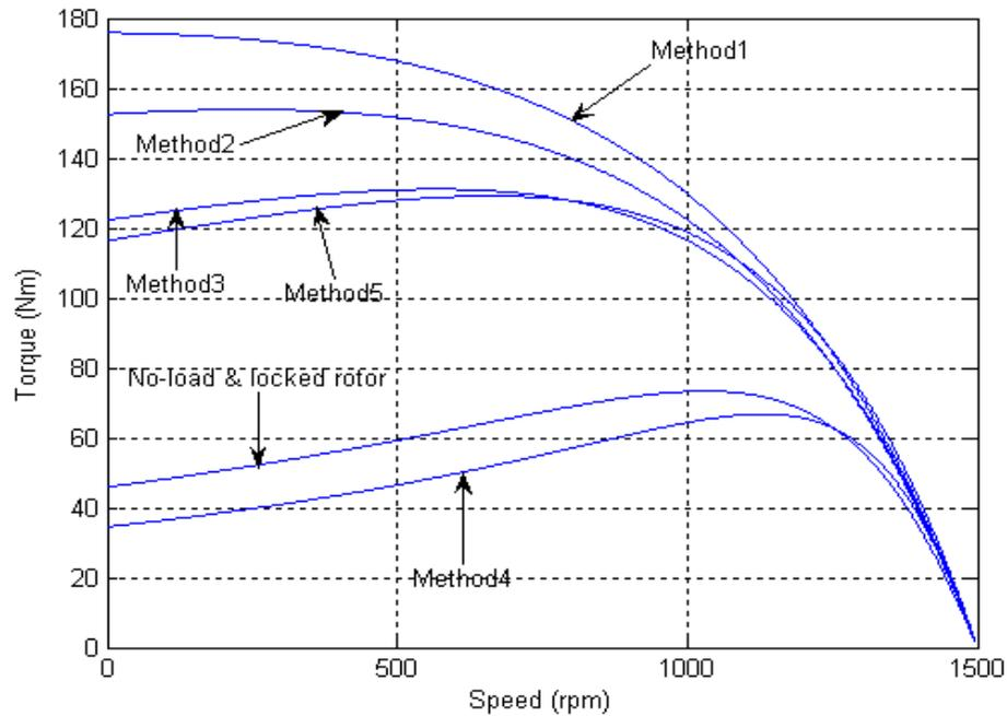
Fig.2.11 Torque-speed curves for 4kW induction motor
