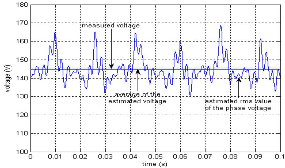
Fig.4.28 Measured and estimated rms value of phase voltage when motor is driven at 30Hz with inverter
