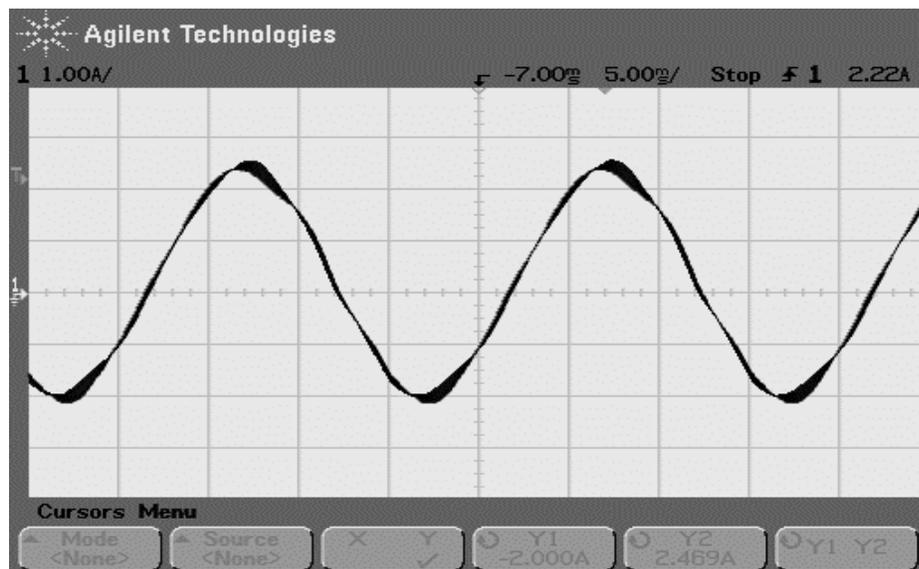
Fig.4.18 Stator phase current obtained from oscilloscope at 50Hz
