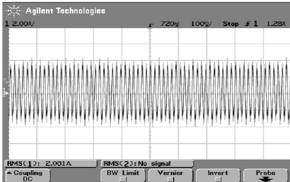
Fig.K.1 Stator phase current at 70 Hz
