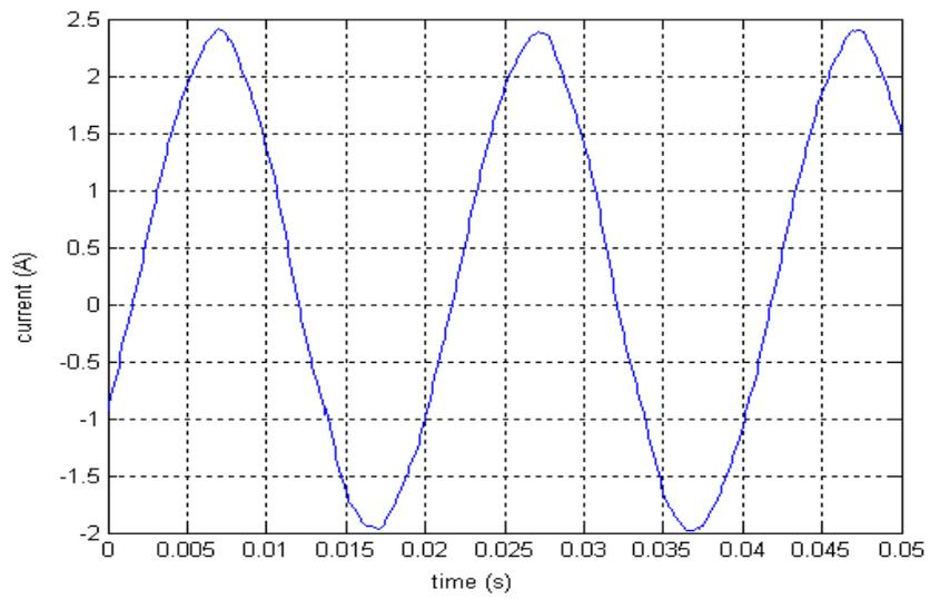
Figure.4.17 Stator phase current obtained from Trace program at 50Hz
