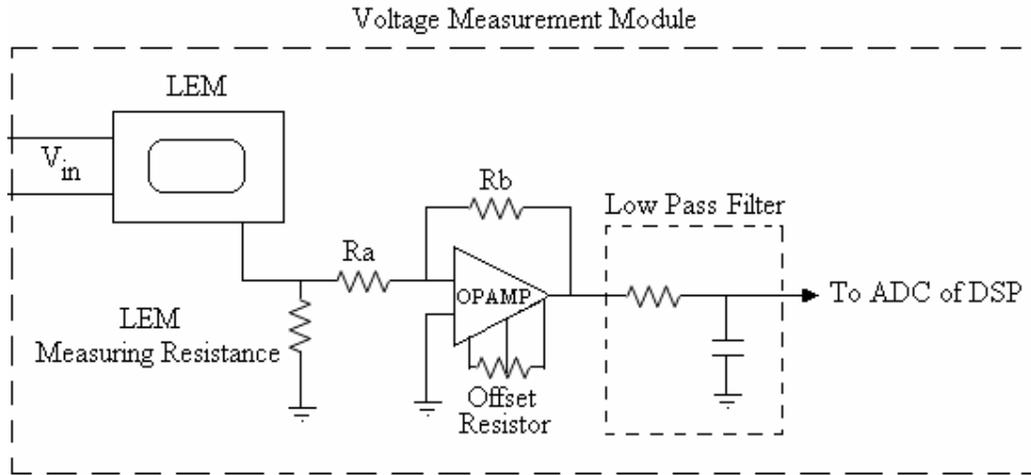
Figure.4.4 Schematic of voltage measurement module
