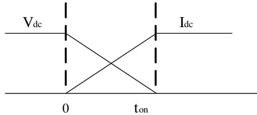
Figure.J.1 Voltage and current on the switch at turn-on of the switch
