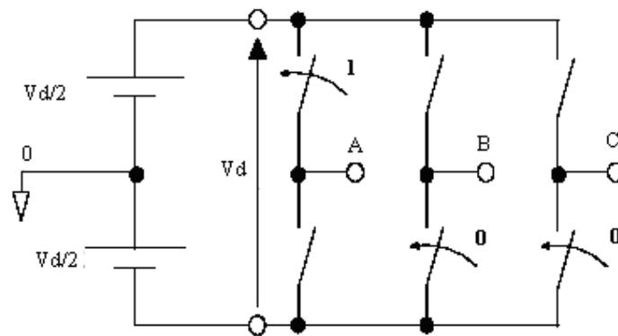
Figure.4.2 Used inverter topology
