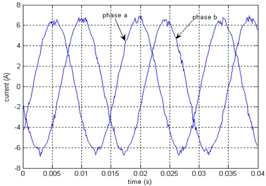
Fig.4.23 Measured stator currents at 70 Hz
