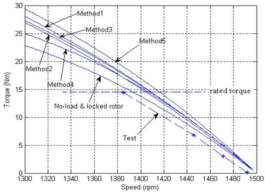
Fig.2.13 Torque-speed curves for 2.2kW induction motor
