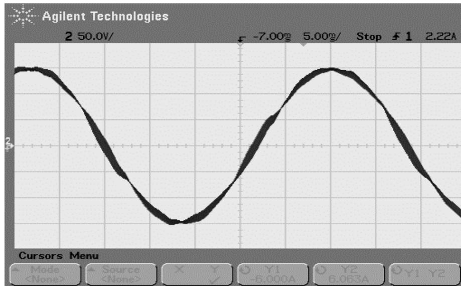
Fig.4.8 Stator phase voltage obtained from oscilloscope at 30Hz
