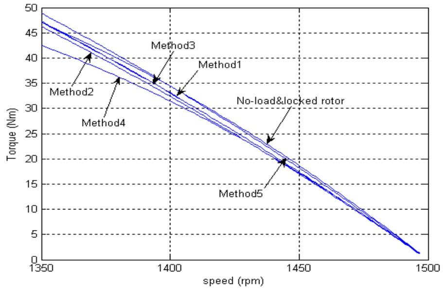
Fig.D.6 Torque-speed curves for 4kW induction motor
