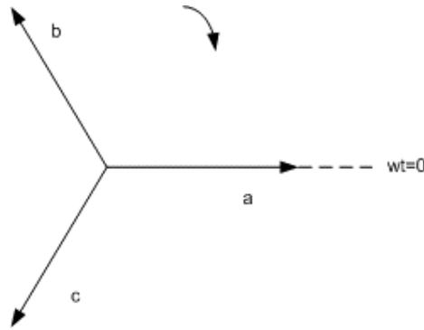
Fig.4.29 Magnetic axes of the motor
