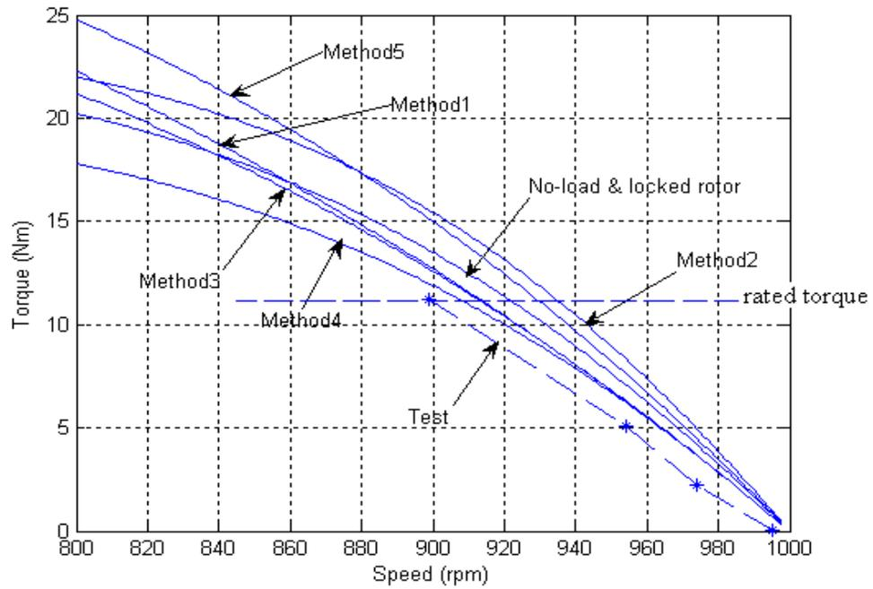
Fig.2.12 Torque-speed curves for 1.1kW induction motor
