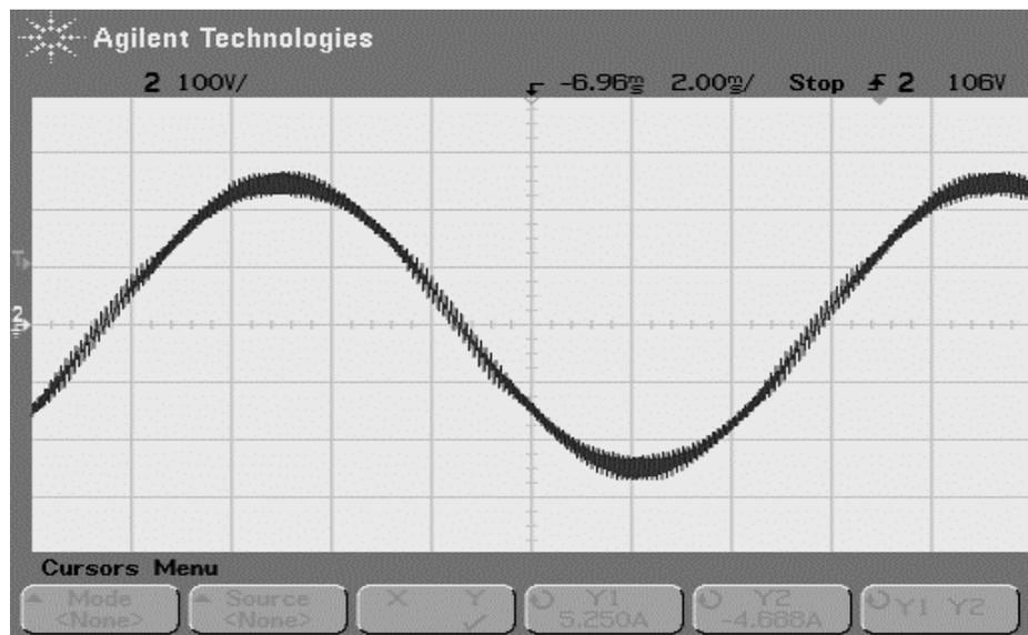
Fig.4.12 Stator phase voltage obtained from oscilloscope at 70Hz
