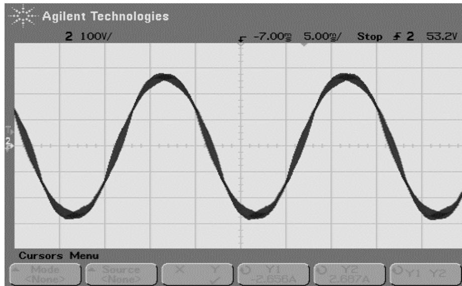
Fig.4.10 Stator phase voltage obtained from oscilloscope at 50Hz
