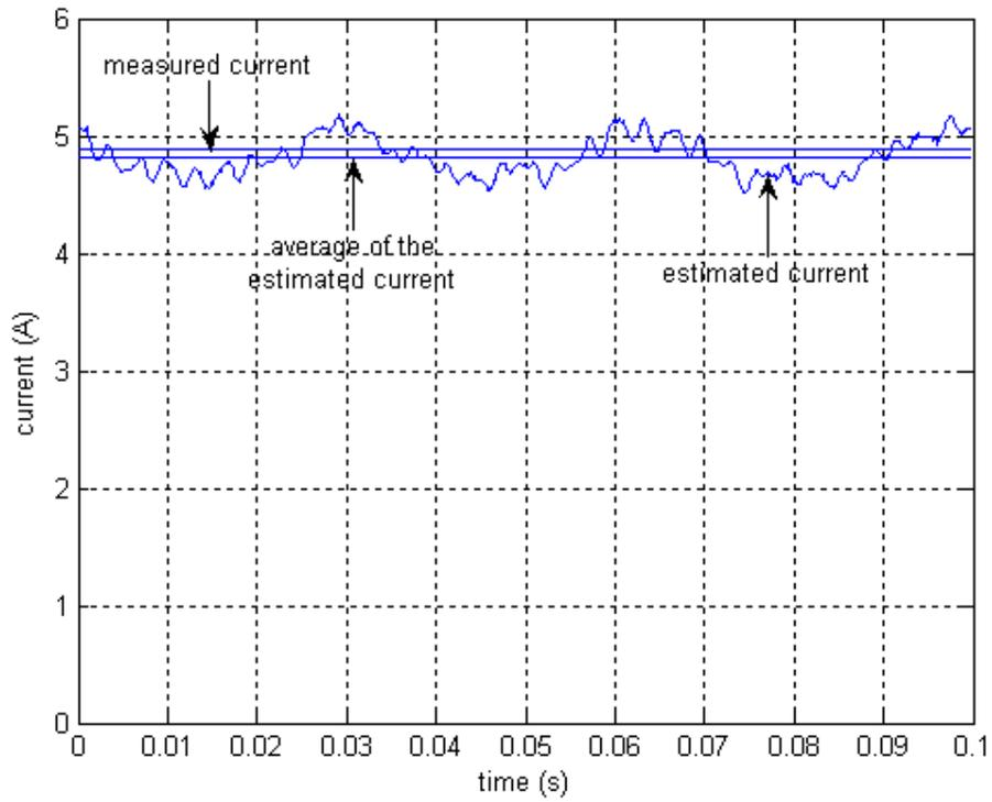
Fig.4.25 Measured and estimated rms value of stator current when motor is driven at 30Hz with inverter
