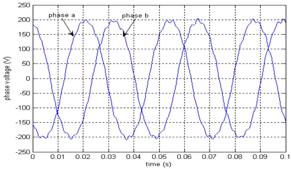
Fig.4.26 Measured phase to neutral voltages at 30Hz.
