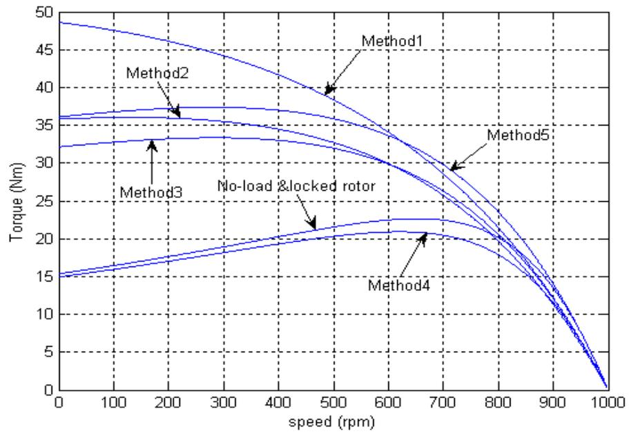
Fig.D.1 Torque-speed curves for 1.1kW induction motor
