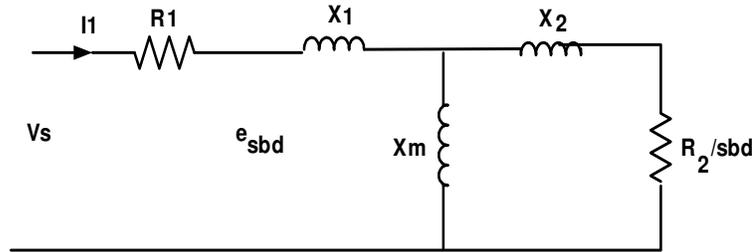
Fig.3.5.Equivalent circuit of induction machine at breakdown torque
