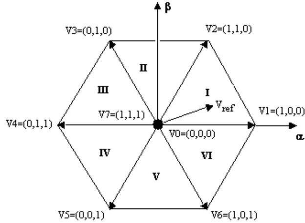
Figure.4.3 Basic space vectors and switching states
