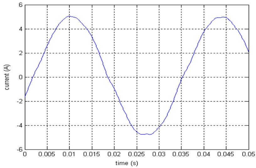
Figure.4.15 Stator phase current obtained from Trace program at 30Hz
