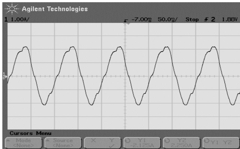
Fig.4.14 Stator phase current obtained from oscilloscope at 10Hz
