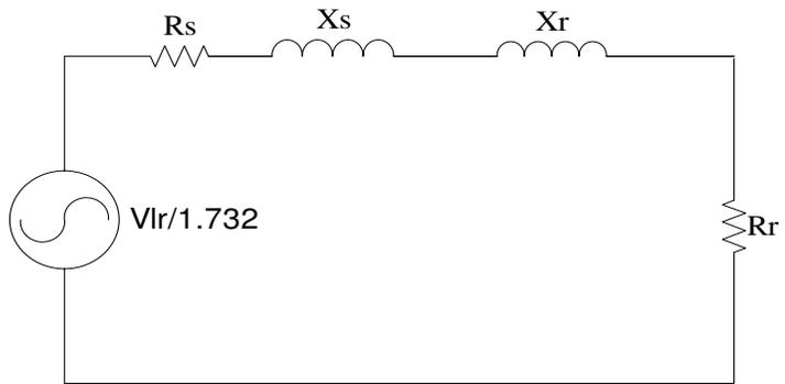
Fig.B.2 Induction motor model in locked rotor test
