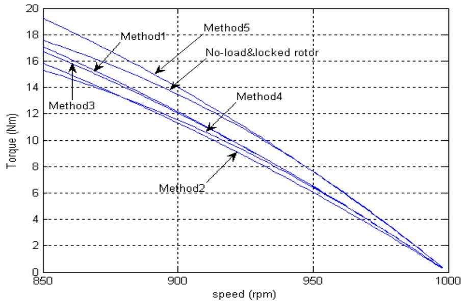
Fig.D.4 Torque-speed curves for 1.1kW induction motor
