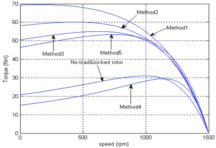
Fig.D.2 Torque-speed curves for 2.2kW induction motor
