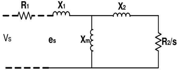
Figure.3.3. Modified equivalent circuit of induction machine
