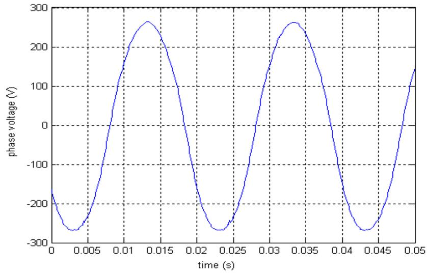
Fig.4.9 Stator phase voltage obtained from Trace program at 50Hz
