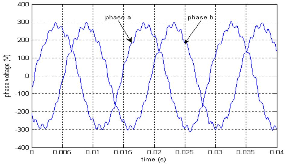
Fig.4.27 Measured phase to neutral voltages at 70Hz
