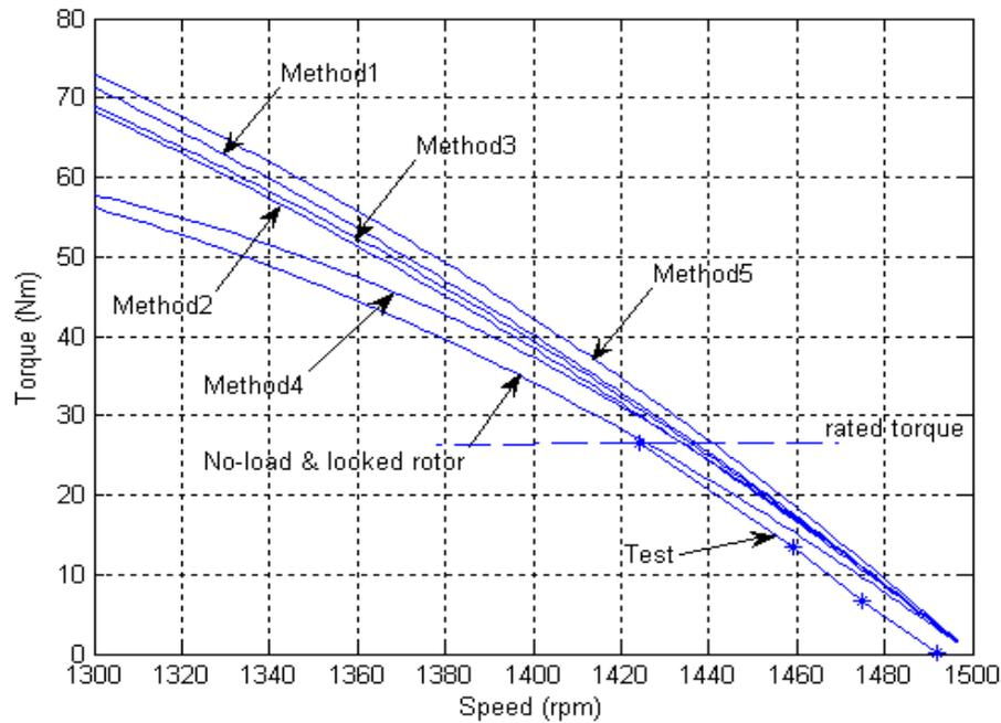
Fig.2.14 Torque-speed curves for 4kW induction motor
