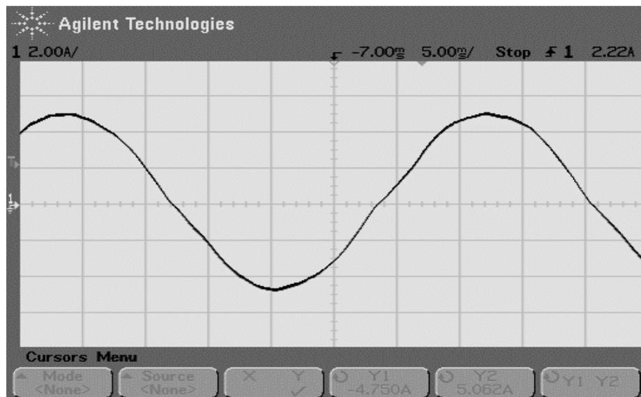
Fig.4.16 Stator phase current obtained from oscilloscope at 30Hz
