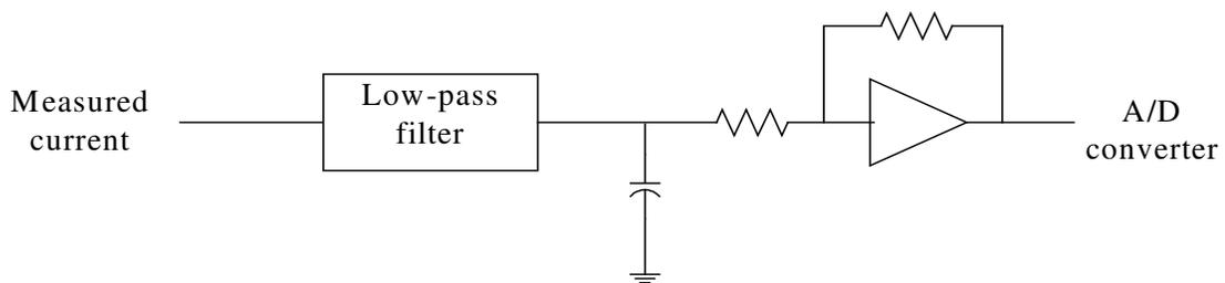
Fig.6.1 Measurement module for rms value of current
