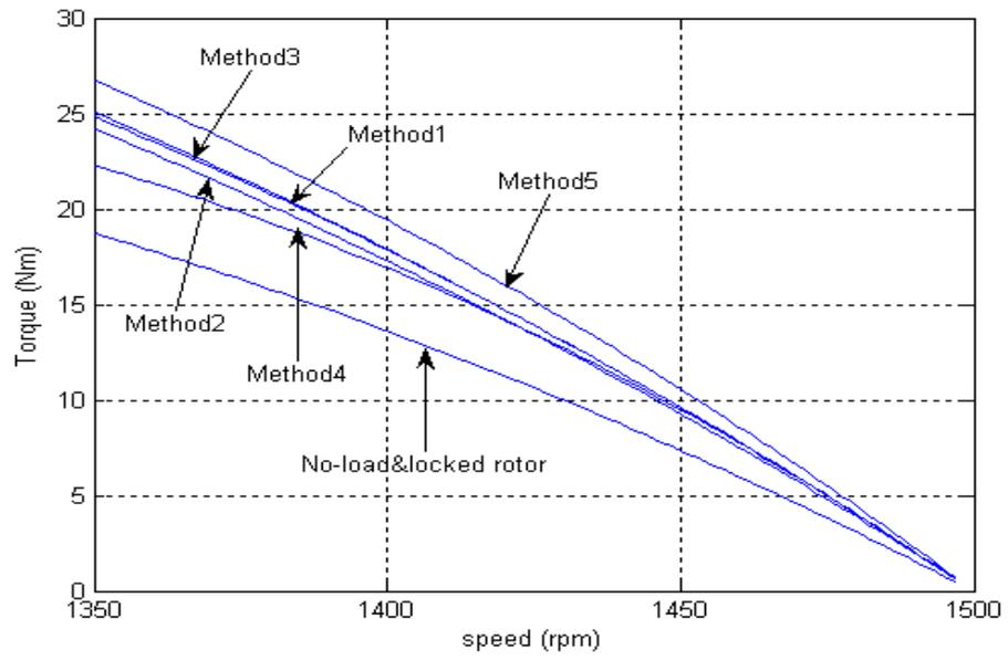
Fig.D.5 Torque-speed curves for 2.2kW induction motor
