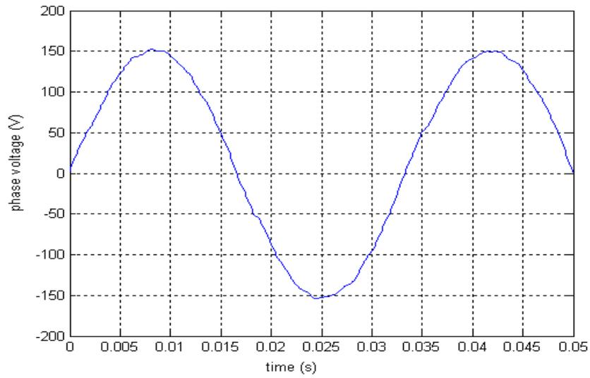
Fig.4.7 Stator phase voltage obtained from Trace program at 30Hz
