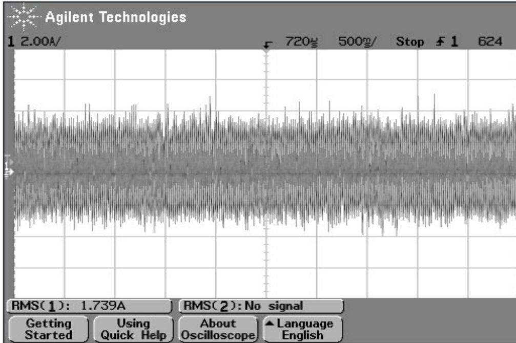
Fig.K.2 Stator phase current at 50 Hz
