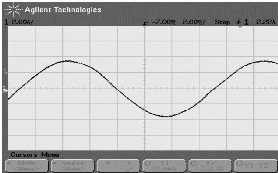
Fig.4.20 Stator phase current obtained from oscilloscope at 70Hz
