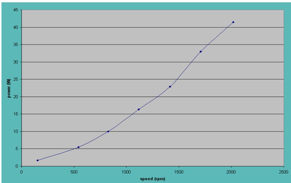
Fig.E.3 Rotational loss curve of 4 kW induction motor
