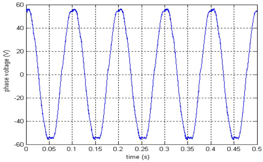
Fig.4.5 Stator phase voltage obtained from Trace program at 10Hz
