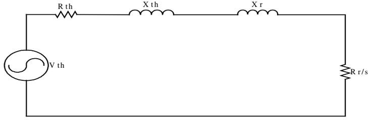
Fig.2.6. Thevenin theorem applied model of the induction machine
