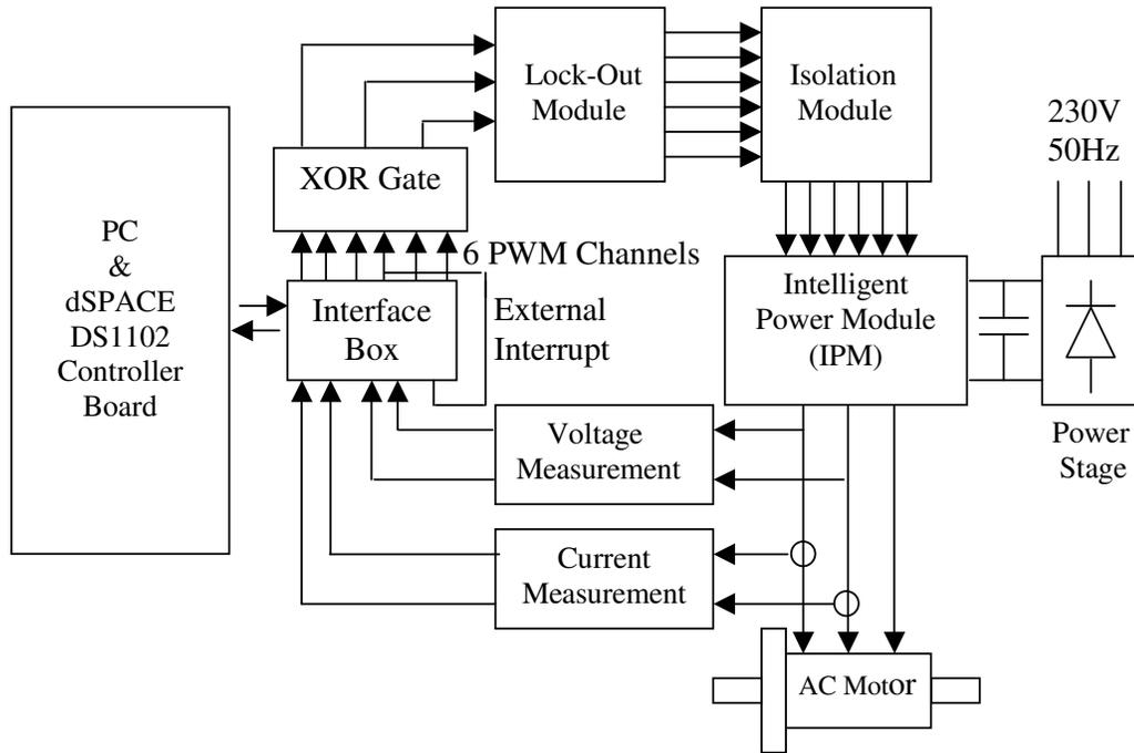
Figure.4.1 Block diagram of hardware
