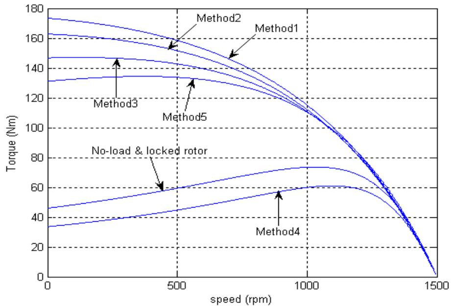
Fig.D.3 Torque-speed curves for 4kW induction motor
