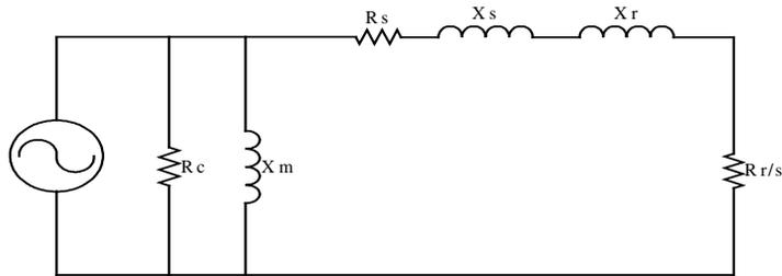
Fig.2.1. Approximate model of Induction Machine
