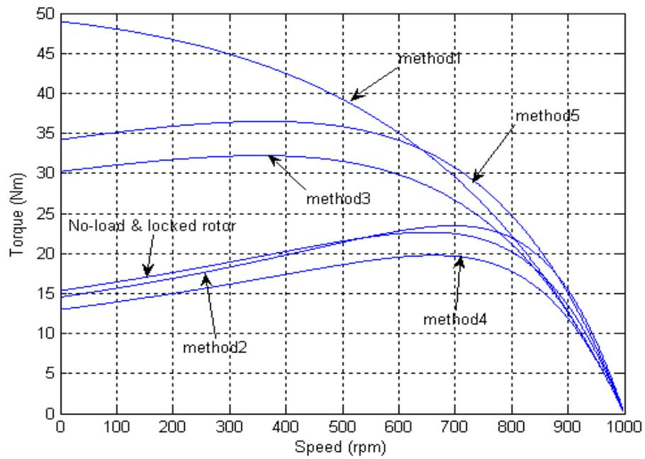
Fig.2.9 Torque-speed curves for 1.1kW induction motor
