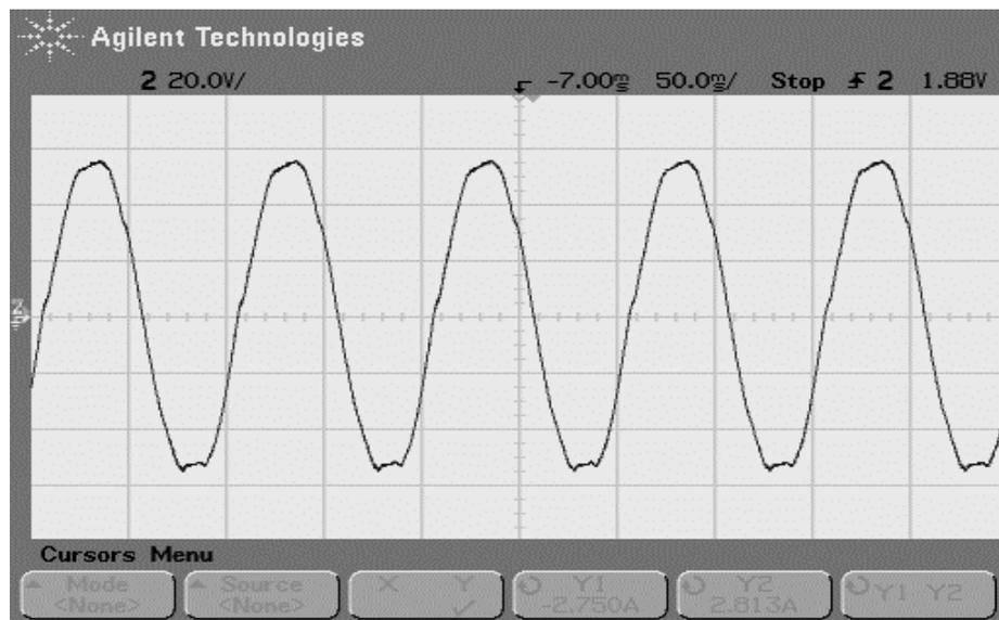
Fig.4.6 Stator phase voltage obtained from oscilloscope at 10Hz
