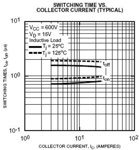
Figure.J.2 Switching times of IPM versus current
