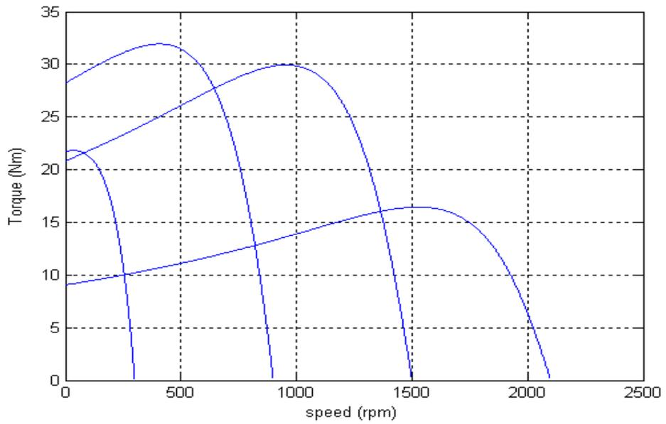
Fig.4.32 Torque-speed curves prepared with simulation for 10, 30, 50 and 70Hz
