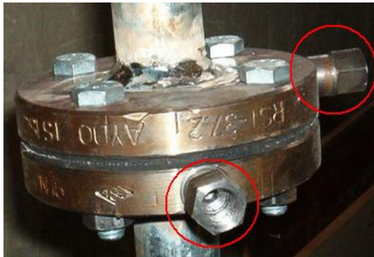
Fig 4.2: Orifice Flanges and Transducer Adapters
