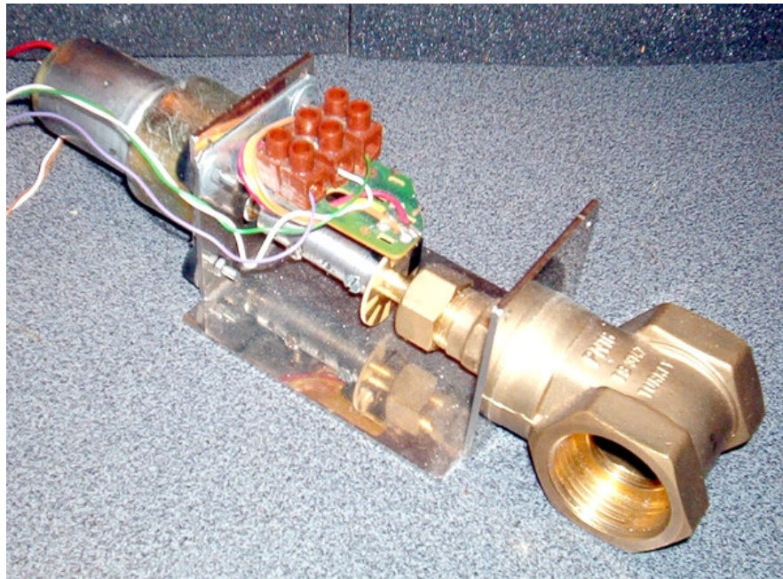
Fig 4.5: DC Motor Operated Wedge Disc Throttling Valve with Position Feedback
