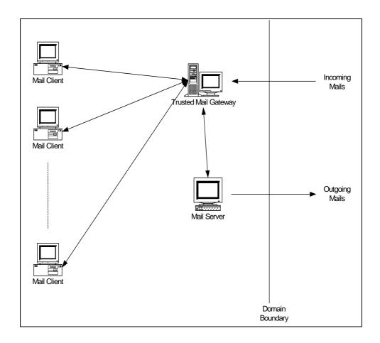
Figure 1: A domain with the Trusted Mail Gateway installed
