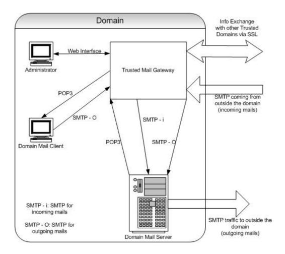
Figure 7: Position of Trusted Mail Gateway in a domain
