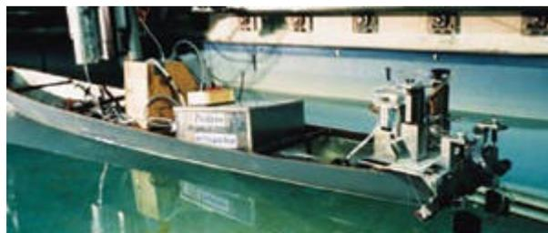
Figure 2.2: Proteus with flapping foils in the test tank (Towtank, 2004)
