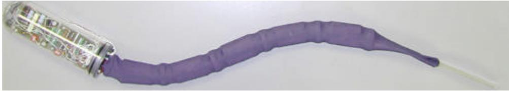
Figure 2.10: SMA actuated lamprey robot
