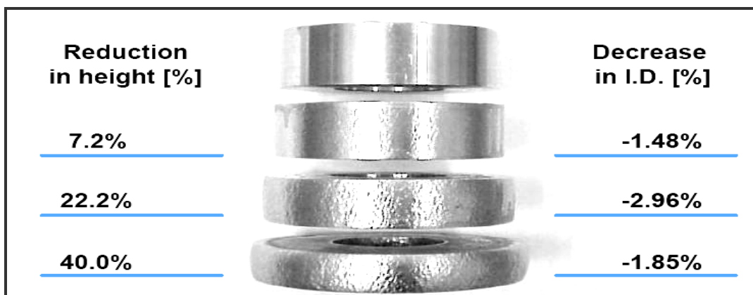
Figure 2.10 Test result for ring compression [22]
