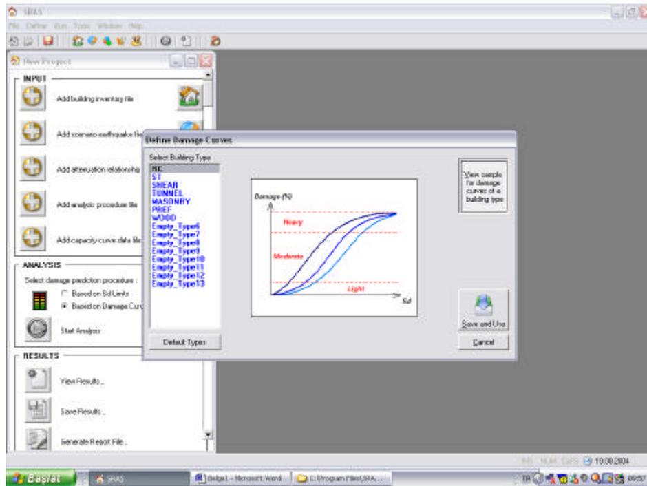
Figure 4. 29 Defining damage curves according to building types.
