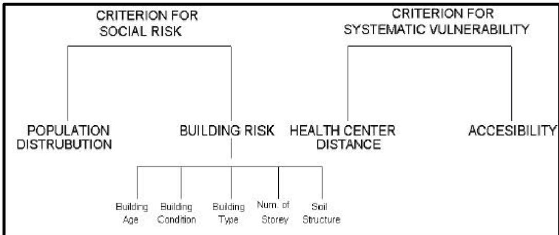
Figure 3. 2 Criterias used in estimating the building damage
