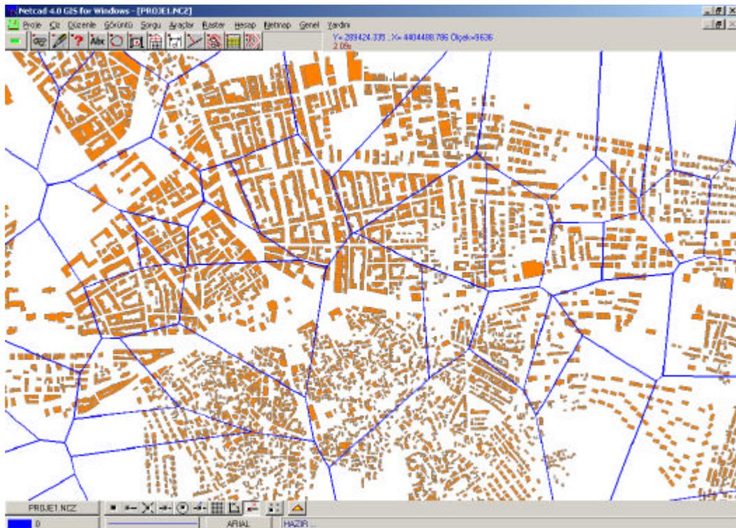
Figure 4. 23 Voronoi polygons derived from soil structure data
