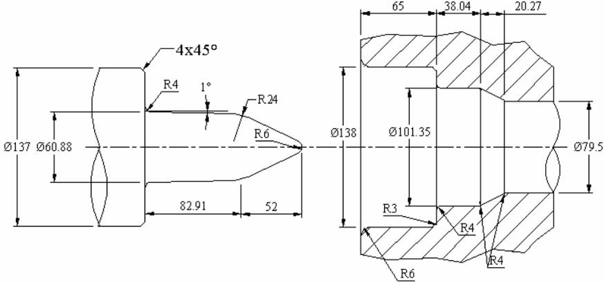
Figure 5.7. Header tool and gripper die of 3<sup>rd</sup> stage [3]
