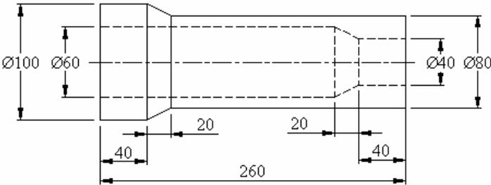
**Figure 5.4.** Shape of part for stage 2 [3]
