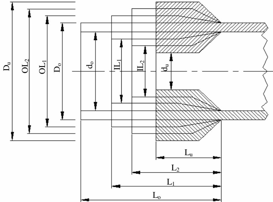
**Figure 2.8.** *Determination of outer and inner profile limits for simultaneous external and internal upsetting [3]*
