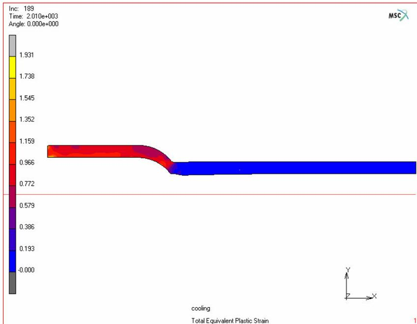
**Figure 7.10.** Total equivalent plastic strain distribution after cooling
