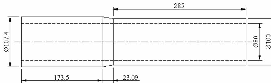
**Figure 4.9.** Shape of part for stage 1 [3]
