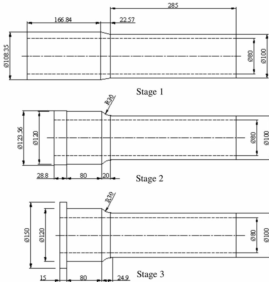
*Figure 4.42. Shape of the tube at intermediate stages [3]*
