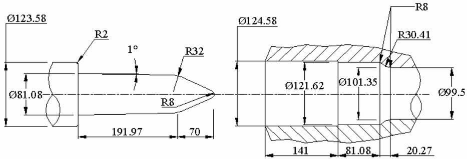
Figure 4.44. Header and gripper dies for 2<sup>nd</sup> stage [3]
