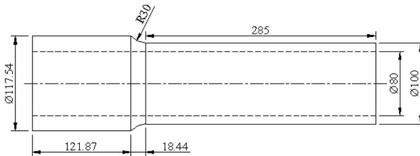
**Figure 4.27.** Modified shape of part at stage 2
