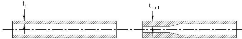
**Figure 2.5.** Wall thickness change during internal upsetting
