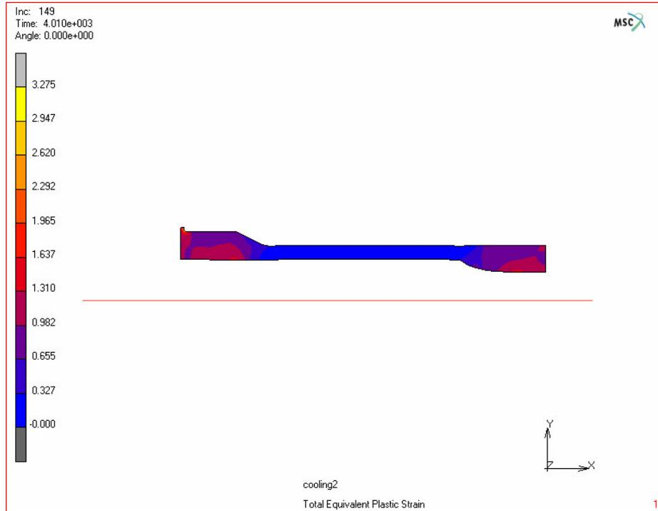
**Figure 5.13.** Total equivalent plastic strain distribution after cooling
