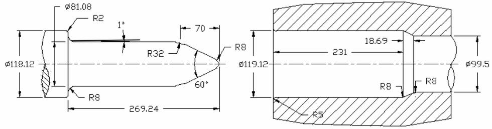
**Figure 4.14.** Header tool and gripper die of 2<sup>nd</sup> stage [3]
