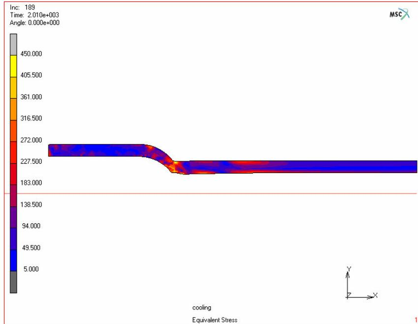
**Figure 7.11.** *Equivalent stress distribution after cooling (MPa)*
