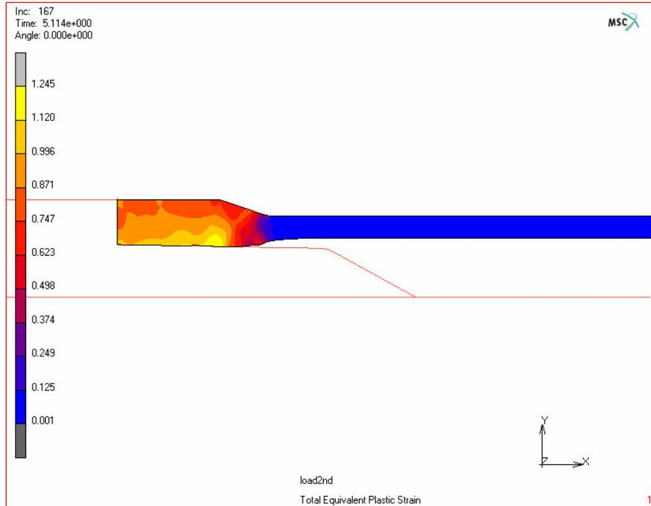
**Figure 6.8.** Total equivalent plastic strain distribution after 2<sup>nd</sup> stage
