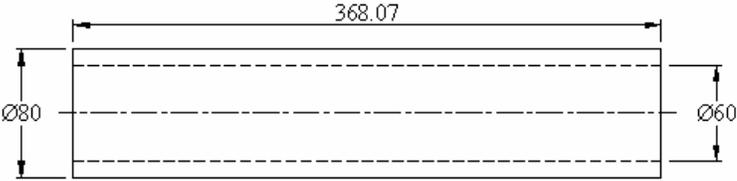
**Figure 5.2.** Required initial tube for upsetting [3]
