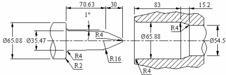
**Figure 6.5.** Header tool and gripper die of 2<sup>nd</sup> stage [3]
