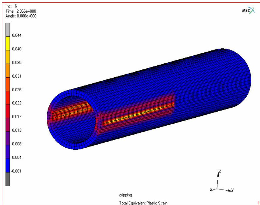
**Figure A.3.** Total equivalent plastic strain distribution after tools are removed
