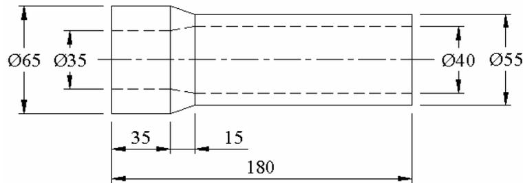
*Figure 6.1. A part requiring upsetting at both ends [3]*
