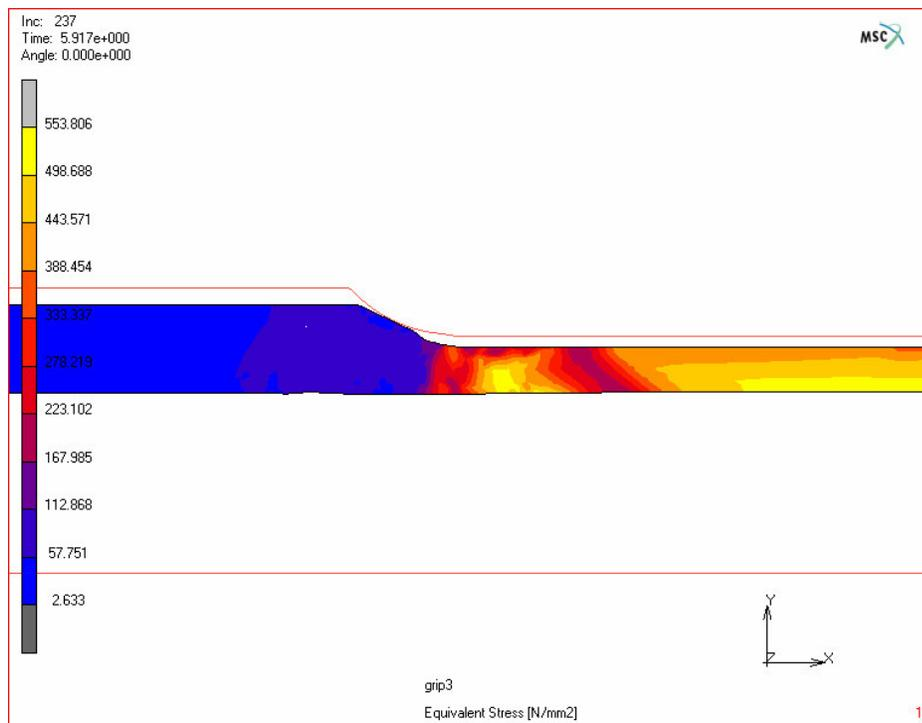
**Figure 4.23.** Equivalent stress distribution during gripping at 3<sup>rd</sup> stage (MPa)
