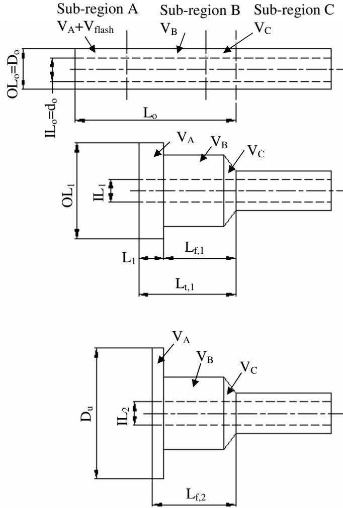
**Figure 2.7.** Volume constancy along the upset region and shape design for intermediate stages [3]
