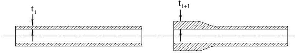
**Figure 2.4.** Wall thickness change during external upsetting
