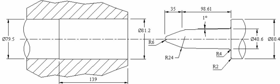
Figure 5.5. Header tool and gripper die of 1<sup>st</sup> stage [3]
