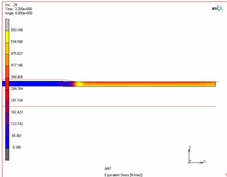
**Figure 4.21.** Equivalent stress distribution during gripping at 1<sup>st</sup> stage (MPa)
