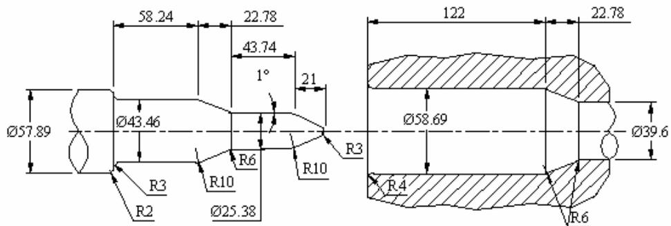
**Figure 7.4.** Header tool and gripper die of 1<sup>st</sup> stage [3]
