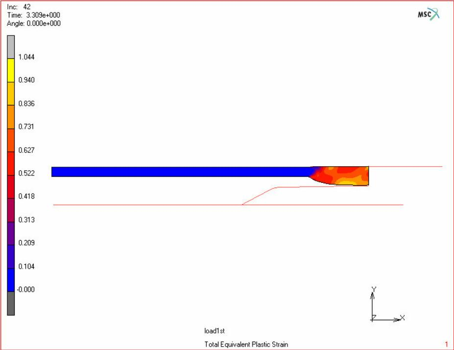
*Figure 5.9. Total equivalent plastic strain distribution after 1<sup>st</sup> stage*
