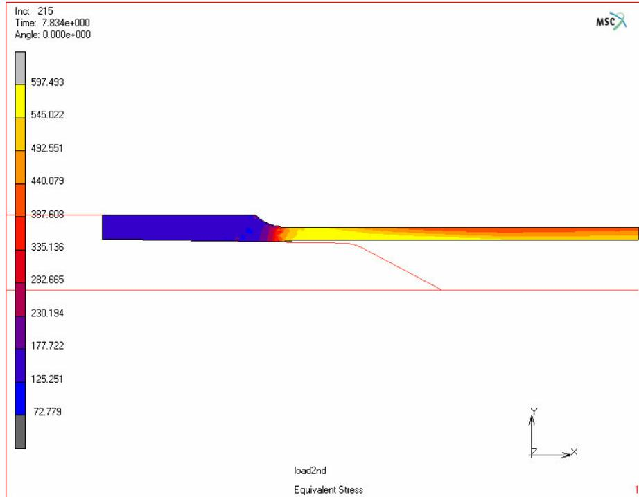
**Figure 4.33.** Equivalent stress distribution after 2<sup>nd</sup> stage (MPa)
