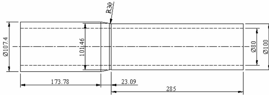
**Figure 4.26.** Modified shape of part at stage 1
