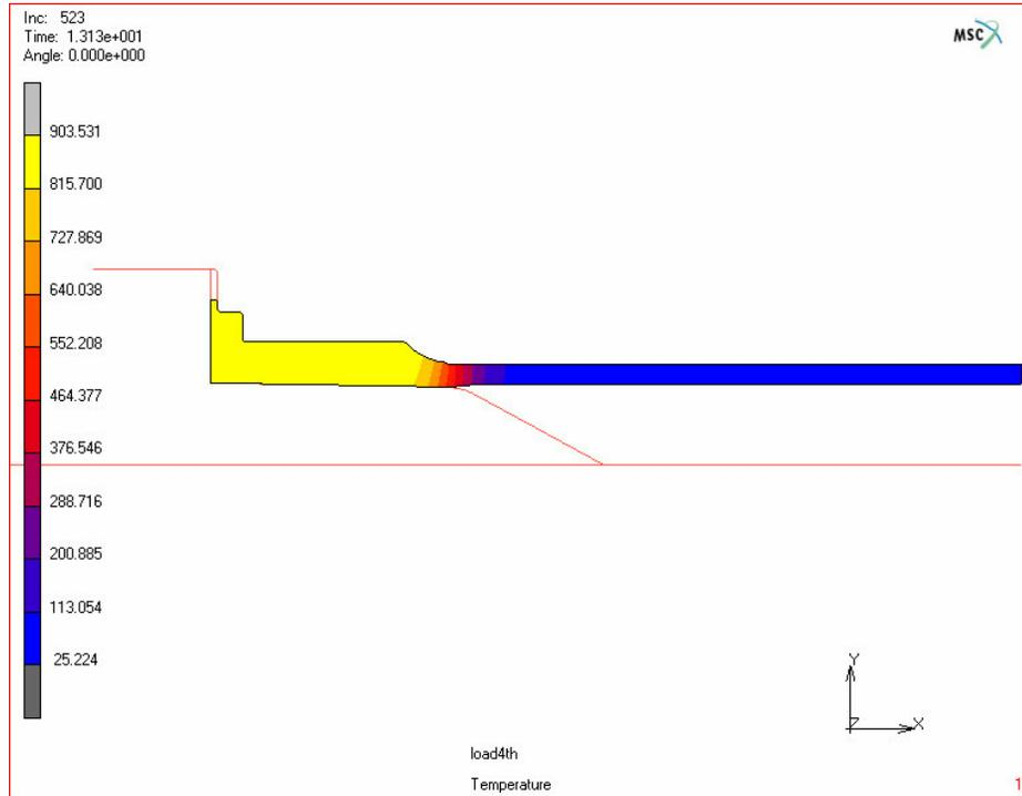
**Figure 4.38.** Temperature distribution after 4<sup>th</sup> stage (°C)
