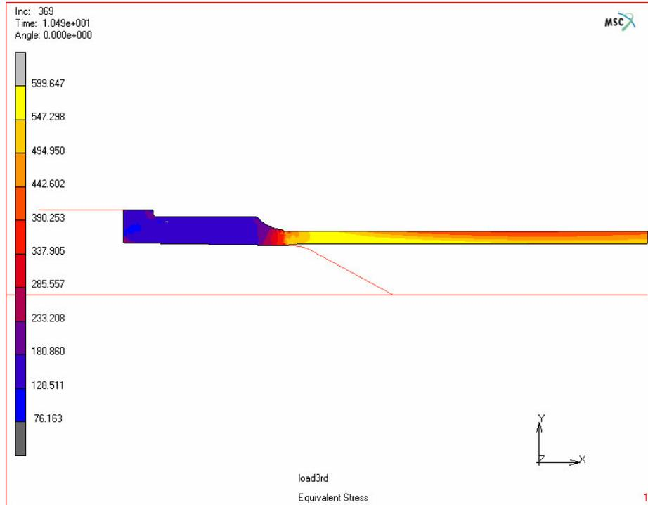
**Figure 4.35.** Equivalent stress distribution after 3<sup>rd</sup> stage (MPa)
