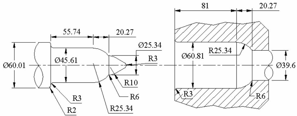
**Figure 7.5.** Header tool and gripper die of 2<sup>nd</sup> stage [3]
