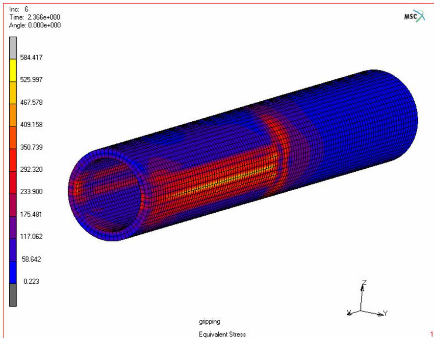
**Figure A.5.** Equivalent stress distribution after tools are removed (MPa)
