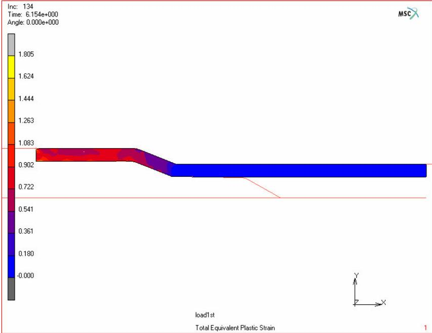
**Figure 7.7.** Total equivalent plastic strain distribution after 1<sup>st</sup> stage
