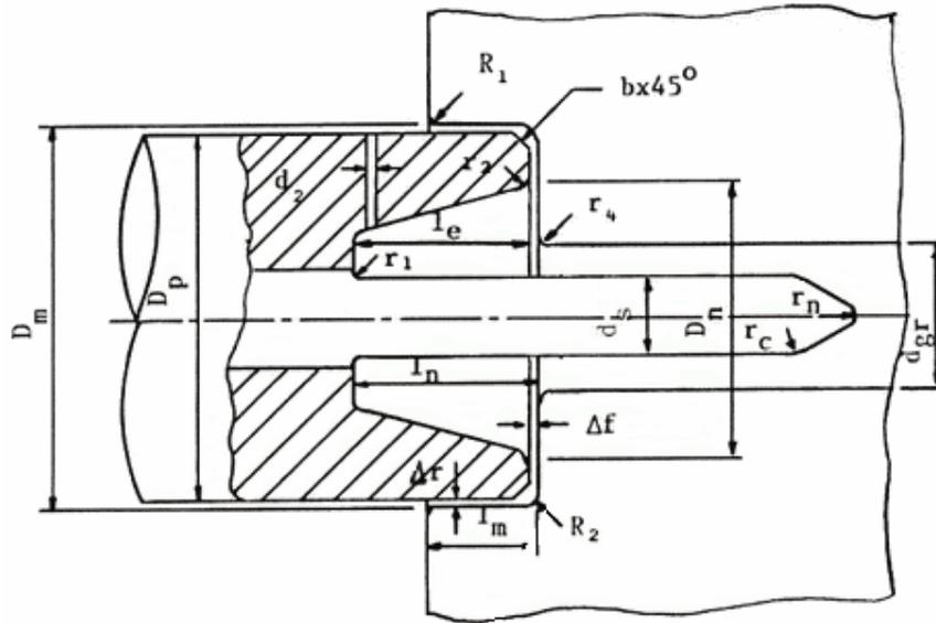
Figure 2.10. Die cavity in header tool [3]
