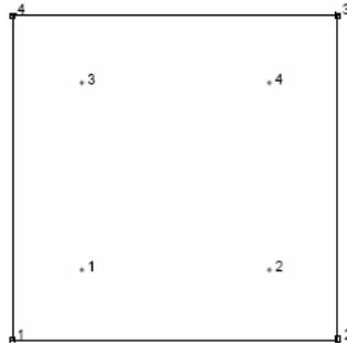
*Figure 3.1. Integration point for element type 10 [25]*
