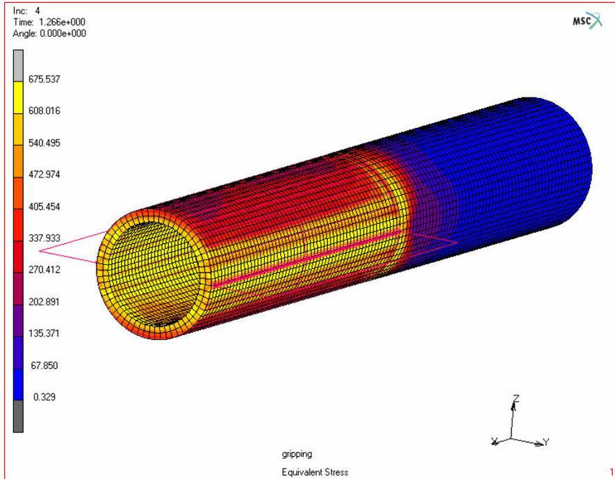
**Figure A.4.** Equivalent stress distribution during gripping (MPa)
