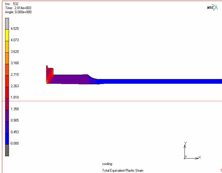
**Figure 4.40.** Total equivalent plastic strain distribution at the end of the analysis
