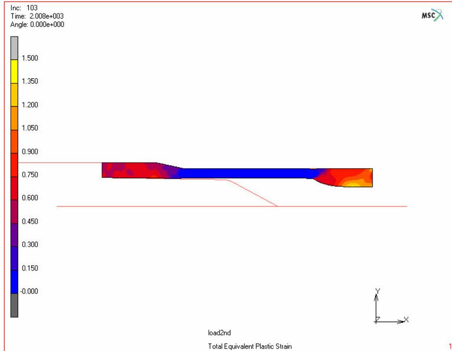
**Figure 5.10.** Total equivalent plastic strain distribution after 2<sup>nd</sup> stage
