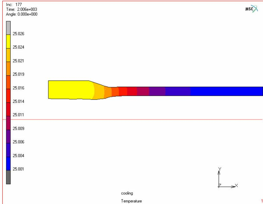
**Figure 6.9.** Temperature distribution after cooling stage (°C)
