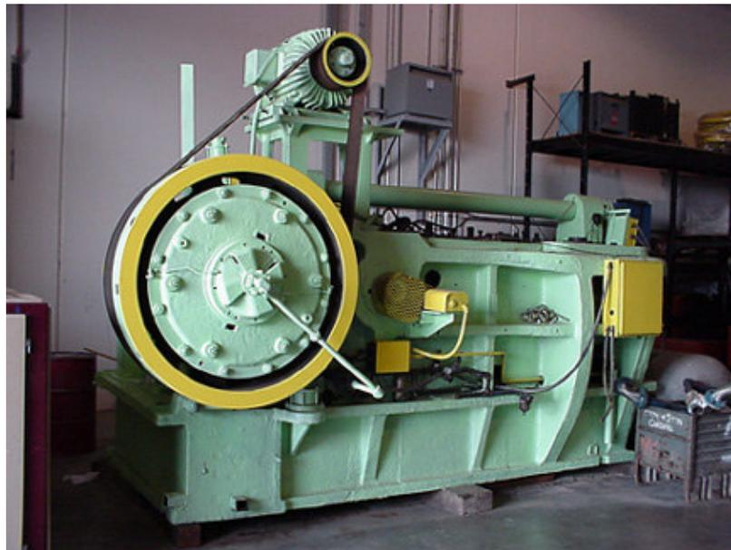
*Figure 1.1. A typical horizontal forging machine for hot upset forging [2]*
