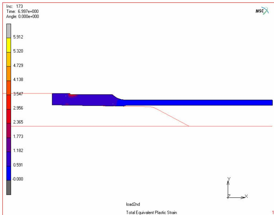
**Figure 4.48.** Total equivalent plastic strain distribution after 2<sup>nd</sup> stage
