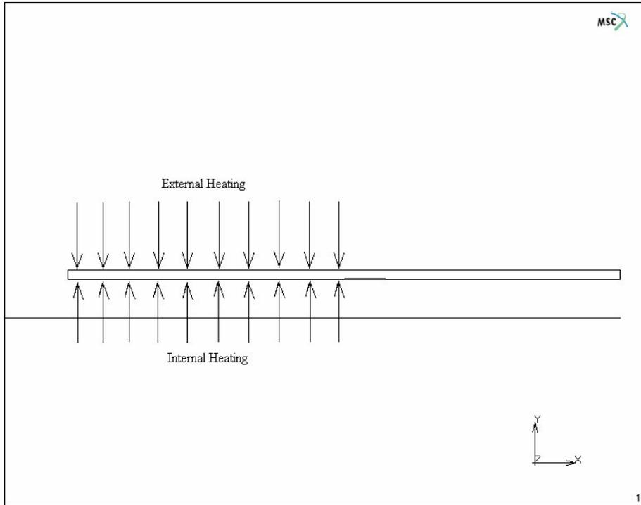
**Figure 4.19.** Heat flux boundary condition in the finite element analysis
