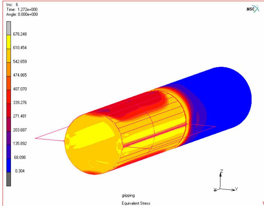
**Figure A.7.** Equivalent stress distribution during gripping with fine mesh (MPa)
