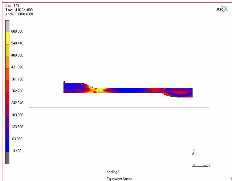
**Figure 5.14.** Equivalent stress distribution after cooling (MPa)
