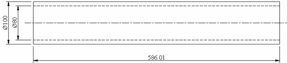
**Figure 4.8.** Required initial tube for upsetting
