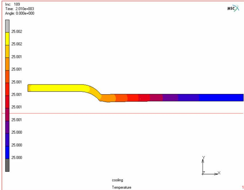
**Figure 7.9.** Temperature distribution after cooling stage ( $^{\circ}\text{C}$ )
