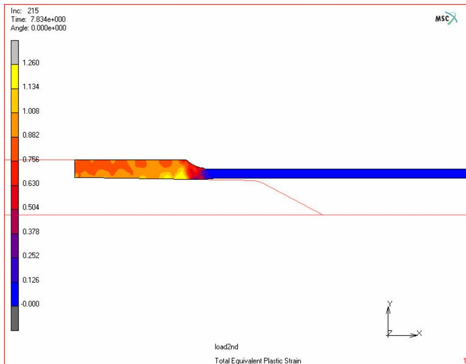
**Figure 4.32.** Total equivalent plastic strain distribution after 2<sup>nd</sup> stage
