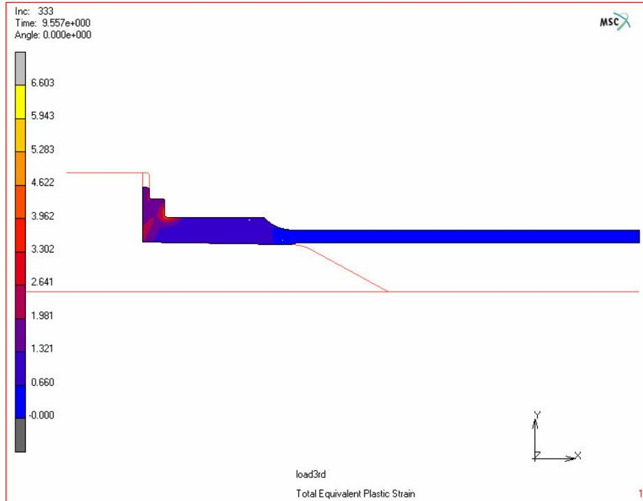
**Figure 4.49.** Total equivalent plastic strain distribution after 3<sup>rd</sup> stage
