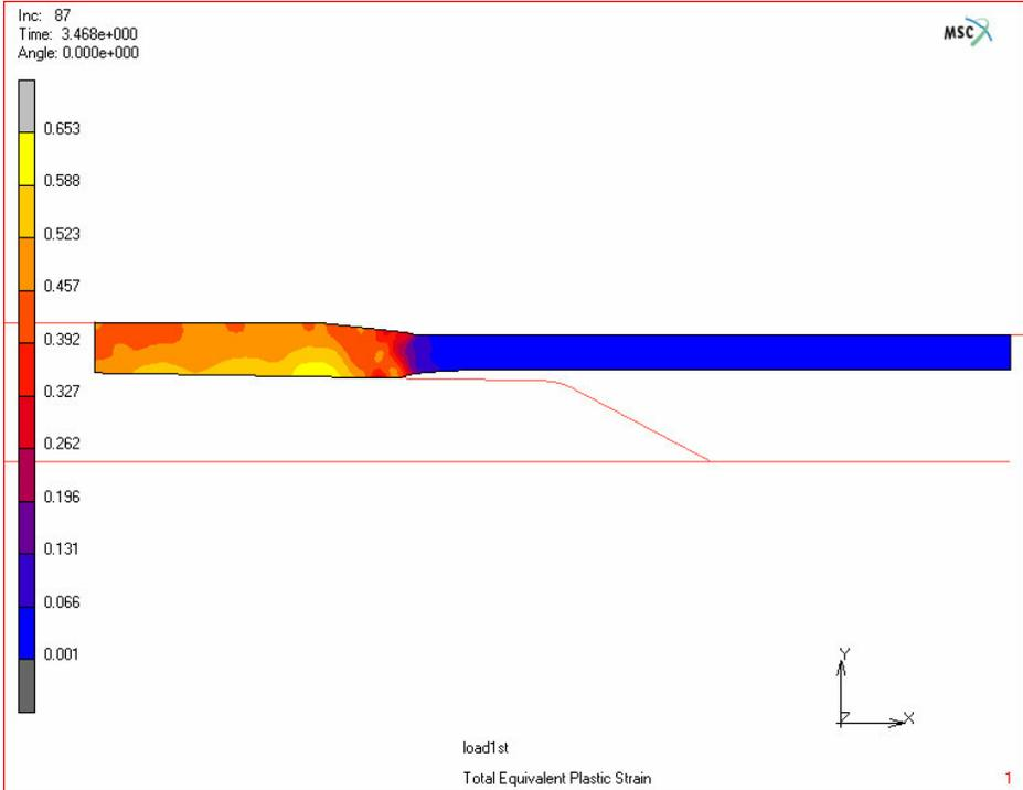
**Figure 6.7.** Total equivalent plastic strain distribution after 1<sup>st</sup> stage
