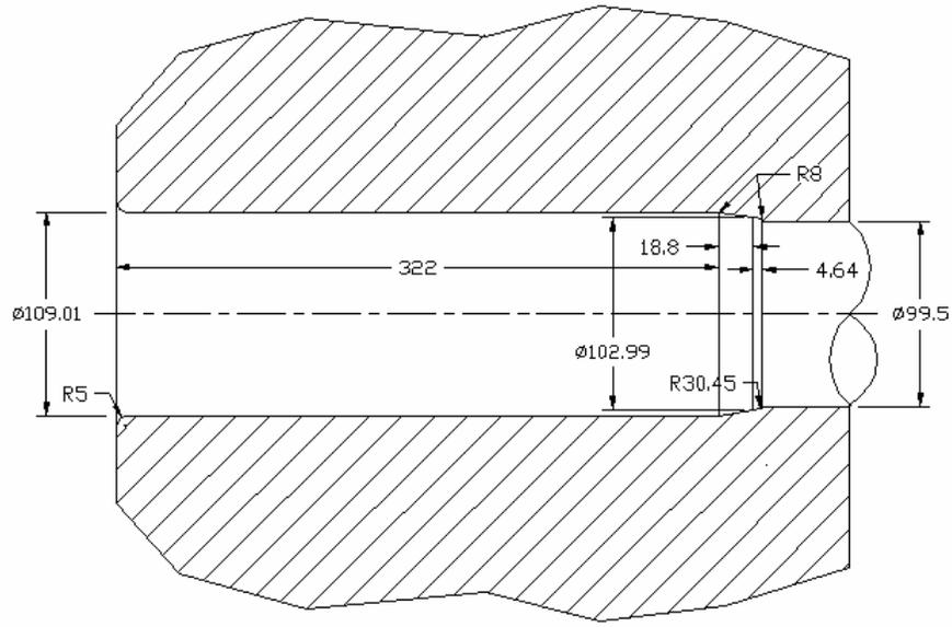
**Figure 4.28.** Modified gripper die of 1<sup>st</sup> stage
