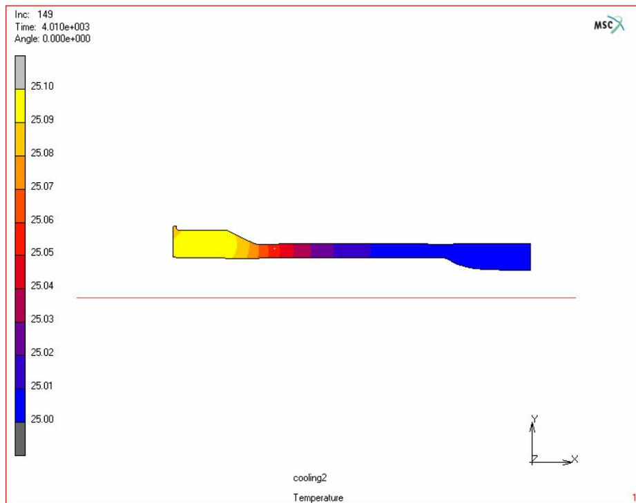
**Figure 5.12.** Temperature distribution after cooling stage (°C)
