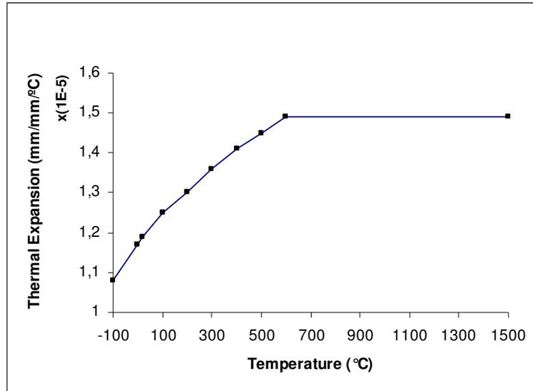
*Figure 4.1. Thermal expansion versus temperature [26]*
