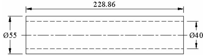
**Figure 6.2.** Required initial tube for upsetting [3]
