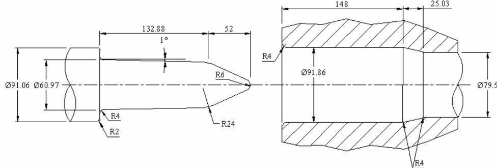
Figure 5.6. Header tool and gripper die of 2<sup>nd</sup> stage [3]
