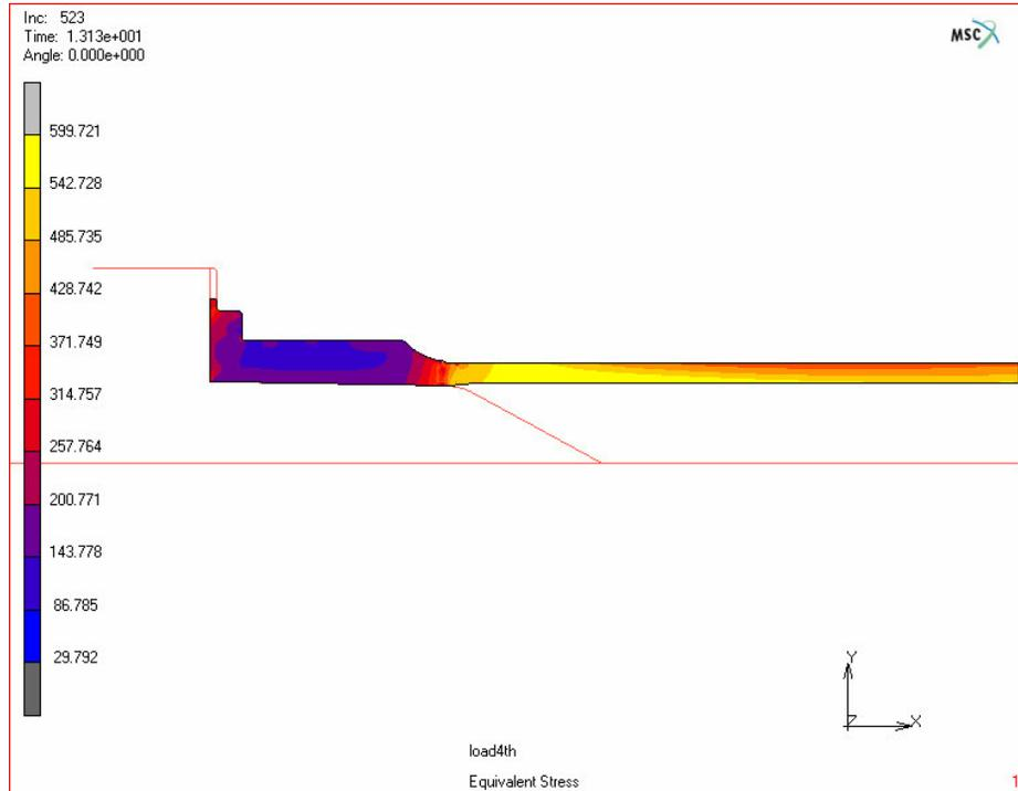
**Figure 4.37.** Equivalent stress distribution after 4<sup>th</sup> stage (MPa)
