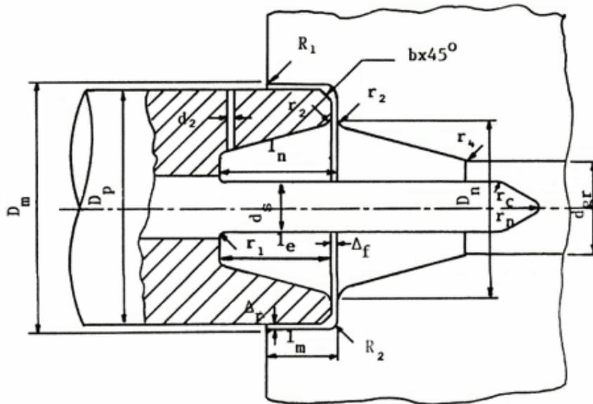
Figure 2.11. Die cavity in both header tool and gripper dies [3]
