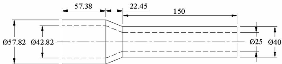
**Figure 7.3.** Shape of part for stage 1 [3]
