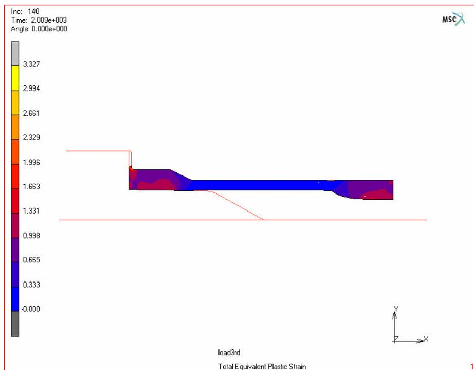
**Figure 5.11.** Total equivalent plastic strain distribution after 3<sup>rd</sup> stage
