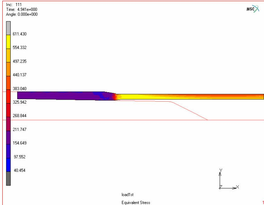
**Figure 4.31.** Equivalent stress distribution after 1<sup>st</sup> stage (MPa)
