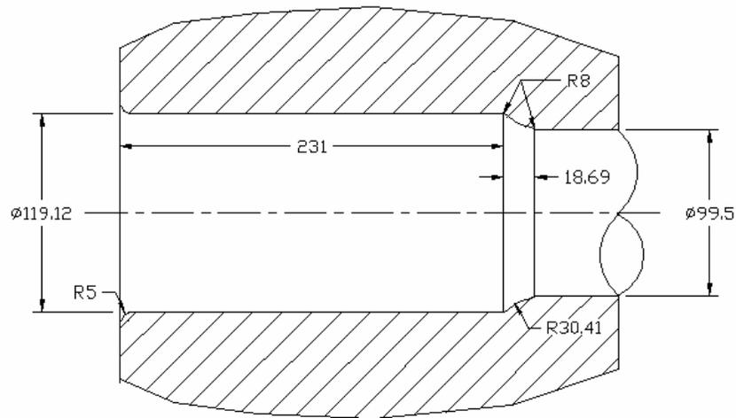
**Figure 4.29.** Modified gripper die of 2<sup>nd</sup> stage
