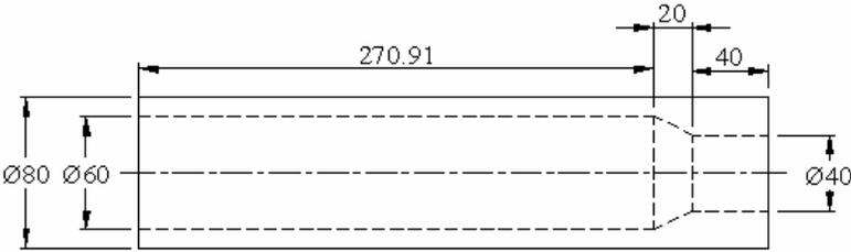
**Figure 5.3.** Shape of part for stage 1 [3]
