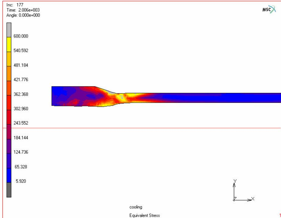
**Figure 6.11.** Equivalent stress distribution after cooling (MPa)
