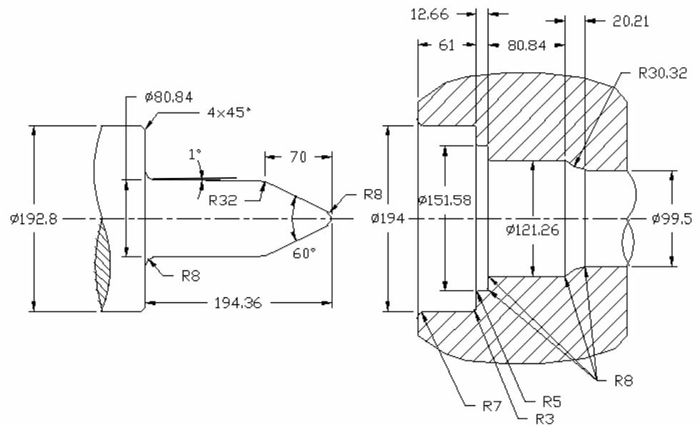
**Figure 4.16.** Header tool and gripper die of 4<sup>th</sup> stage [3]
