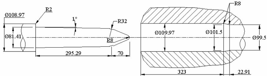
Figure 4.43. Header and gripper dies for 1<sup>st</sup> stage [3]
