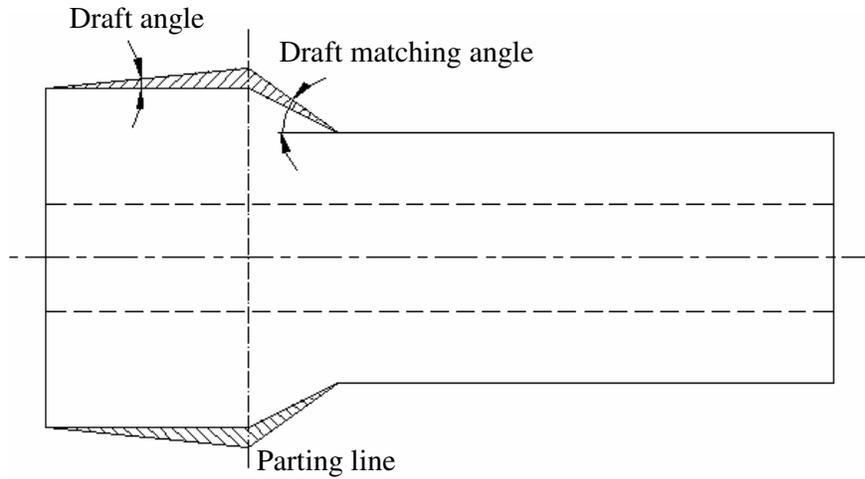
**Figure 2.1.** Draft angle and draft matching angle [3]
