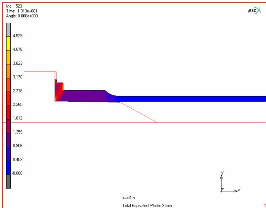
**Figure 4.36.** Total equivalent plastic strain distribution after 4<sup>th</sup> stage
