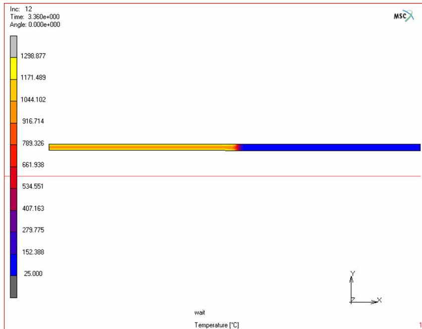
**Figure 4.20.** Temperature distribution after heating (°C)
