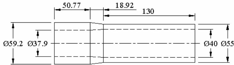
**Figure 6.3.** Shape of part for stage 1 [3]
