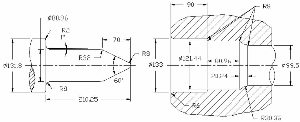
**Figure 4.15.** Header tool and gripper die of 3<sup>rd</sup> stage [3]
