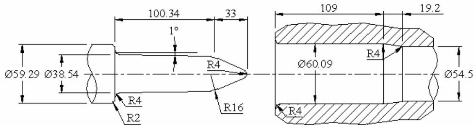
**Figure 6.4.** Header tool and gripper die of 1<sup>st</sup> stage [3]
