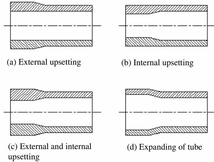
*Figure 1.3. Types of tube upsetting [3]*
