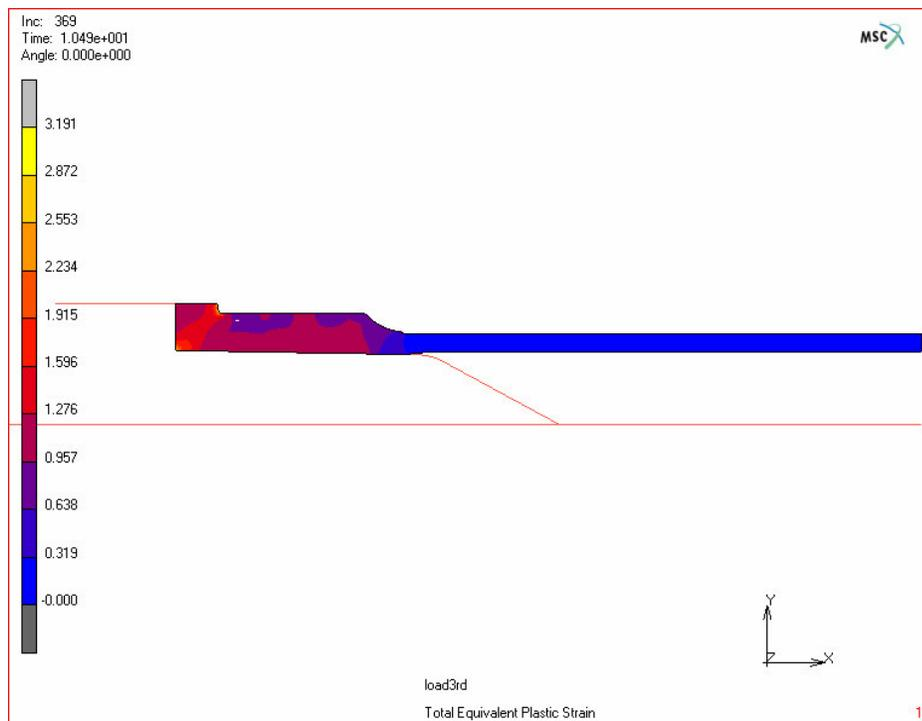
**Figure 4.34.** Total equivalent plastic strain distribution after 3<sup>rd</sup> stage
