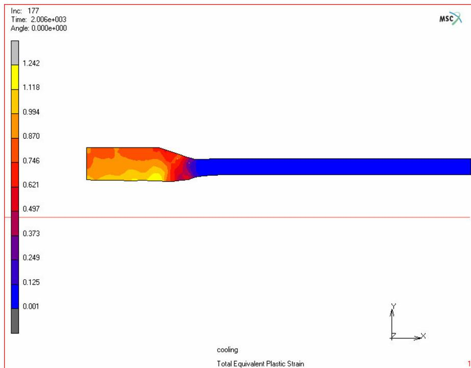
**Figure 6.10.** Total equivalent plastic strain distribution after cooling
