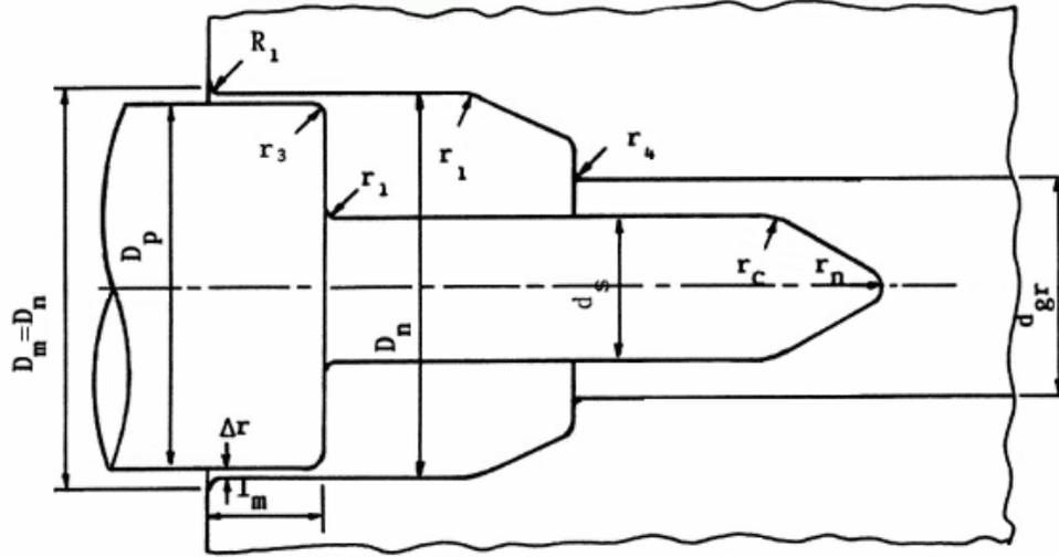
Figure 2.12. Die cavity in gripper dies for flashless forging [3]
