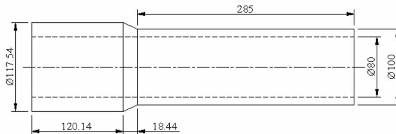
**Figure 4.10.** Shape of part for stage 2 [3]
