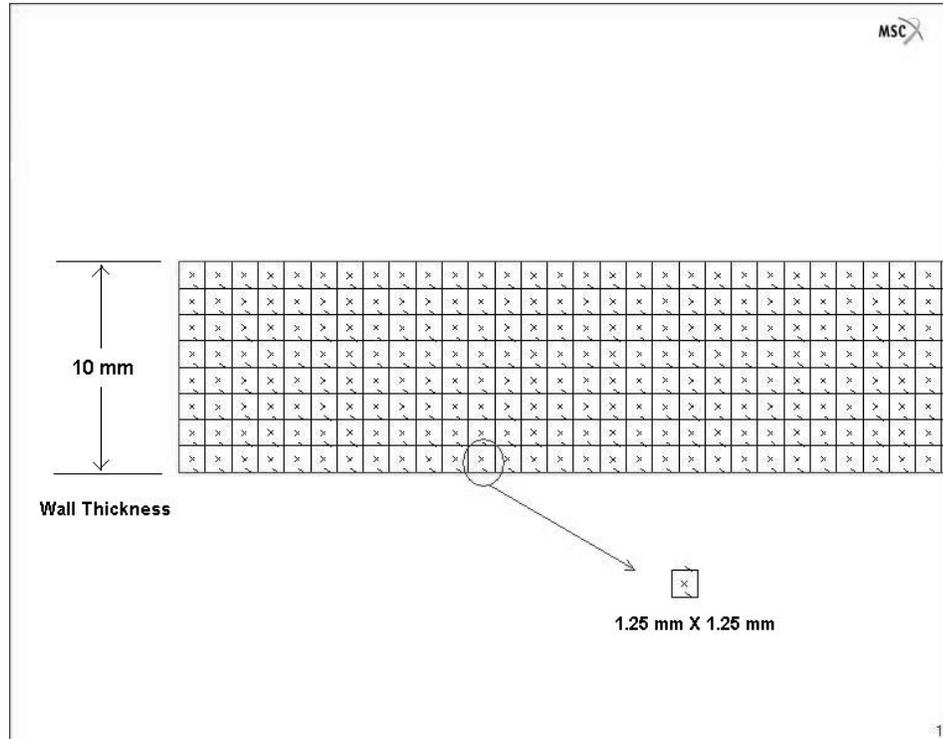
**Figure 4.18.** Elements used in the finite element model
