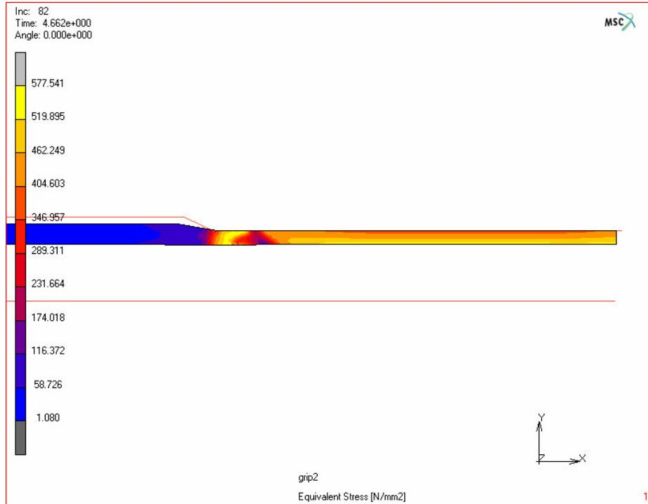
**Figure 4.22.** Equivalent stress distribution during gripping at 2<sup>nd</sup> stage (MPa)
