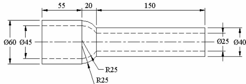
*Figure 7.1. A part requiring upsetting at both ends [3]*
