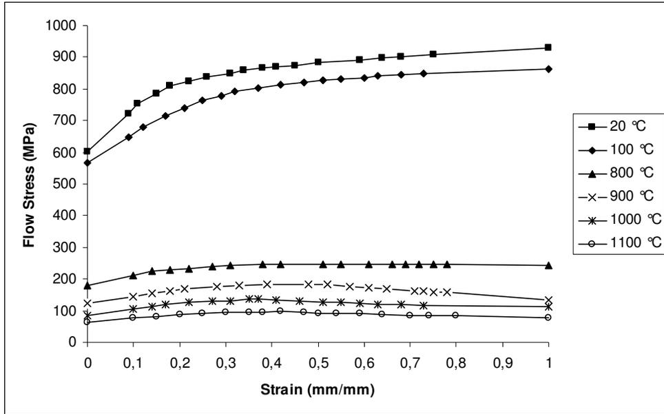
Figure 4.5. Flow stress-strain curves for 1/s strain rate [26]
