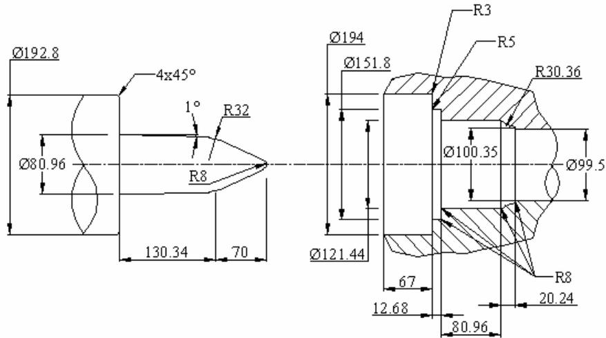
Figure 4.45. Header and gripper dies for 3<sup>rd</sup> stage [3]
