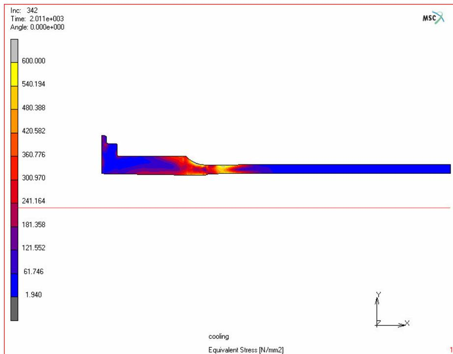
**Figure 4.50.** Equivalent stress distribution after cooling (MPa)
