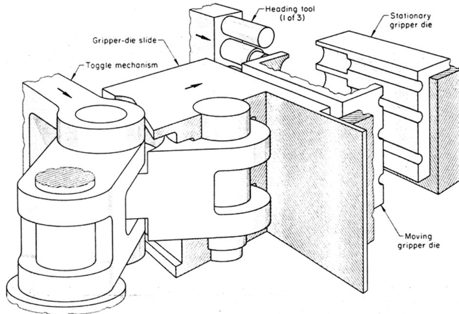
**Figure 1.2.** Basic actions of the gripper dies and heading tools of an upsetter [1]
