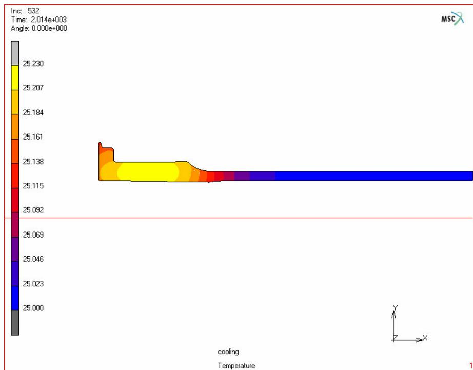
**Figure 4.39.** Temperature distribution after cooling stage (°C)
