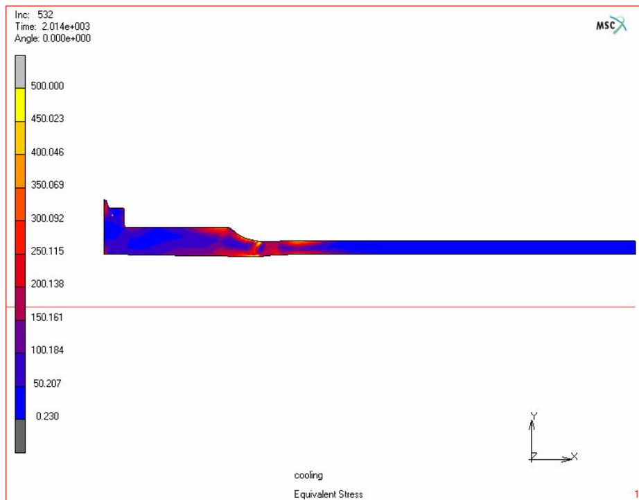
**Figure 4.41.** Equivalent stress distribution at the end of the analysis (MPa)
