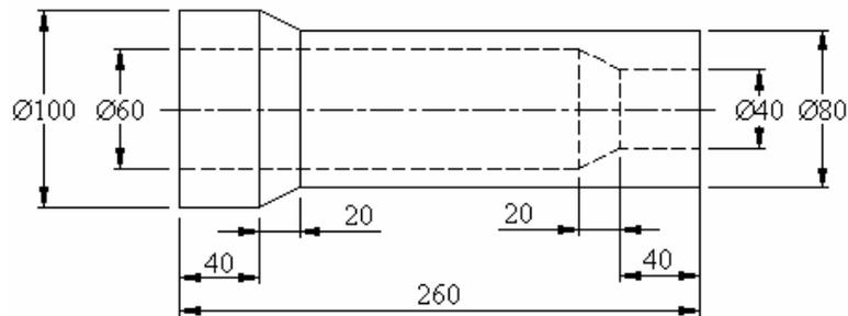
*Figure 5.1. A part requiring upsetting at both ends [3]*
