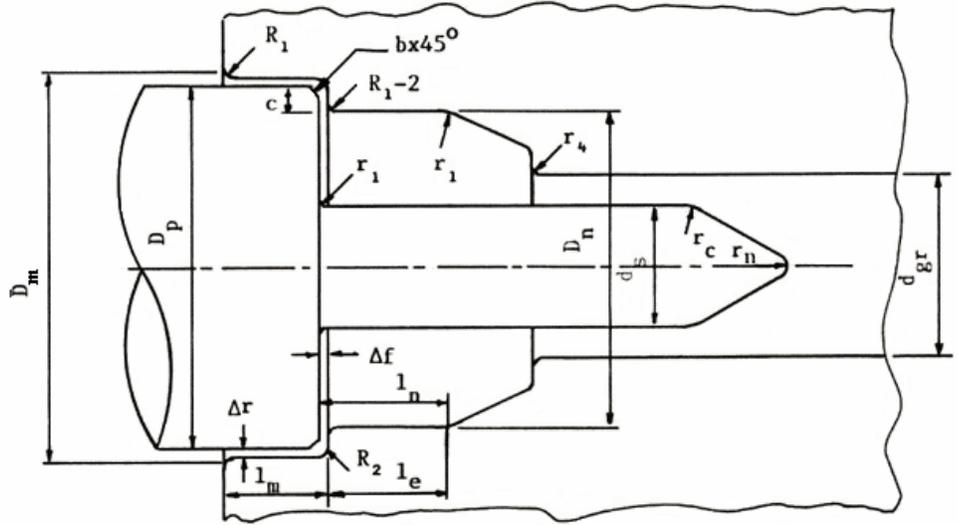
Figure 2.13. Die cavity in gripper die for forging with flash [3]
