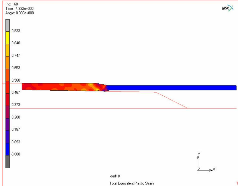
**Figure 4.47.** Total equivalent plastic strain distribution after 1<sup>st</sup> stage
