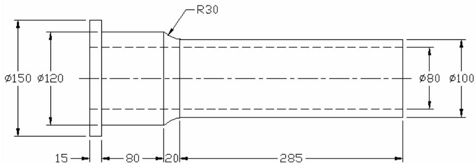
Figure 4.6. A part flanged at one end [3]
