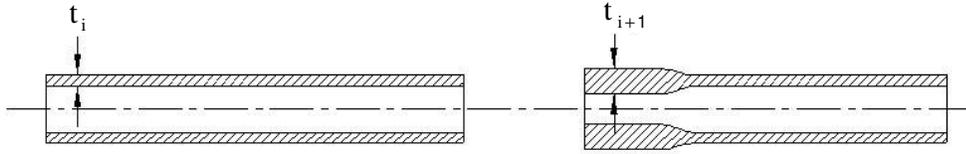
**Figure 2.6.** Wall thickness change during simultaneous internal and external upsetting
