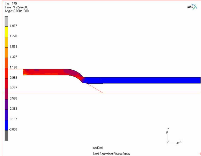
**Figure 7.8.** Total equivalent plastic strain distribution after 2<sup>nd</sup> stage
