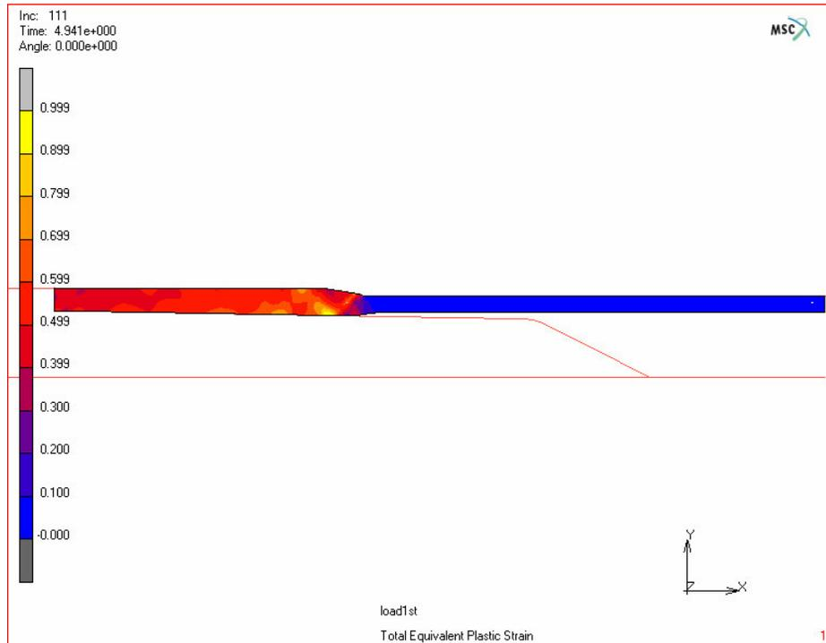
**Figure 4.30.** Total equivalent plastic strain distribution after 1<sup>st</sup> stage
