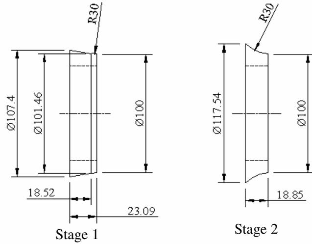
**Figure 4.25.** Shape of Sub-region C for Stages 1 and 2
