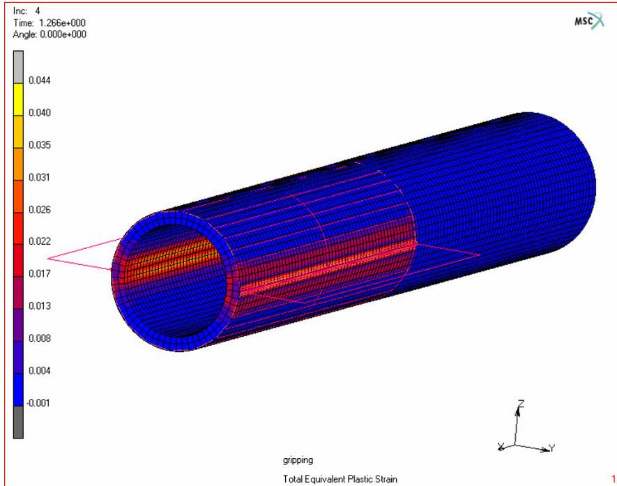
**Figure A.2.** Total equivalent plastic strain distribution at the end of gripping
