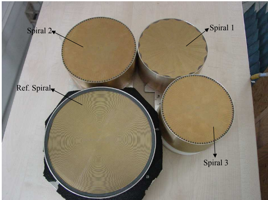
Figure 5.1 Spiral antennas designed for this study and reference spiral
