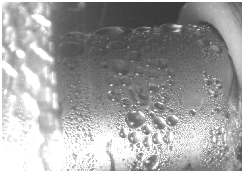
Figure 4.12 Dropwise condensation on the gold coated condenser surface
