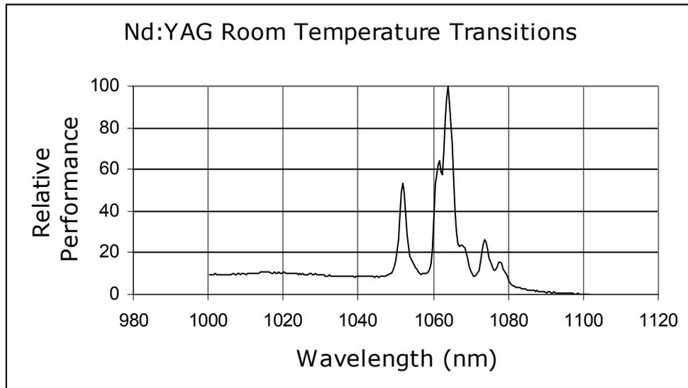
Figure-4.2: Measured Nd:YAG room temperature transitions above 1000nm.
