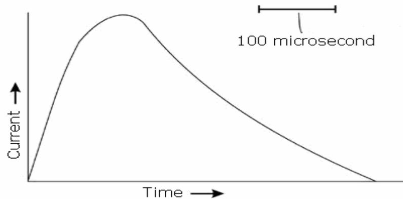
Figure-2.8: Typical waveform for a flashlamp current pulse lasting a few hundred microseconds.
