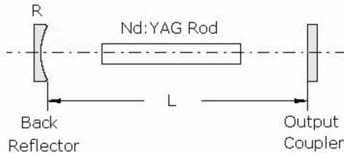
Figure-3.11: Hemispherical resonator.  $R = 2.0$  m.
