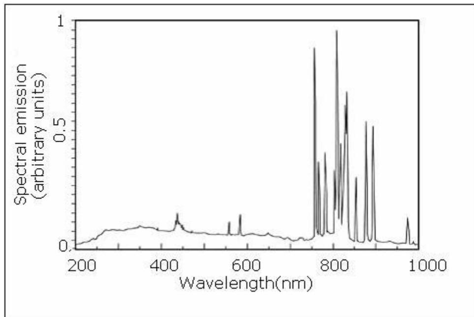
Figure-3.18: Spectral emission of krypton filled flash lamp pressure of 700 torr at low electrical loading (100-microfarad capacitor charged to 500 V).
