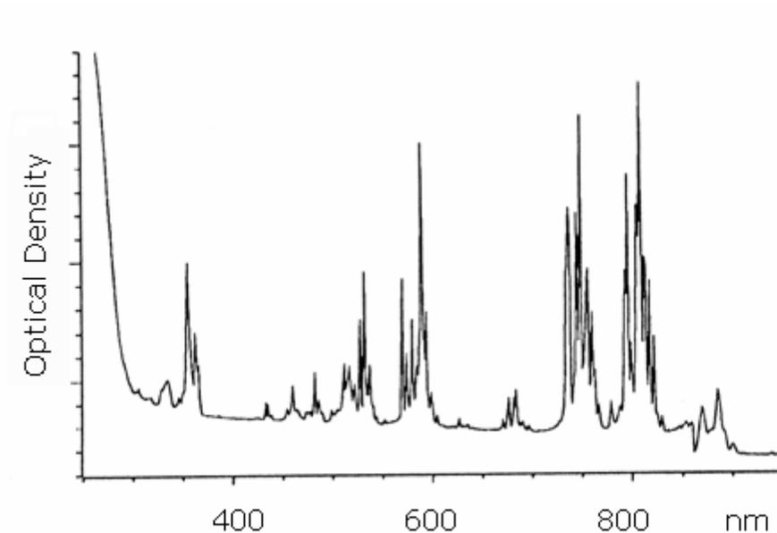
Figure-2.5: Spectral absorption of Nd:YAG
