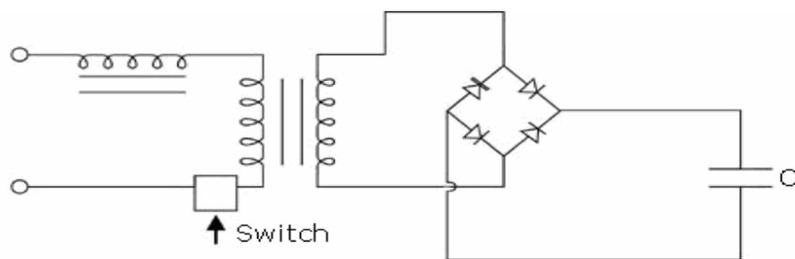
Figure-3.23: Charging supply with current limiting inductor.
