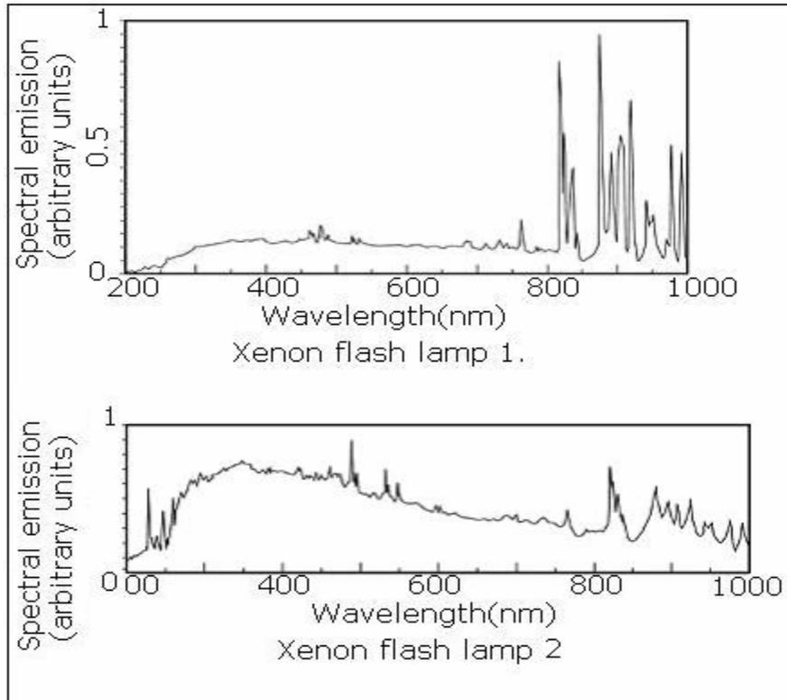
Figure-3.17: 1. Spectral emission from xenon flashlamp filled to a pressure of 390 torr at low electrical loading (100-microfarad capacitor charged to 500 V). 2. Spectral emission from xenon flashlamp filled to a pressure of 390 torr at high electrical loading (200-microfarad capacitor charged to 1000 V).
