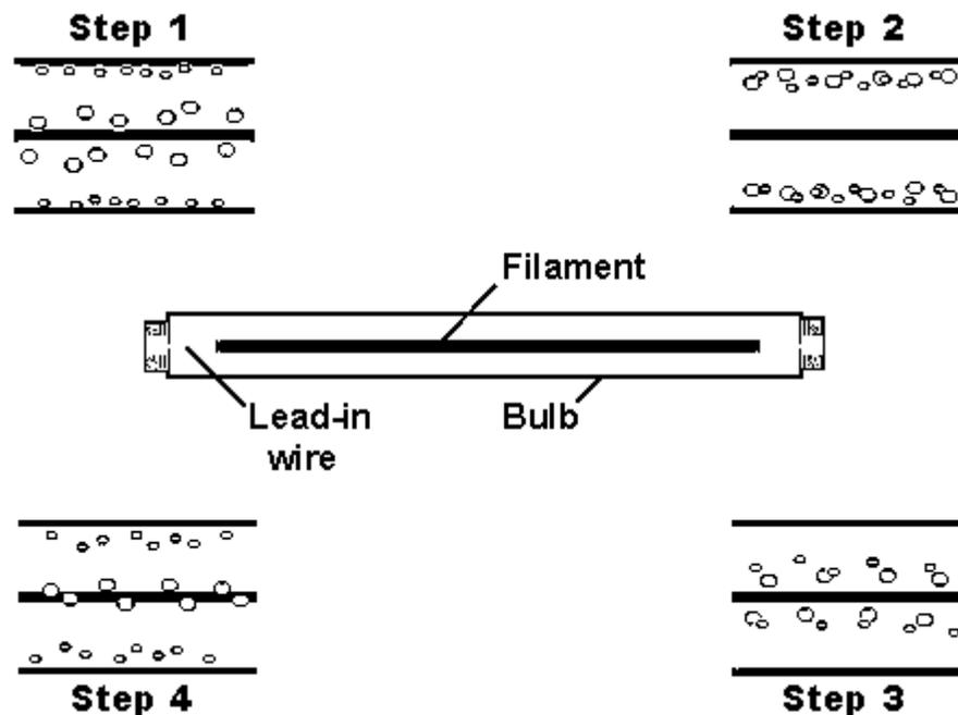
Figure-2.9: Tungsten halogen lamp and halogen cycle.
