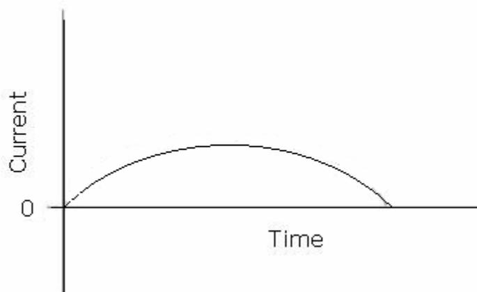
Figure-0.31: Overdamped current waveform from a flashlamp discharge circuit.
