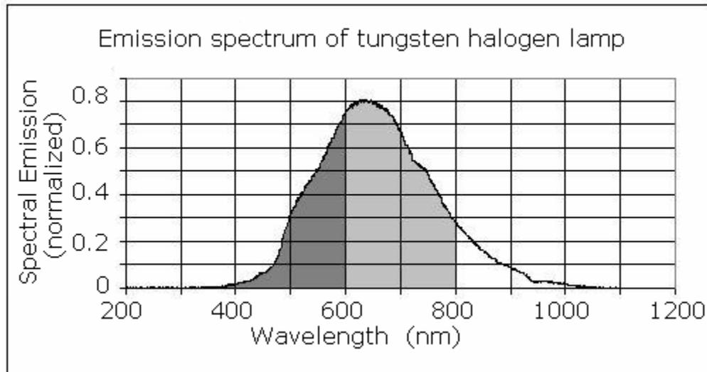
Figure-3.19: Spectral emission of tungsten halogen lamp 5 minutes later after it is initiated.
