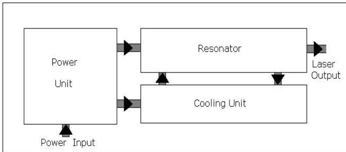
Figure-3.10: Block diagram showing a typical laser
