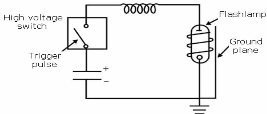
Figure-3.25: Overvoltage trigger circuit.
