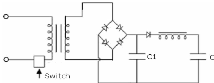
Figure-3.24: Charging supply with resonant charging unit.
