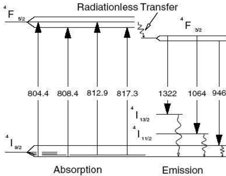
Figure-2.1.: Absorption and emission levels of Nd:YAG
