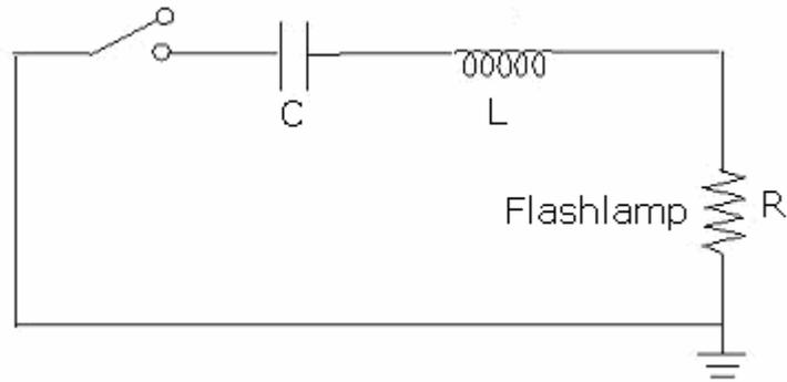
Figure-3.29: RLC discharge circuit
