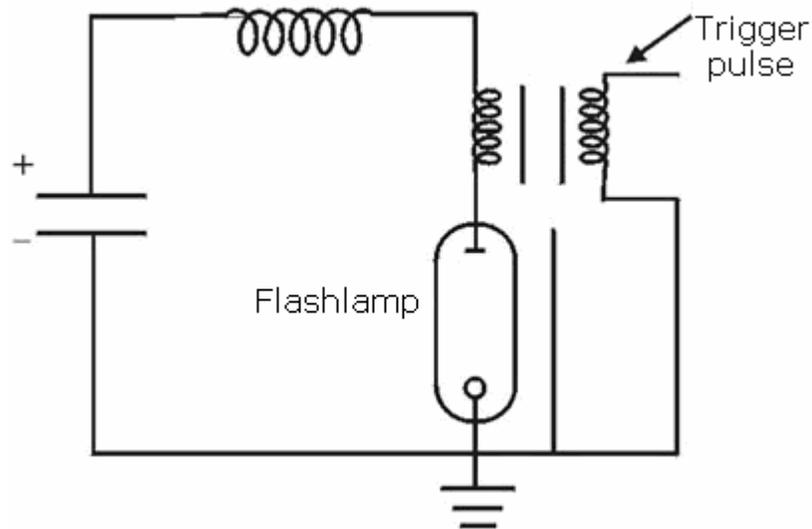
Figure-3.27: Series trigger circuit
