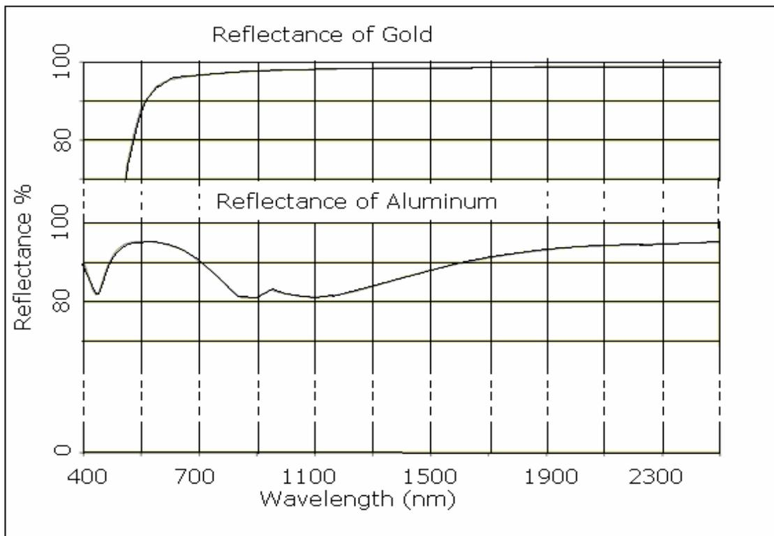
Figure-3.16: Spectral reflectance of gold and aluminum.
