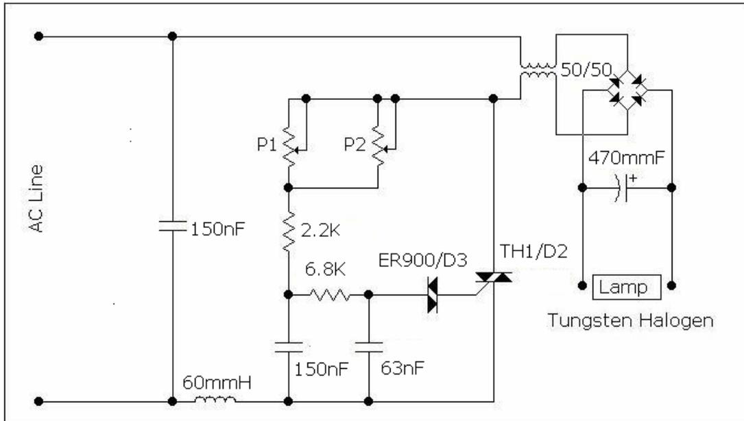
Figure-3.34: Tungsten halogen lamp power supply.
