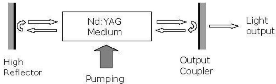
Figure-2.4: Gain process, resonator and Nd:YAG medium
