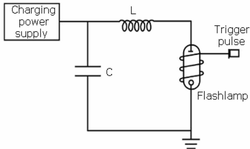
Figure-3.20: A prototype supply for flash lamp operation.
