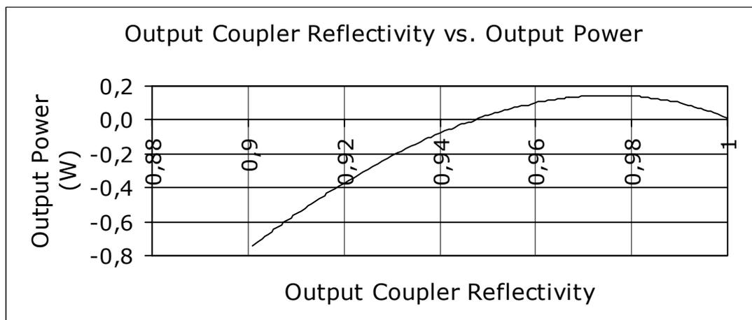
Figure-4.3: Power dependence of output coupler reflectivity.
