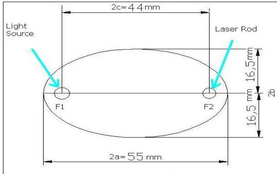
Figure-3.14: Cross section of elliptical cavity with small eccentricity.
