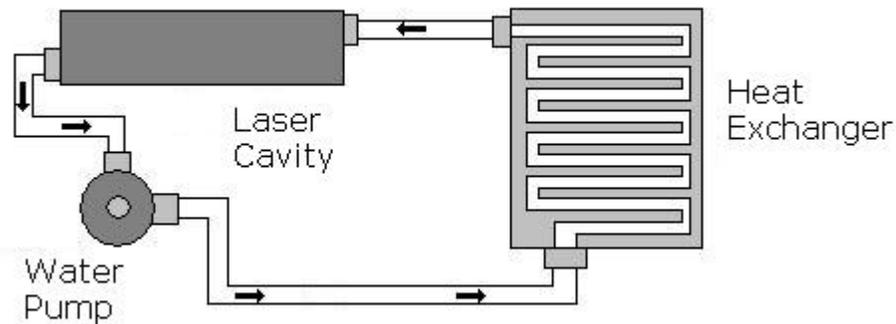
Figure-3.35: Closed loop cooling system.
