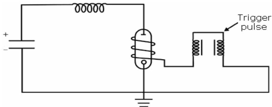
Figure-3.26: External trigger circuit
