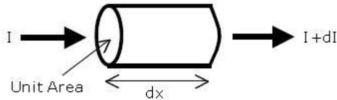
Figure-2.3: Gain in laser medium
