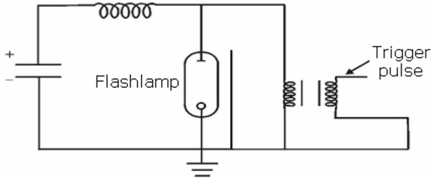
Figure-3.28: Parallel trigger circuit
