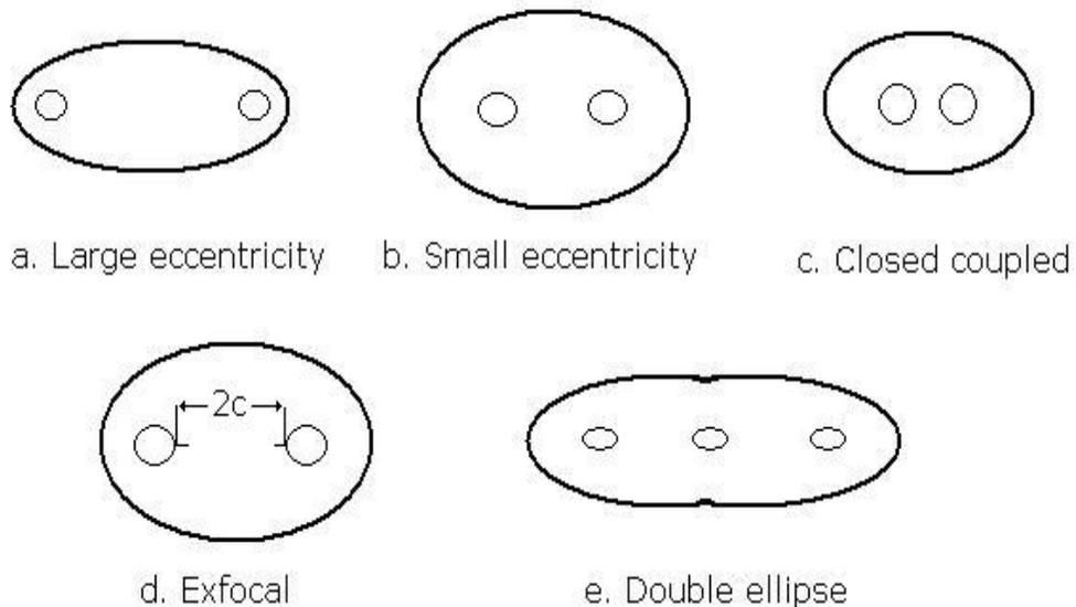
Figure-3.12: Elliptical pump cavities.
