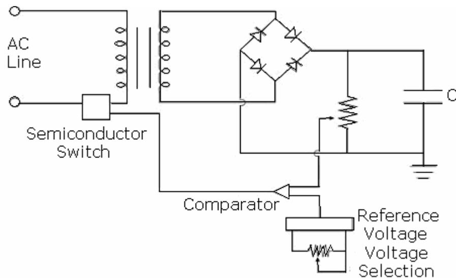
Figure-3.21: Charging supply with SCR control.
