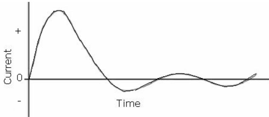
Figure-3.30: Underdamped current waveform from a flashlamp discharge circuit.
