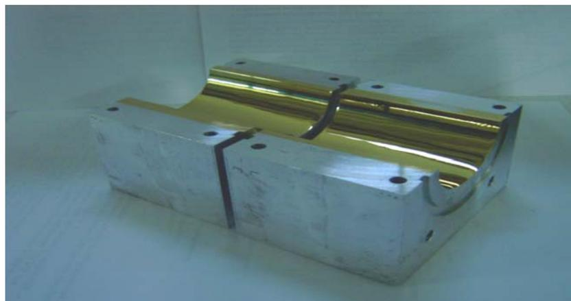
Figure-3.15: Elliptical cylinder cavity; upper and lower sides together.
