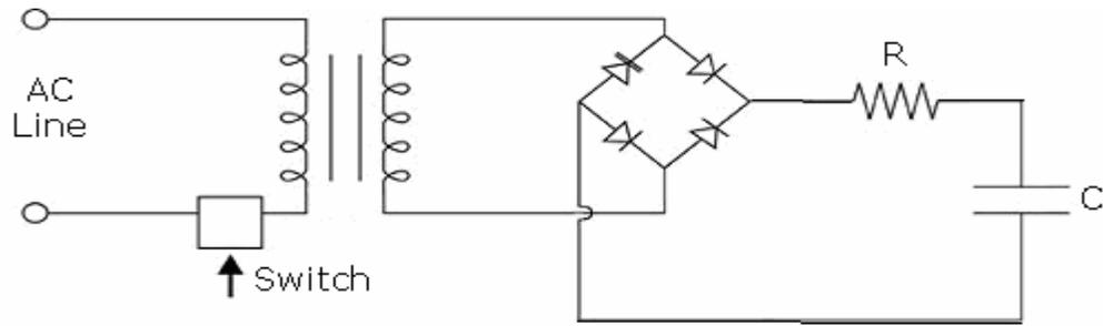
Figure-3.22: Charging supply with current limiting resistor.
