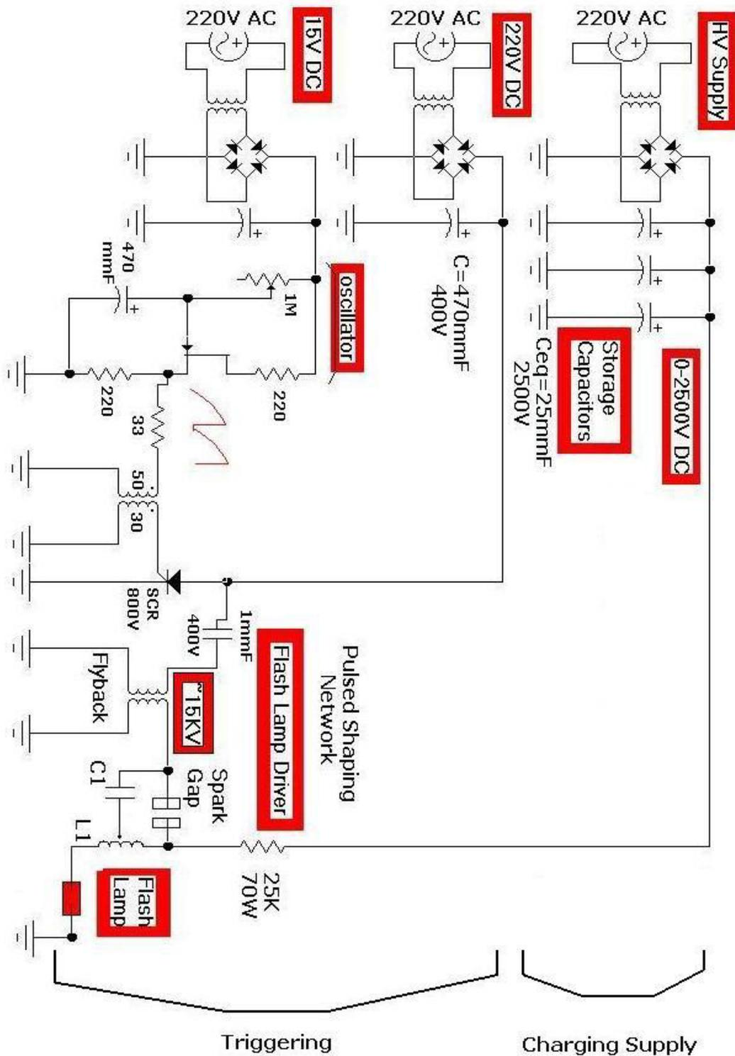
Figure-3.33: Designed and constructed pulsed Nd:YAG Laser flash lamp electronics. Charging supply, triggering and pulse shaping circuits.
