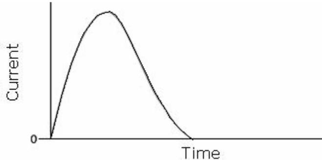
Figure-3.32: Critically damped current waveform from a flashlamp discharge circuit.
