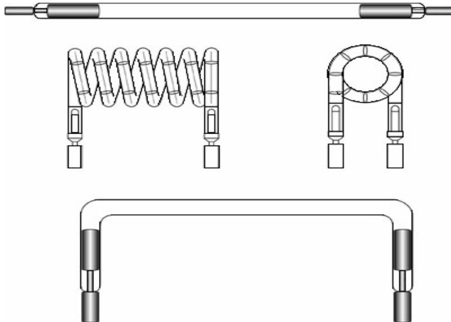
Figure-2.6: Flash lamps with various geometries.
