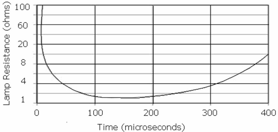
Fig-2.7: Typical behavior of the electrical resistance of a small flashlamp during a current pulse with duration of a few hundred microseconds[8].
