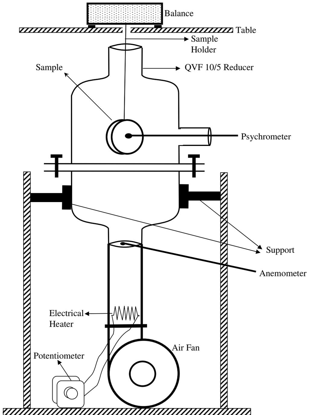
**Figure 2.1** Schematic Drawing of the Laboratory Batch Dryer
