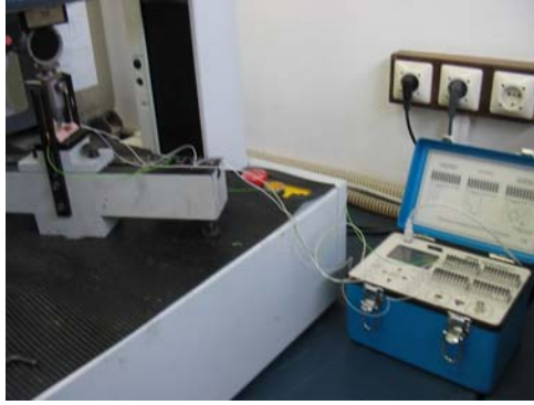
(c) Lloyd Universal Standard Testing Machine and Vishay Strain Indicator
