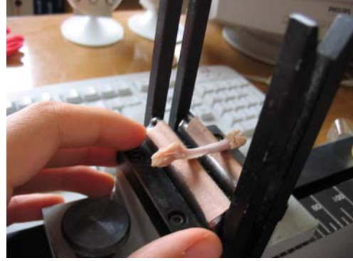
(d) Lloyd Three Point Bending Set Up and Custom Made Roller Supports
