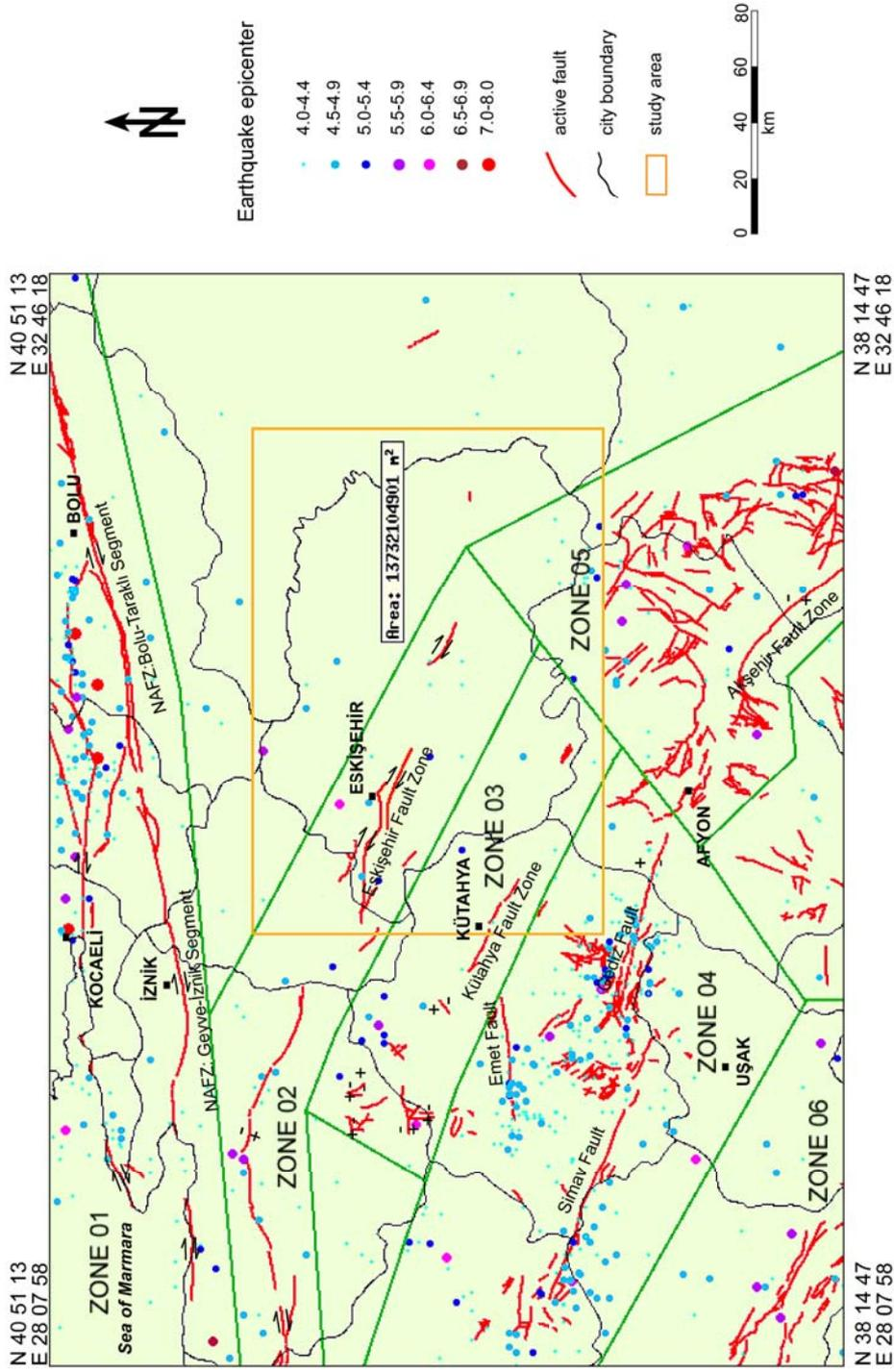
**Figure 6.1.** Seismic Source Zones.
