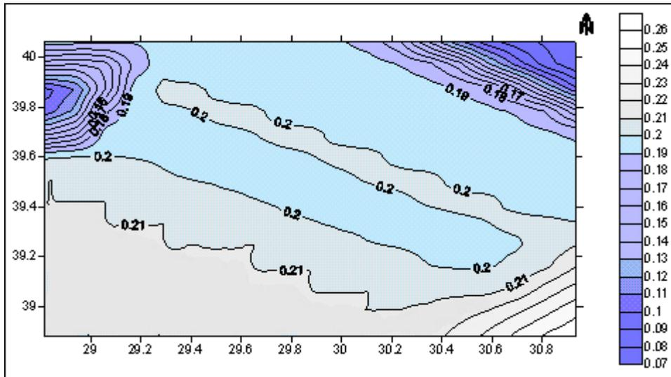
**Figure 8.3.** PSH Map for rock sites based on Ambraseys et al. attenuation relationship (1996) (475-year return period)
