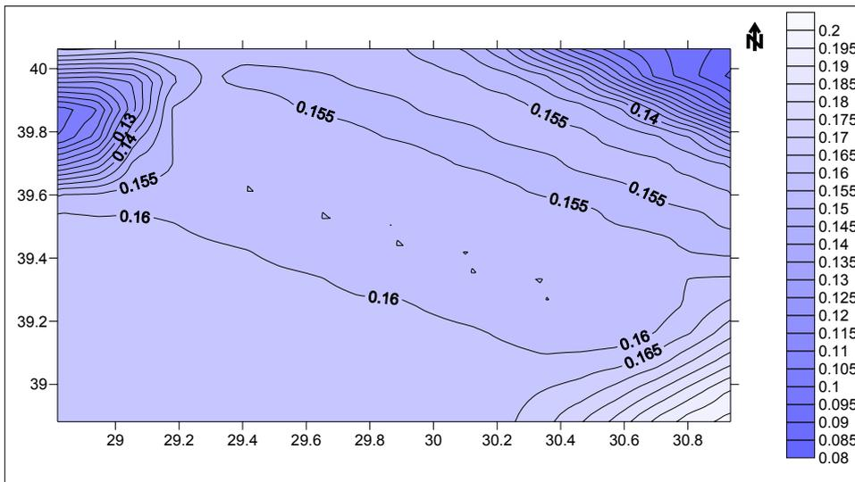
**Figure 8.2.** PSH Map for rock sites based on Boore et al. attenuation relationship (1997) (475-year return period)
