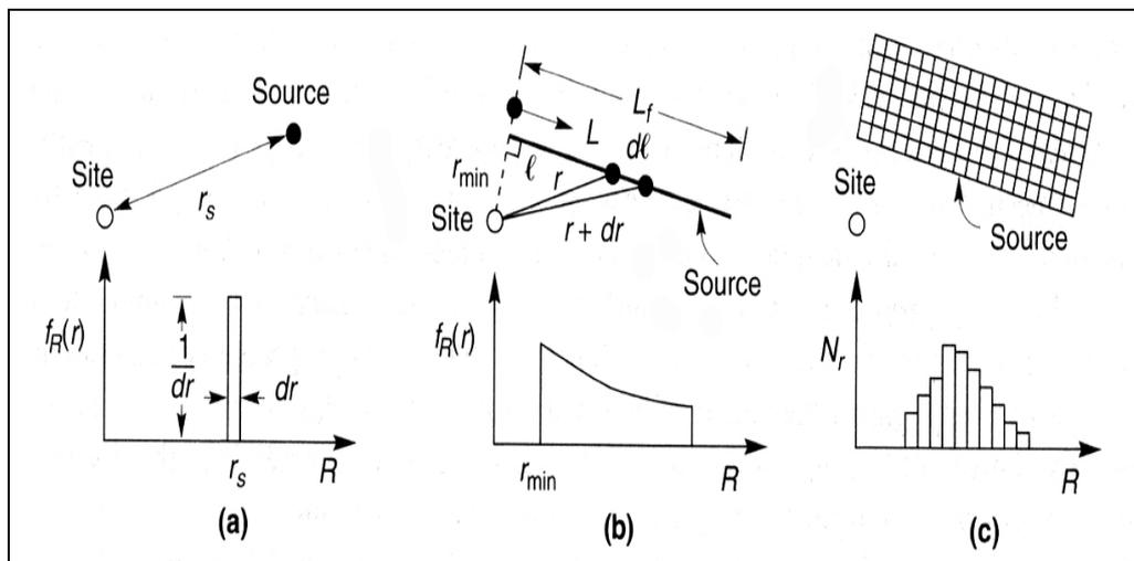
**Figure 3.3.** Examples of variations of source-to-site distance for different source zone geometries (Kramer,1996)
