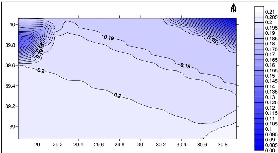
**Figure 8.8.** PSH Map for rock sites based on Gülkan and Kalkan attenuation relationship (2002) (1000-year return period)
