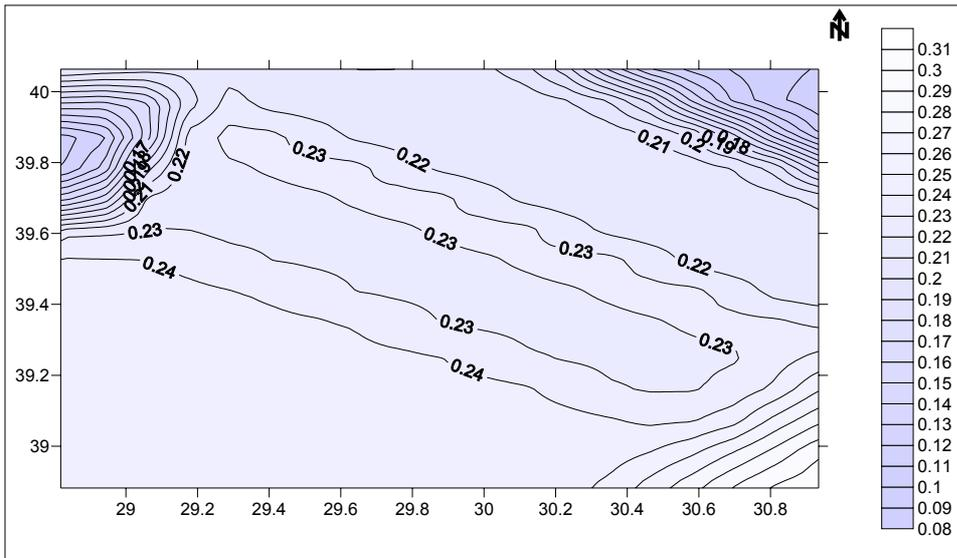
**Figure 8.1.** PSH Map for rock sites based on Abrahamson and Silva attenuation relationship (1997) (475-year return period)
