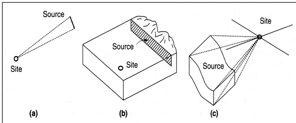
**Figure 3.2.** Examples of some of the source zone geometries (a) short fault modeled as a point source; (b) shallow fault modeled as a linear source; (c) three-dimensional source zone (Kramer, 1996).
