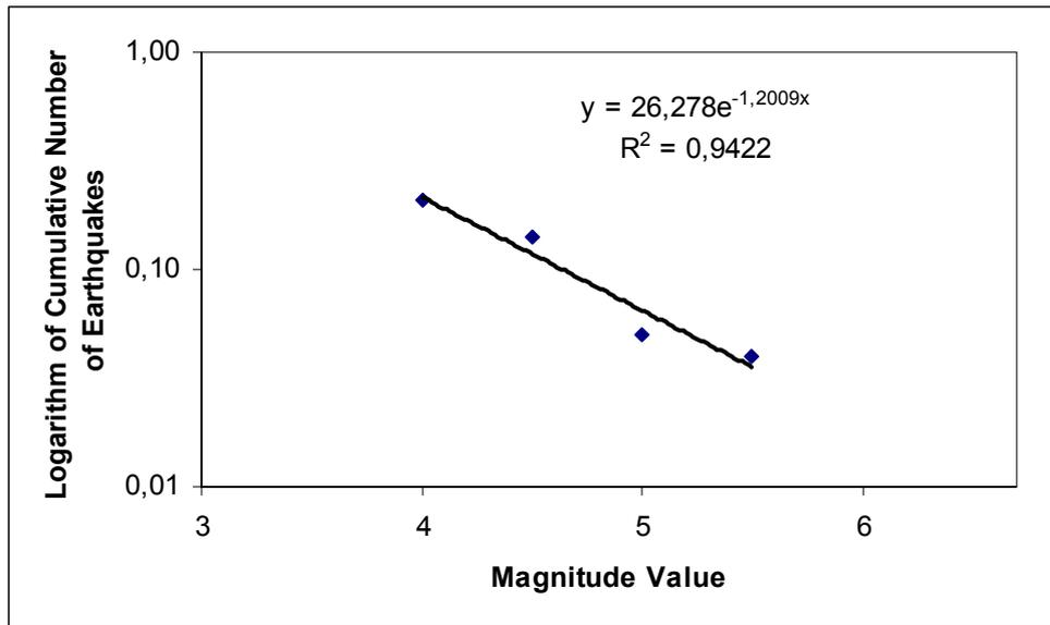
**Figure 6.7.** Gutenberg-Richter recurrence relationship curve for source zone 6 (Gediz Graben System)
