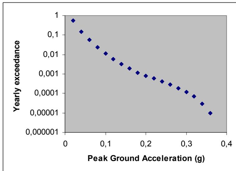
**Figure 8.12.** PGA Hazard Curve based on Boore et al. attenuation relationship (1997) for rock sites
