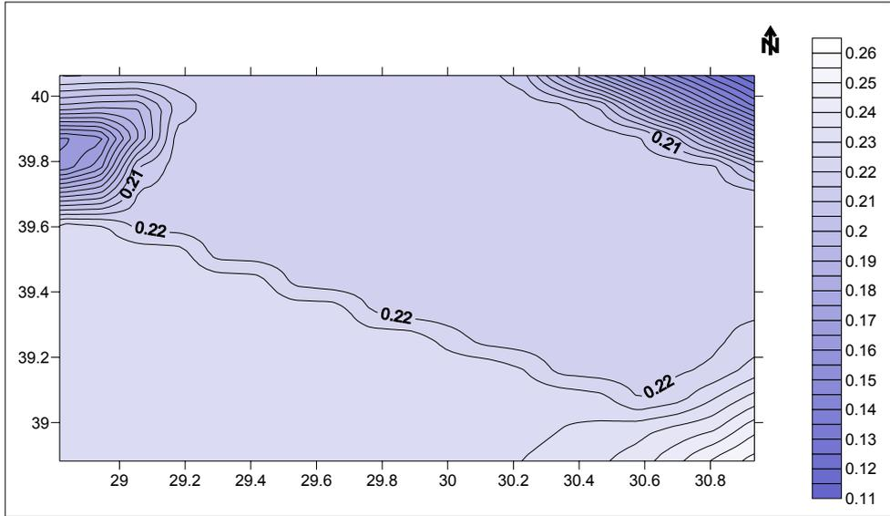
**Figure 8.23.** PSH map for site class D ( $V_s=250$  m/s) based on Boore et al. attenuation relationship (1997) (475-year return period)
