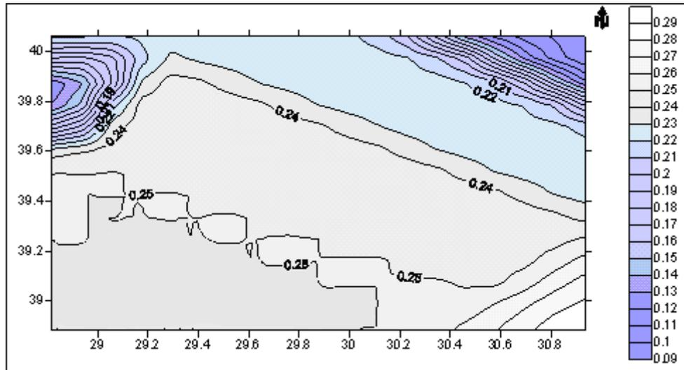
**Figure 8.22.** PSH Map by logic tree method with Boore et al. (1997) and Abrahamson and Silva (1997) attenuation relationships with a minimum magnitude variation for rock sites (1000-year return period)
