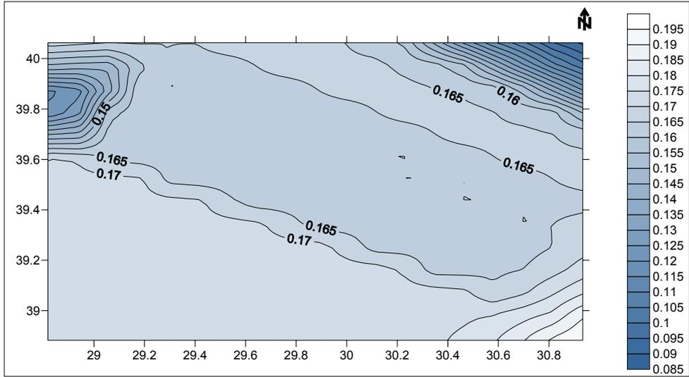
**Figure 8.25.** PSH map for site class C ( $V_s=520$  m/s) based on Boore et al. attenuation relationship (1997) (475-year return period)
