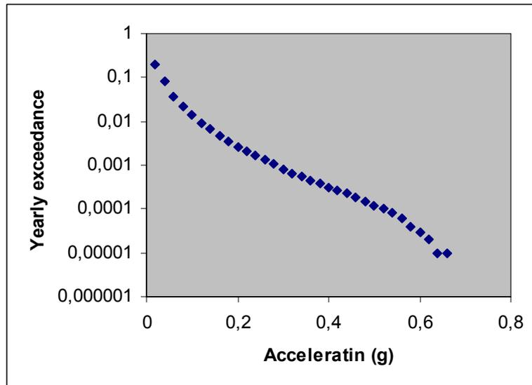
**Figure 8.11.** PGA Hazard Curve based on Abrahamson and Silva attenuation relationship (1997) for rock sites
