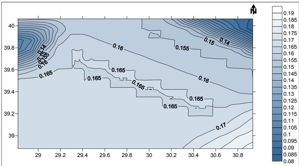
**Figure 8.19.** PSH Map based on Boore et al. attenuation relationship (1997) with a minimum magnitude variation for rock sites (475-year return period)
