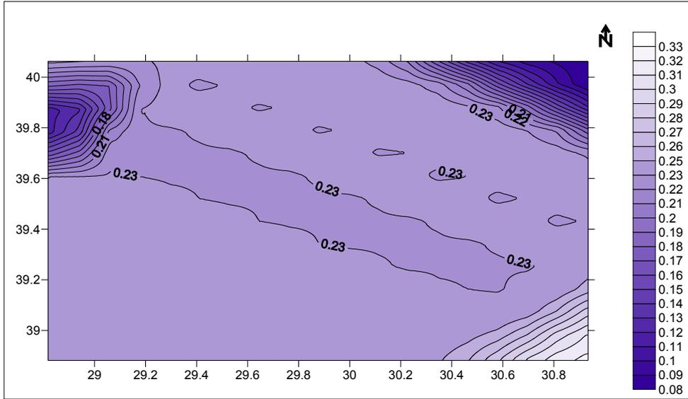
**Figure 8.7.** PSH Map for rock sites based on Ambraseys et al. attenuation relationship (1996) (1000-year return period)
