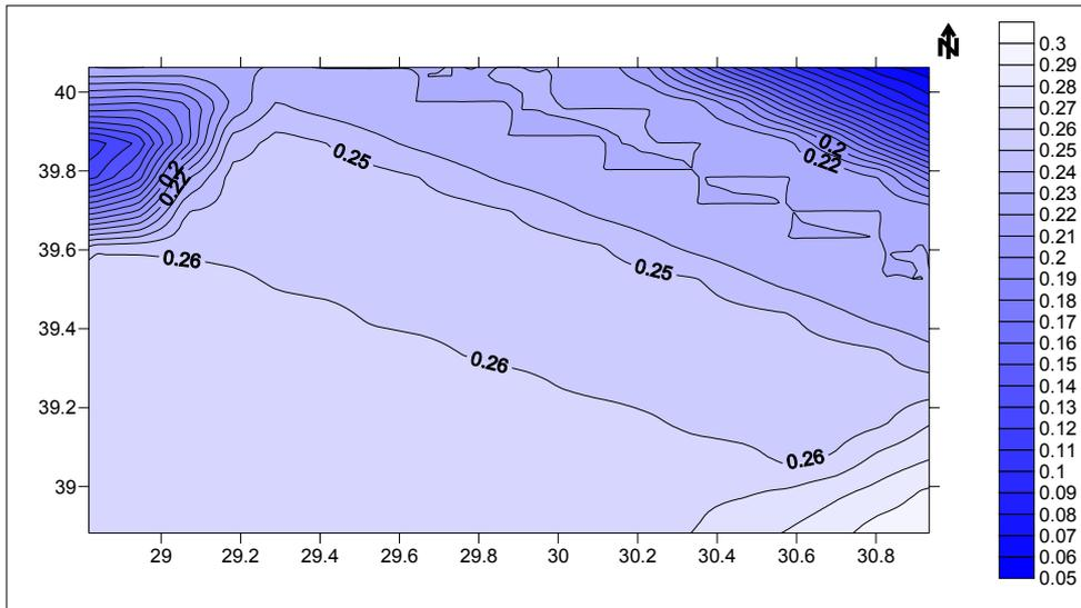
**Figure 8.29.** PSH map for 'stiff' site class based on Ambraseys et al. attenuation relationship (1996) (475-year return period)
