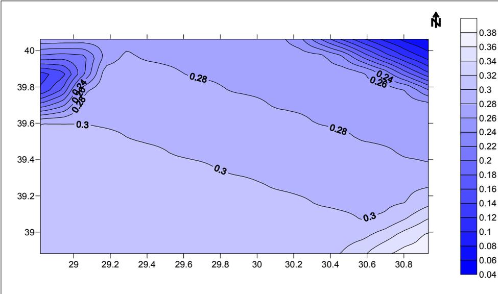
**Figure 8.28.** PSH map for 'soft' site class based on Ambraseys et al. attenuation relationship (1996) (1000-year return period)
