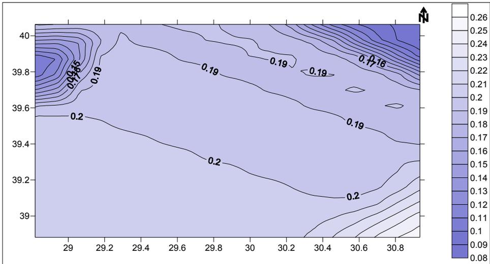
**Figure 8.9.** PSH Map for rock sites by Logic Tree method for 475 year return period
