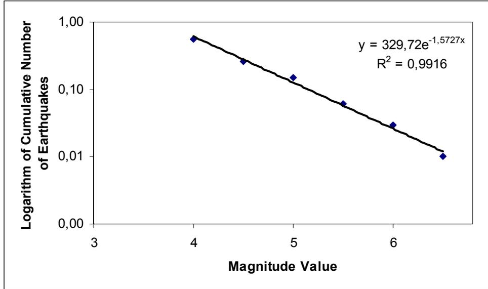
**Figure 6.6.** Gutenberg-Richter recurrence relationship curve for source zone 5 (Akşehir-Afyon Graben System)
