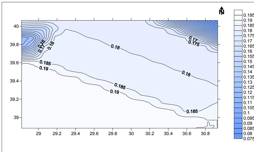
**Figure 8.4.** PSH Map for rock sites based on Gülkan and Kalkan attenuation relationship (2002) (475-year return period)
