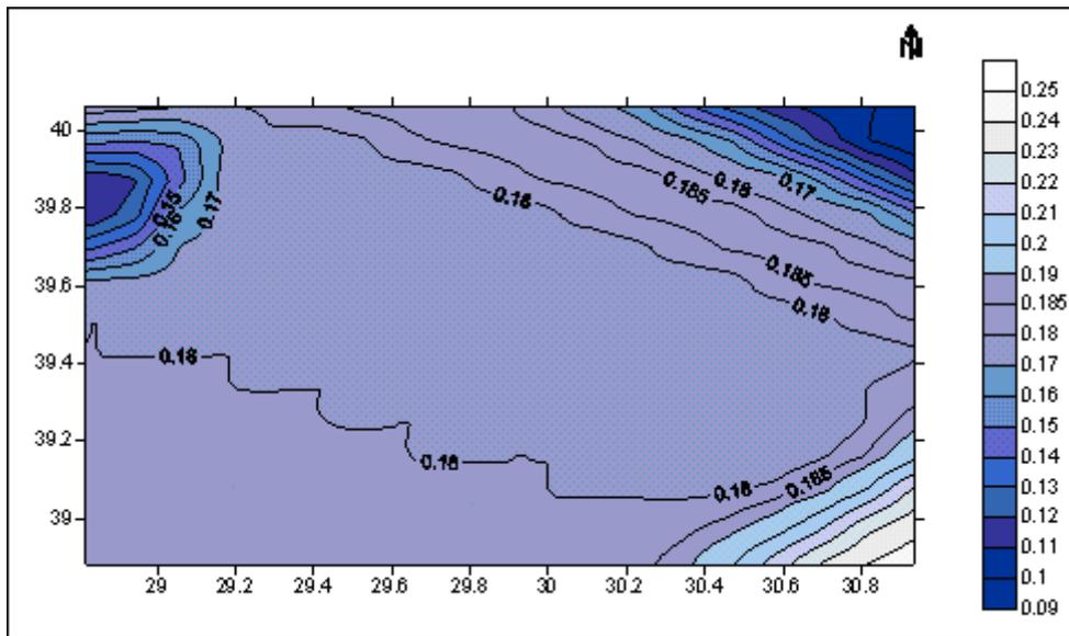
**Figure 8.6.** PSH Map for rock sites based on Boore et al. attenuation relationship (1997) (1000-year return period)
