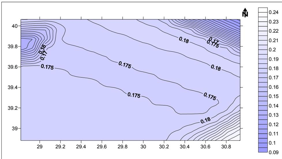
**Figure 8.26.** PSH map for site class C ( $V_s=520$  m/s) based on Boore et al. attenuation relationship (1997) (1000-year return period)
