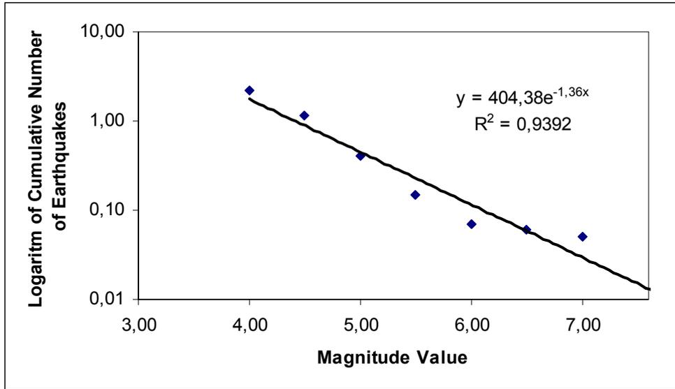
**Figure 6.2.** Gutenberg-Richter recurrence relationship curve for source zone 1
