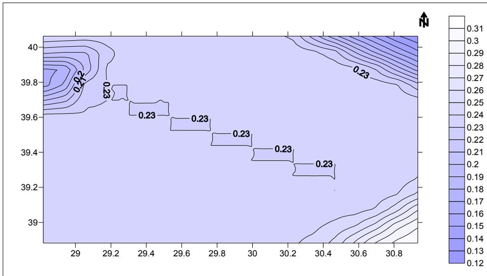
**Figure 8.24.** PSH map for site class D ( $V_s=250$  m/s) based on Boore et al. attenuation relationship (1997) (1000-year return period)
