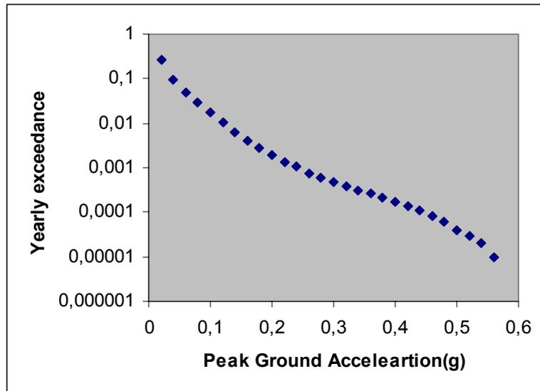
**Figure 8.13.** PGA Hazard Curve based on Ambraseys et al. attenuation relationship (1996) for rock sites
