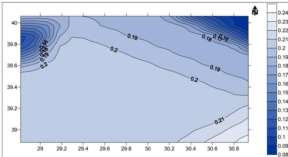
**Figure 8.21.** PSH Map by logic tree method with Boore et al. (1997) and Abrahamson and Silva (1997) attenuation relationships with a minimum magnitude variation for rock sites (475-year return period)
