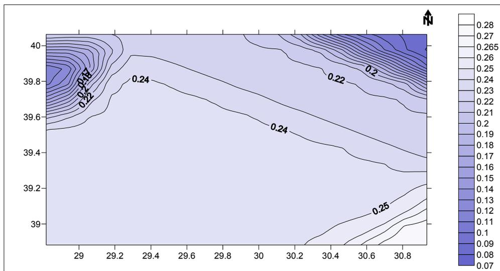
**Figure 8.17.** PSH Map based on Abrahamson and Silva attenuation relationship (1997) with a minimum magnitude variation for rock sites (475-year return period)
