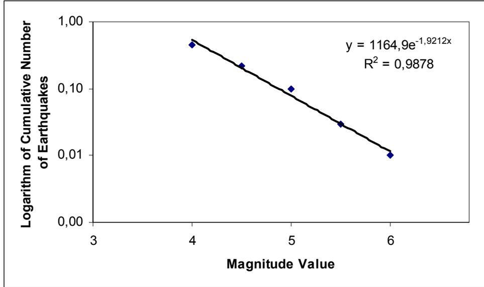
**Figure 6.3.** Gutenberg-Richter recurrence relationship curve for source zone 2 (Eskişehir Fault Zone).
