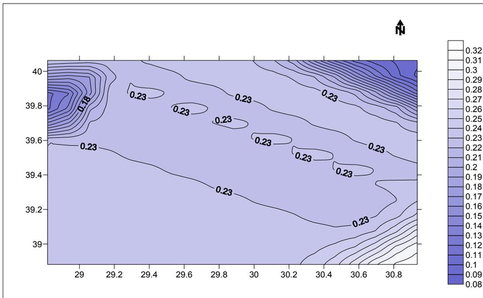
**Figure 8.10.** PSH Map for rock sites by Logic Tree method for 1000 year return period
