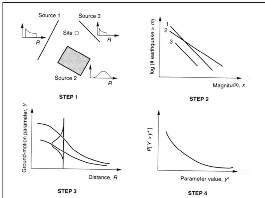
**Figure 3.1.** Four Steps of a probabilistic seismic hazard analysis (Kramer, 1996).
