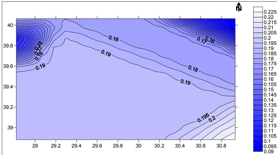
**Figure 8.20.** PSH Map based on Boore et al. attenuation relationship (1997) with a minimum magnitude variation for rock sites (1000-year return period)
