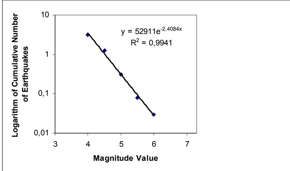
**Figure 6.5.** Gutenberg-Richter recurrence relationship curve for source zone 4 (Simav Graben System).
