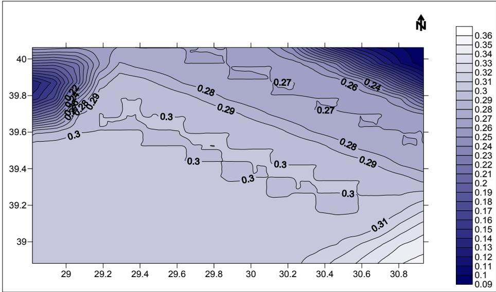
**Figure 8.18.** PSH Map based on Abrahamson and Silva attenuation relationship (1997) with a minimum magnitude variation for rock sites (1000-year return period)
