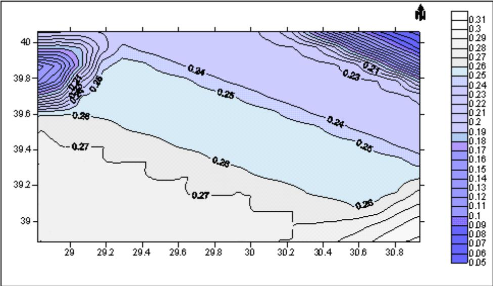
**Figure 8.27.** PSH map for 'soft' site class based on Ambraseys et al. attenuation relationship (1996) (475-year return period)
