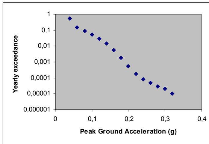
**Figure 8.14.** PGA Hazard Curve based on Gülkan and Kalkan attenuation relationship (2002) for rock sites
