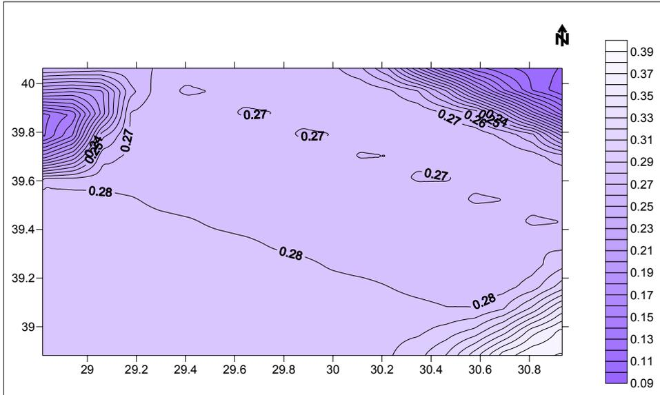
**Figure 8.5.** PSH Map for rock sites based on Abrahamson and Silva attenuation relationship (1997) (1000-year return period)
