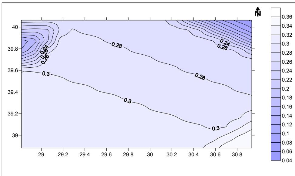
**Figure 8.30.** PSH map for 'stiff' site class based on Ambraseys et al. attenuation relationship (1996) (1000-year return period)
