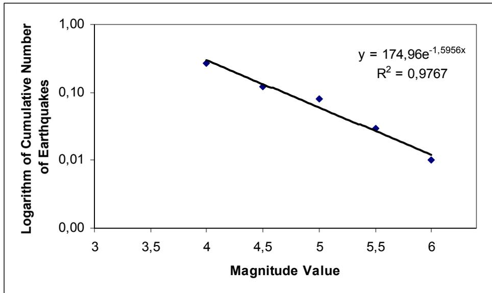
**Figure 6.4.** Gutenberg-Richter recurrence relationship curve for source zone 3 (Kütahya Fault zone).
