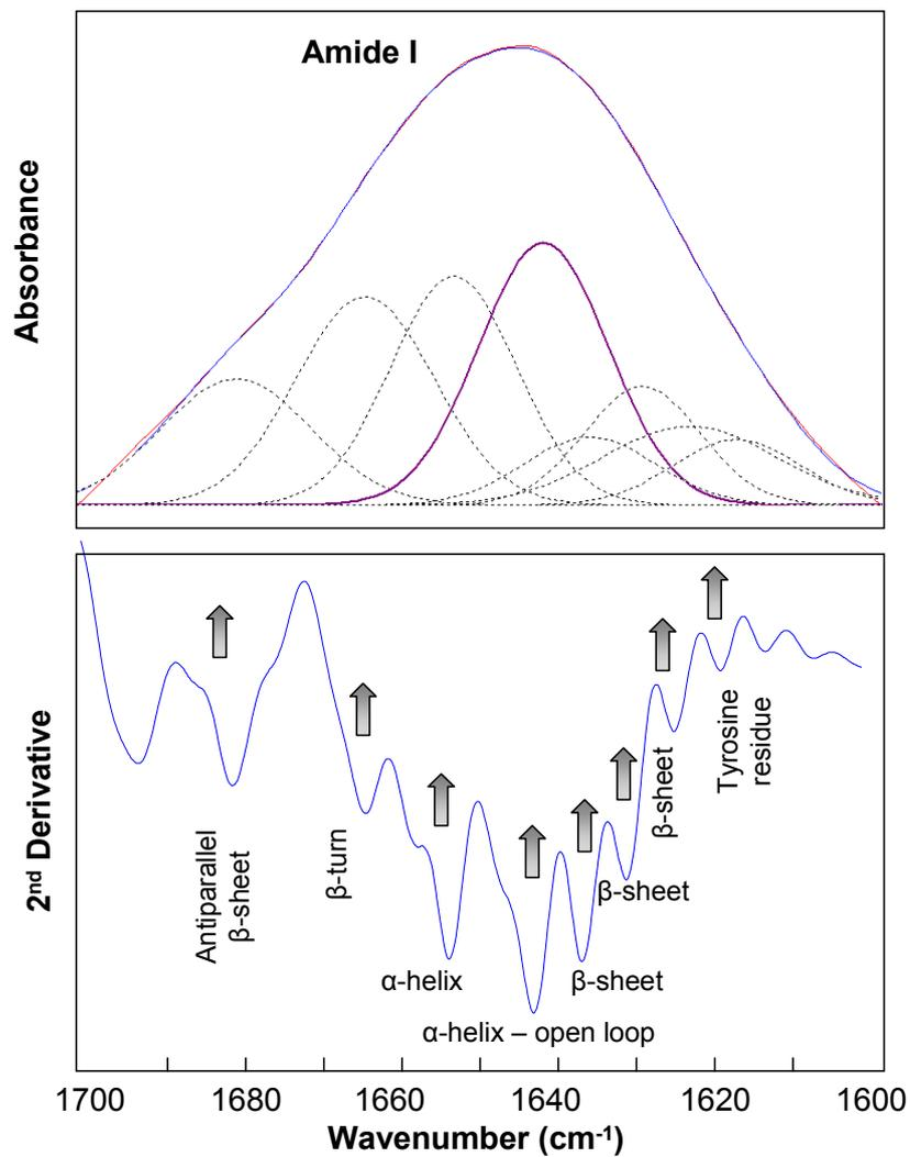
**Figure 4.16.** Curve fitting analysis (upper part) and second derivative spectrum (lower part) of GST-E4orf3 Amide I band. Arrows indicate the location of the sub-bands and their corresponding secondary structures.
