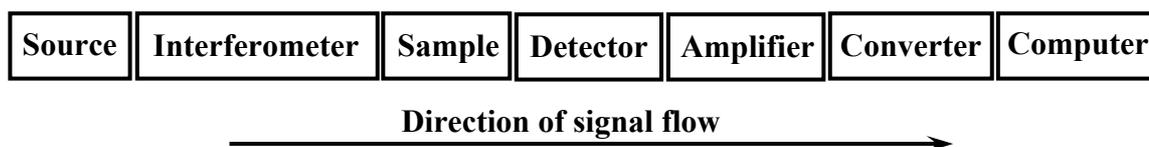
**Figure 2.9.** The schematic instrumentation of the components of an FTIR spectrometer (Stuart, 1997).
