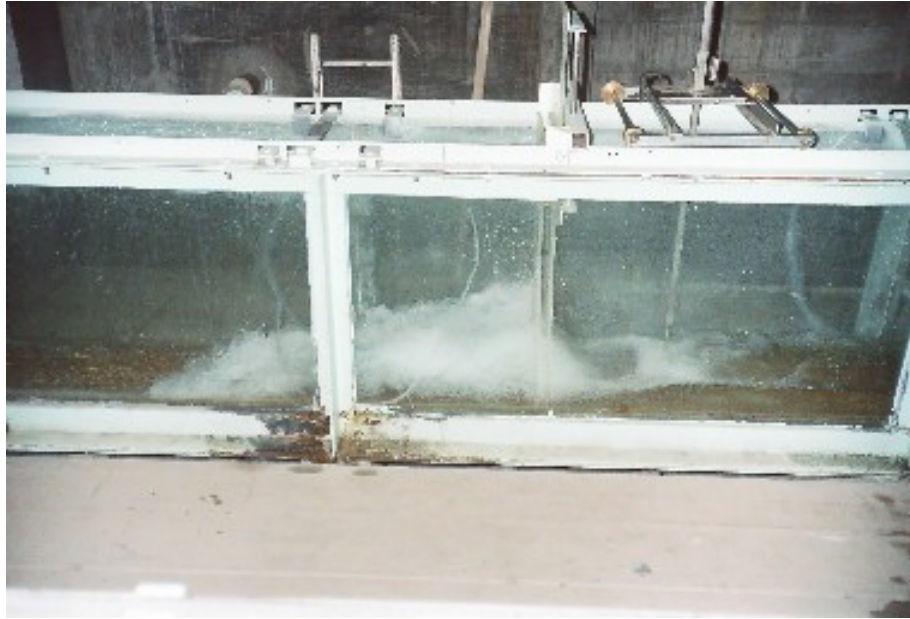
Figure 3.7 Sample view of vertical screens for Case 2
