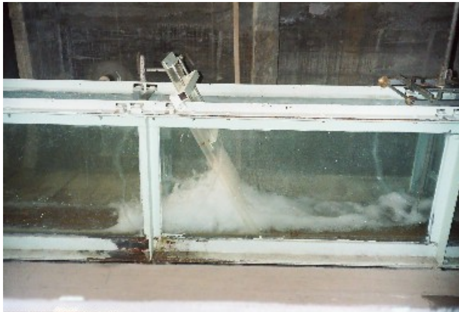
Figure 3.6 Sample view of inclined screens for Case 2
