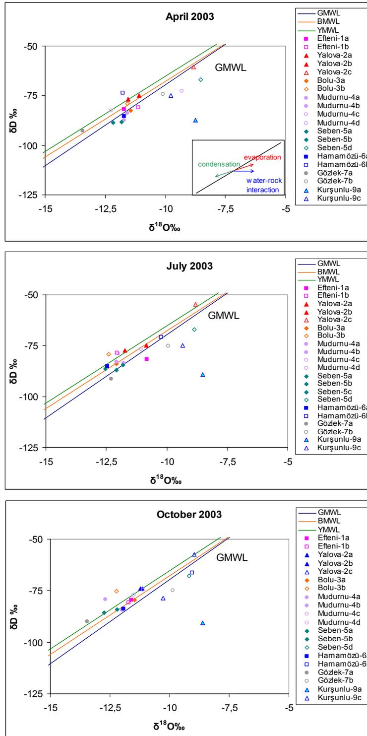
**Figure 7.1.b.**  $\delta^{18}\text{O}$ - $\delta\text{D}$  diagrams of the sampled waters for 2003 sampling periods (GMWL: Global Meteoric Water Line (Craig,1961), BMWL: Bursa Meteoric Water Line (Öztürk, 2001), YMWL: Yozgat Meteoric Water Line (Şimşek, 1995)).
