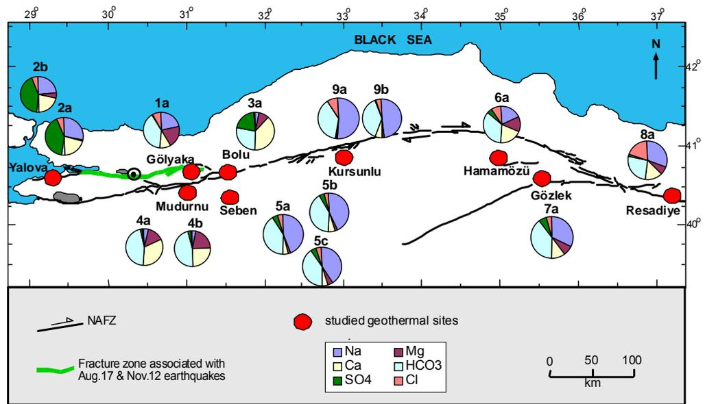
**Figure 6.3.a.** Pie diagrams of the thermal waters (relative percentages of ions are the averages of all sampling periods; TDS contents of samples are not to scale, i.e. not reflected in the diameter of the circles)
