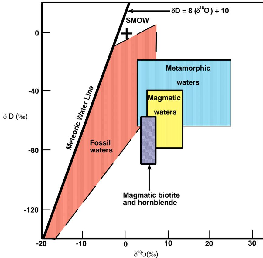
**Figure 2.1.**  $\delta D$ - $\delta^{18}O$  diagram showing isotopic compositions of different water types and the effects of physico-chemical processes on the water compositions (meteoric water line-Craig, 1961; magmatic waters-Taylor, 1974; Sheppard, 1977; metamorphic waters-Taylor, 1974; Sheppard, 1981; fossil waters-Taylor, 1974; magmatic biotite and hornblende-Taylor, 1974).
