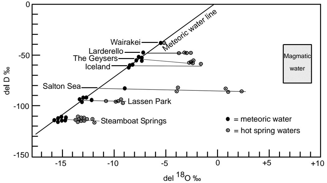
**Figure 2.2.**  $\delta^{18}\text{O}$  and  $\delta\text{D}$  values for meteoric and thermal waters in several geothermal fields (Ellis and Mahon, 1977).
