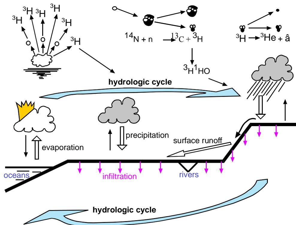
**Figure 2.3.** Origin and distribution of tritium in the hydrologic cycle.
