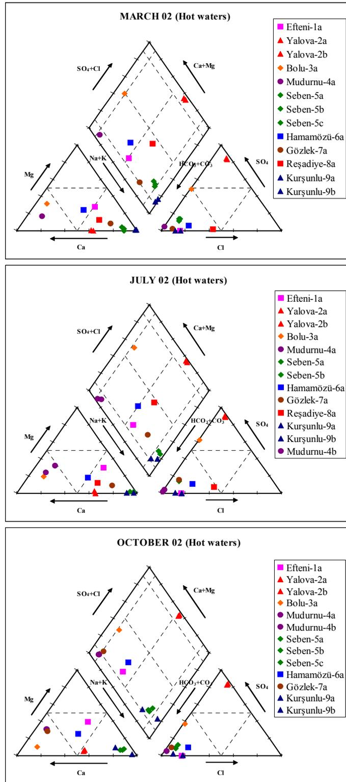
Figure 6.1.a. Piper diagrams of the hot waters for 2002 sampling periods.
