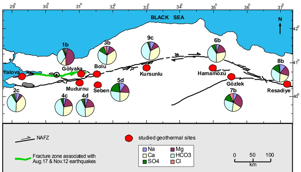
**Figure 6.3.b.** Pie diagrams of the cold waters. (relative percentages of ions are the averages of all sampling periods; TDS contents of samples are not to scale, i.e. not reflected in the diameter of the circles).
