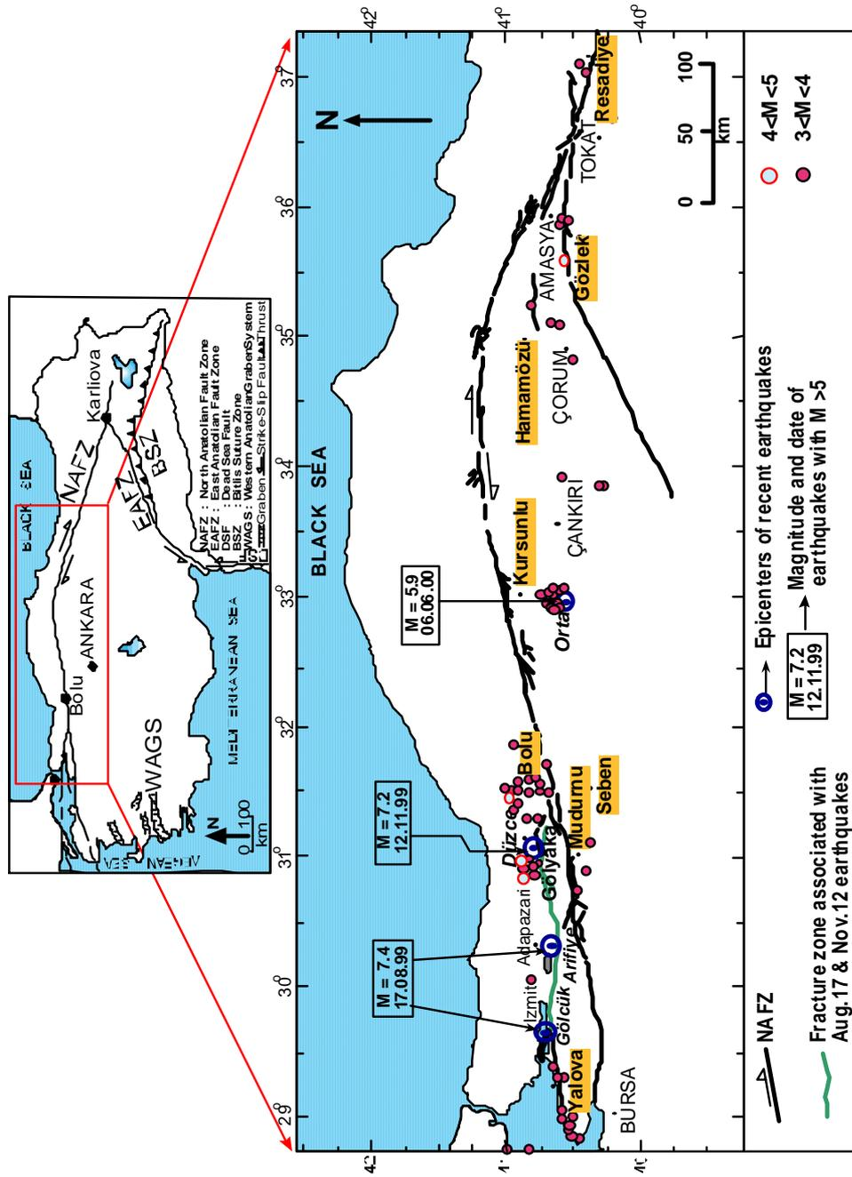
Figure 3.1. Recent seismic activities (2002-2003) along the NAFZ, close to the sampled geothermal fields.
