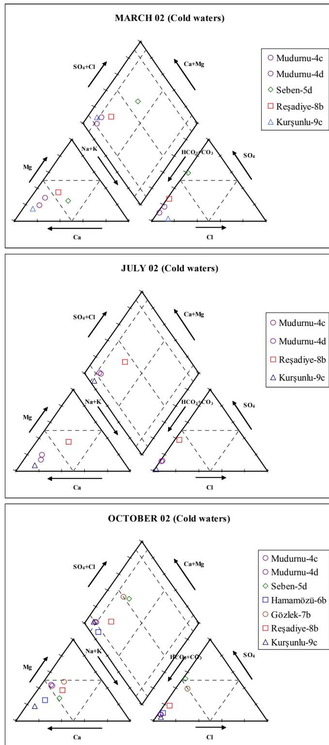
Figure 6.2.a. Piper diagrams of the cold waters for 2002 sampling periods.
