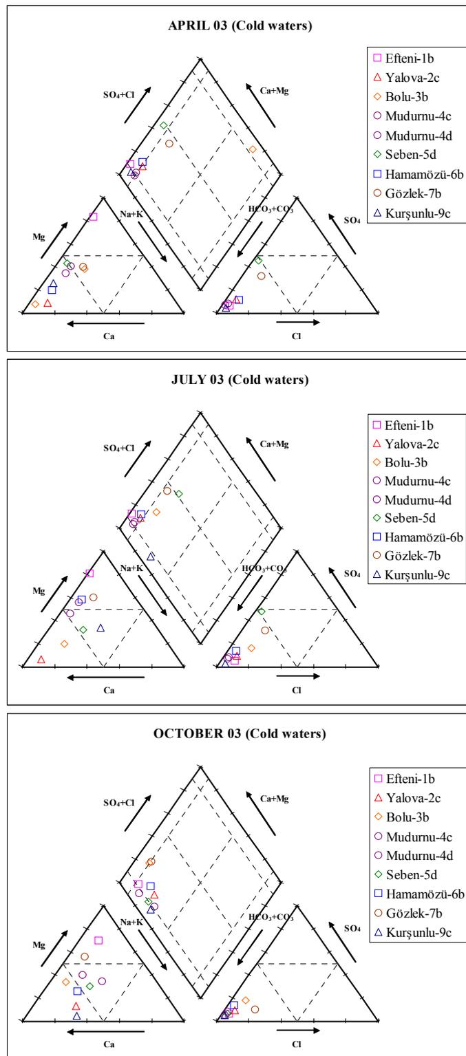
Figure 6.2.b. Piper diagrams of the cold waters for 2003 sampling periods.
