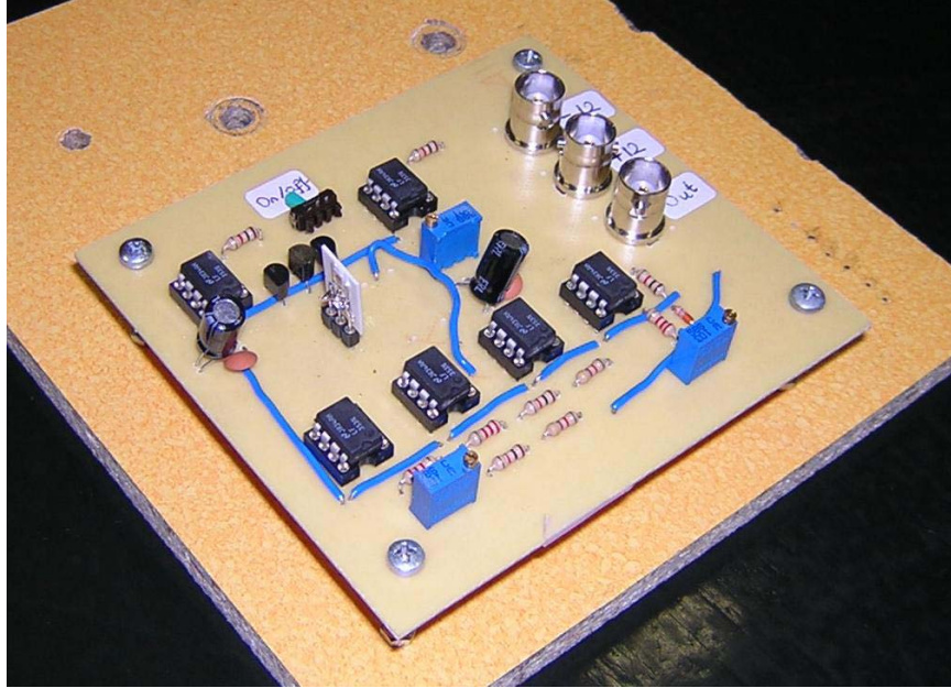
Figure 5.31: The second generation hybrid accelerometer system. This system uses a nickel accelerometer, and has bias circuitries and amplifier stages additional to first generation hybrid system.
