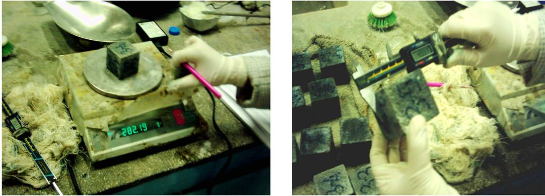
**Figure 15 Weight and Dimensional Measurements of Cubic Specimens**
