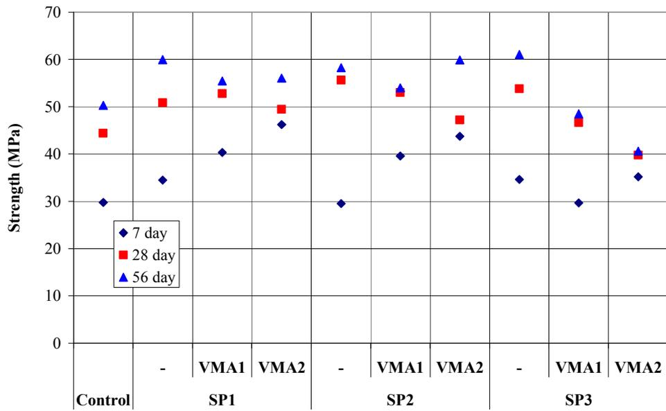
**Figure 19 Effect of Chemical Admixtures on the Strength of SCMs**
