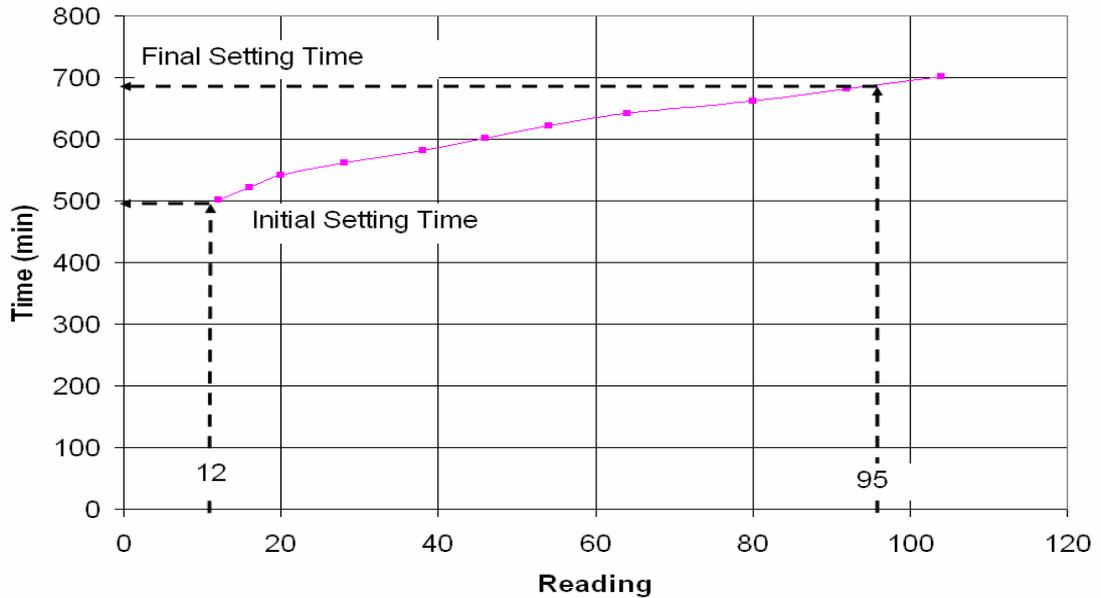
**Figure 11 Determination of Initial and Final Setting Time by Interpolation**
