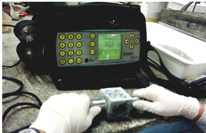
**Figure 16 UPV Testing on Cubic Specimens**
