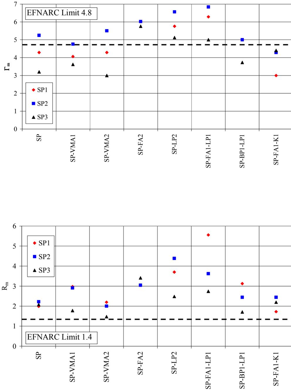
**Figure 25 Effects of Ternary Mixes on the Workability of SCMs**
