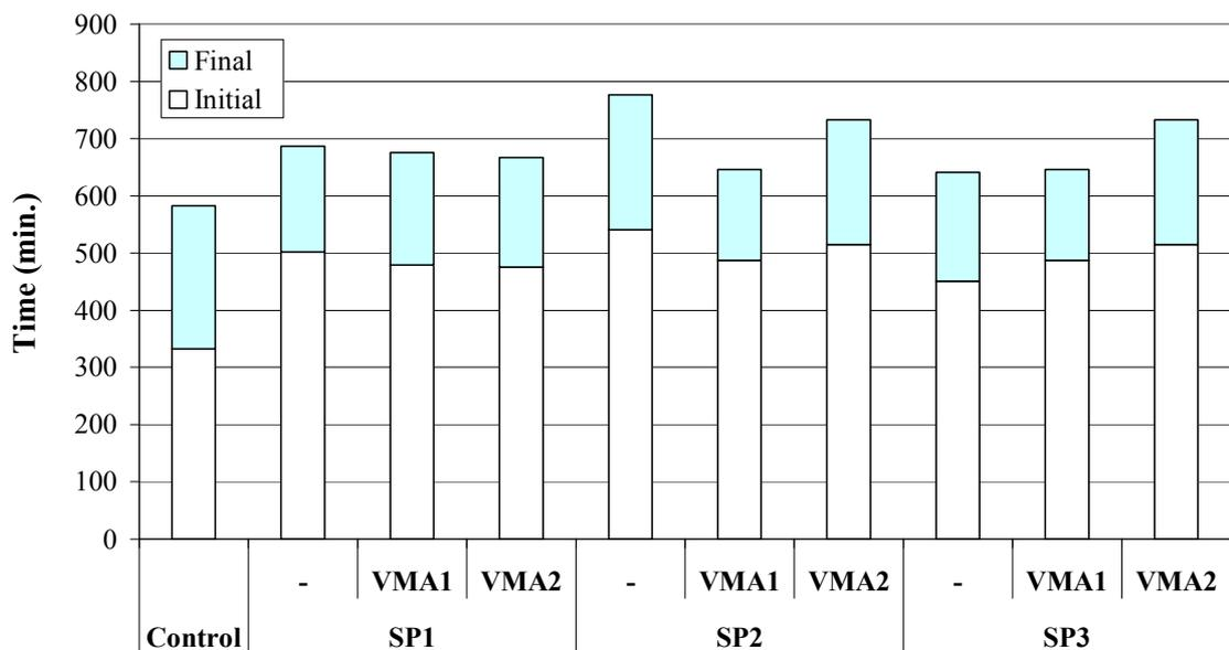
**Figure 18 Effect of Chemical Admixture on Setting Time of SCMs**
