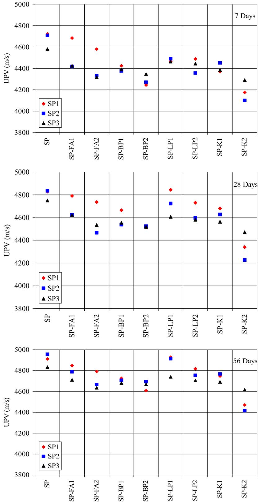
**Figure 24 Effect of Mineral Admixtures on UPV of SCMs**
