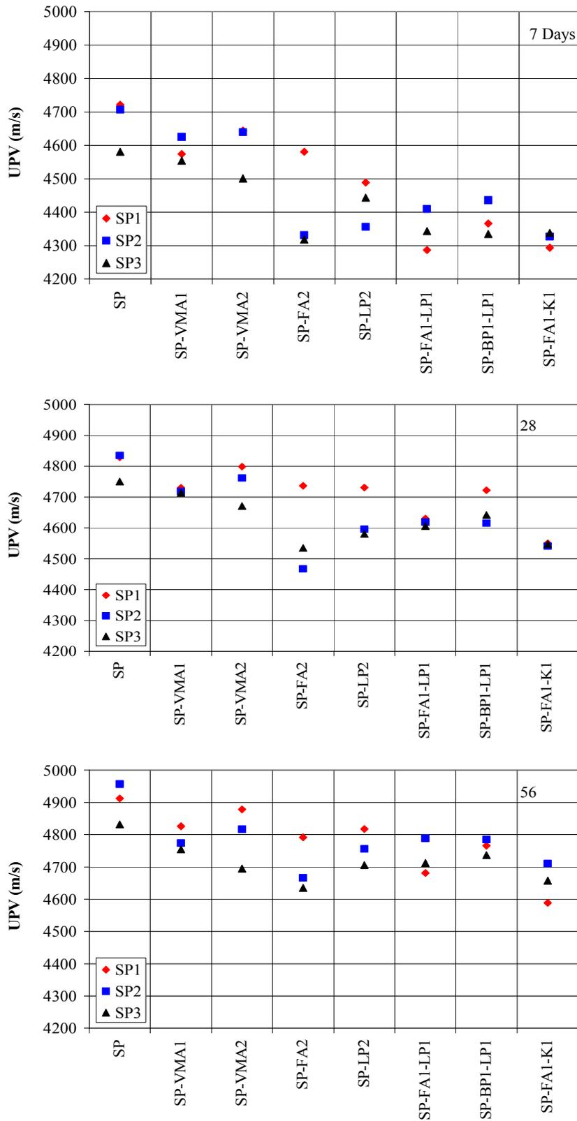
**Figure 28 Effects of Ternary Mixes on the UPV of SCMs**
