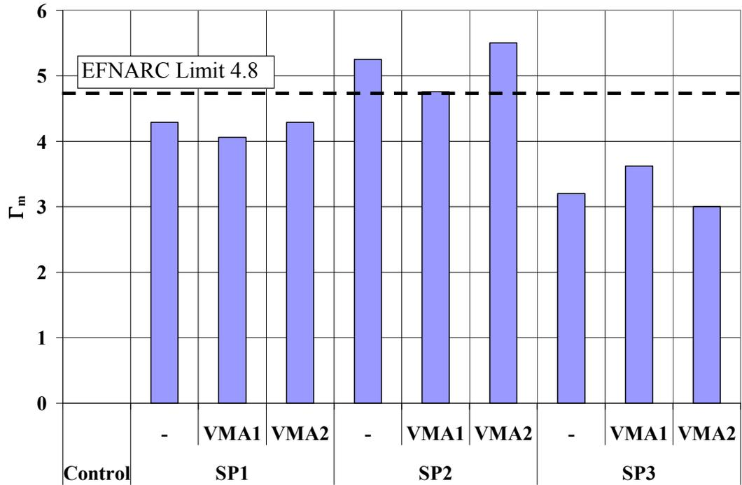
(a) Slump Flow Test
