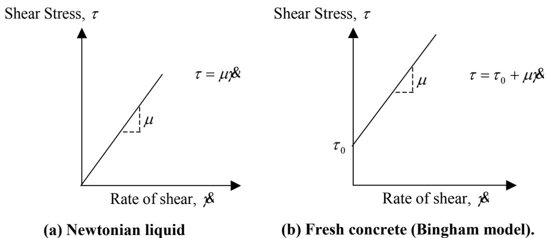
**Figure 1 Flow Properties of Materials**
