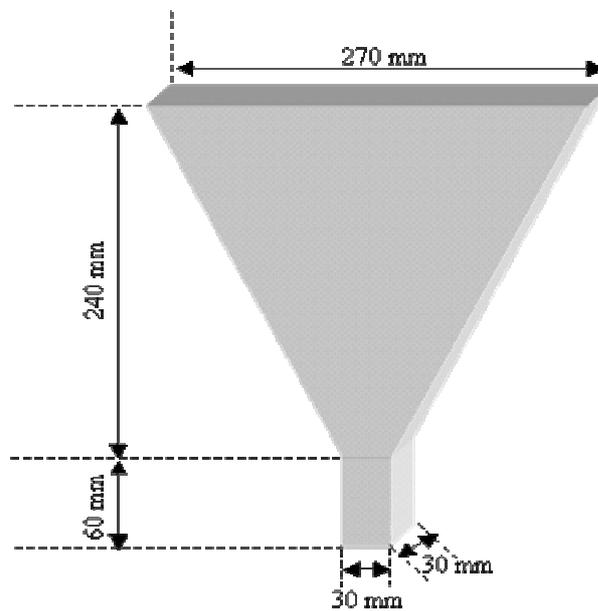
**Figure 13 V-Funnel to Determine the Flow Time of Mortar**
