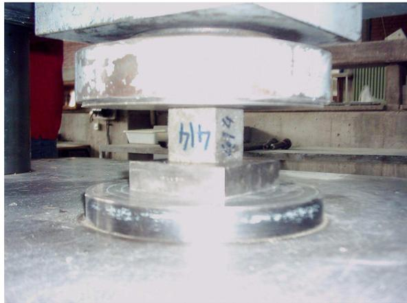
**Figure 14 Determination of Compressive Strength**
