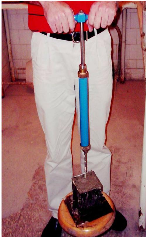
**Figure 10 Apparatus for Testing Setting Time**
