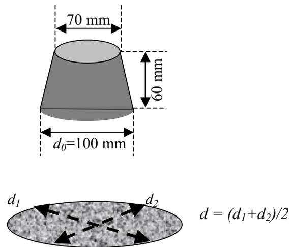
**Figure 12 Flow Cone and Determination of the Slump Flow**
