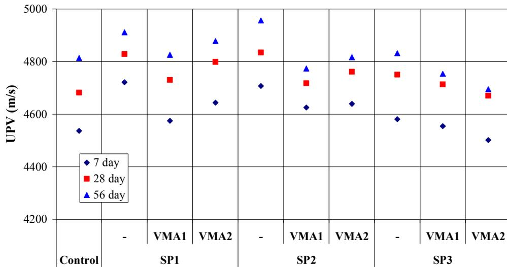
**Figure 20 Effect of Chemical Admixture on UPV of SCMs**
