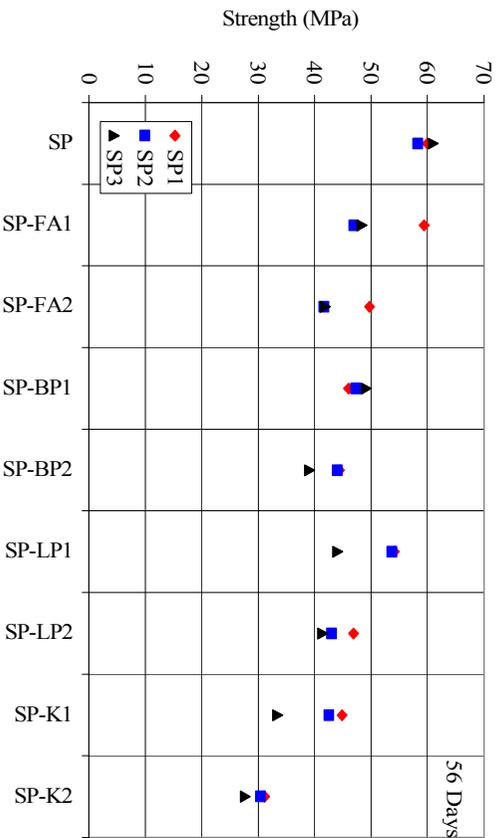
Figure 23 Effect of Mineral Admixtures on Strength of SCM
