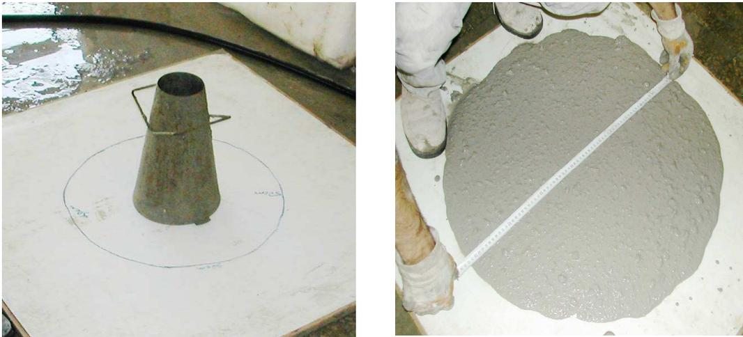
**Figure 2 Slump Flow Test**
