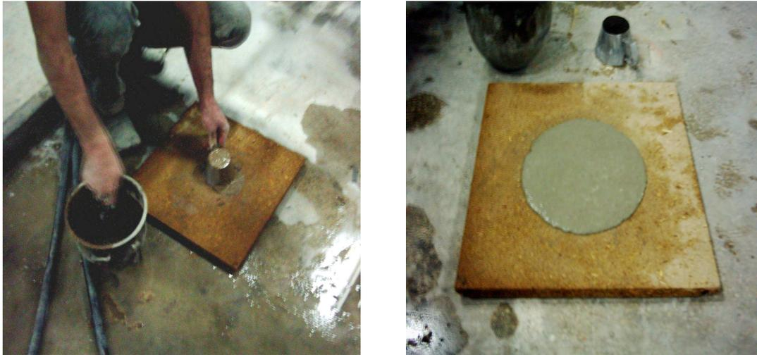
**Figure 3 Mini Slump Cone**
