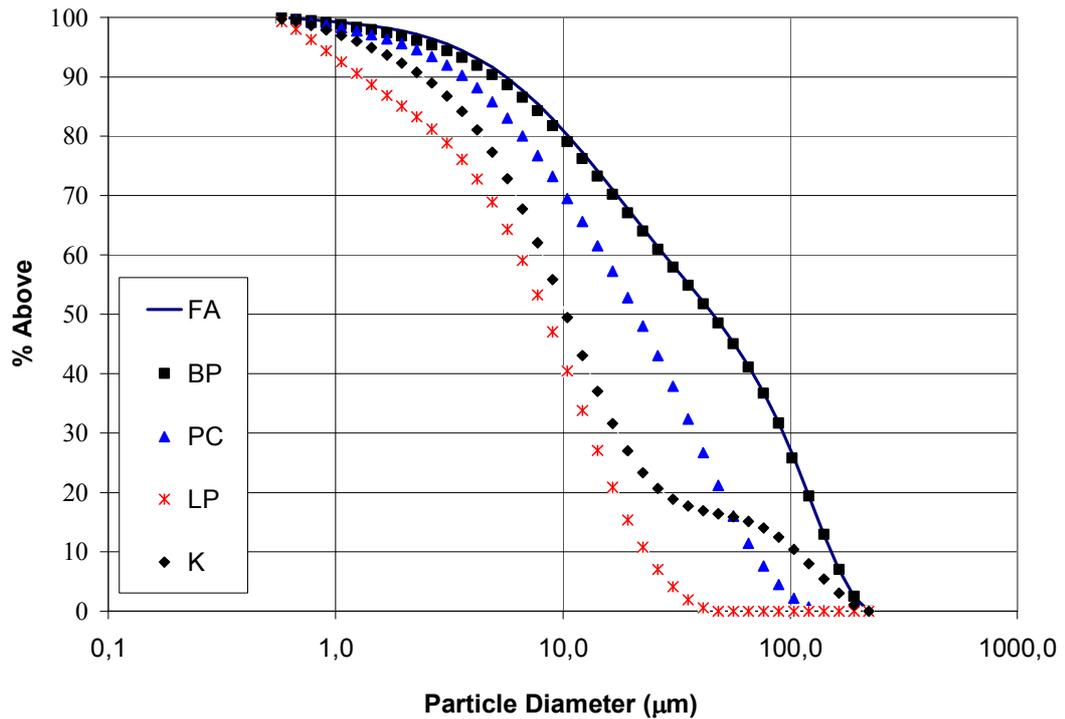
**Figure 6 Particle Size Distributions of Cement and Mineral Admixtures**
