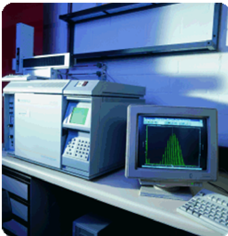
Figure 3.3 Gas chromatograph coupled to a mass spectrometer [23]
