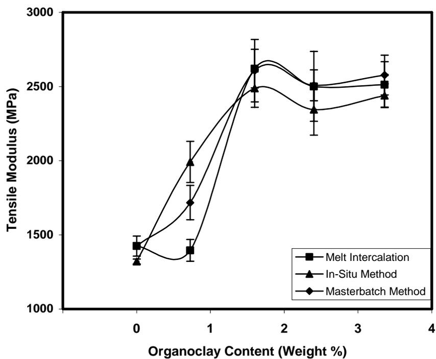
**Figure 4.22** Effect of organoclay content on the tensile modulus of the nanocomposites prepared by the three methods.
