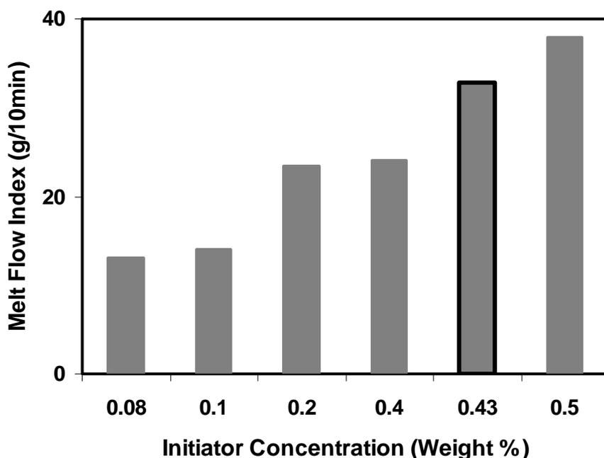
**Figure 4.15** Effect of initiator concentration on the melt flow index of polystyrene
