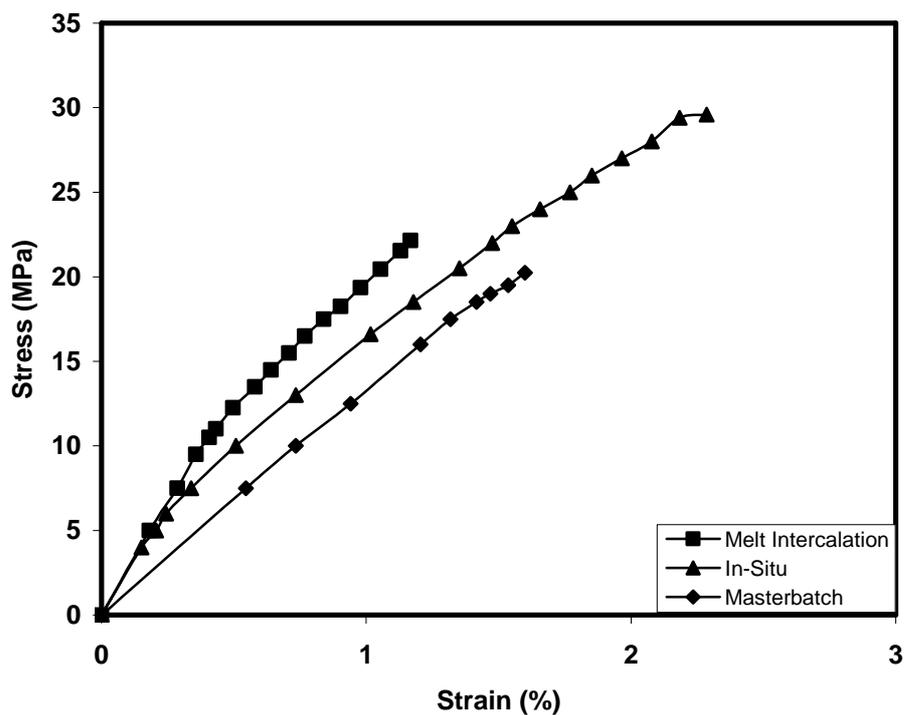
**Figure 4.18** Tensile stress-strain (%) curves of the nanocomposites prepared by the three methods containing 1.6 wt. % organoclay.
