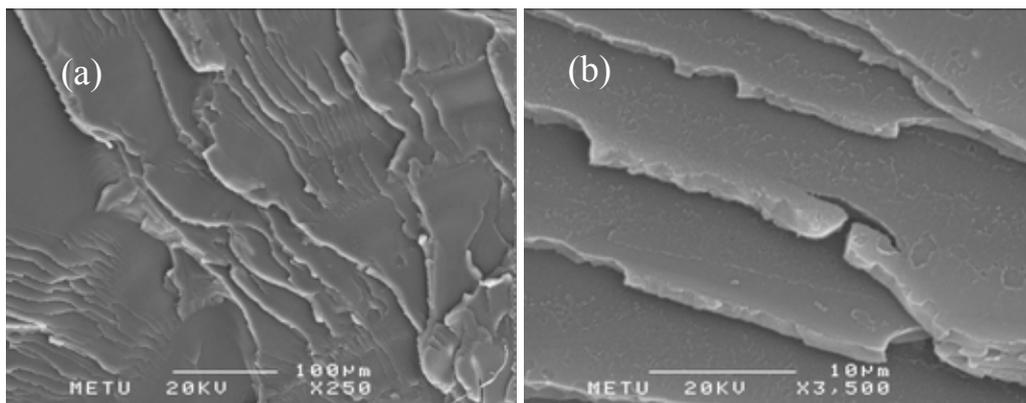
**Figure 4.1** SEM micrographs of the commercial polystyrene at (a) 250 (b) 3500 magnifications.
