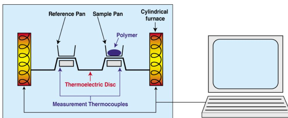
**Figure 2.8** Differential Scanning Calorimeter cell [36].
