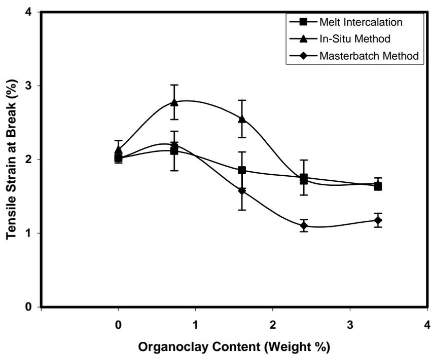
**Figure 4.23** Effect of organoclay content on the tensile strain at break (%) of the nanocomposites prepared by the three methods.
