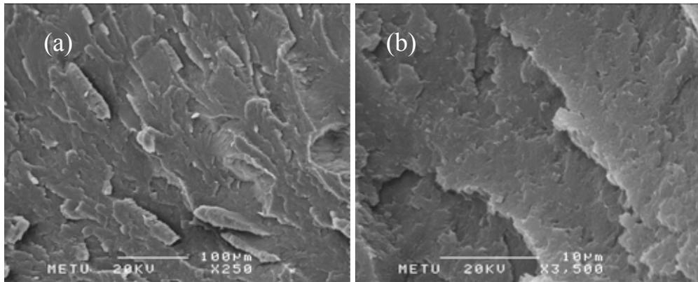
**Figure 4.14** SEM micrographs of the nanocomposite prepared by masterbatch method containing 3.36 wt. % MMT at (a) 250 (b) 3500 magnifications.
