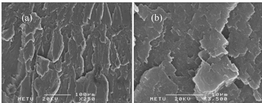
**Figure 4.12** SEM micrographs of the nanocomposite prepared by masterbatch method containing 1.6 wt. % MMT at (a) 250 (b) 3500 magnifications.
