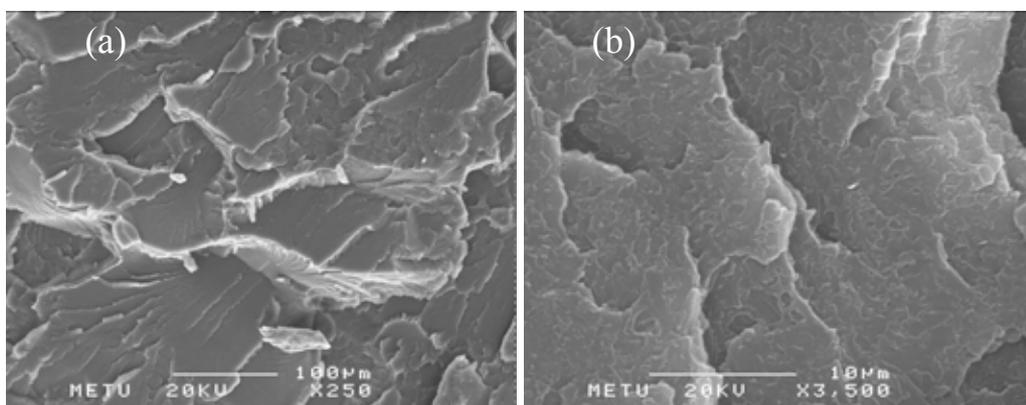
**Figure 4.11** SEM micrographs of the nanocomposite prepared by masterbatch method containing 0.73 wt. % MMT at (a) 250 (b) 3500 magnifications.
