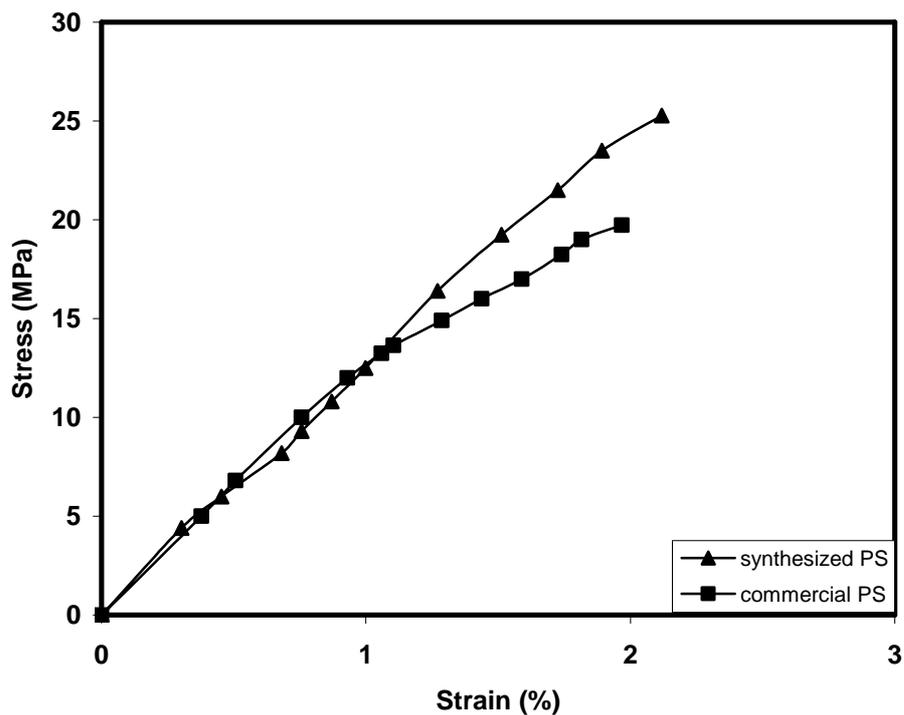
**Figure 4.16** Tensile stress-strain (%) curves of the commercial polystyrene and synthesized polystyrene.
