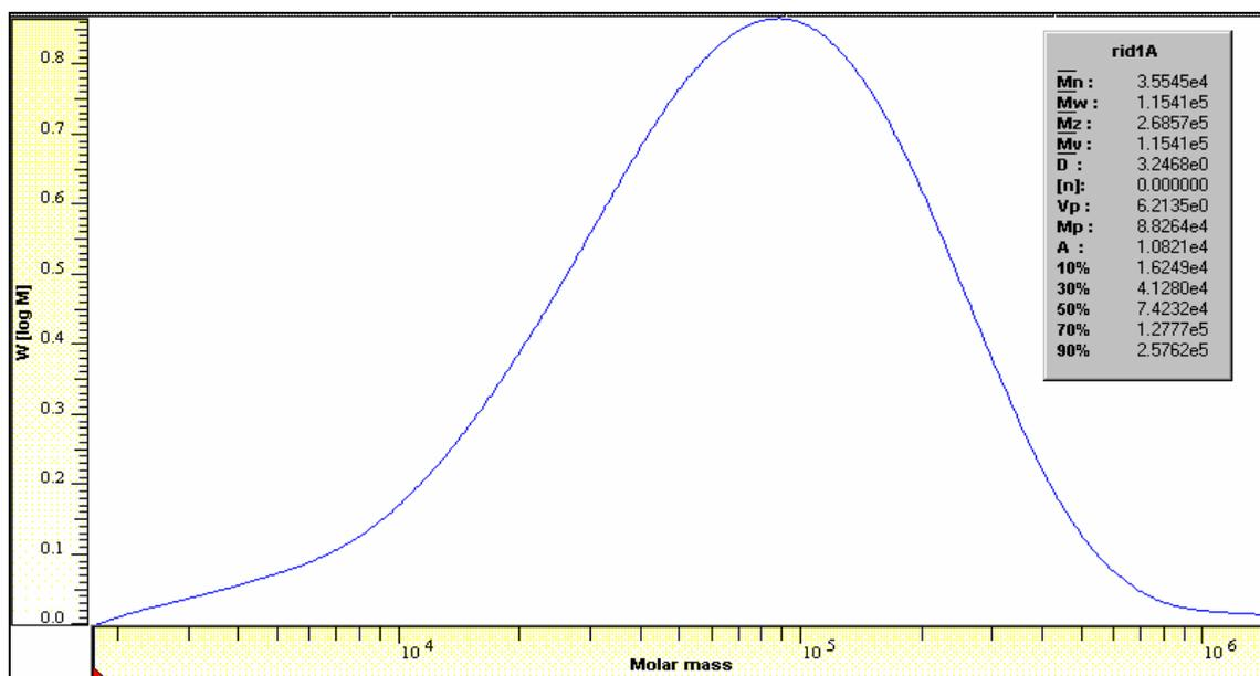
D.1.1 Molecular weight distribution curve of commercial polystyrene
