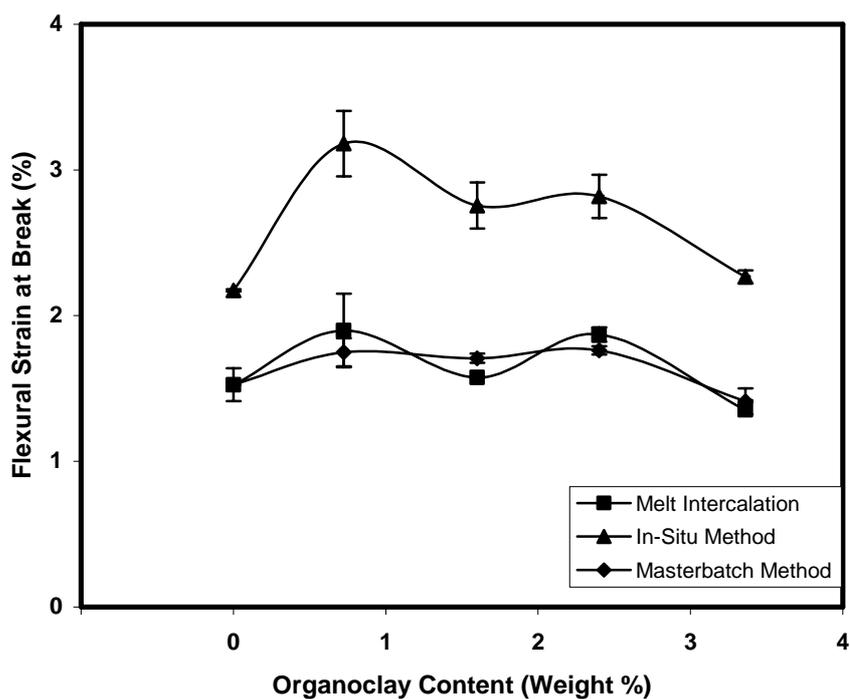
**Figure 4.26** Effect of organoclay content on the flexural strain at break (%) of the nanocomposites prepared by the three methods.
