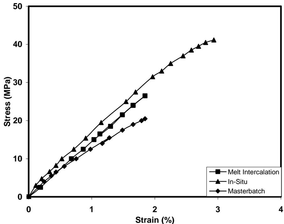
**Figure 4.17** Tensile stress-strain (%) curves of the nanocomposites prepared by the three methods containing 0.73 wt. % organoclay.
