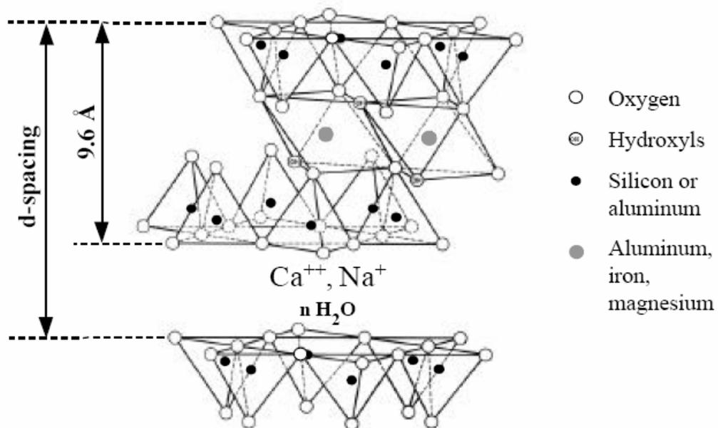
**Figure 2.1** Idealized structure of 2:1 layered silicate showing two tetrahedral-site sheets fused to an octahedral-site sheet [16].
