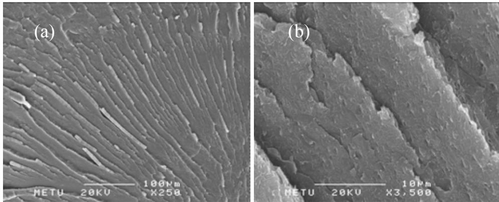
**Figure 4.13** SEM micrographs of the nanocomposite prepared by masterbatch method containing 2.4 wt. % MMT at (a) 250 (b) 3500 magnifications.
