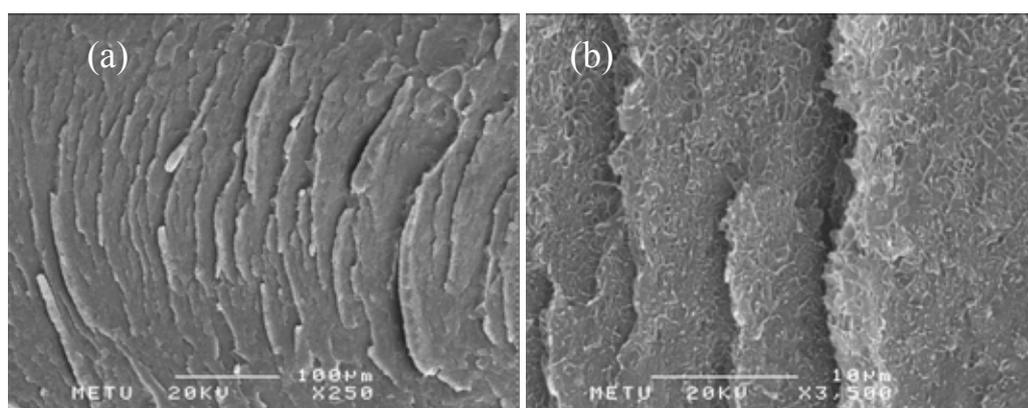
**Figure 4.6** SEM micrographs of the nanocomposite prepared by in-situ polymerization method containing 3.36 wt. % MMT at (a) 250 (b) 3500 magnifications.
