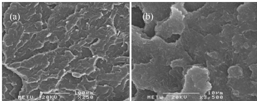
**Figure 4.4** SEM micrographs of the nanocomposite prepared by in-situ polymerization method containing 1.6 wt. % MMT at (a) 250 (b) 3500 magnifications.
