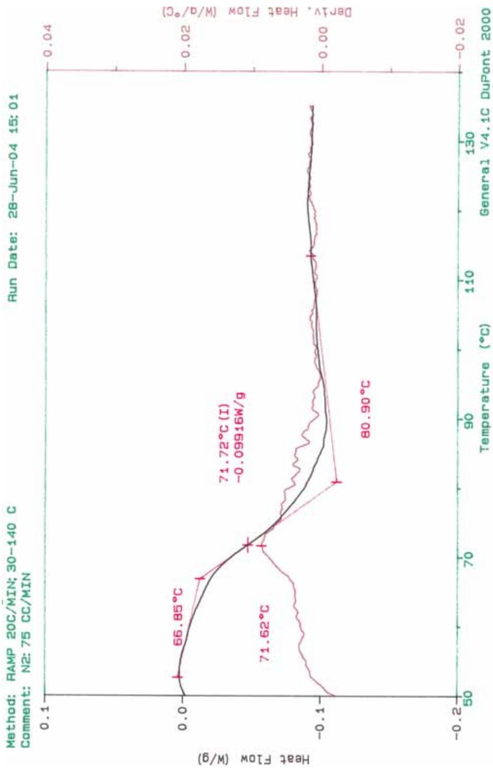
**Figure B.1.10** DSC Diagram of nanocomposite prepared by in-situ polymerization containing 2.4 wt. % MMT
