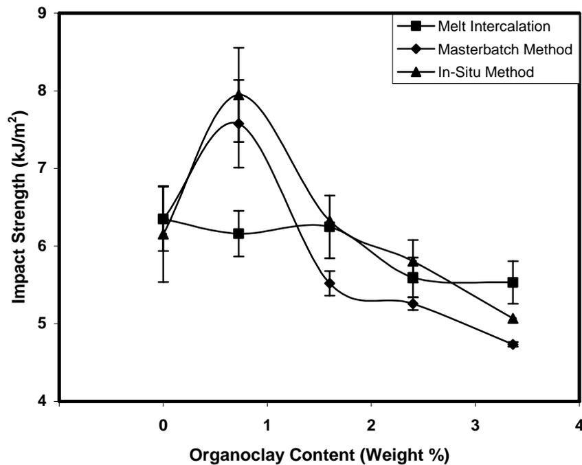
**Figure 4.27** Effect of organoclay content on the impact strength of the nanocomposites prepared by the three methods.
