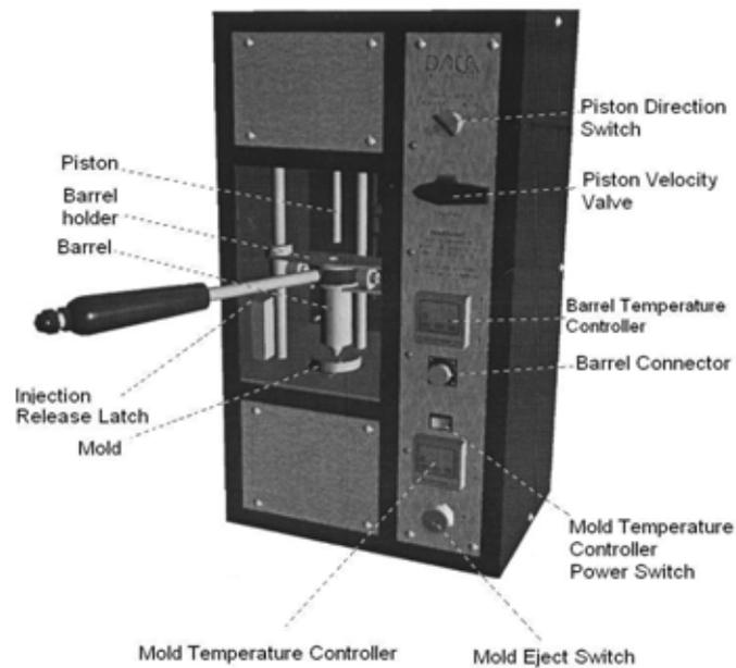
**Figure 3.5** Schematic representation of injection molding machine
