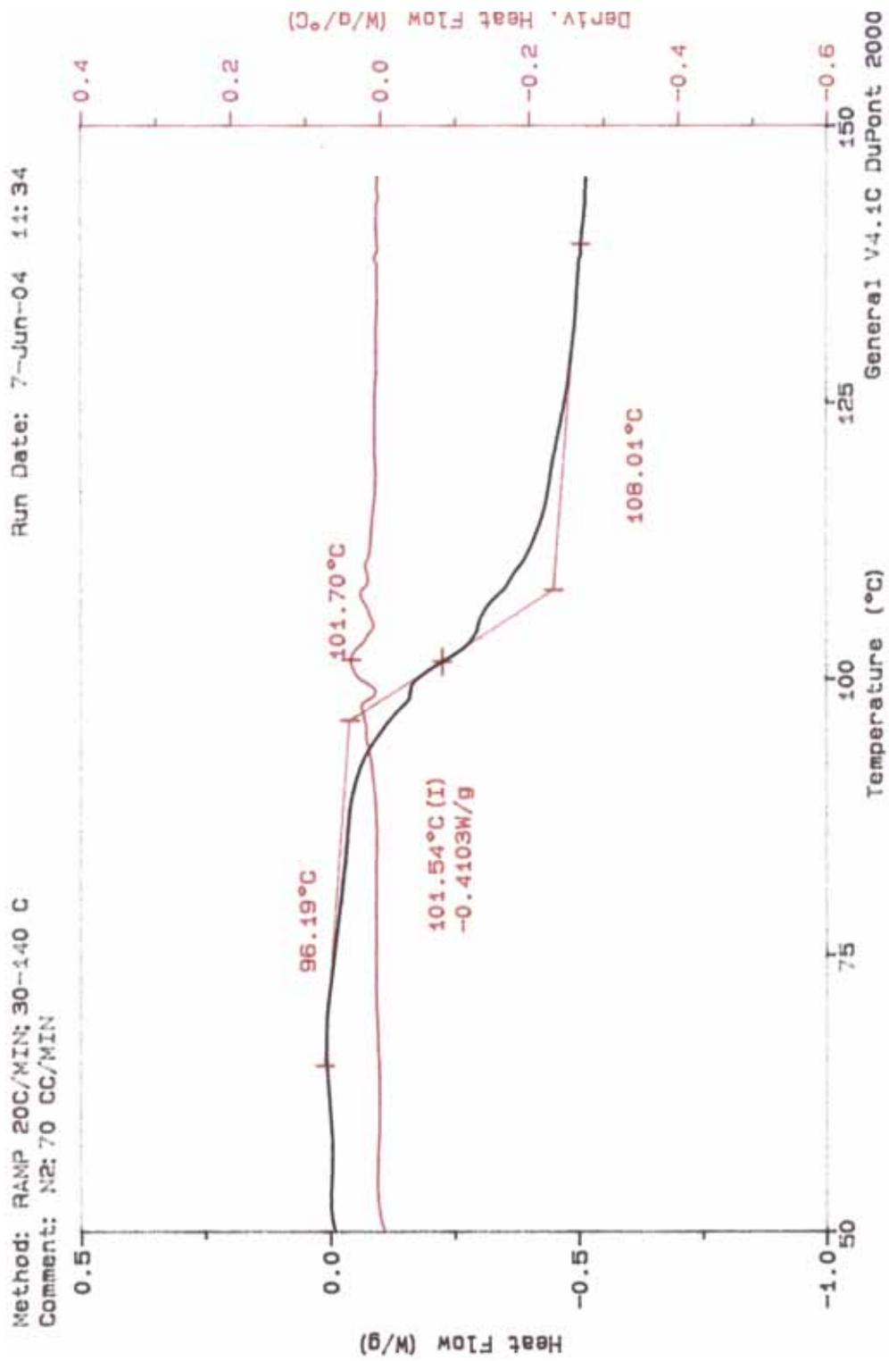
**Figure B.1.12** DSC Diagram of nanocomposite prepared by masterbatch containing 0.73 wt. % MMT
