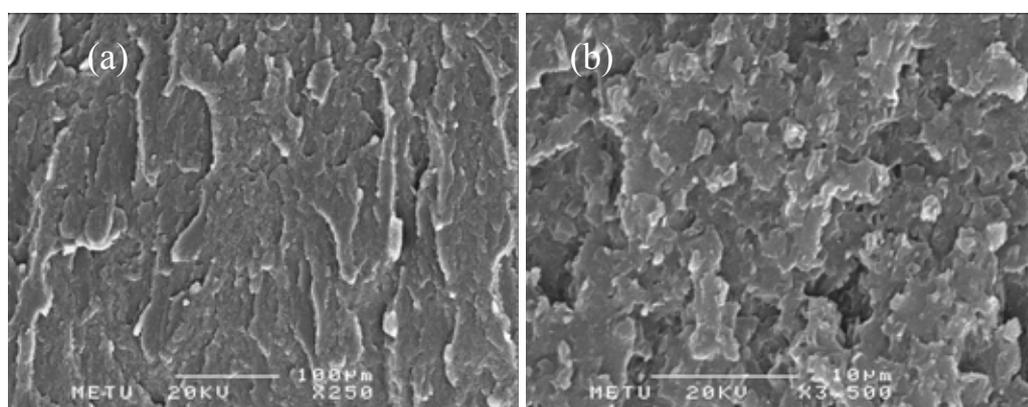
**Figure 4.5** SEM micrographs of the nanocomposite prepared by in-situ polymerization method containing 2.4 wt. % MMT at (a) 250 (b) 3500 magnifications.
