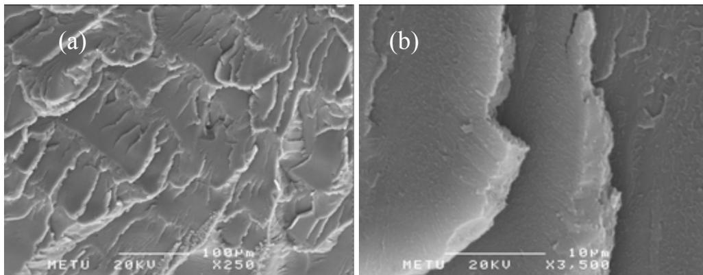
**Figure 4.7** SEM micrographs of the nanocomposite prepared by melt intercalation method containing 0.73 wt. % MMT at (a) 250 (b) 3500 magnifications.
