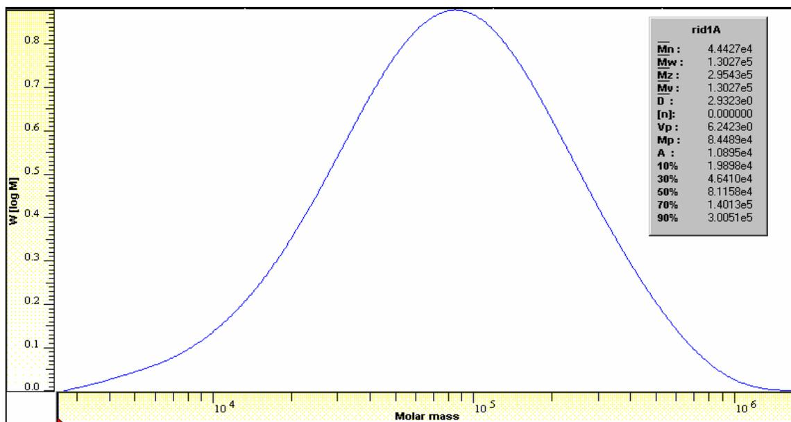
D.1.2 Molecular weight distribution curve of synthesized polystyrene
