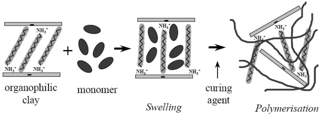
**Figure 2.3** Schematic representation of the *in situ* polymerization method [16].
