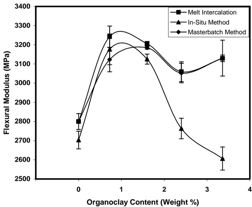
**Figure 4.25** Effect of organoclay content on the flexural modulus of the nanocomposites prepared by the three methods.
