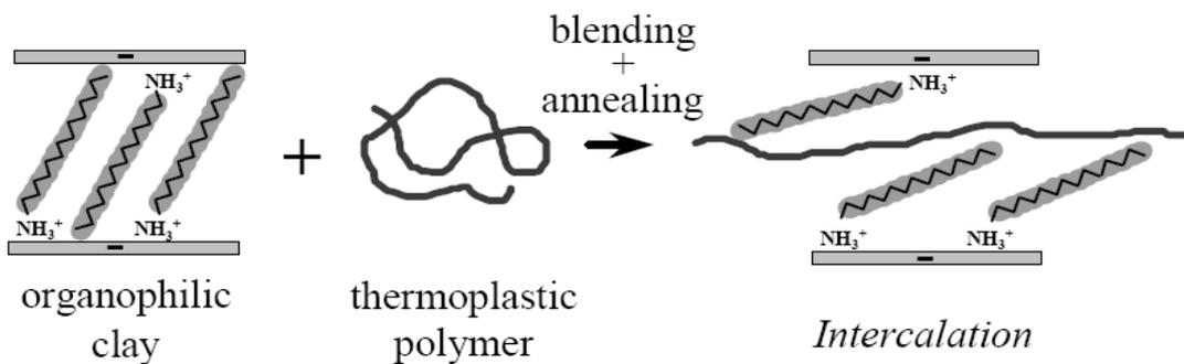
**Figure 2.4** Schematic representation of the melt intercalation method [16].
