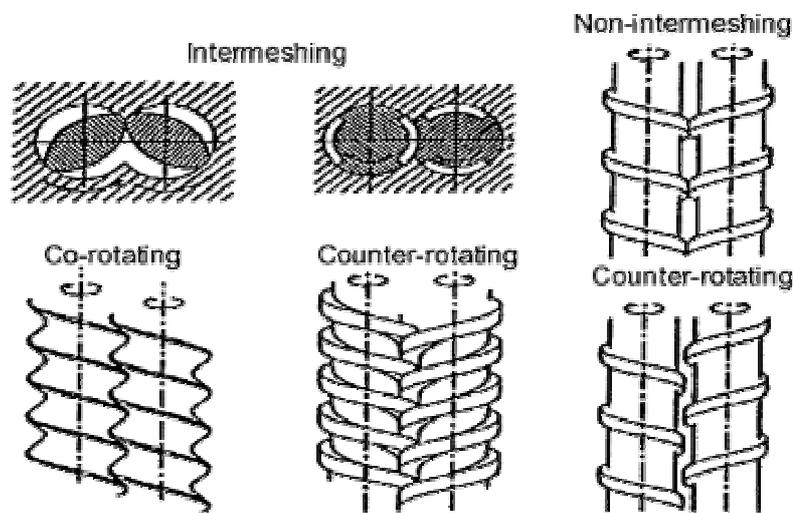
**Figure 2.7** Different twin screw designs [31].
