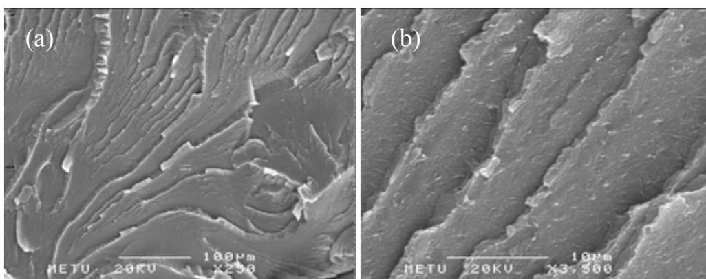
**Figure 4.9** SEM micrographs of the nanocomposite prepared by melt intercalation method containing 2.4 wt. % MMT at (a) 250 (b) 3500 magnifications.
