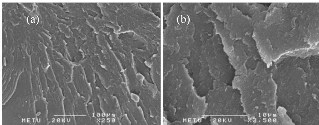
**Figure 4.10** SEM micrographs of the nanocomposite prepared by melt intercalation method containing 3.36 wt. % MMT at (a) 250 (b) 3500 magnifications.
