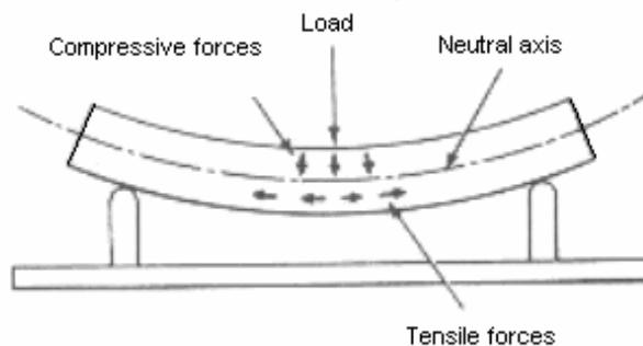
**Figure 2.10** The stresses on the sample during flexural testing [39].
