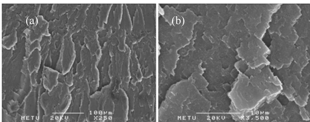
**Figure 4.8** SEM micrographs of the nanocomposite prepared by melt intercalation method containing 1.6 wt. % MMT at (a) 250 (b) 3500 magnifications.
