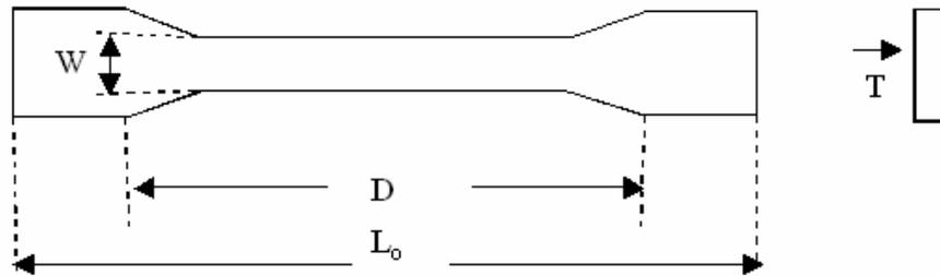
**Figure 2.9** Tensile test specimen [37].
