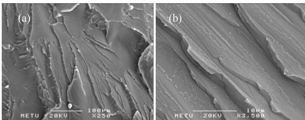
**Figure 4.2** SEM micrographs of the synthesized polystyrene at (a) 250 (b) 3500 magnifications.
