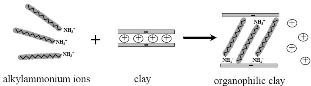
**Figure 2.2** Schematic representation of the cation exchange process [16].
