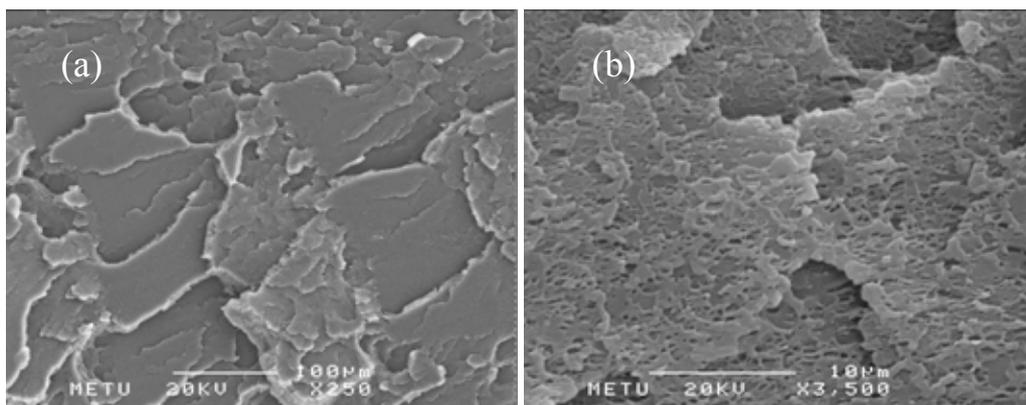
**Figure 4.3** SEM micrographs of the nanocomposite prepared by in-situ polymerization method containing 0.73 wt. % MMT at (a) 250 (b) 3500 magnifications.
