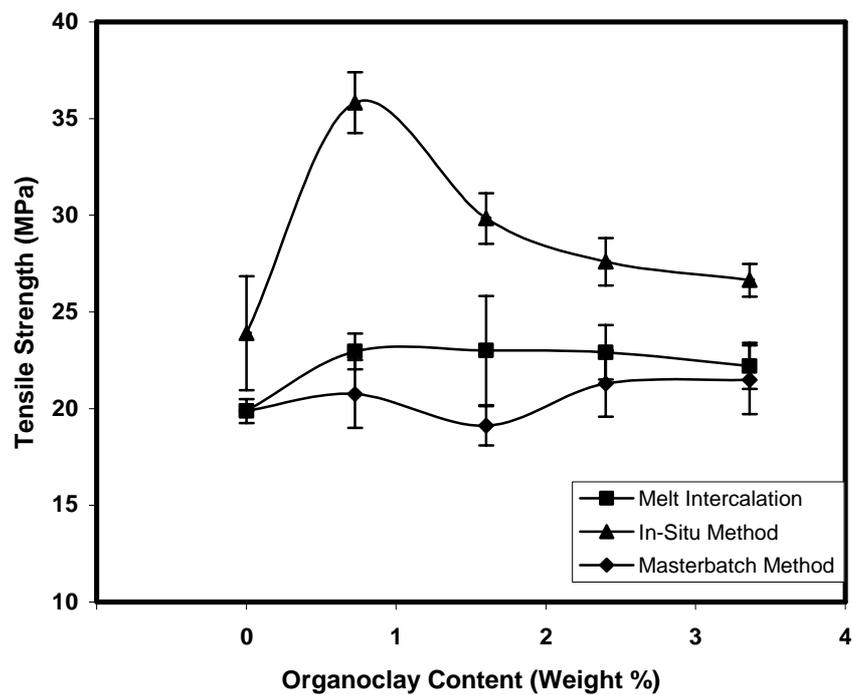
**Figure 4.21** Effect of organoclay content on the tensile strength of the nanocomposites prepared by the three methods.
