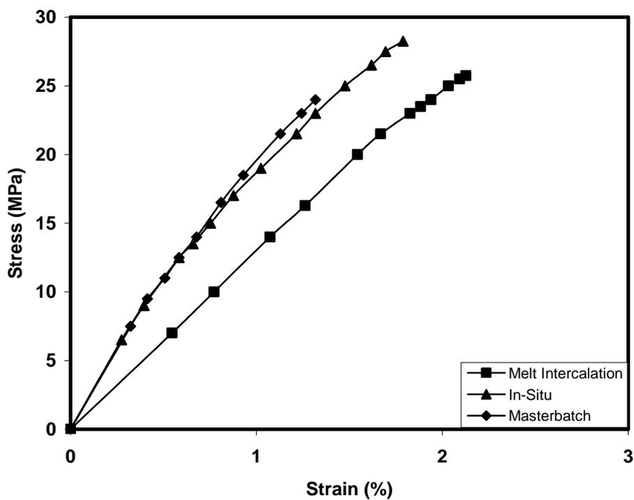
**Figure 4.19** Tensile stress-strain (%) curves of the nanocomposites prepared by the three methods containing 2.4 wt. % organoclay.
