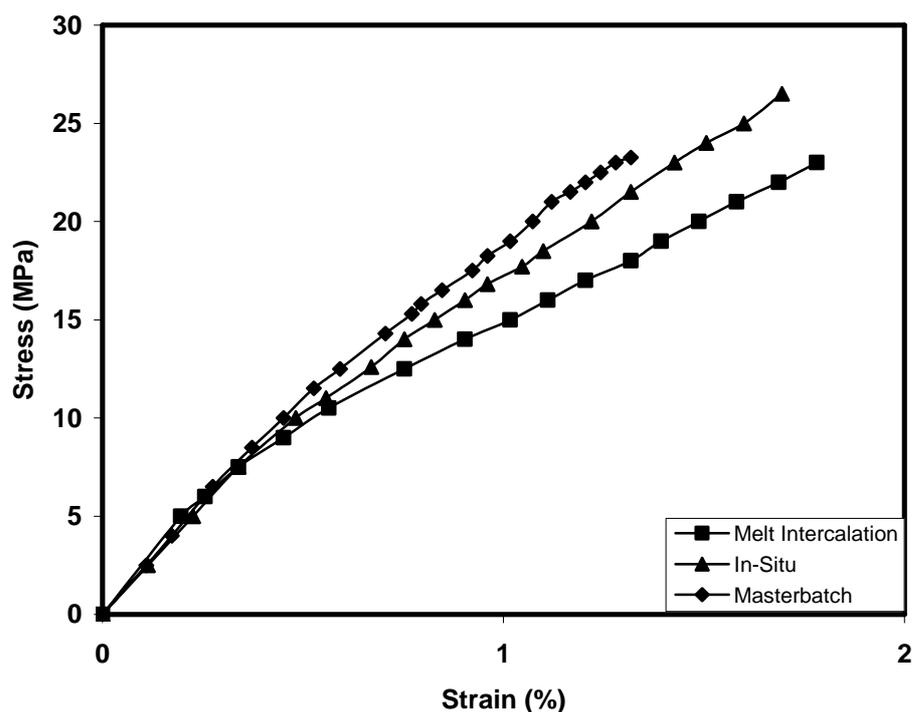
**Figure 4.20** Tensile stress-strain (%) curves of the nanocomposites prepared by the three methods containing 3.36 wt. % organoclay.
