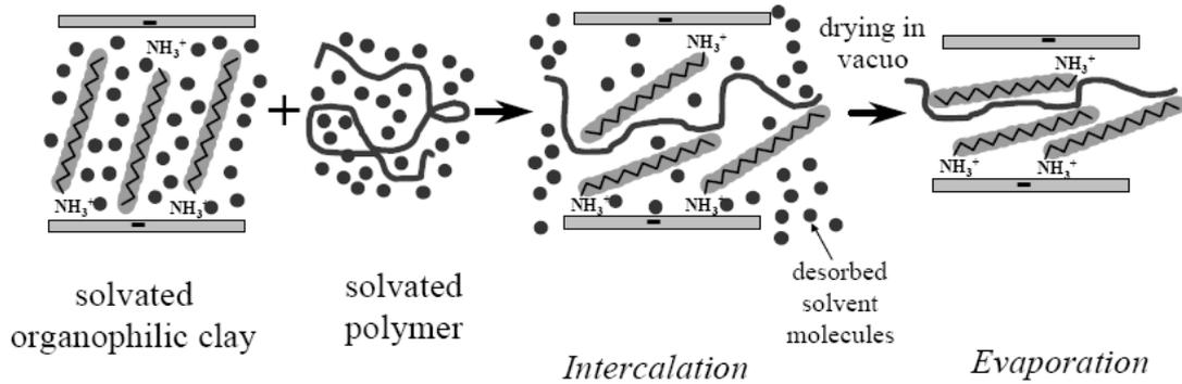
**Figure 2.5** Schematic representation of the solution method [16].
