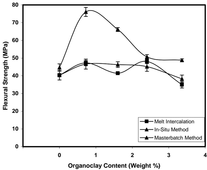
**Figure 4.24** Effect of organoclay content on the flexural strength of the nanocomposites prepared by the three methods.
