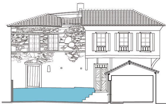
Figure 4.10 Material and construction system, timber frame walls type 3 and concrete walls
