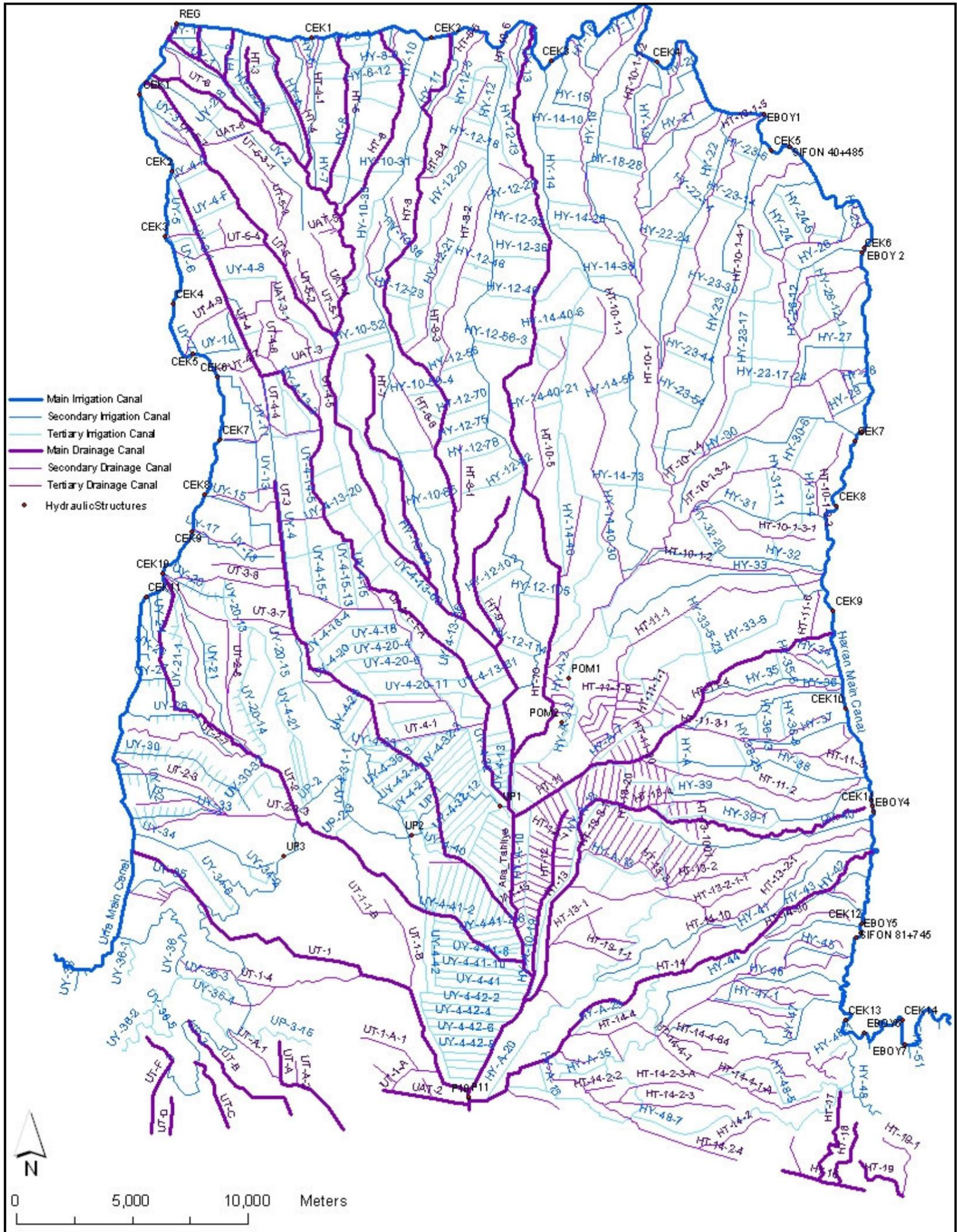
Figure 3.23: Irrigation and Drainage System
