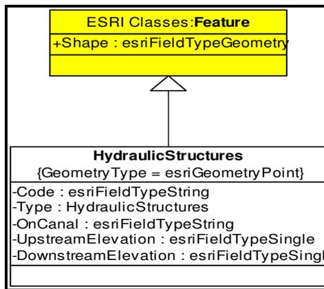
**Figure 3.16:** Hydraulic Structures Diagram
