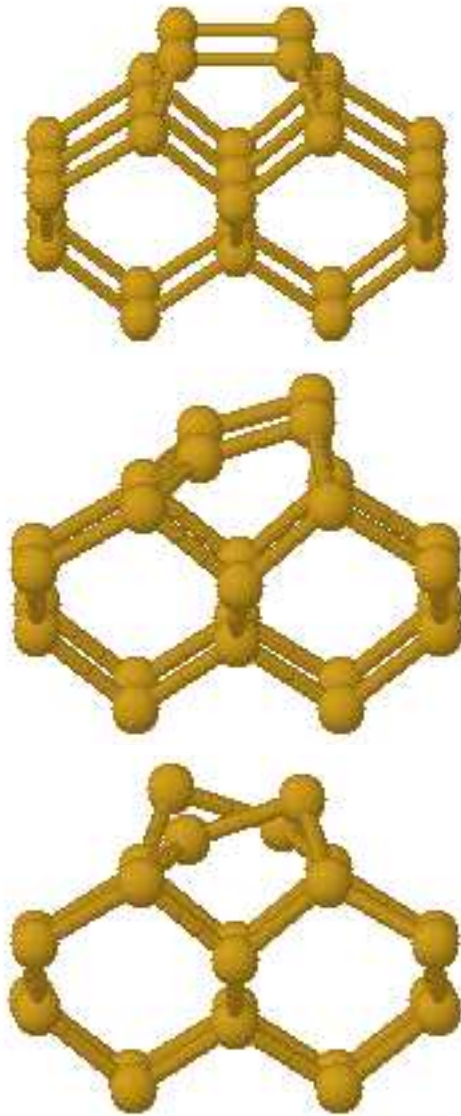
Figure I.1: Different Si(001) reconstructions, top one is symmetric ( 2 \times 1 ), middle one is asymmetric ( 2 \times 1 ), below one is p(2 \times 2) reconstruction.
