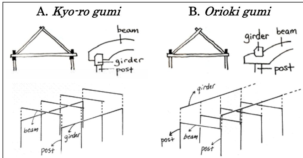
Figure 4-29 Beam construction of the Japanese house
