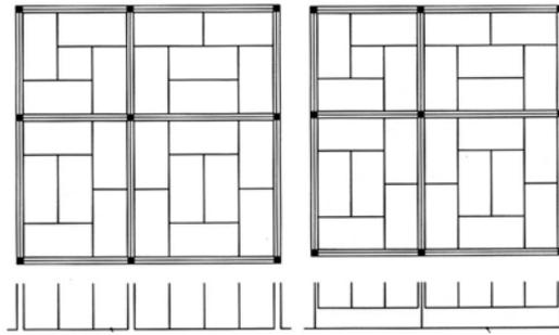
Figure 4-31 *Kyo-ma* (left) and *edo-ma* (right)
