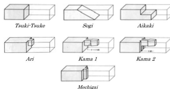
Figure 4-25 Typical extension joints for joists, sleepers, girders and beams (Source: Hamashima, 1984: 36)
