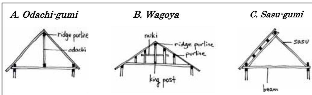
Figure 4-38 Three types of typical roof structure of the Japanese house
