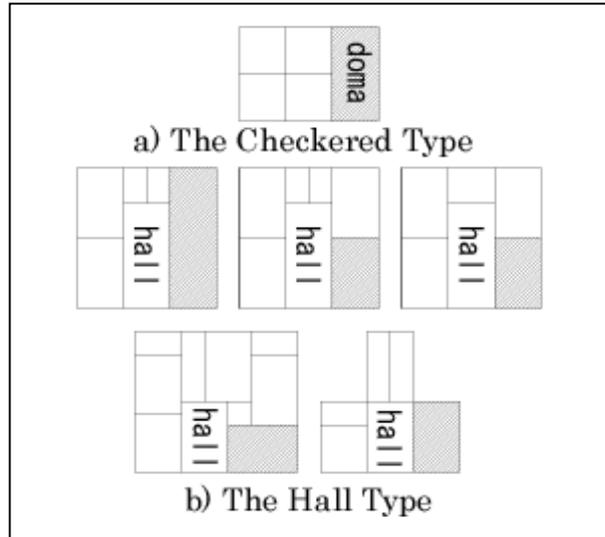
Figure 2-10 The typical floor plan of the Japanese house
