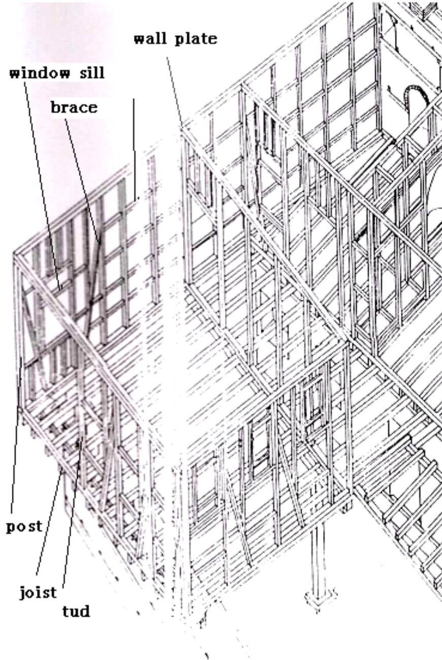
Figure 4-9 Timber Structure and Components of the Turkish House
