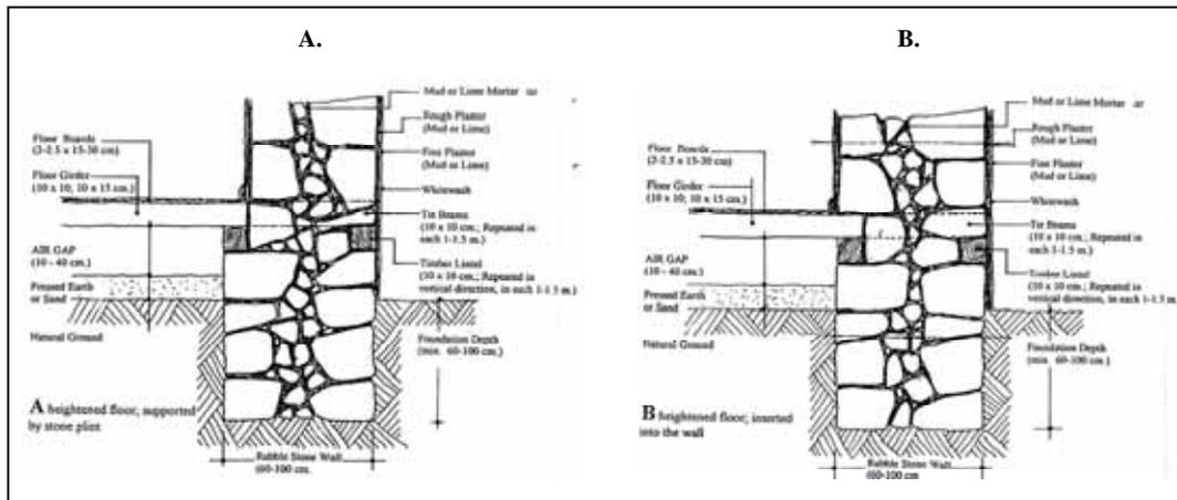
Figure 4-13 Two types of timber boarded ground floor of the Turkish house (Source: Şahin, 1996: 191)
