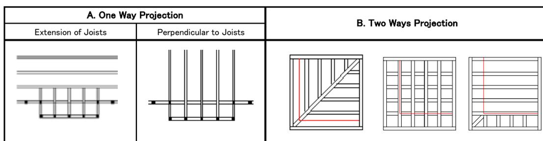
Figure. 4-18 Floor joists arrangement of the projection.
