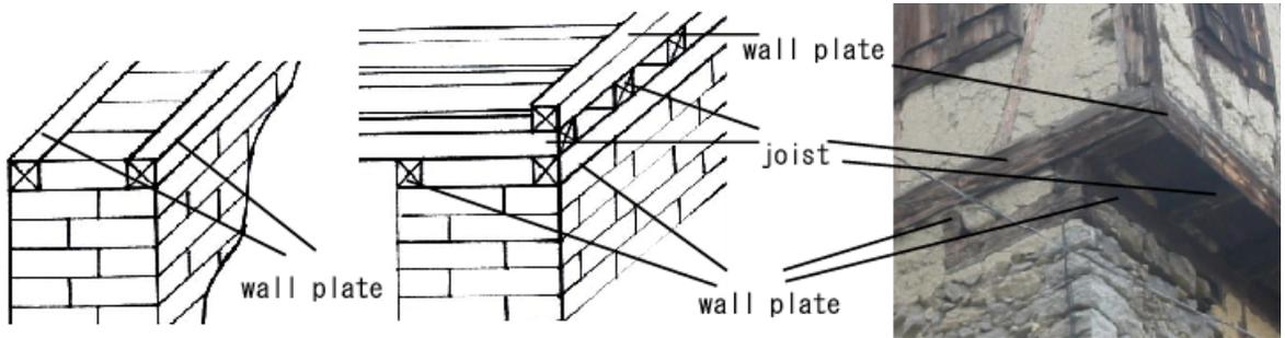
Figure. 4-11 Construction of the floor framing
