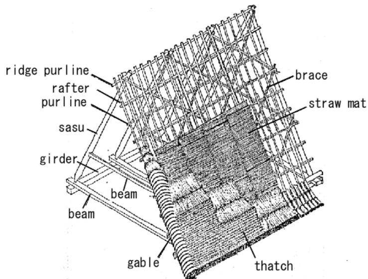
Figure 4-39 The structure of the gassyo-zukuri
