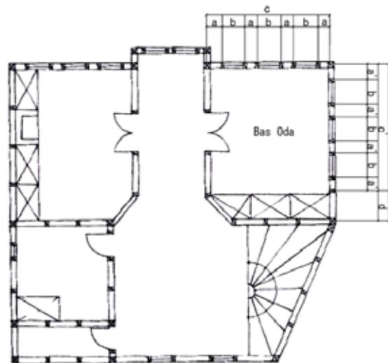
Figure 4-19 The Post arrangement of the *baş oda*.
