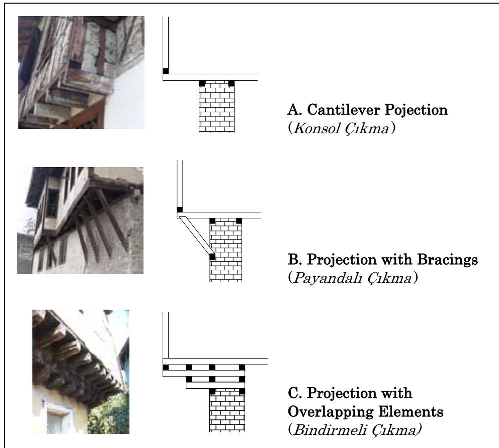
Figure 4-17 Three types of the projection
