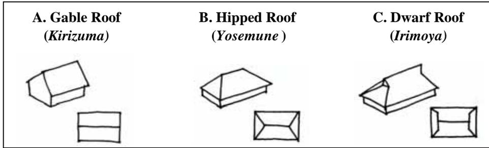
Figure 4-37 Three types of typical Japanese roof
