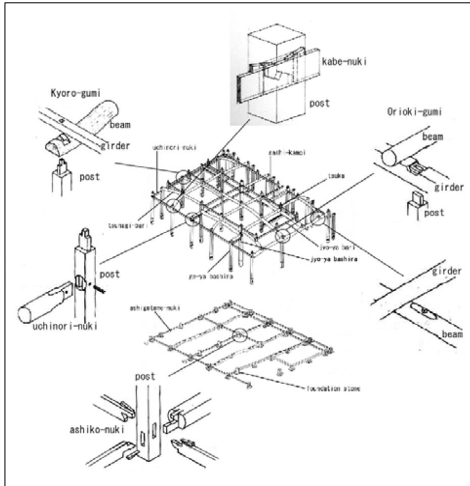
Figure 4-28 Joint of the Japanese timber framing
