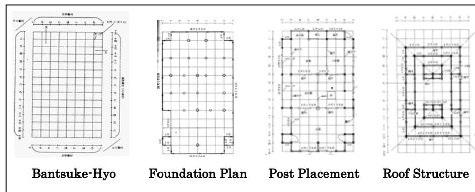
Figure 4-32 *Bantsuke-hyo* and arrangement of the structural components (Source: Fukaya, 2001: Mokuzou Kenchiku Dentou Gihou Jiten: 568-571)
