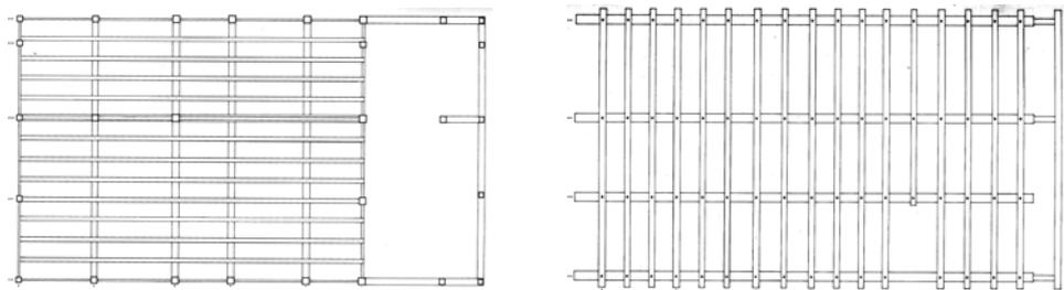
Figure 4-24 The floor joists of the ground floor (right) and the upper floor (left) (Source: Toyama Prefecture, 1979: 22)
