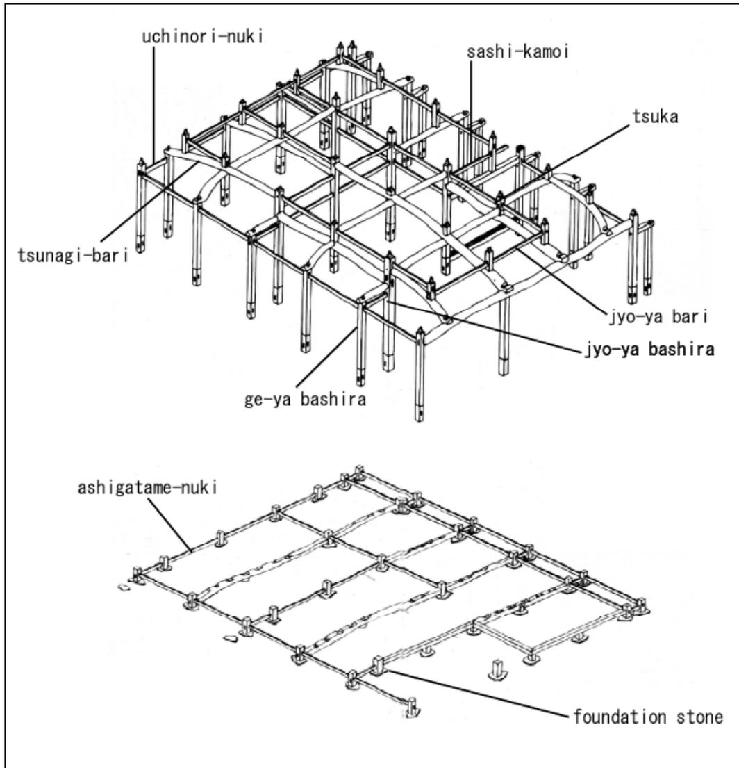
Figure 4-10 Timber structure and components of the Japanese House
