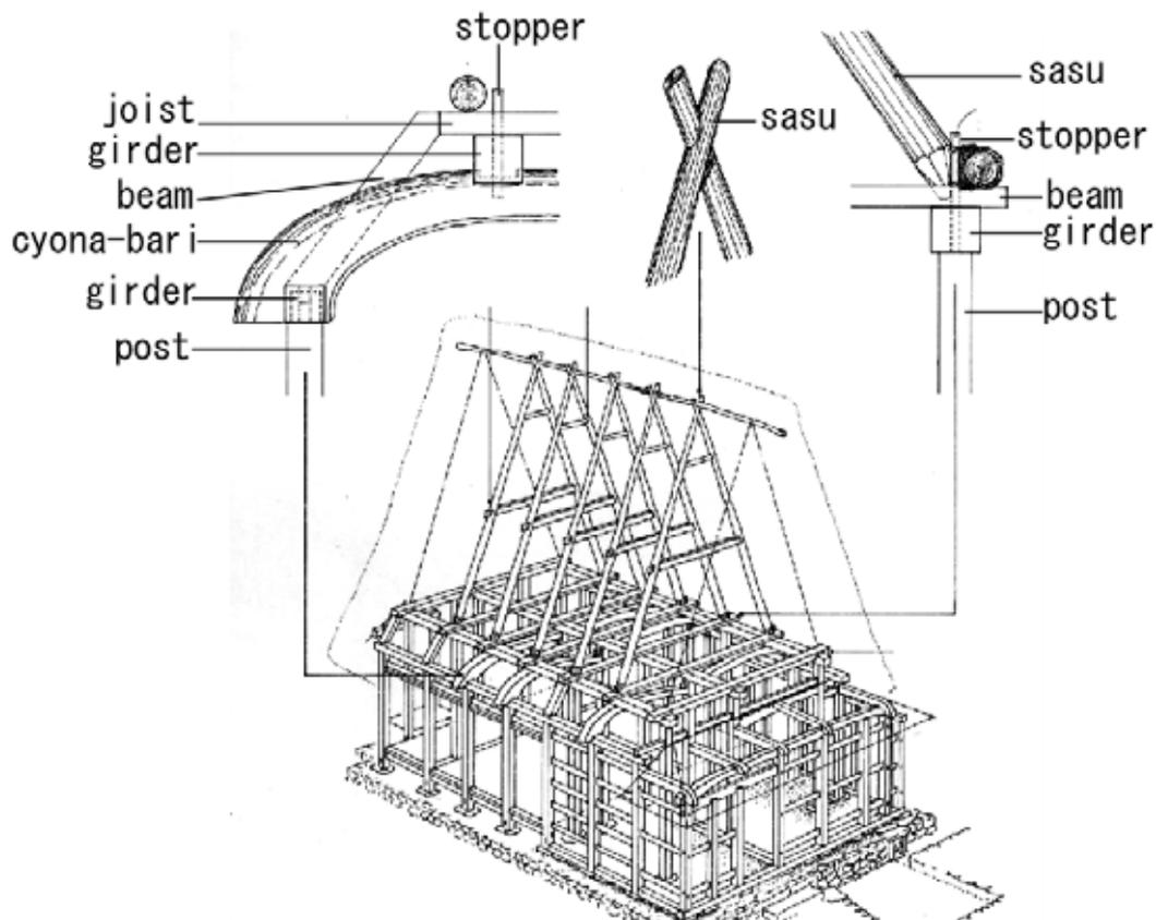
Figure 4-40 The joints used in the roof structure
