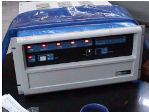
*Figure 3.20 LDS PA 500 power amplifier*
