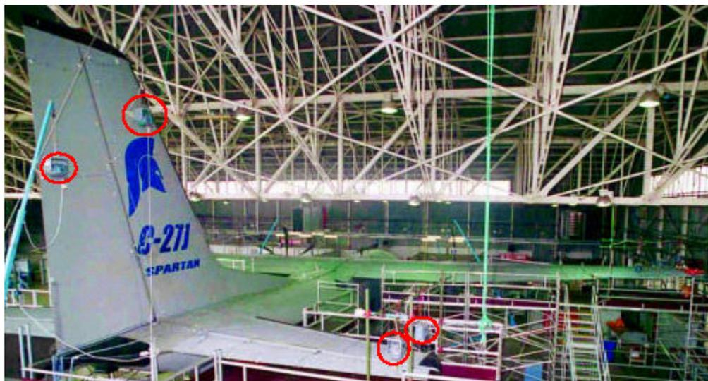
*Figure 2.17 Suspended shakers (inside the circles) [16]*
