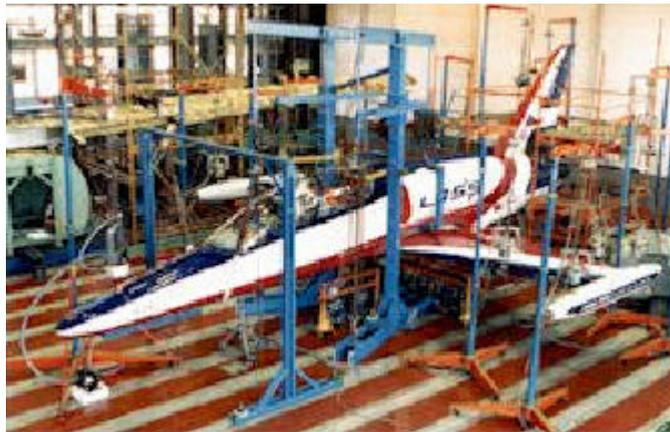
*Figure 1.1* Vibration test and analysis for a plane
