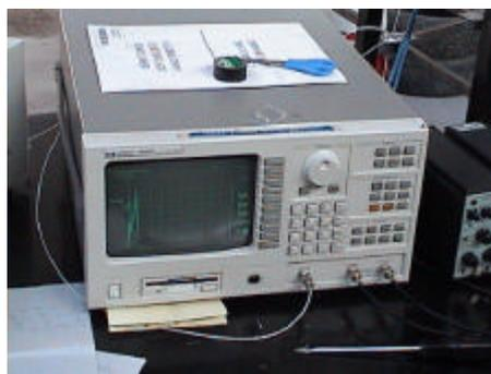
*Figure 3.21 Agilent 35665A 2-channel dynamic signal analyzer*
