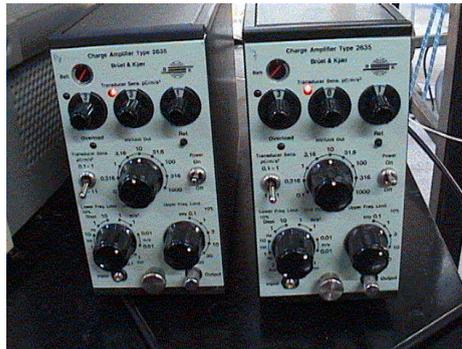
*Figure 3.24 B&K charge amplifier type 2635*
