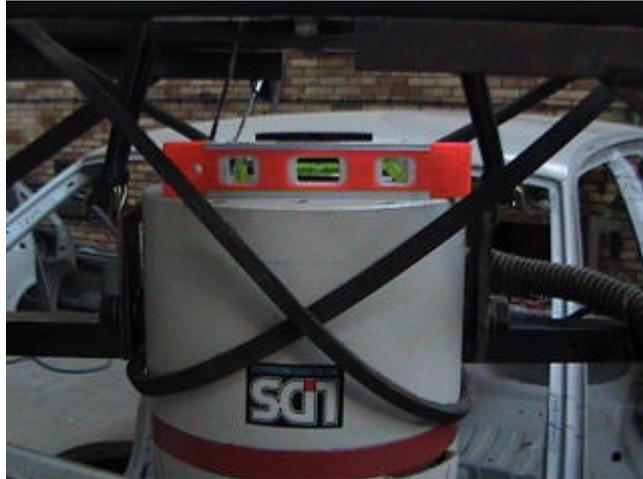
*Figure 3.10 Alignment adjustments for shaker*
