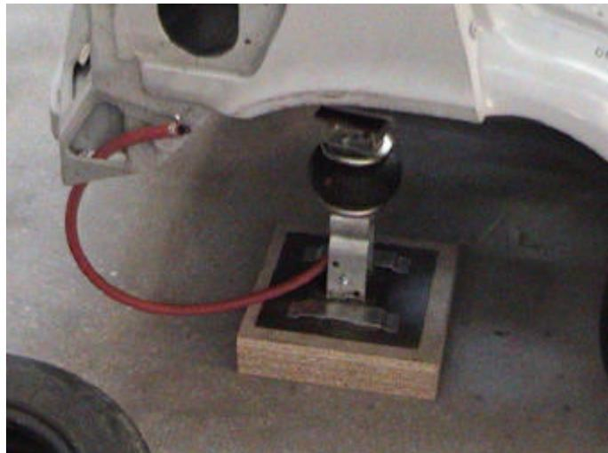
*Figure 3.6 Rear support assembled*
