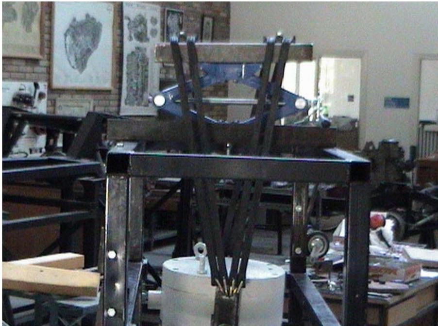
*Figure 3.9 Elastic ropes and mechanical jack*
