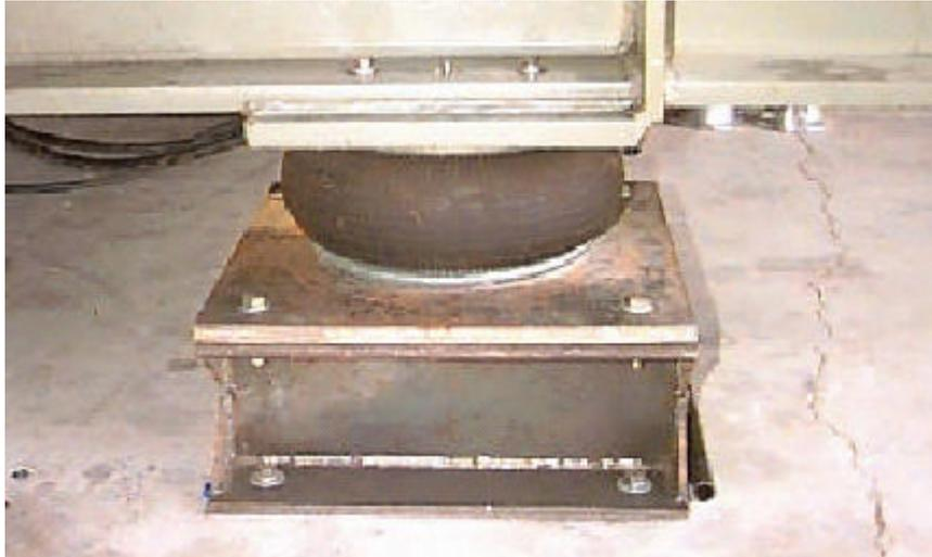
*Figure 2.11 Locomotive cab supported with air springs*
