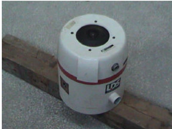
*Figure 3.18 LDS V450 electrodynamic shaker*
