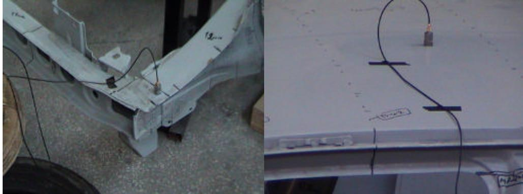
*Figure 3.16 Accelerometer mounted on body using bees-wax*
