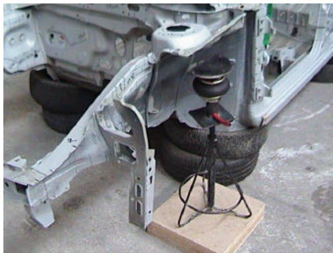
*Figure 3.3 Front air spring support parts together*
