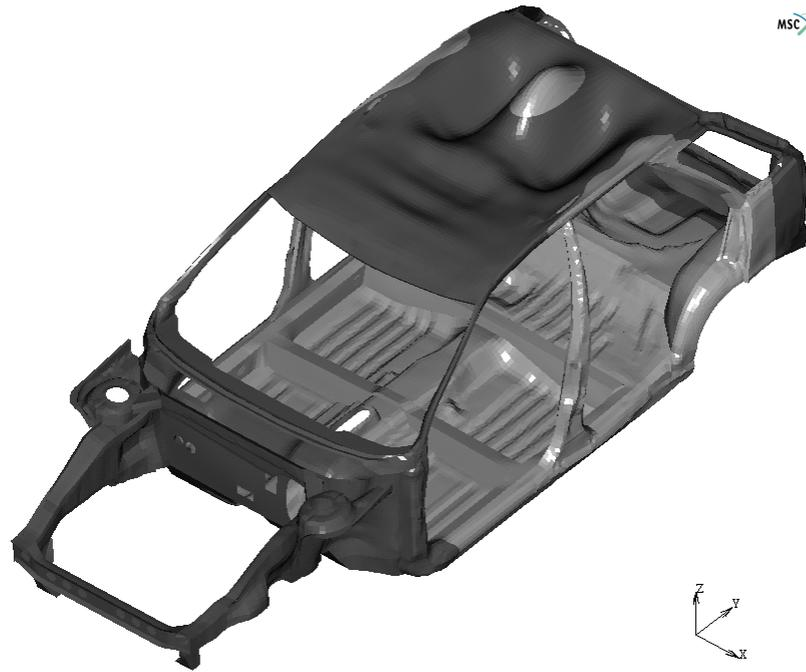
*Figure 5.9 1<sup>st</sup> bending mode @42.2 Hz, FEA*
