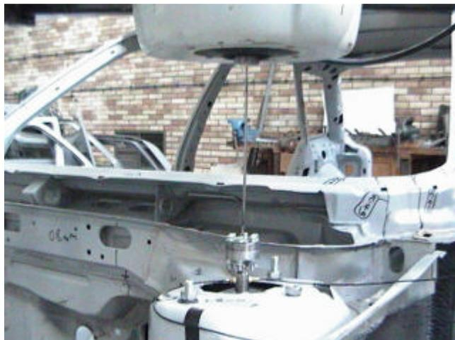
*Figure 3.11 Stinger and its connections*
