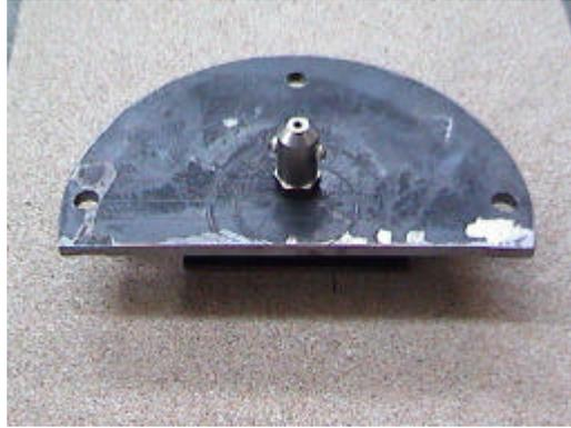
*Figure 3.13 Impedance head attached to front top adaptor part*
