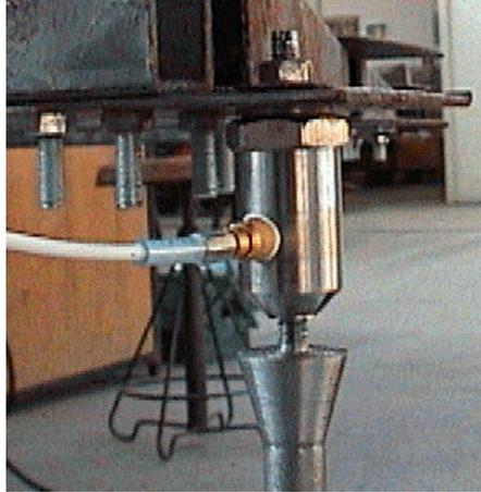
*Figure 2.18 Impedance head connected to bridge base model [17]*
