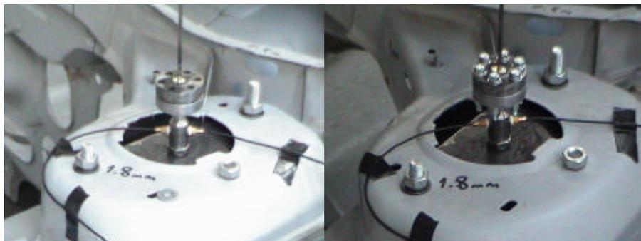
*Figure 3.15 Stinger and cable connections to impedance head*
