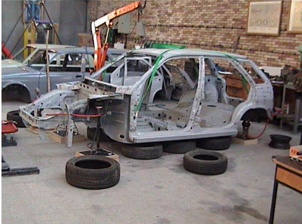
*Figure 3.7 Body-in-white with air spring supports*
