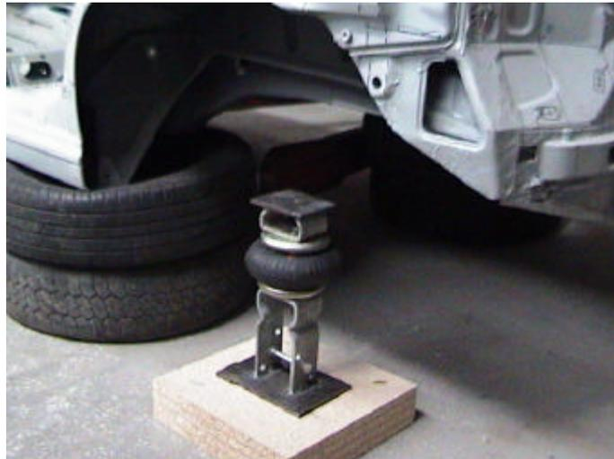
*Figure 3.5 Rear air spring support parts together*
