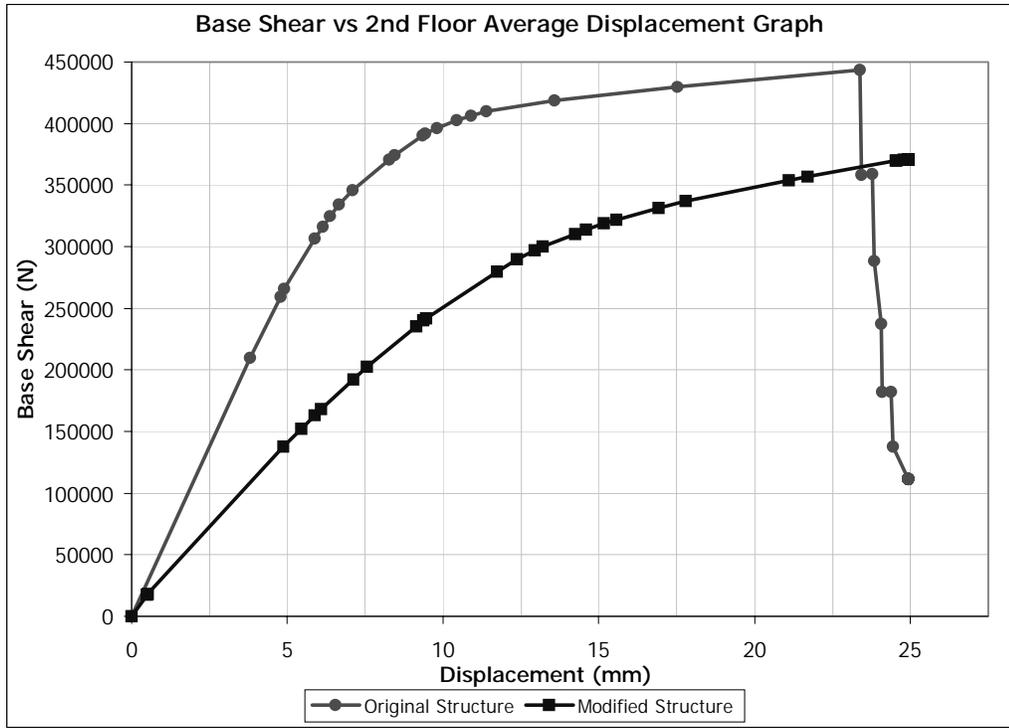
Figure 5.50 (+) X Direction Pushover for Building 2. Removed Member: C0109
