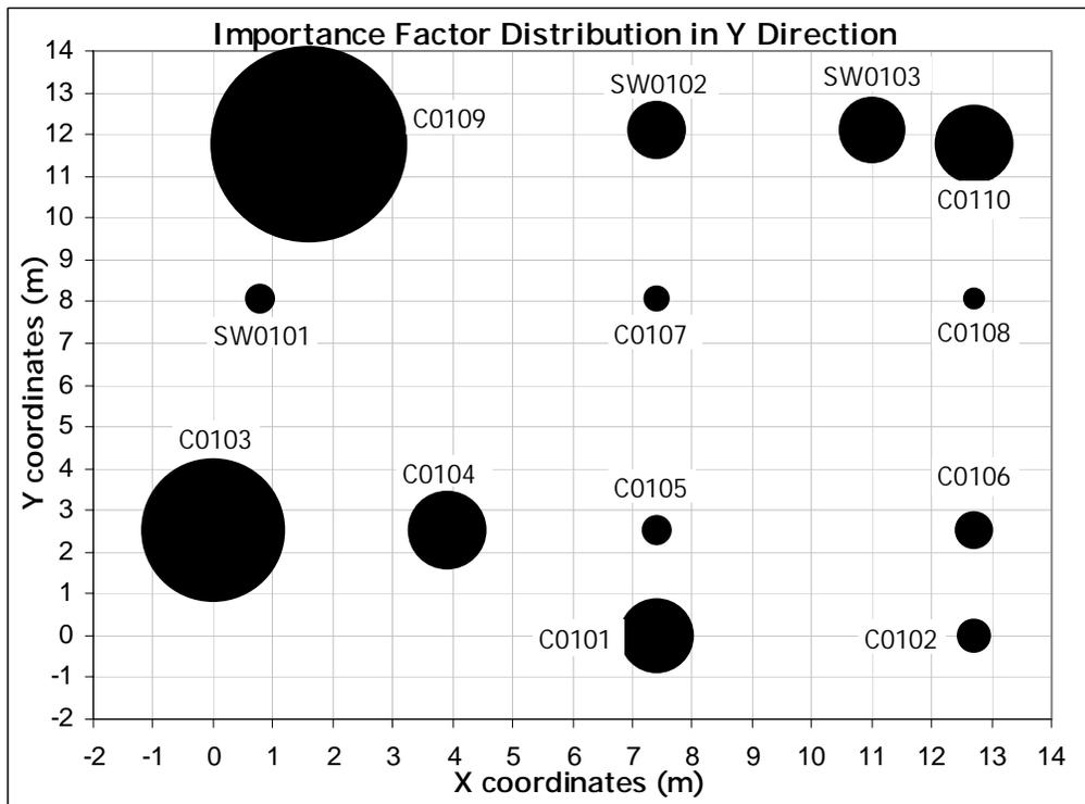
Figure 5.129 Importance Factor Distribution in Y Direction for Building 4
