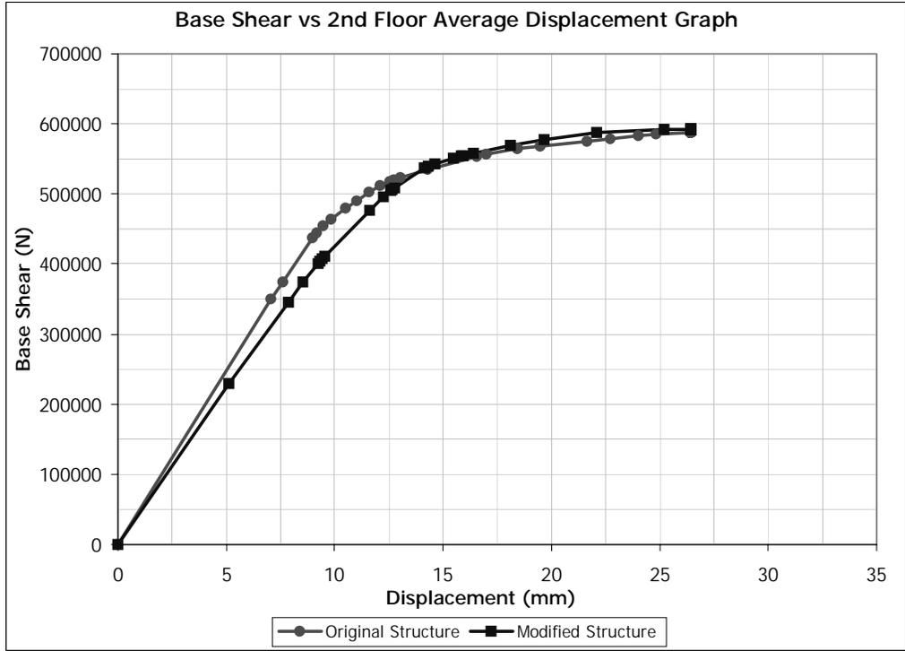
Figure 5.18 (-) X Direction Pushover for Building 1. Removed Member: C0101
