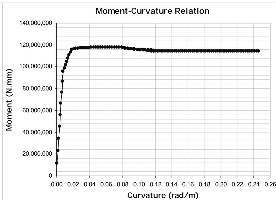
Figure 3.8 Moment Curvature Relation for Axial Load = 0 kN
