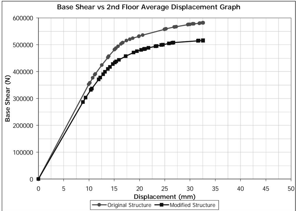
Figure 5.75 (-) Y Direction Pushover for Building 3. Removed Member: C0103
