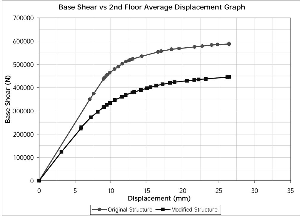
Figure 5.24 (-) X Direction Pushover for Building 1. Removed Member: C0107
