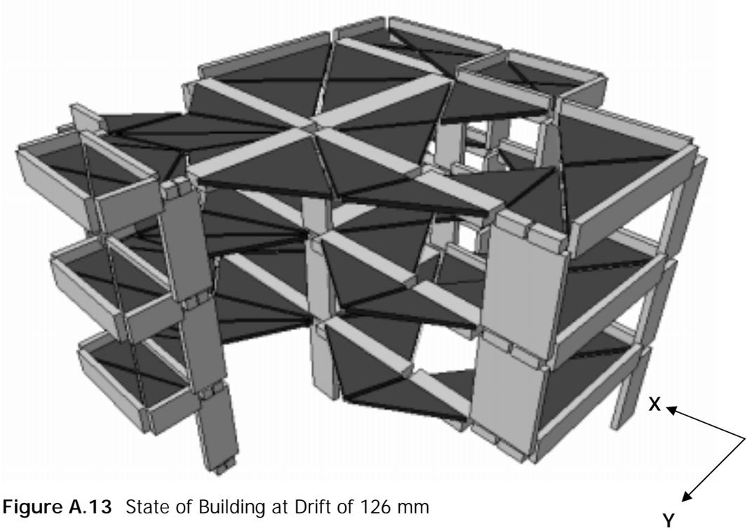
Figure A.13 State of Building at Drift of 126 mm
