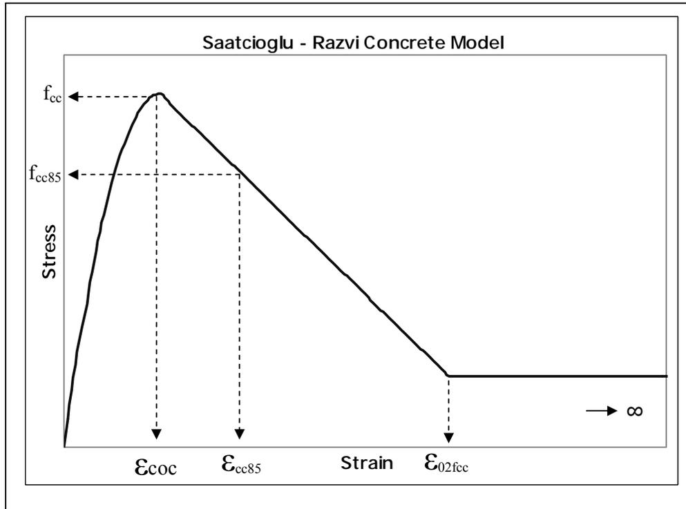
Figure 3.3 Saatcioglu – Razvi Concrete Model
