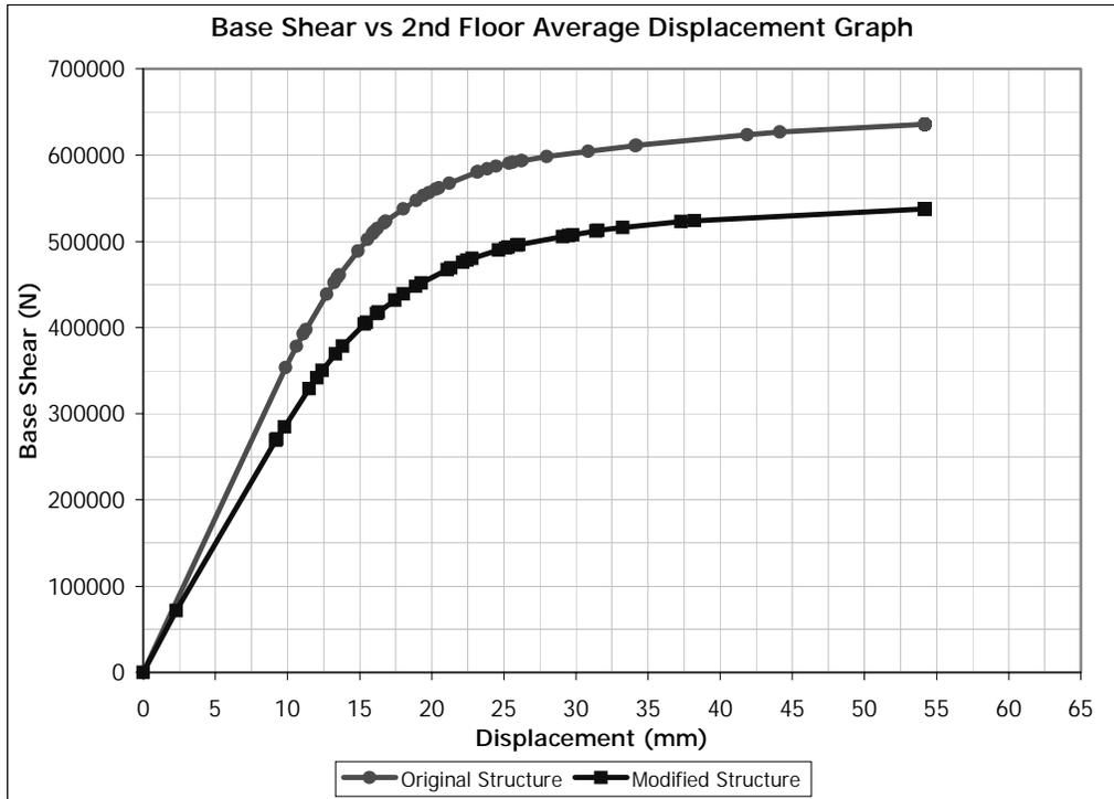
Figure 5.32 (-) Y Direction Pushover for Building 1. Removed Member C0106
