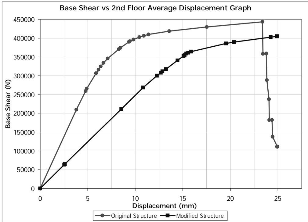
Figure 5.51 (+) X Direction Pushover for Building 2. Removed Member: SW0101
