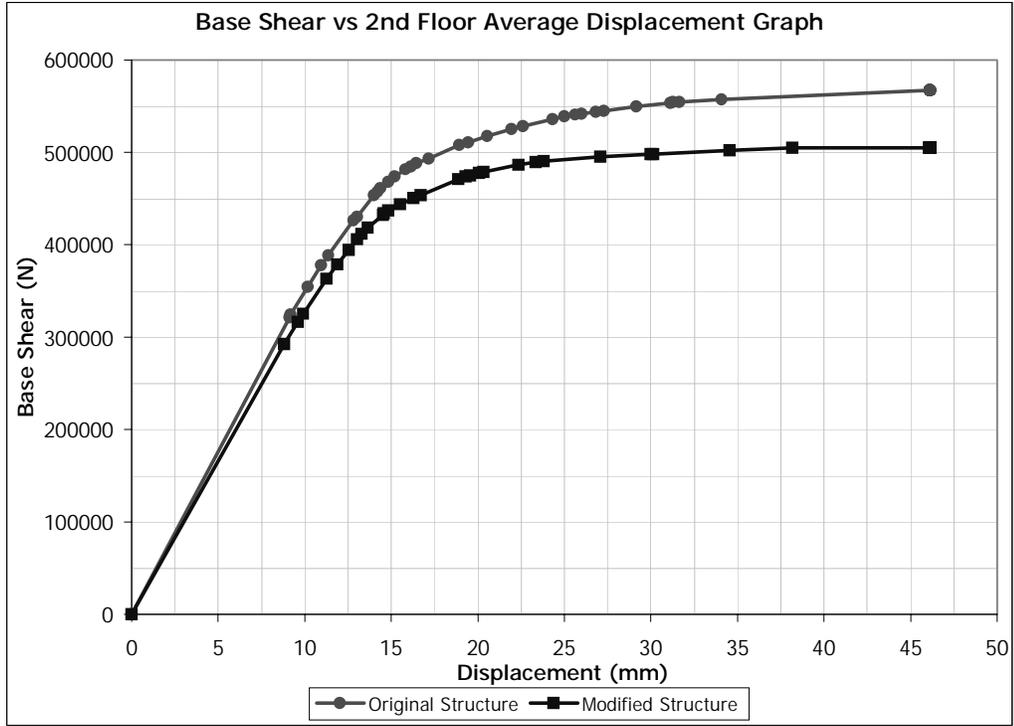
Figure 5.74 (+) Y Direction Pushover for Building 3. Removed Member: C0102
