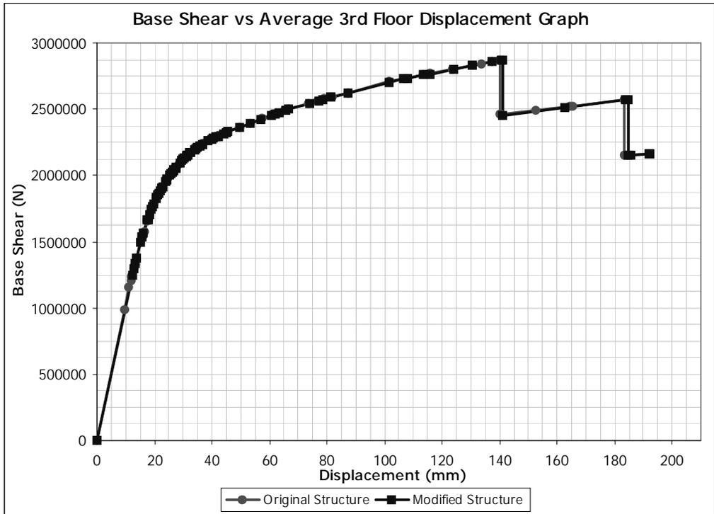
Figure 5.132 (+) Y Direction Pushover for Building 4. Removed Member: B0116
