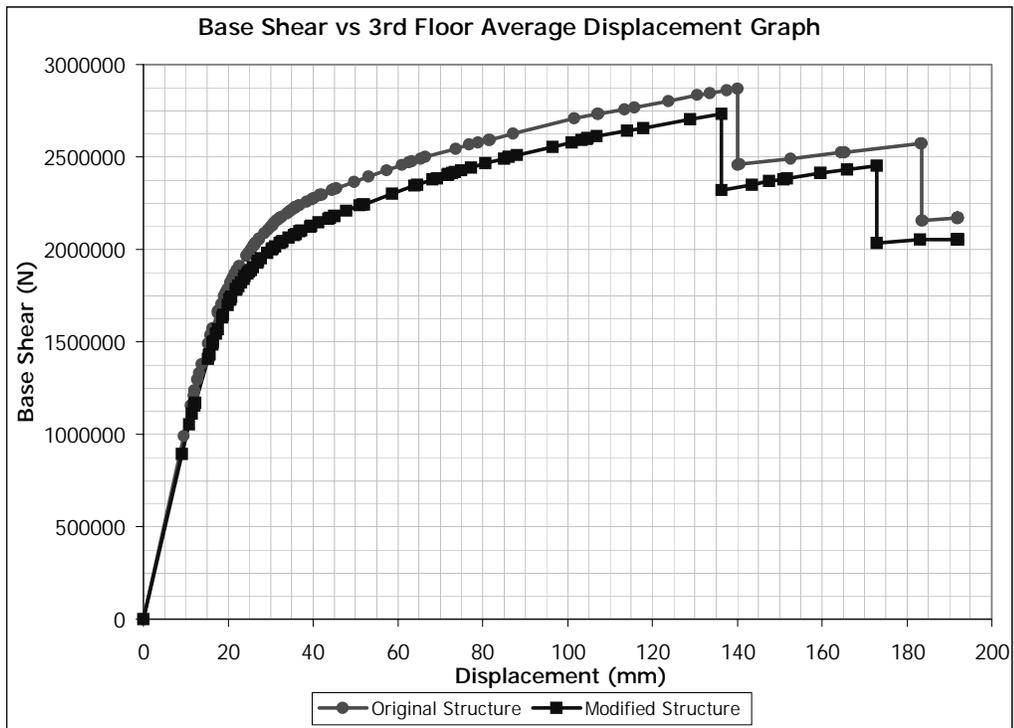
Figure 5.118 (+) Y Direction Pushover for Building 4. Removed Member: C0105
