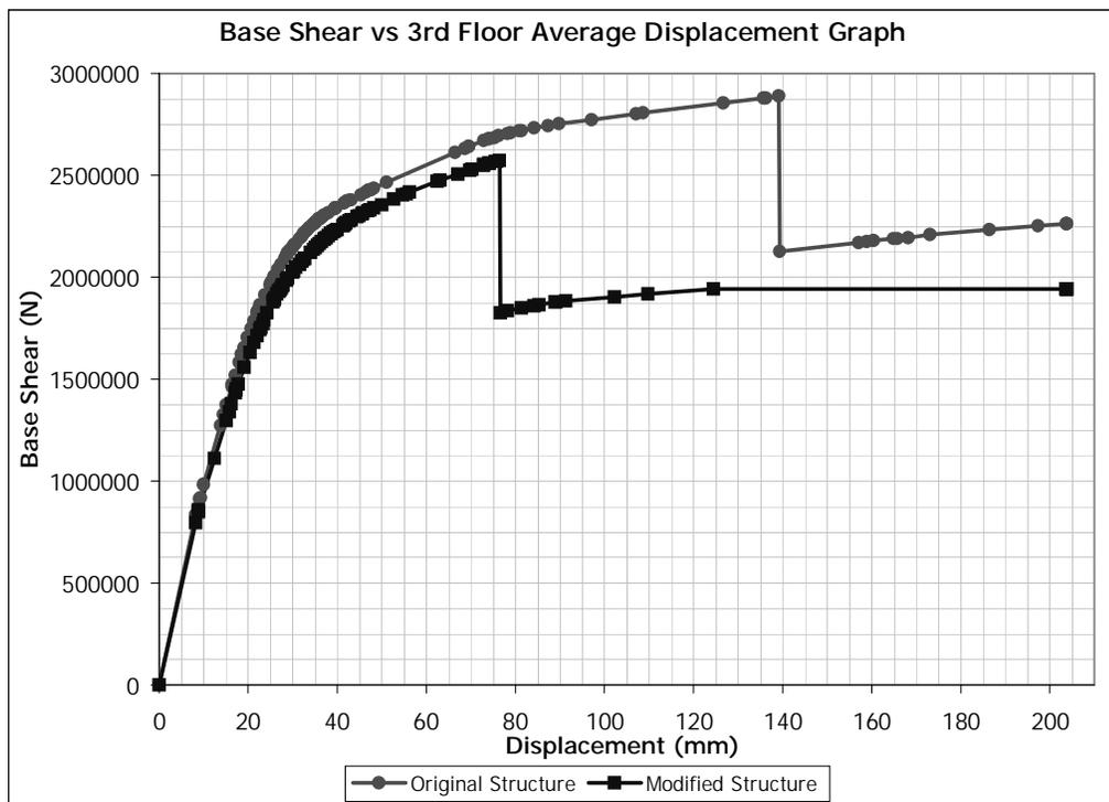
Figure 5.108 (+) X Direction Pushover for Building 4. Removed Member: C0108
