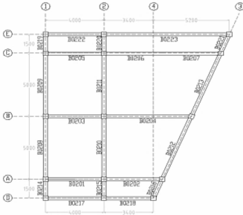
**Figure 5.9** 2<sup>nd</sup> Floor Plan of Test Building
