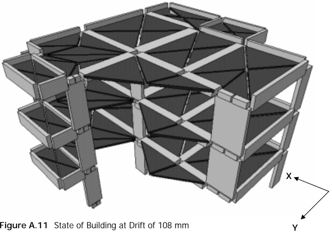
Figure A.11 State of Building at Drift of 108 mm
