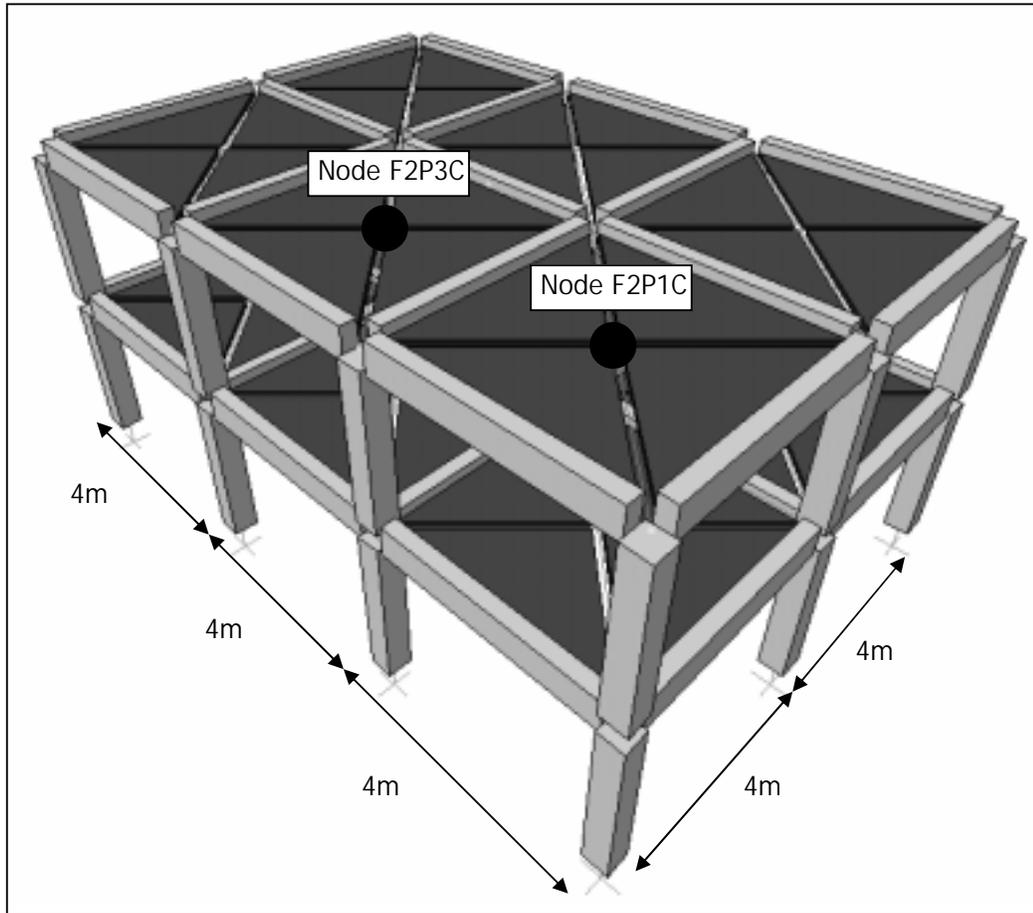
Figure B.1 3D Model of the Test Building with Floor Plan dimensions
