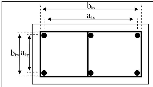
Figure 3.4 Cross-Section Dimension Variables
