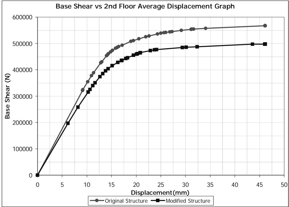
Figure 5.76 (+) Y Direction Pushover for Building 3. Removed Member: C0104
