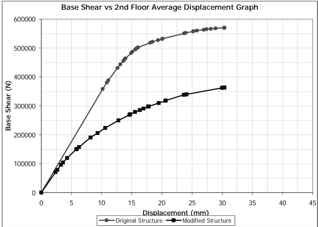
Figure 5.59 (-) Y Direction Pushover for Building 2. Removed Member: SW0101
