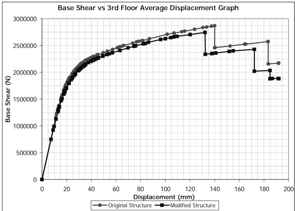
Figure 5.124 (+) Y Direction Pushover for Building 4. Removed Member: SW0101
