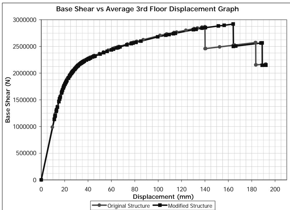
Figure 5.134 (+) Y Direction Pushover for Building 4. Removed Member: B0118
