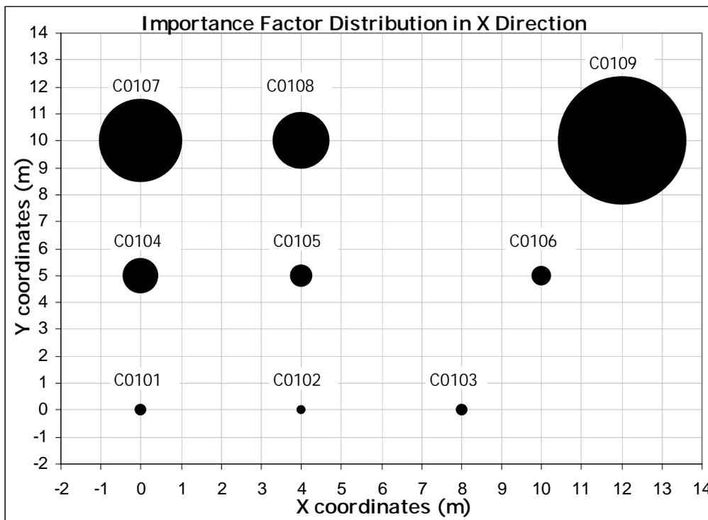
Figure 5.39 Importance Factor Distribution in X Direction for Building 1
