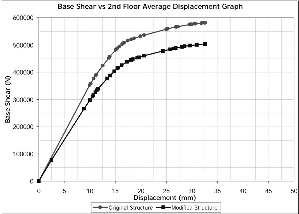
Figure 5.78 (-) Y Direction Pushover for Building 3. Removed Member: C0106
