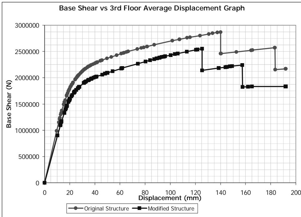
Figure 5.114 (+) Y Direction Pushover for Building 4. Removed Member: C0101
