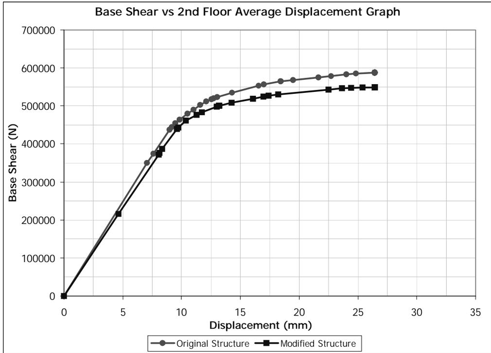
Figure 5.23 (-) X Direction Pushover for Building 1. Removed Member: C0106
