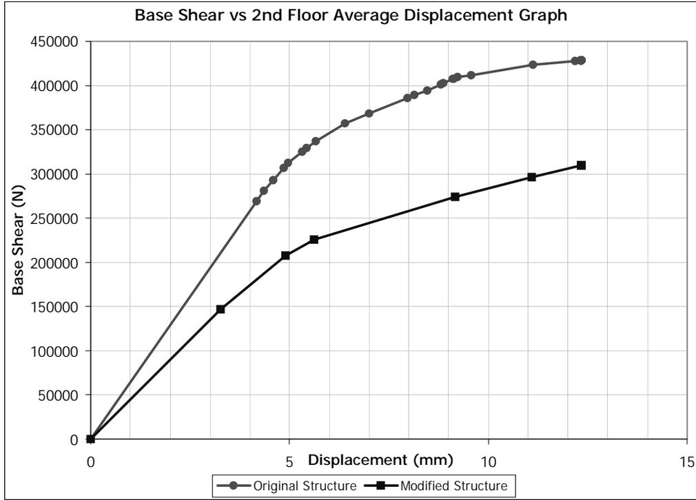
Figure 5.72 (+) X Direction Pushover for Building 3. Removed Member: SW0102
