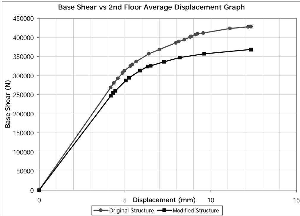
Figure 5.71 (+) X Direction Pushover for Building 3. Removed Member: C0109
