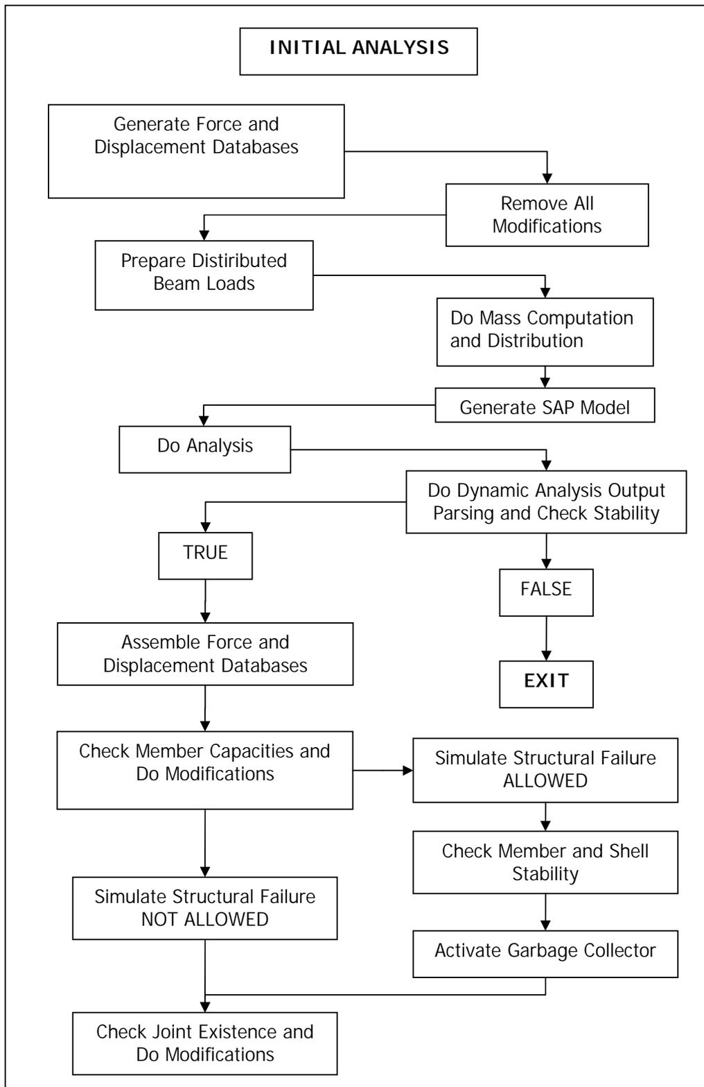
**Figure 2.3** "Initial Analysis" Module Program Layout
