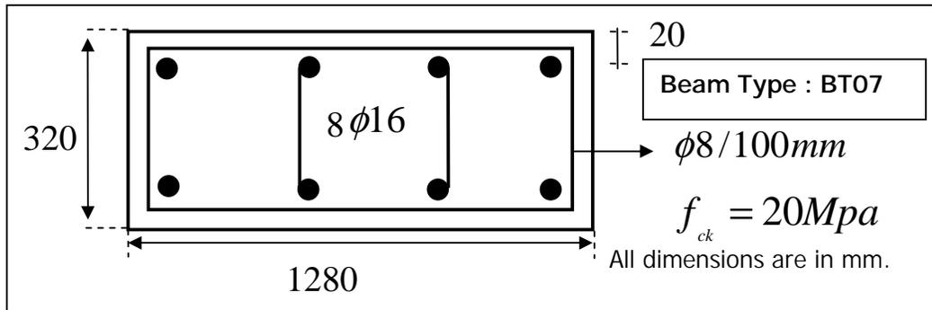
Figure 5.90 Details of Beam Type BT07
