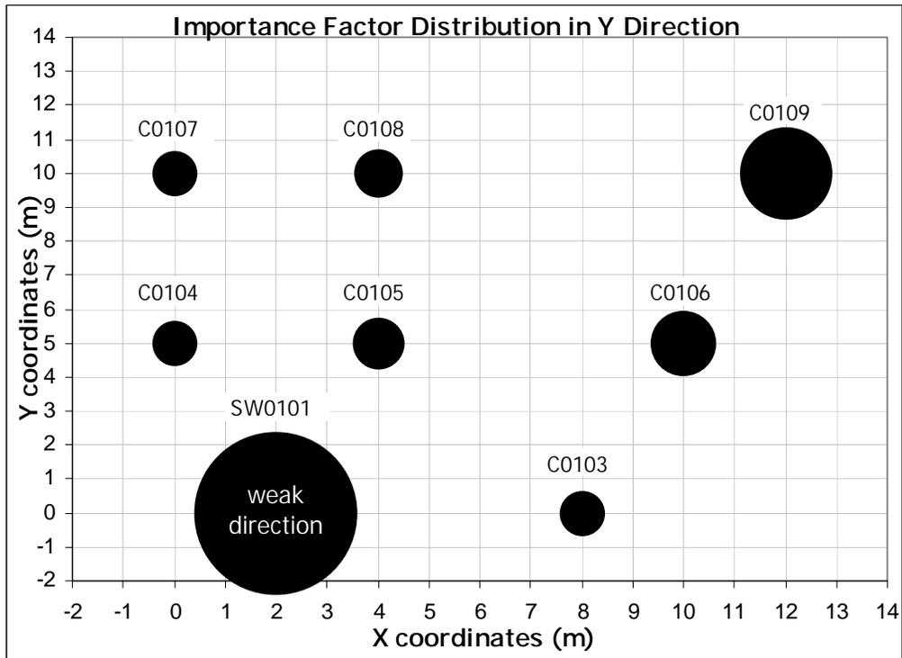
Figure 5.62 Importance Factor Distribution in Y Direction for Building 2
