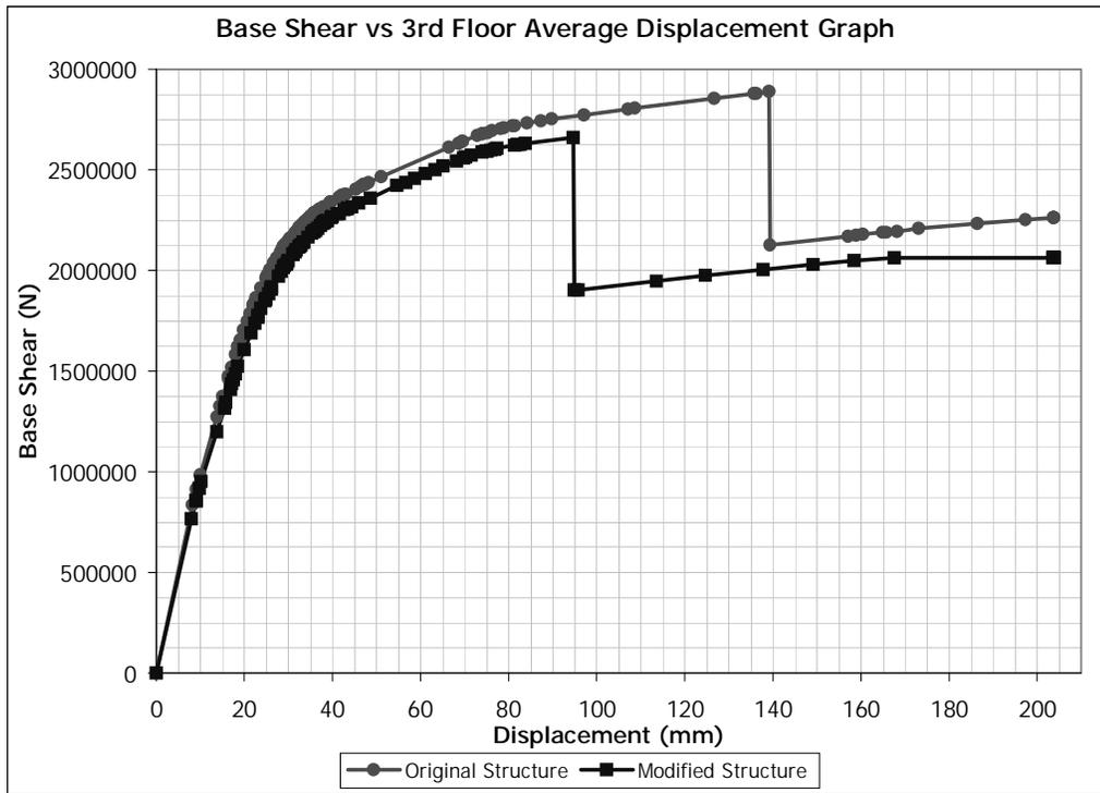
Figure 5.110 (+) X Direction Pushover for Building 4. Removed Member: C0110
