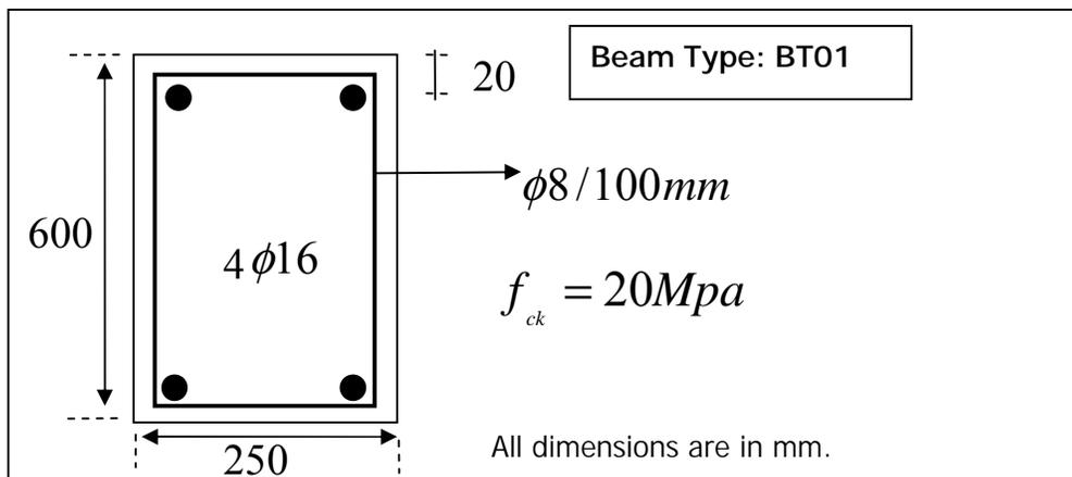
Figure 5.4 Details of Beam Type BT01
