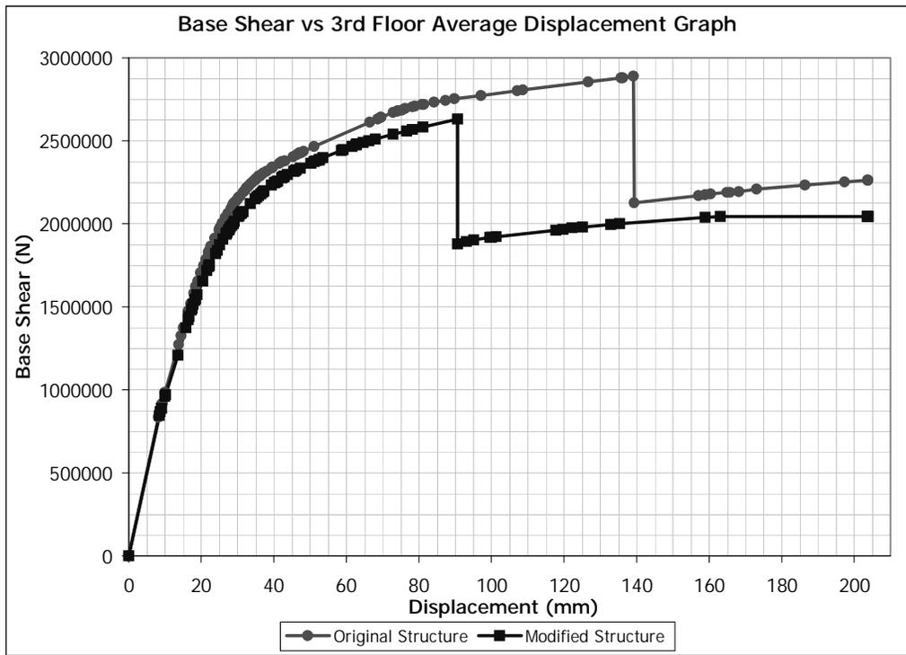
Figure 5.109 (+) X Direction Pushover for Building 4. Removed Member: C0109
