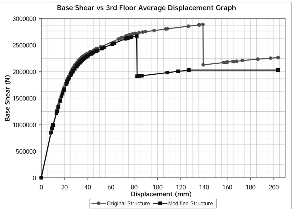
Figure 5.102 (+) X Direction Pushover for Building 4. Removed Member: C0102
