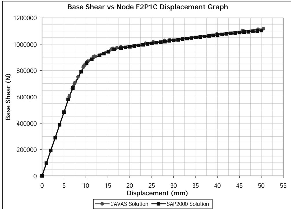
**Figure B.9** Pushover Curves obtained by CAVAS and SAP2000 in Y Direction
