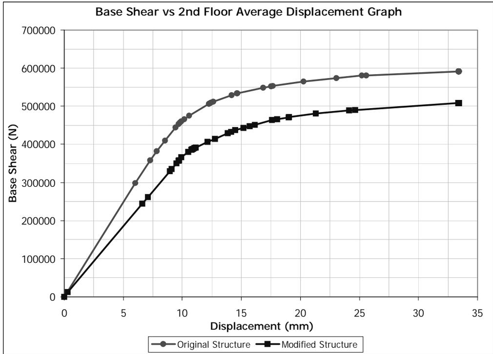
Figure 5.25 (+) X Direction Pushover for Building 1. Removed Member: C0108
