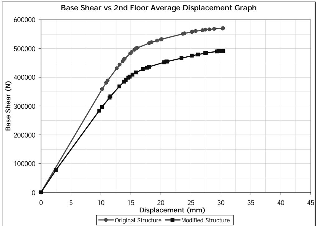
Figure 5.55 (-) Y Direction Pushover for Building 2. Removed Member: C0106
