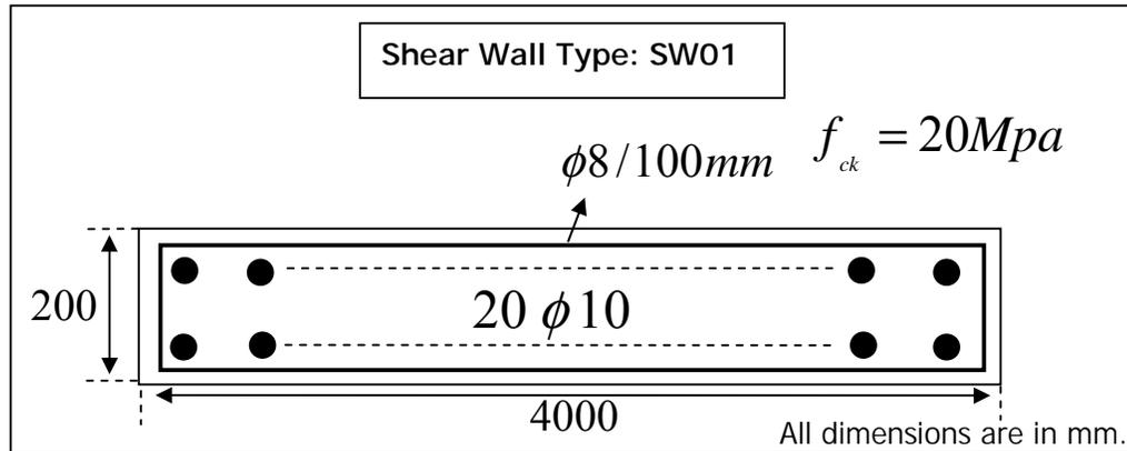
**Figure 5.41** Details of Shear Wall Type SW01
