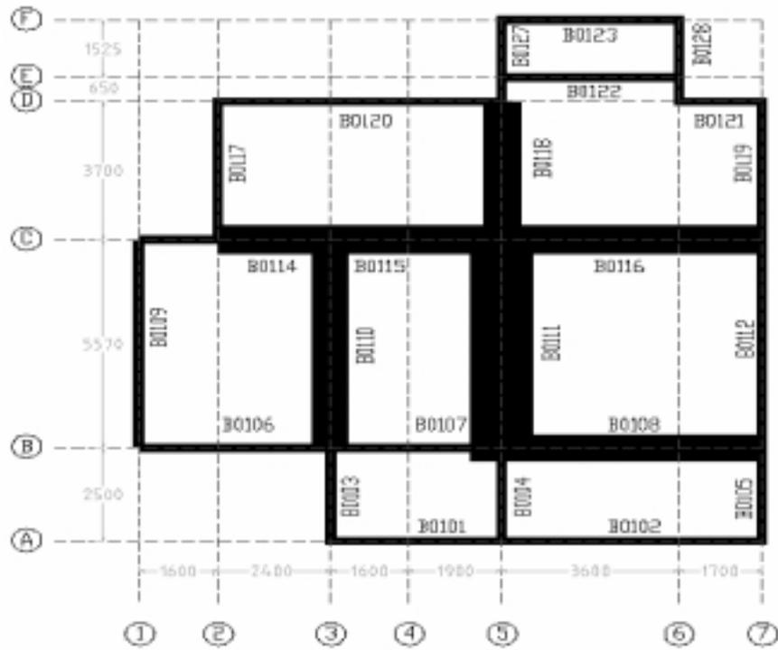
Figure 5.95 First Floor Beam Layout of Building 4
