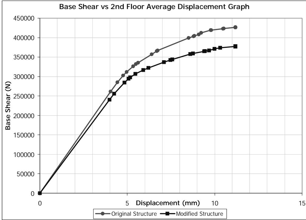
Figure 5.68 (-) X Direction Pushover for Building 3. Removed Member: C0104
