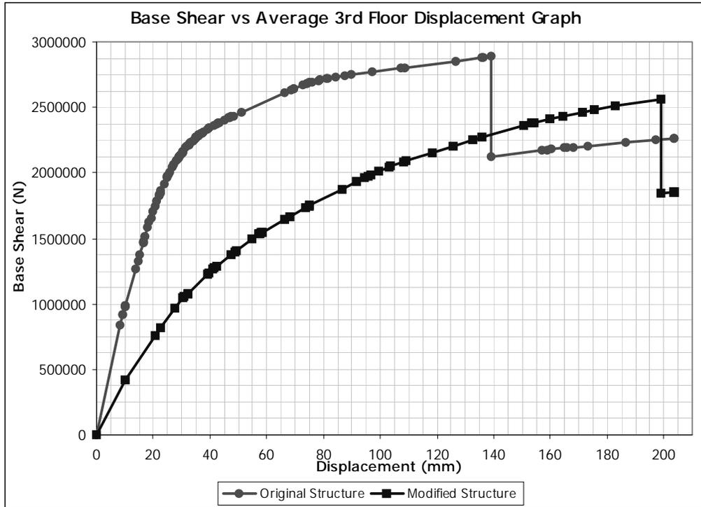
Figure 5.137 (+) X Direction Pushover for Building 4. All Floor Beams are removed
