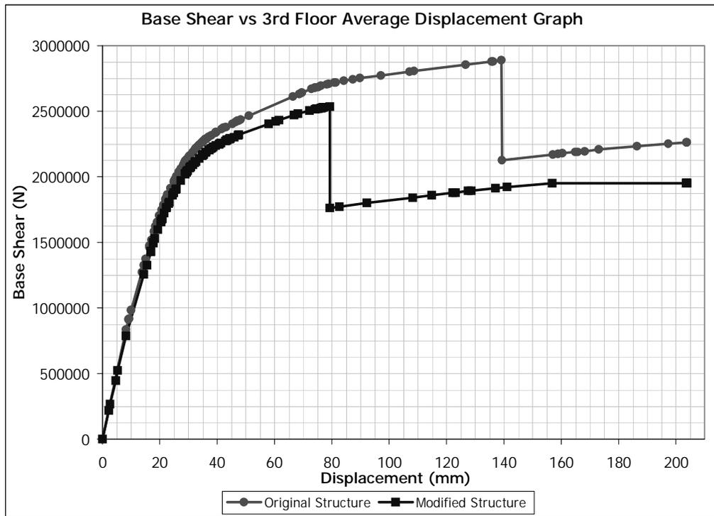
Figure 5.107 (+) X Direction Pushover for Building 4. Removed Member: C0107
