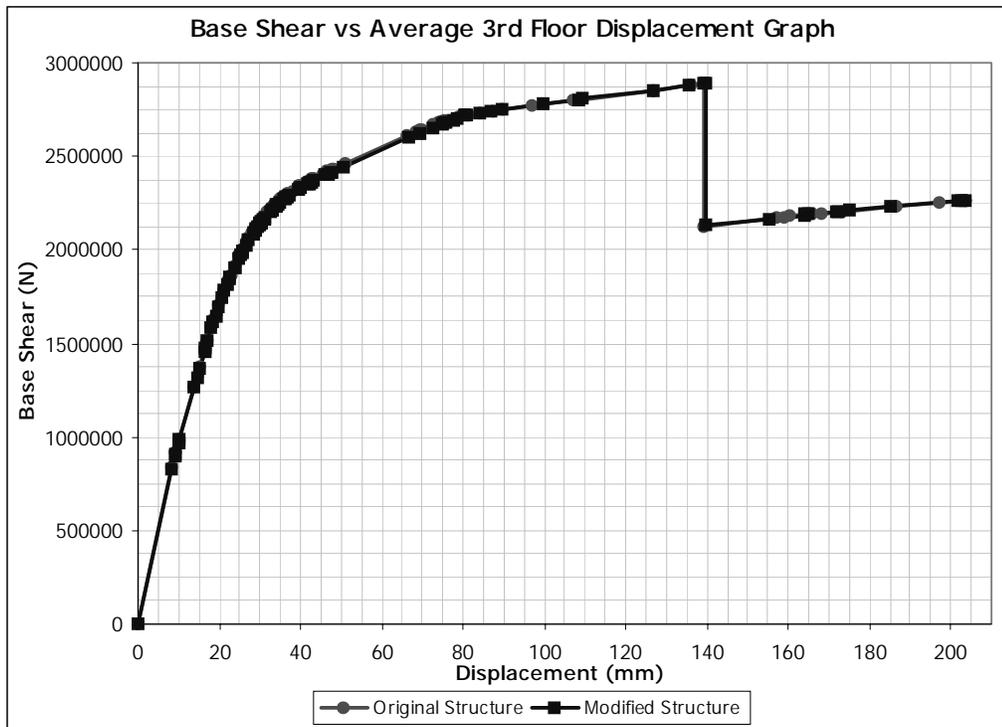
Figure 5.133 (+) X Direction Pushover for Building 4. Removed Member: B0118
