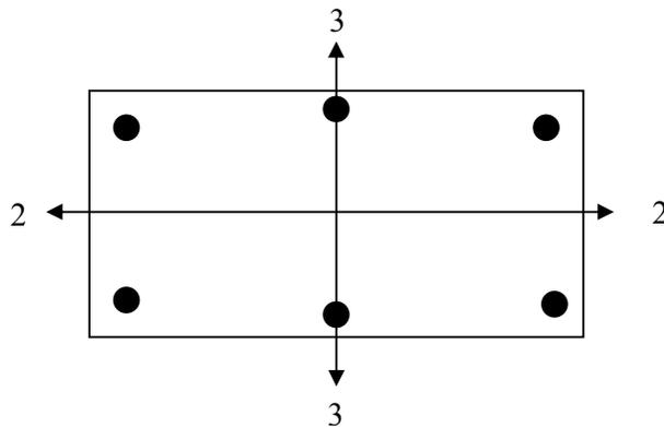
Figure 3.6 Section Axes Designation
