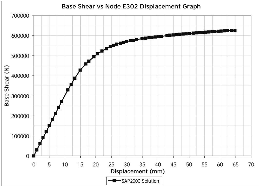
Figure 5.13 SAP2000 Pushover analysis result conducted in Y Direction
