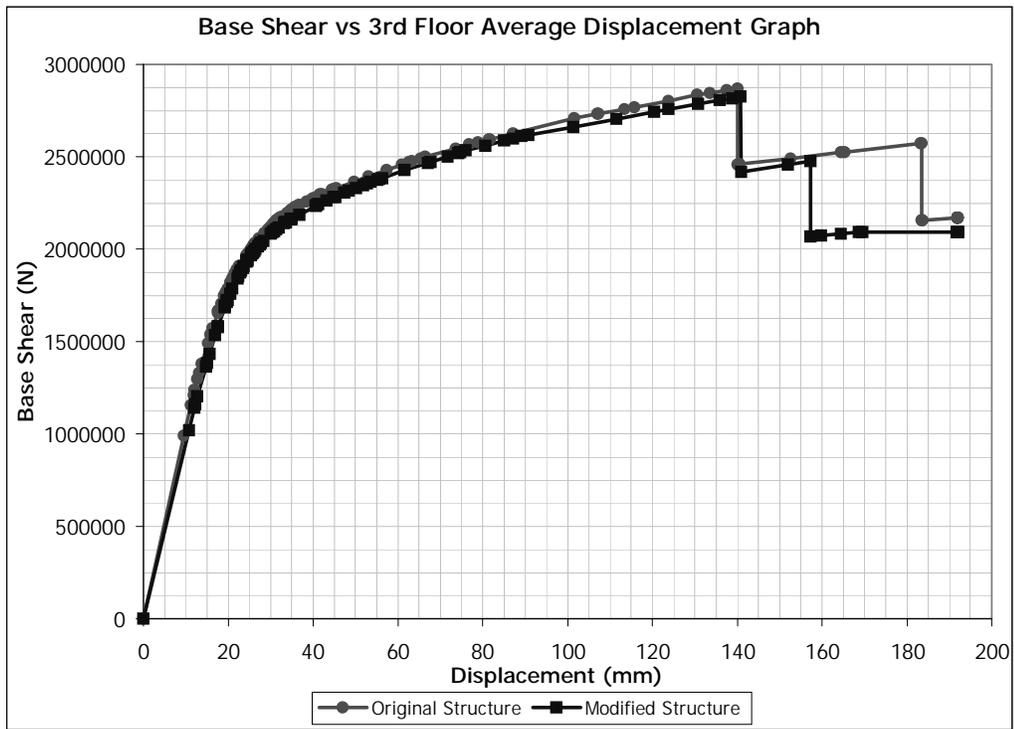
Figure 5.121 (+) Y Direction Pushover for Building 4. Removed Member: C0108
