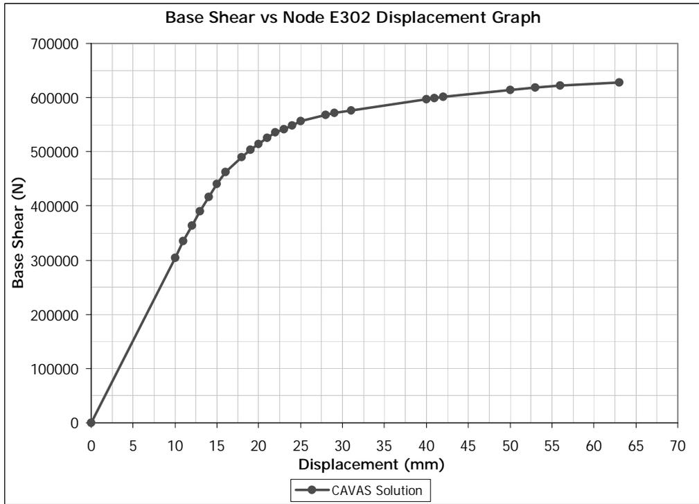
**Figure 5.11** CAVAS Pushover analysis result conducted in Y Direction
