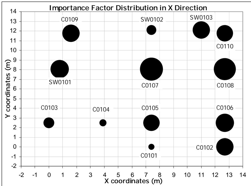
Figure 5.128 Importance Factor Distribution in X Direction for Building 4
