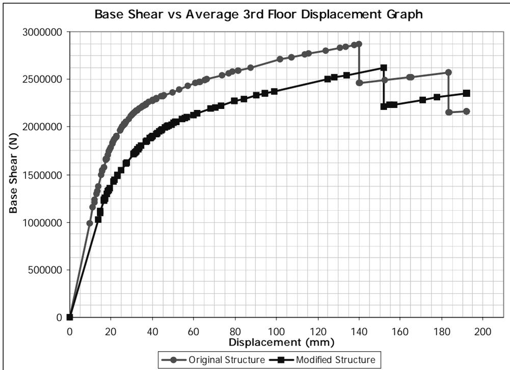
Figure 5.136 (+) Y Direction Pushover for Building 4.All First Floor Beams are removed
