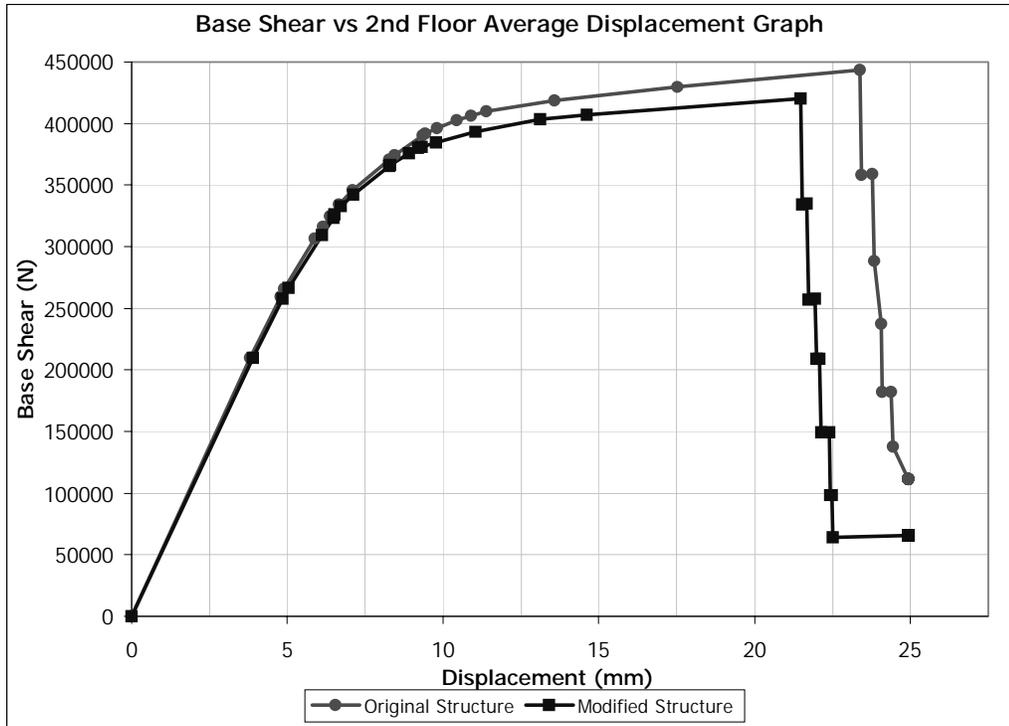
Figure 5.44 (+) X Direction Pushover for Building 2. Removed Member: C0103
