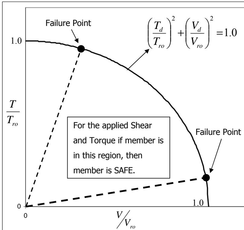
Figure 3.13 Behavior of Section under Torsion and Shear
