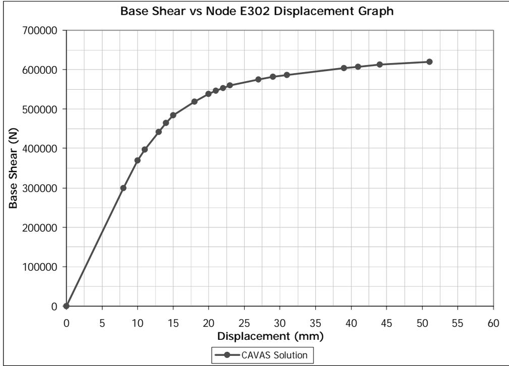
**Figure 5.10** CAVAS Pushover analysis result conducted in X Direction
