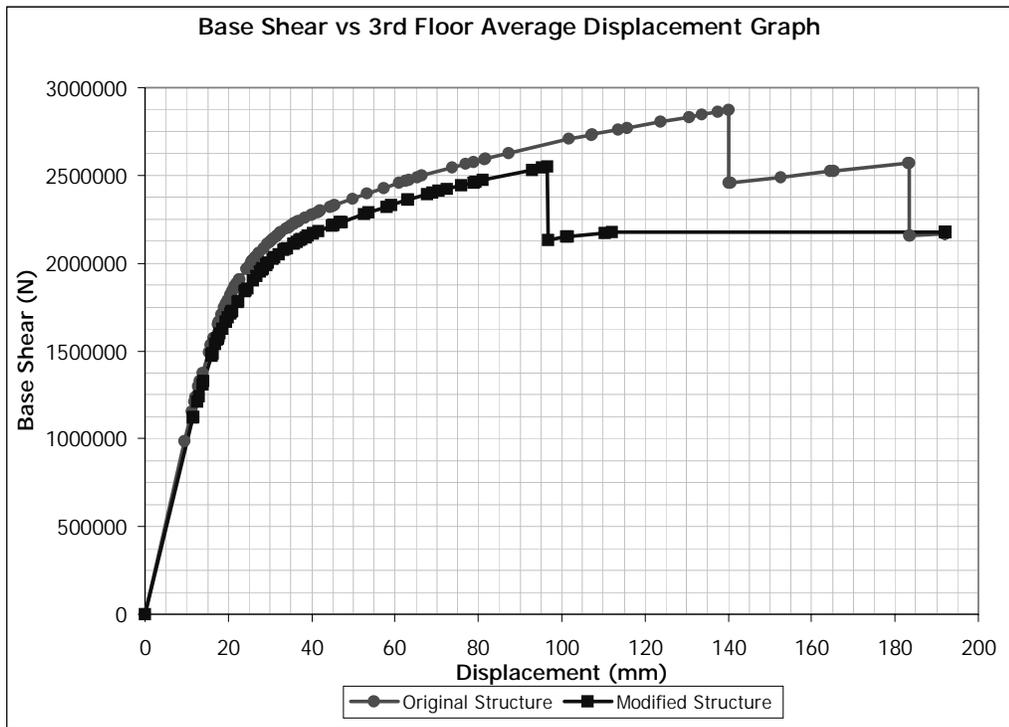
Figure 5.125 (+) Y Direction Pushover for Building 4. Removed Member: SW0102
