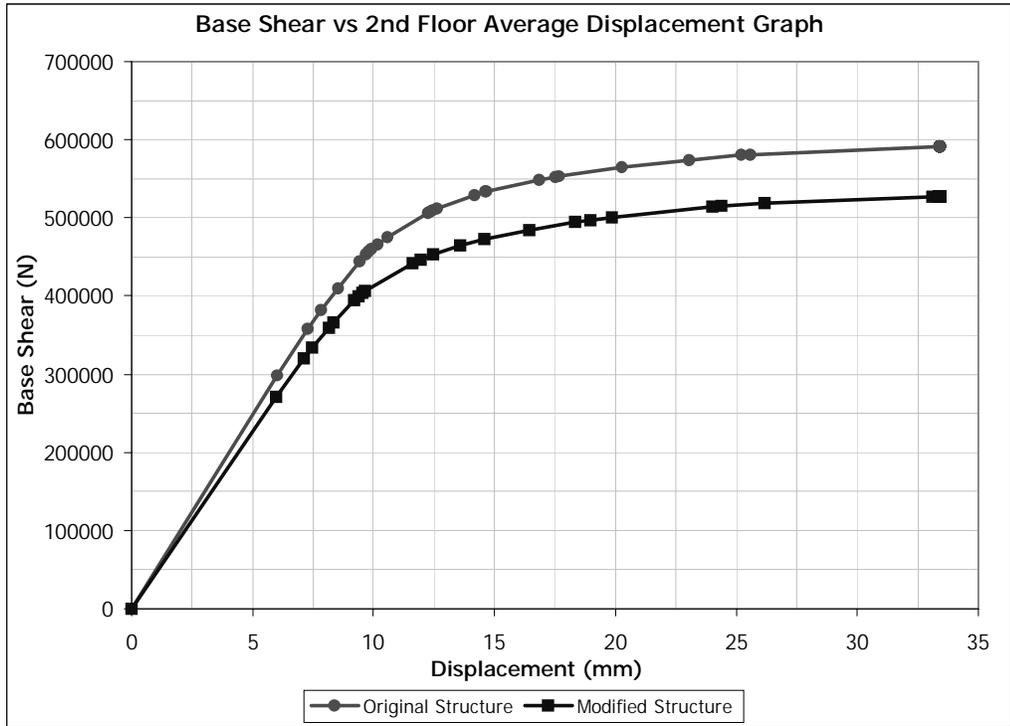
Figure 5.21 (+) X Direction Pushover for Building 1. Removed Member: C0104
