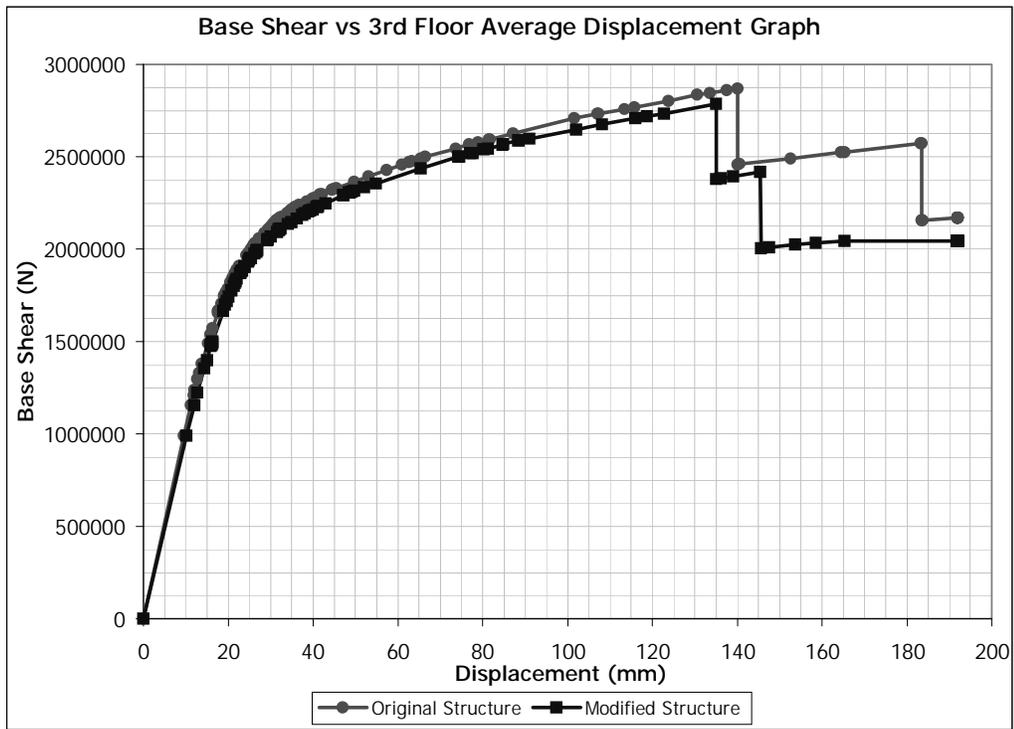
Figure 5.115 (+) Y Direction Pushover for Building 4. Removed Member: C0102
