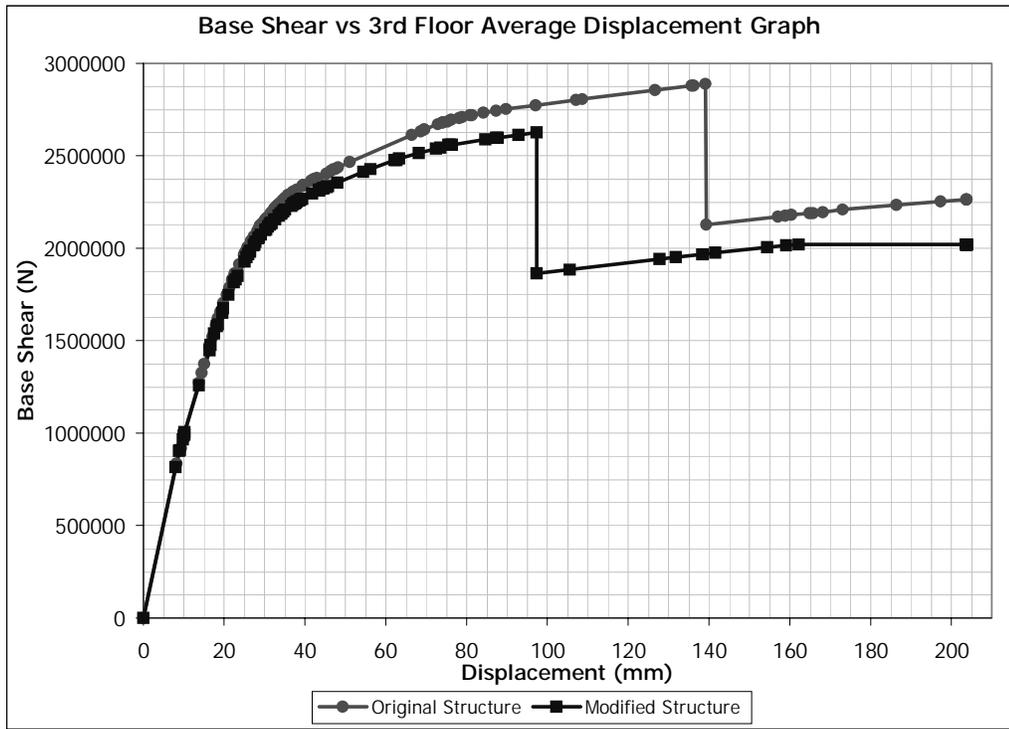
Figure 5.105 (+) X Direction Pushover for Building 4. Removed Member: C0105
