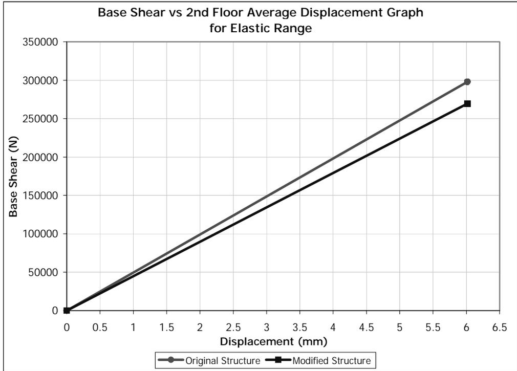
**Figure 5.37** (+) Y Direction Pushover for Elastic Range. Removed Member: C0101
