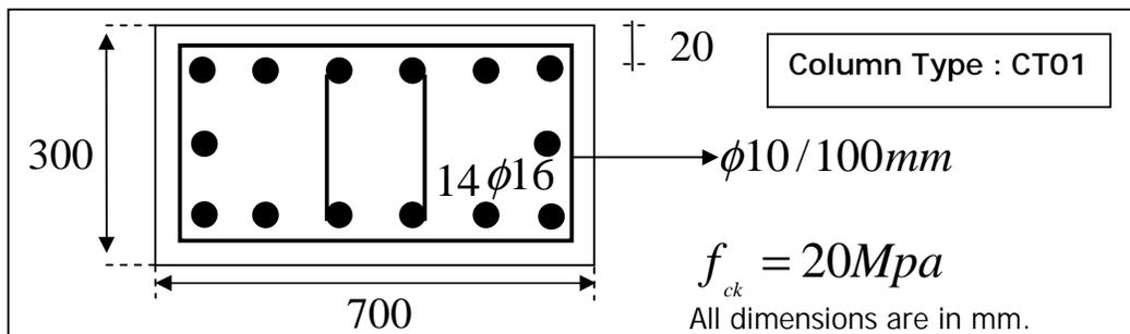
Figure 5.92 Details of Column Type CT01
