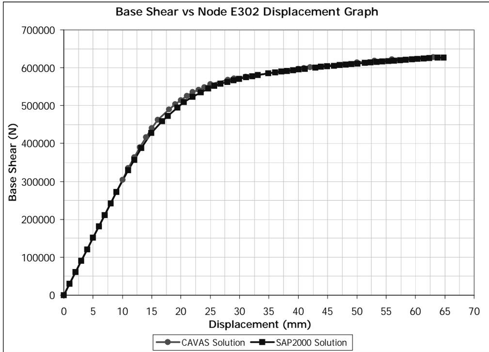
Figure 5.15 Pushover Curves obtained by CAVAS and SAP2000 in Y Direction
