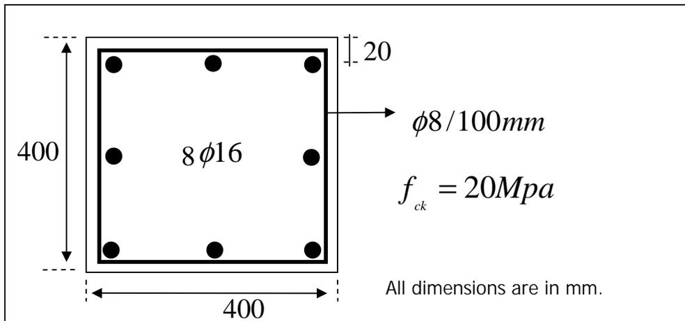
Figure B.2 Details of Columns
