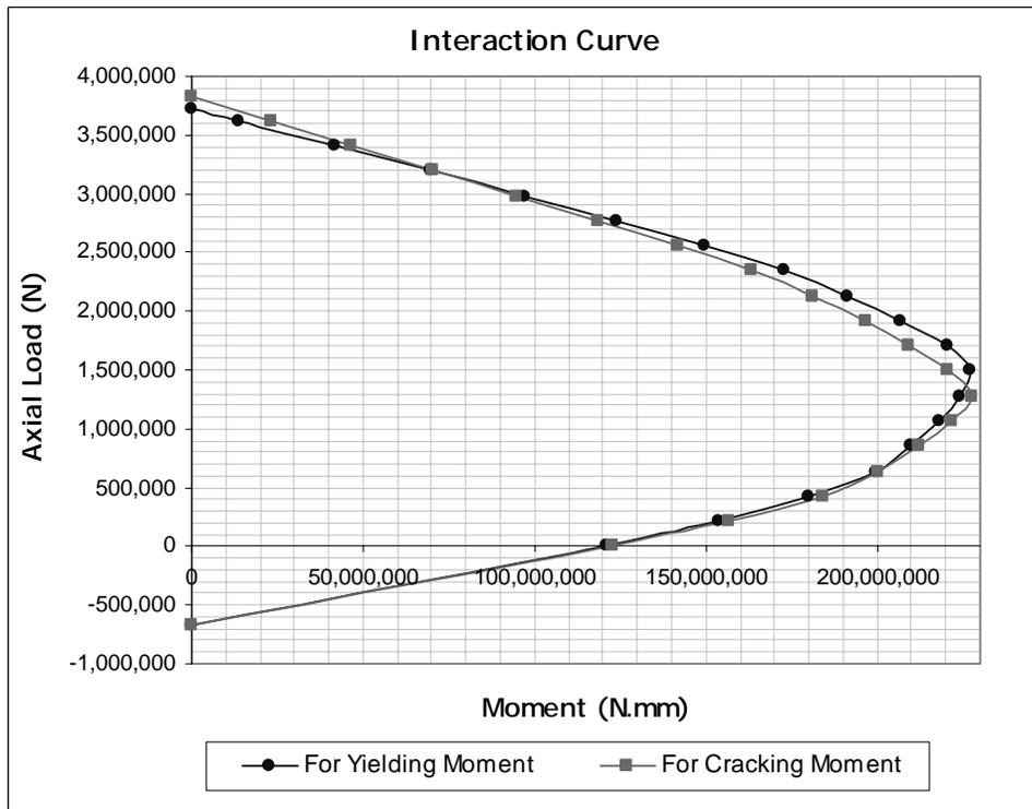
Figure 3.12 Interaction Relation for Cover Concrete Thickness = 20mm
