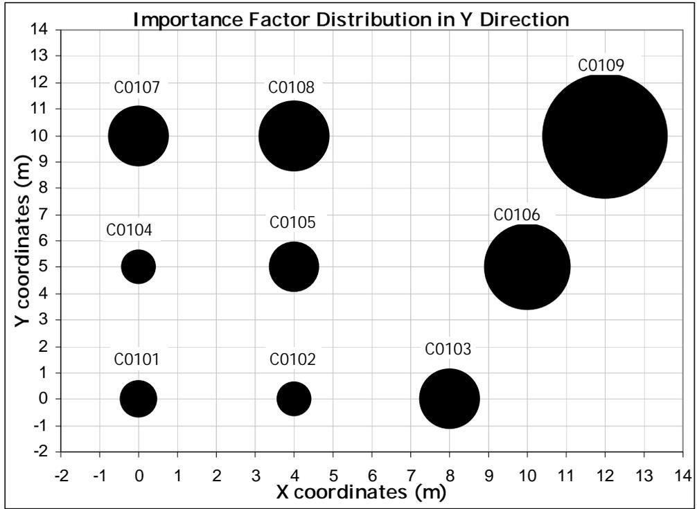
Figure 5.40 Importance Factor Distribution in Y Direction for Building 1
