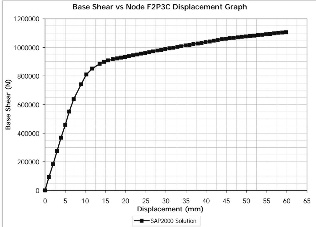
**Figure B.5** SAP2000 Pushover analysis result conducted in X Direction
