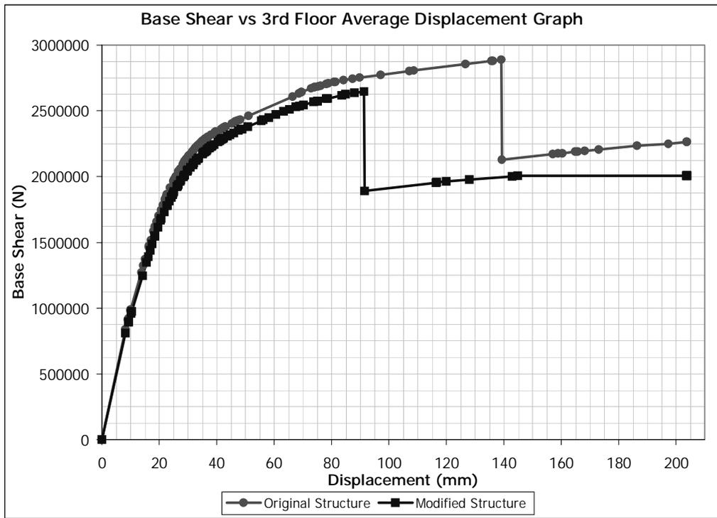
Figure 5.113 (+) X Direction Pushover for Building 4. Removed Member: SW0103
