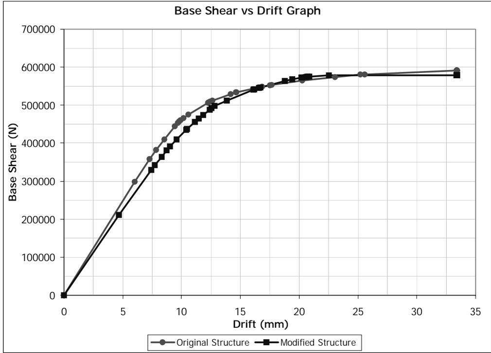
Figure 5.20 (+) X Direction Pushover for Building 1. Removed Member: C0103
