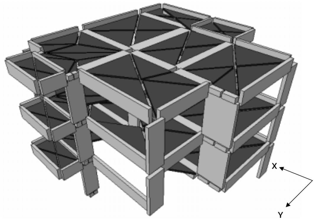
Figure A.10 State of Building at Drift of 105 mm
