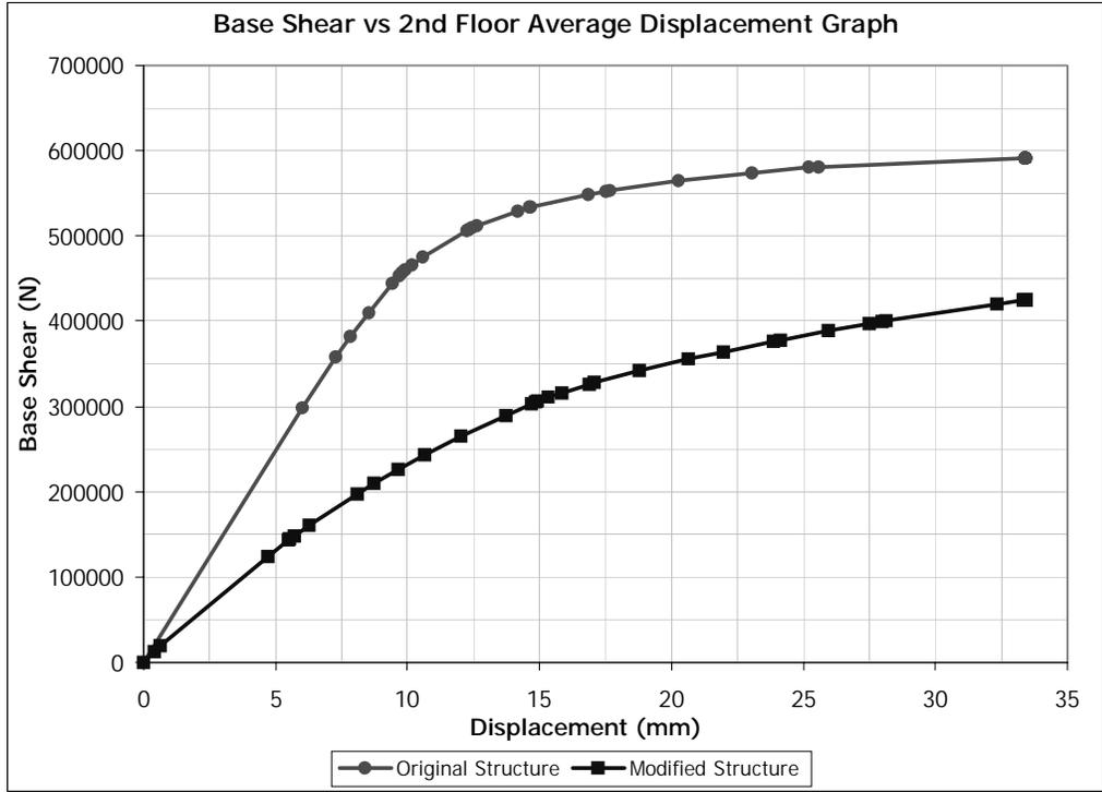
Figure 5.26 (+) X Direction Pushover for Building 1. Removed Member: C0109
