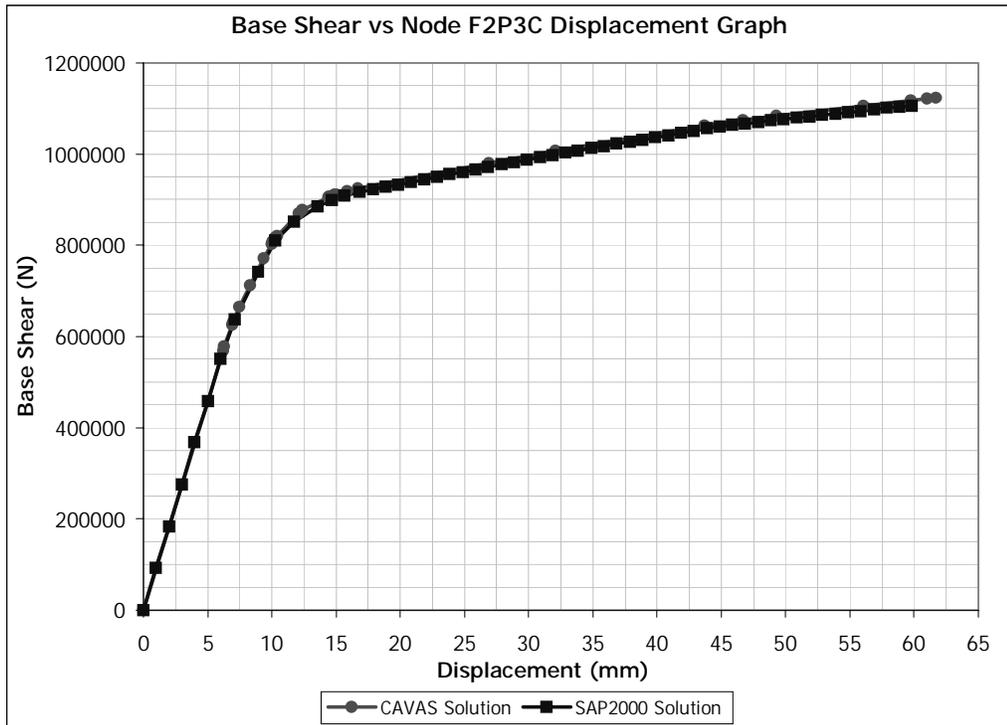
**Figure B.6** Pushover Curves obtained by CAVAS and SAP2000 in X Direction
