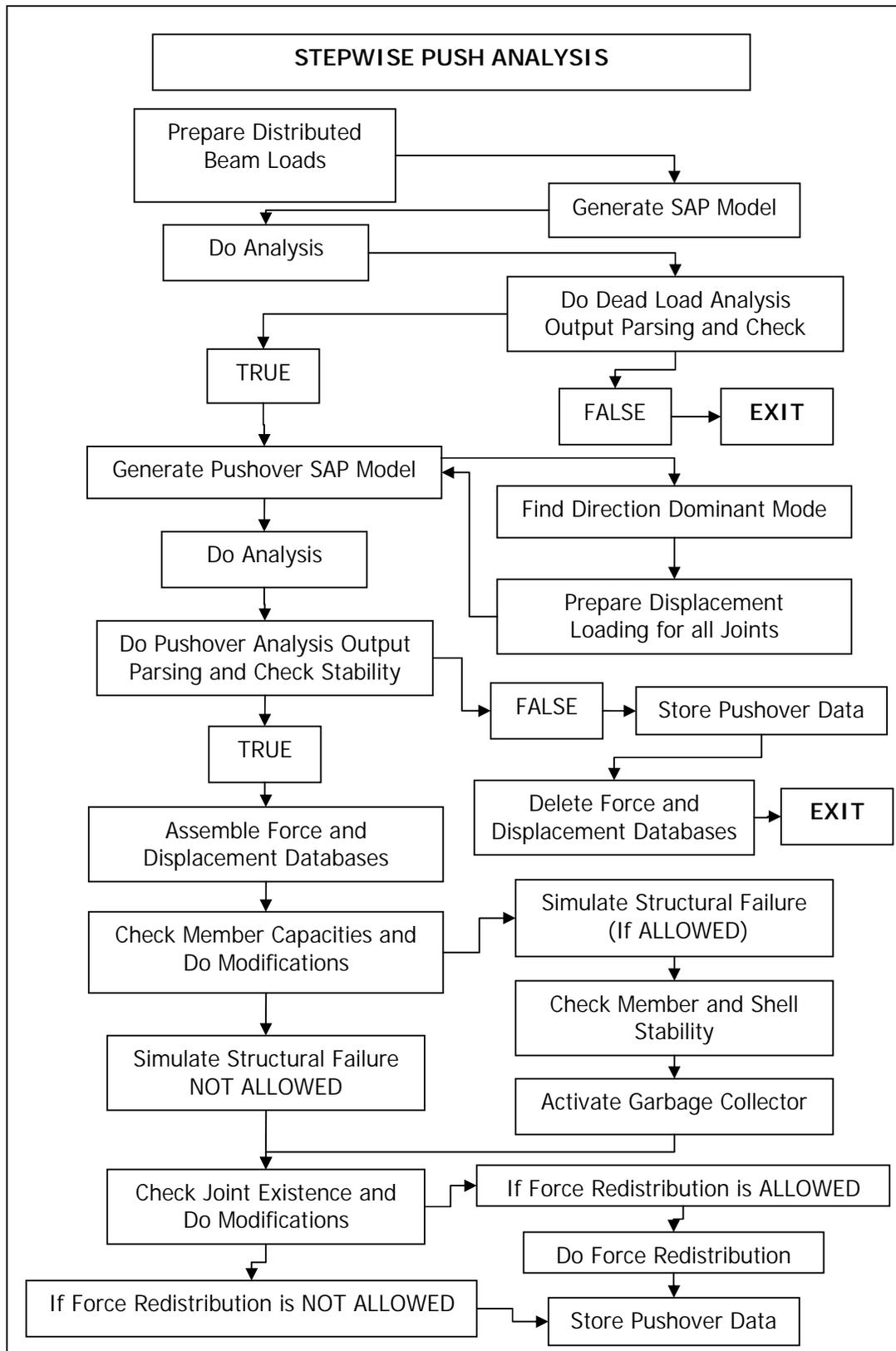
Figure 2.4 "Stepwise Push Analysis" Module Program Layout
