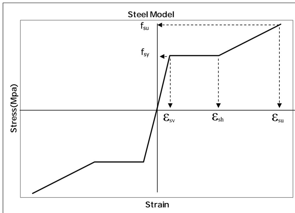
Figure 3.5 Tri-linear Steel Model
