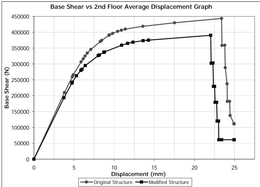
Figure 5.45 (+) X Direction Pushover for Building 2. Removed Member: C0104
