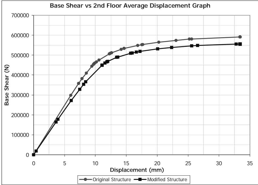
Figure 5.22 (+) X Direction Pushover for Building 1. Removed Member: C0105
