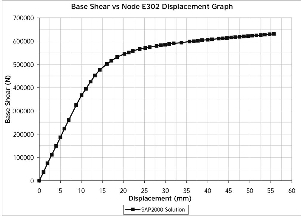
Figure 5.12 SAP2000 Pushover analysis result conducted in X Direction
