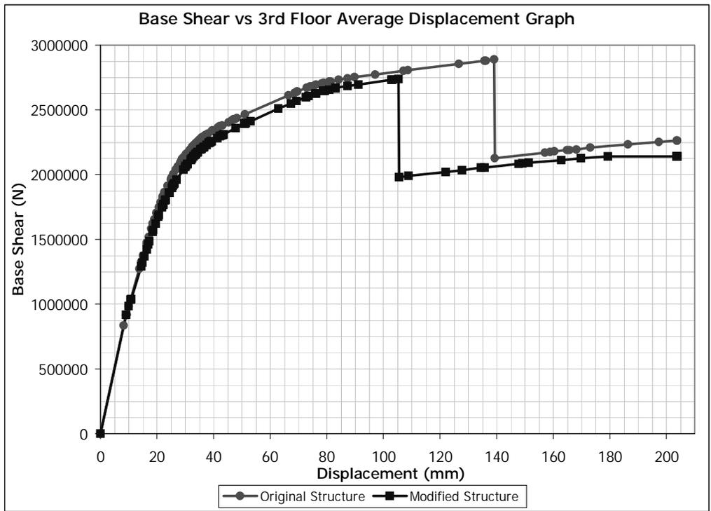
Figure 5.103 (+) X Direction Pushover for Building 4. Removed Member: C0103
