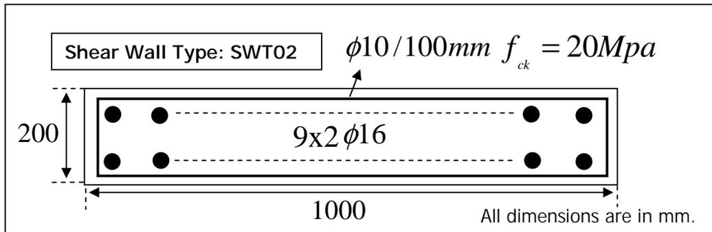
Figure 5.93 Details of Shear Wall Type SWT02
