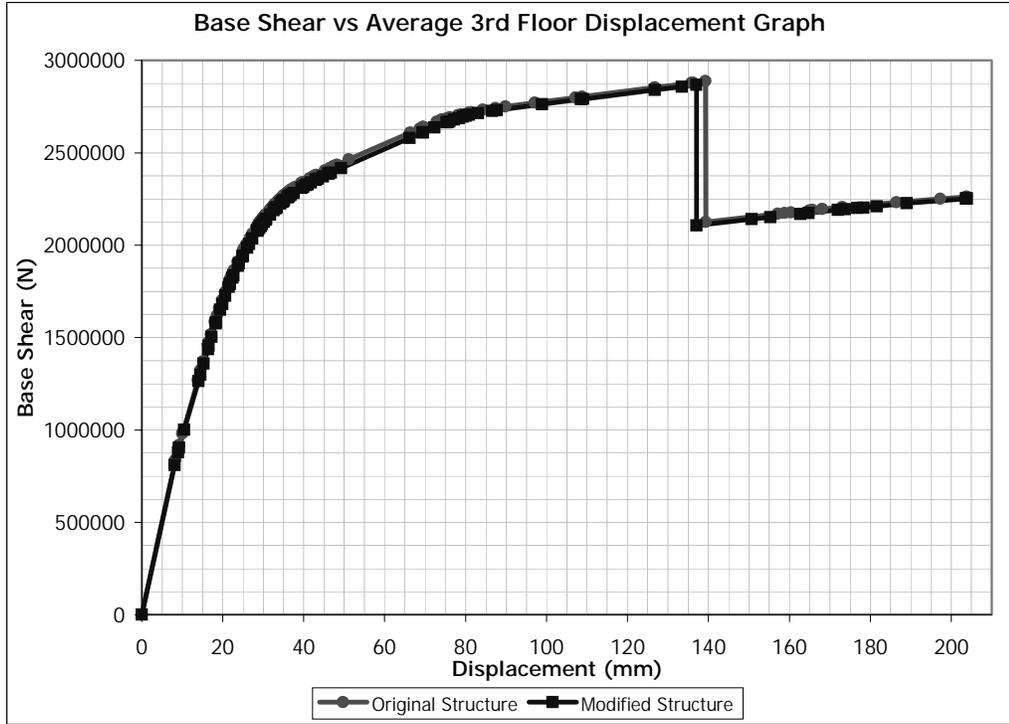
Figure 5.131 (+) X Direction Pushover for Building 4. Removed Member: B0116
