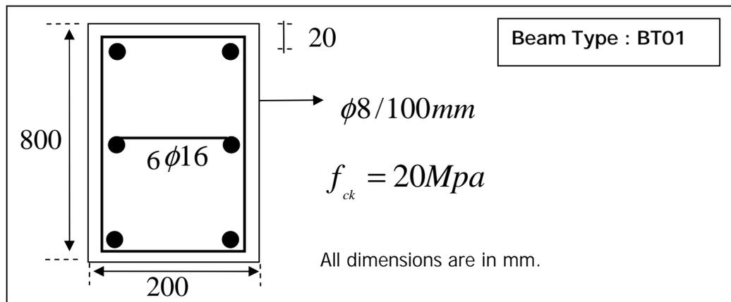
Figure 5.84 Details of Beam Type BT01
