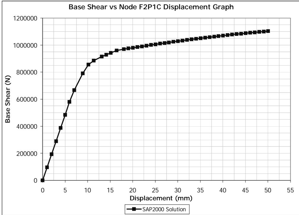
**Figure B.8** SAP2000 Pushover analysis result conducted in Y Direction
