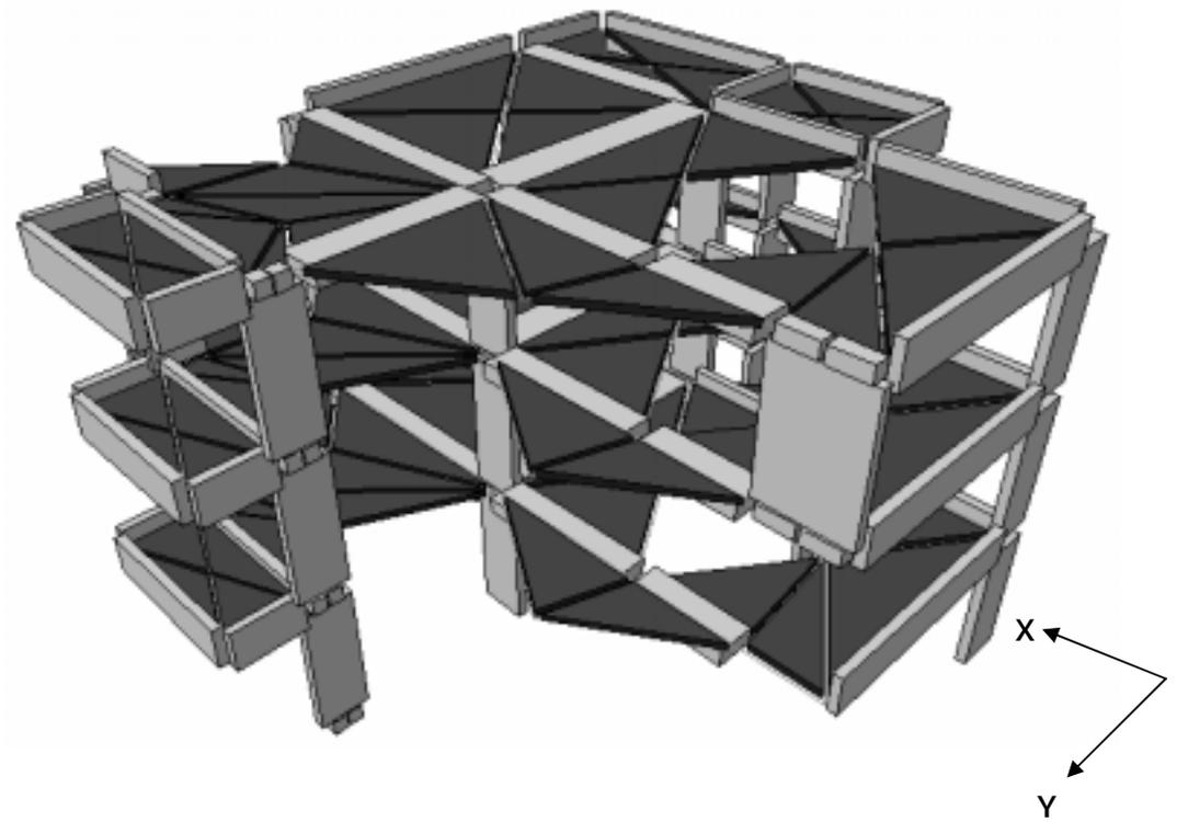
**Figure A.15** State of Building When Mechanism is formed at Drift of 141 mm
