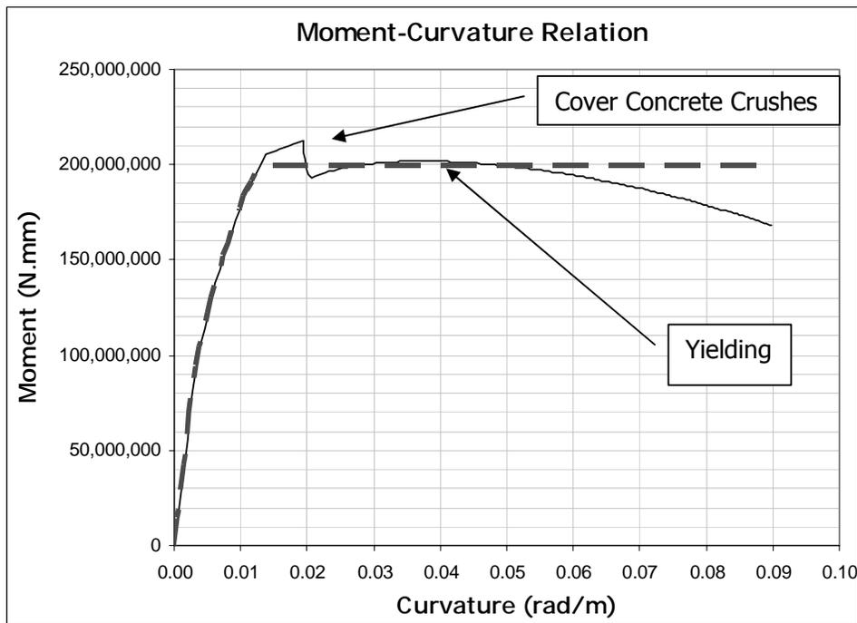
Figure 3.10 Modified Moment Curvature Relation
