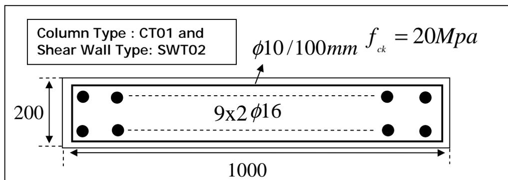
Figure A.2 Details of Column Type CT01 & Shear Wall Type SWT02
