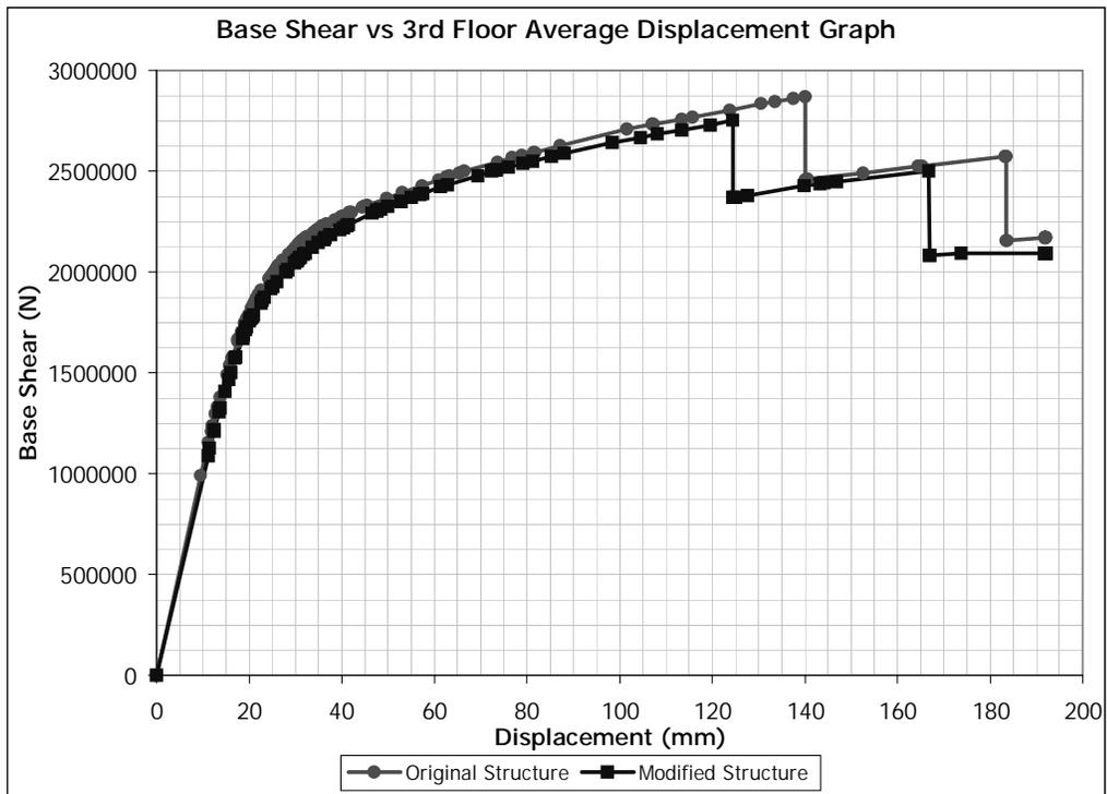
Figure 5.120 (+) Y Direction Pushover for Building 4. Removed Member: C0107
