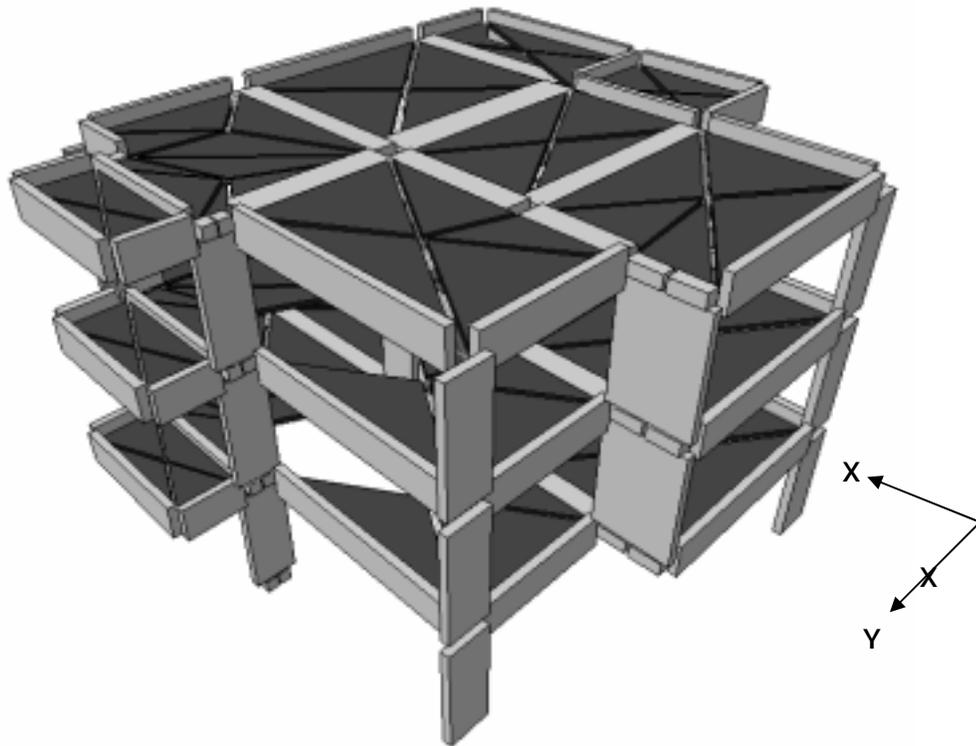
**Figure A.8** State of Building at Drift of 90 mm
