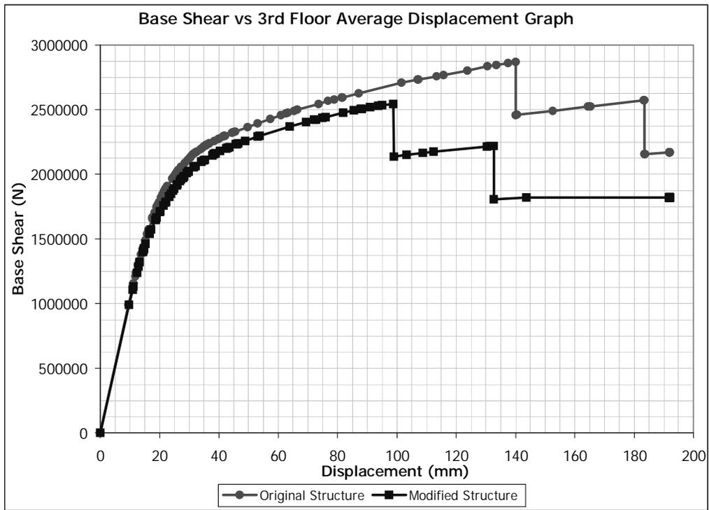
Figure 5.117 (+) Y Direction Pushover for Building 4. Removed Member: C0104
