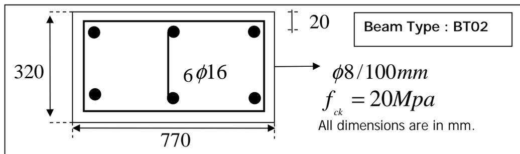
Figure 5.85 Details of Beam Type BT02
