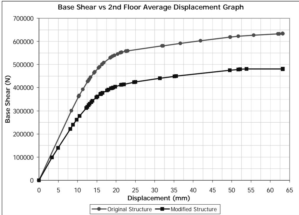
Figure 5.35 (+) Y Direction Pushover for Building 1. Removed Member: C0109
