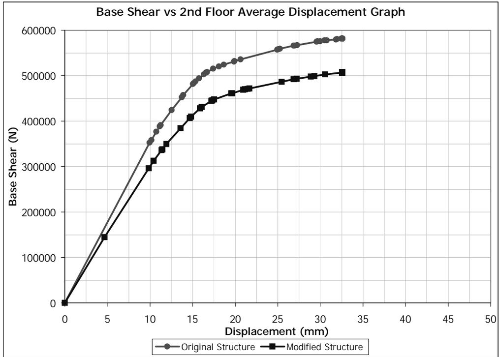
Figure 5.77 (-) Y Direction Pushover for Building 3. Removed Member: C0105
