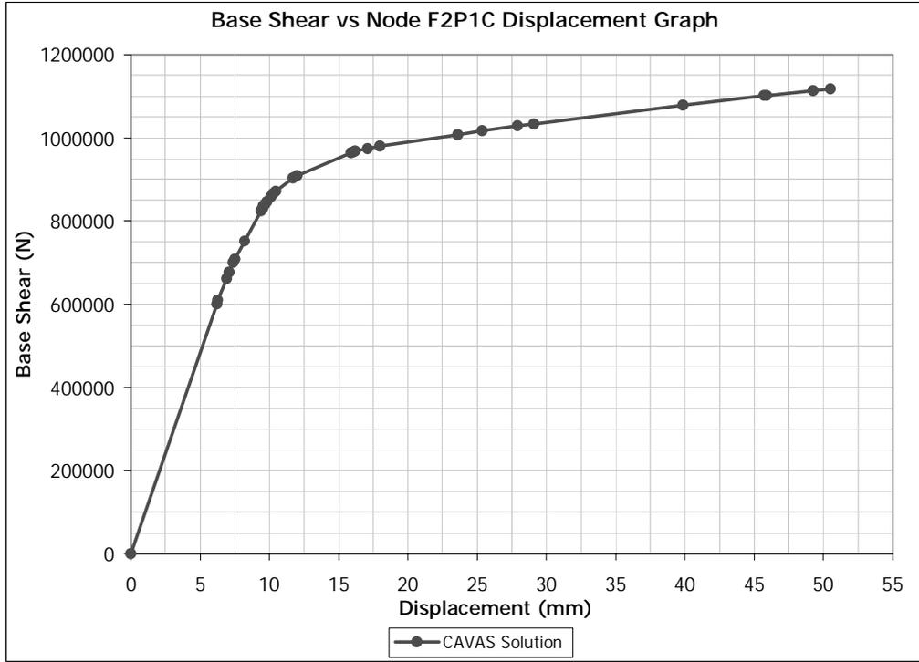
**Figure B.7** CAVAS Pushover analysis result conducted in Y Direction
