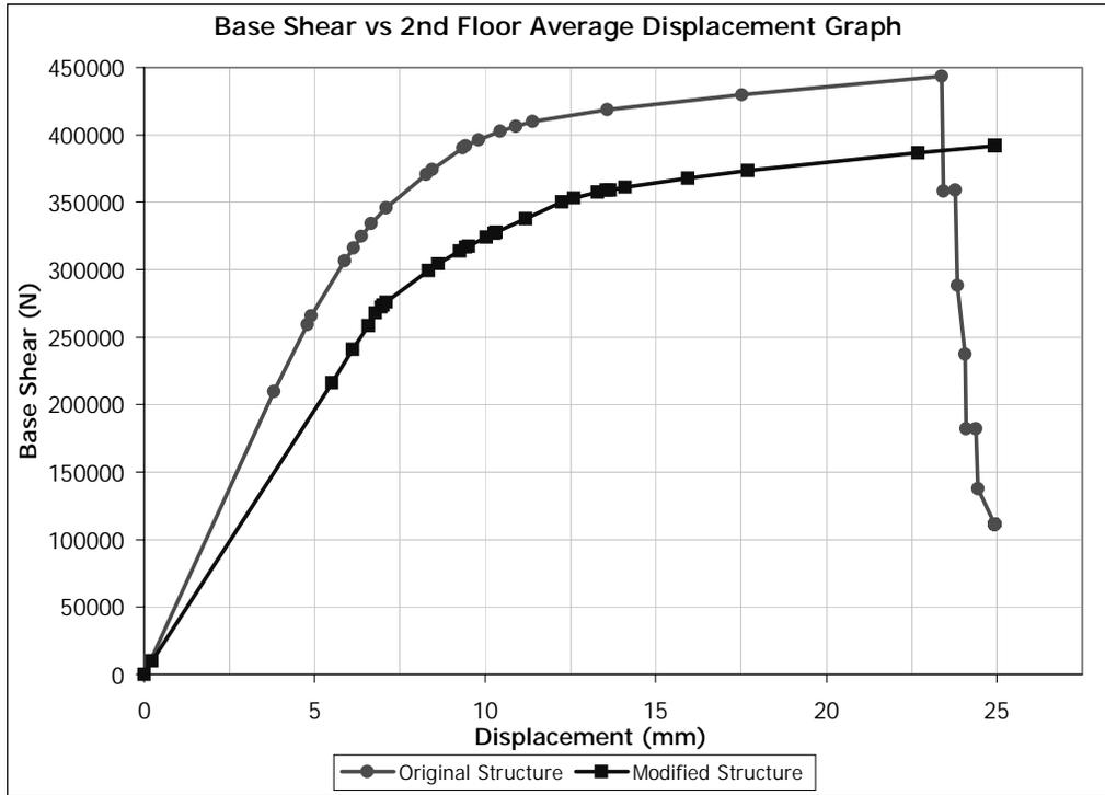
Figure 5.47 (+) X Direction Pushover for Building 2. Removed Member: C0106
