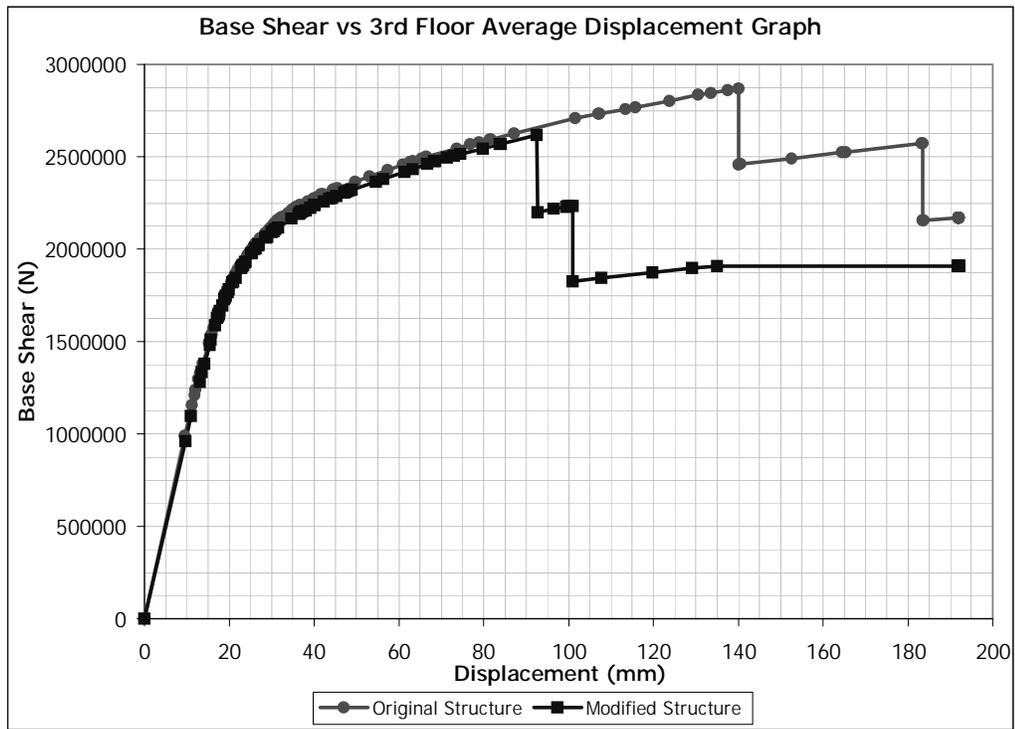
Figure 5.123 (+) Y Direction Pushover for Building 4. Removed Member: C0110
