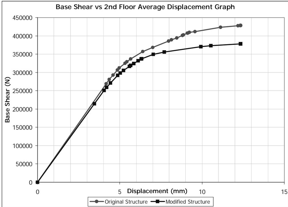
Figure 5.69 (+) X Direction Pushover for Building 3. Removed Member: C0105
