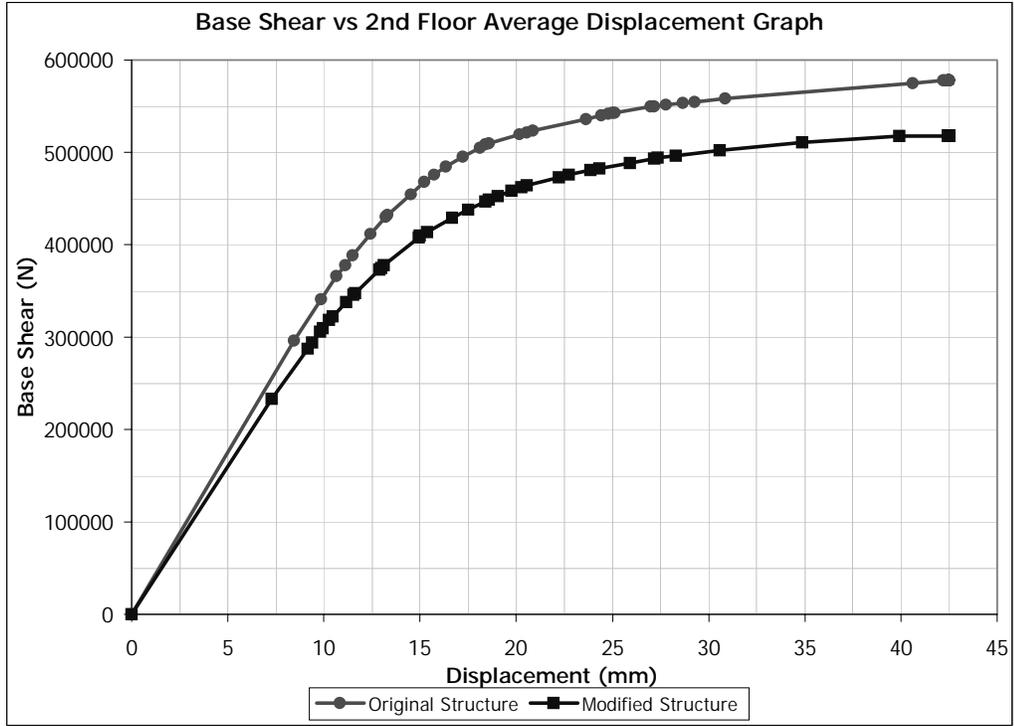
Figure 5.56 (+) Y Direction Pushover for Building 2. Removed Member: C0107
