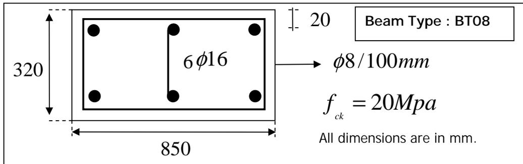
Figure 5.91 Details of Beam Type BT08
