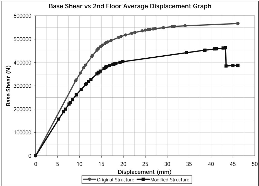
Figure 5.79 (+) Y Direction Pushover for Building 3. Removed Member: C0109
