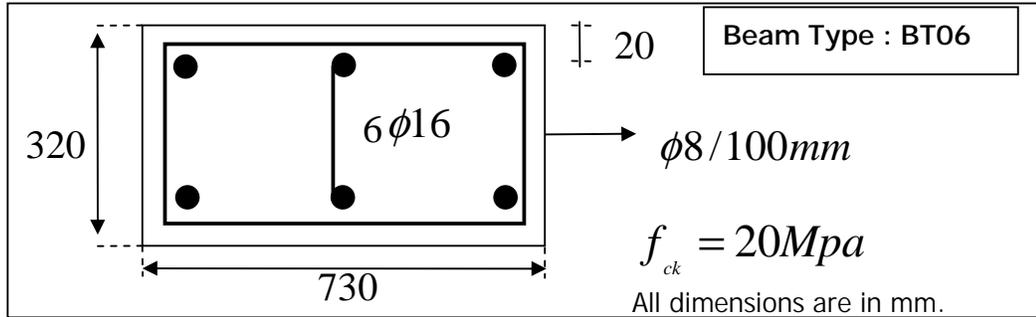
Figure 5.89 Details of Beam Type BT06
