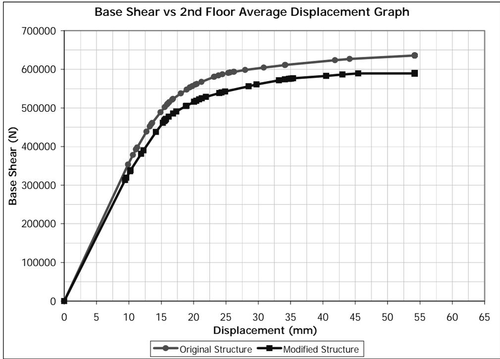
Figure 5.27 (-) Y Direction Pushover for Building 1. Removed Member : C0101
