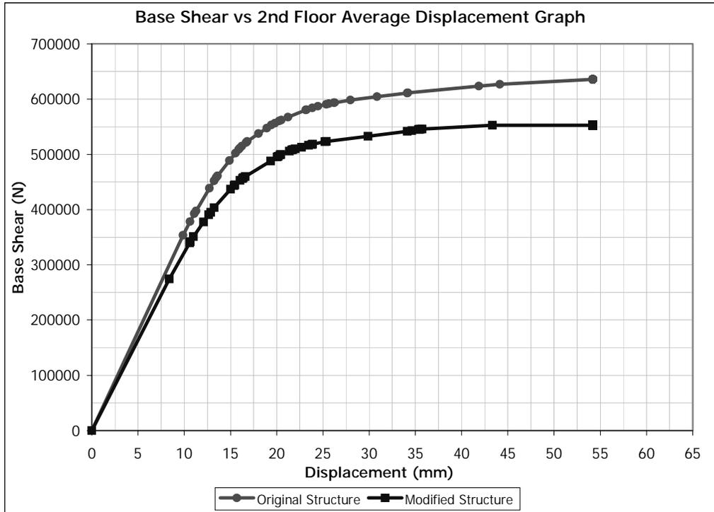
Figure 5.29 (-) Y Direction Pushover for Building 1. Removed Member : C0103
