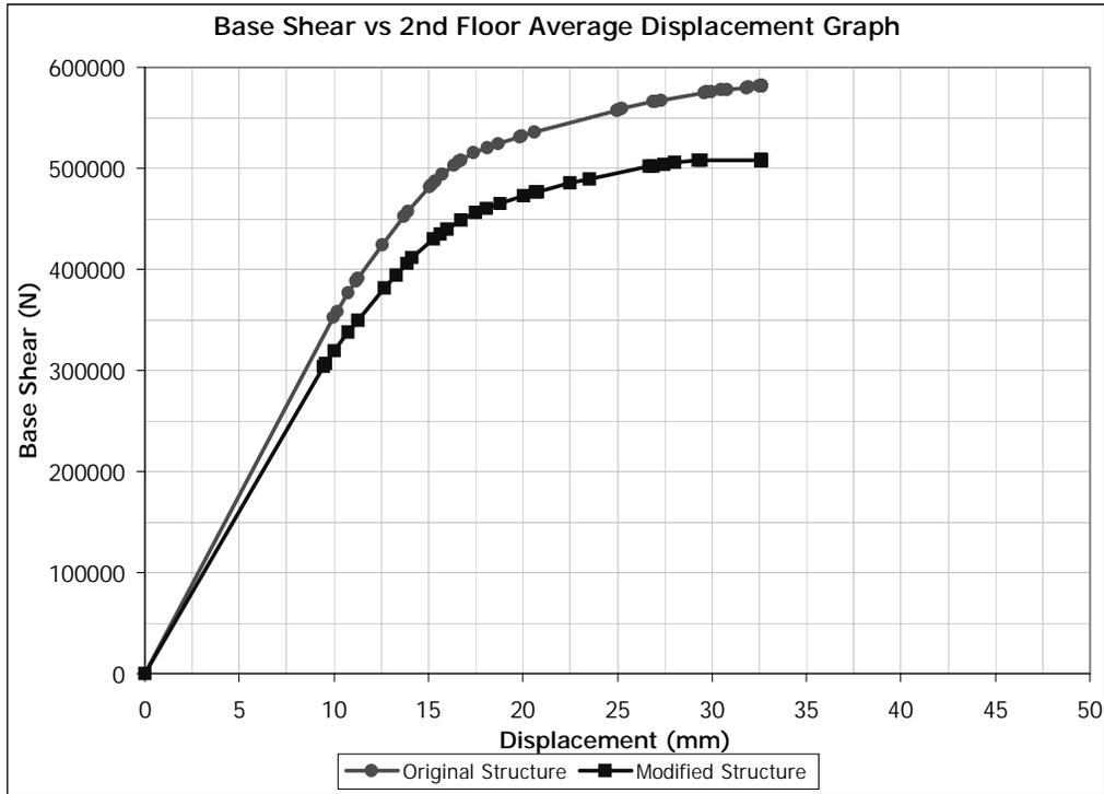
Figure 5.73 (-) Y Direction Pushover for Building 3. Removed Member: C0101
