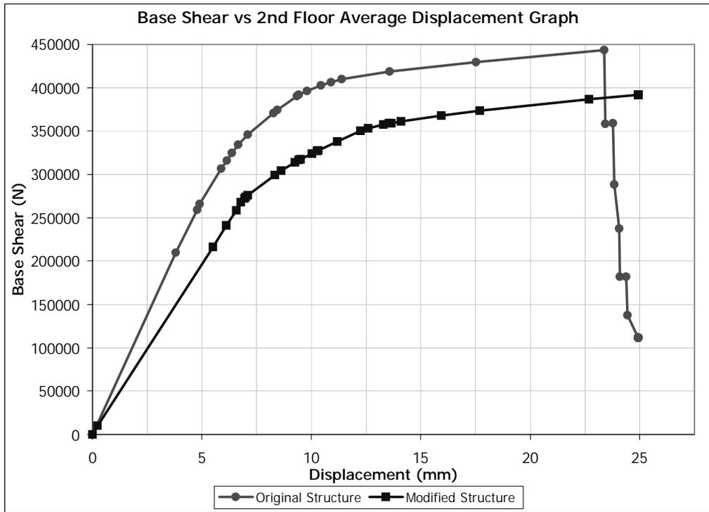
Figure 5.49 (-) X Direction Pushover for Building 2. Removed Member: C0108
