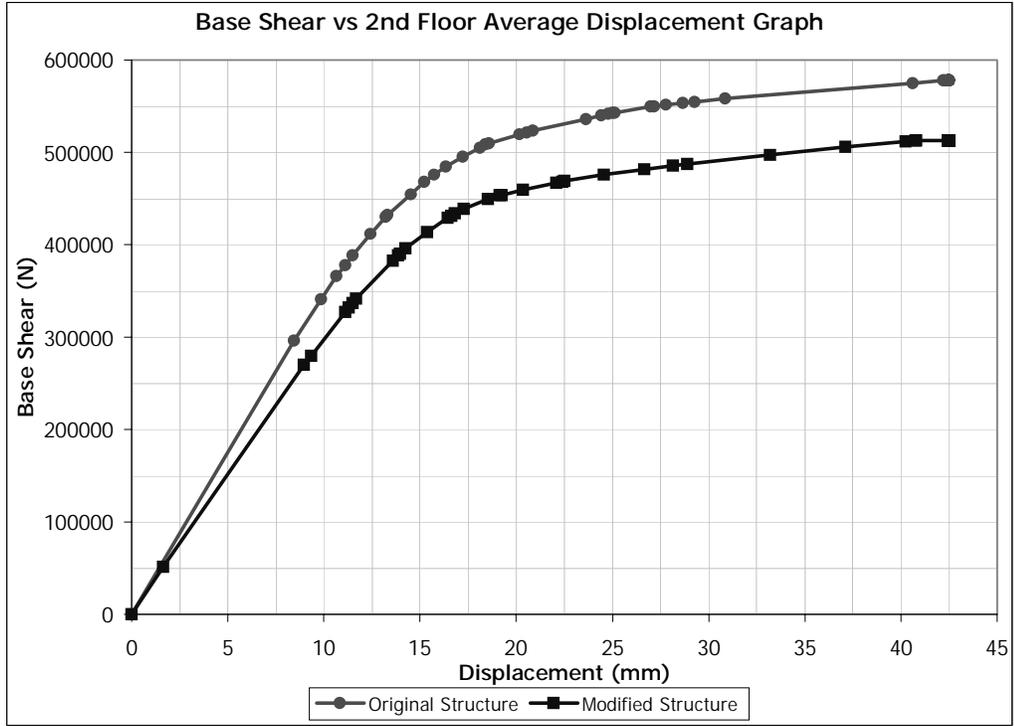
Figure 5.54 (+) Y Direction Pushover for Building 2. Removed Member: C0105
