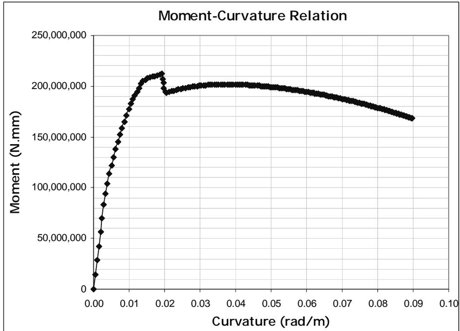
Figure 3.9 Moment Curvature Relation for Axial Load = 1000 kN (Compression)
