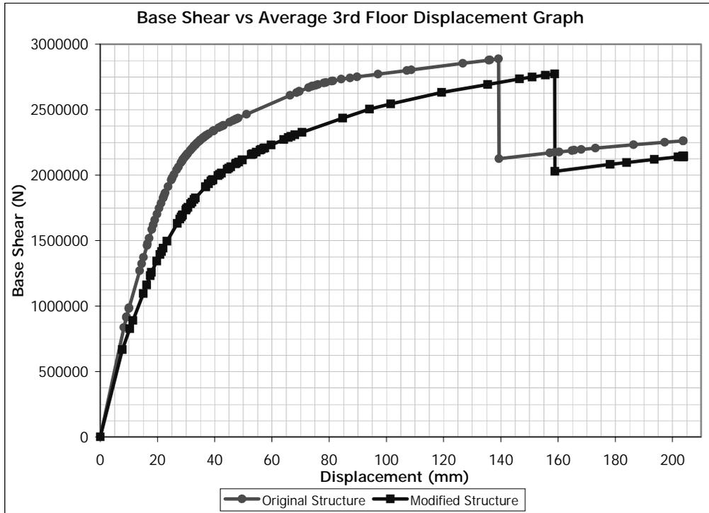
Figure 5.135 (+) X Direction Pushover for Building 4.All First Floor Beams are removed
