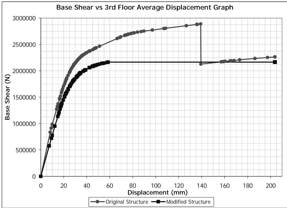
Figure 5.111 (+) X Direction Pushover for Building 4. Removed Member: SW0101
