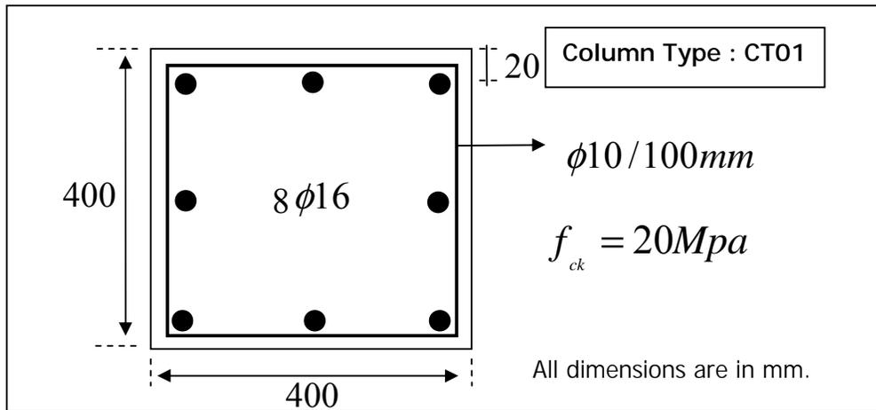
Figure 5.1 Details of Column Type CT01
