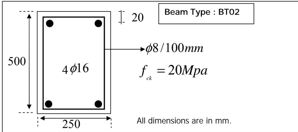
Figure 5.3 Details of Beam Type BT02
