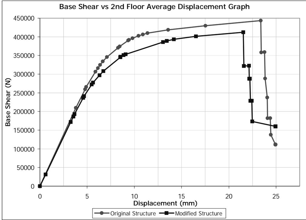
Figure 5.46 (+) X Direction Pushover for Building 2. Removed Member: C0105
