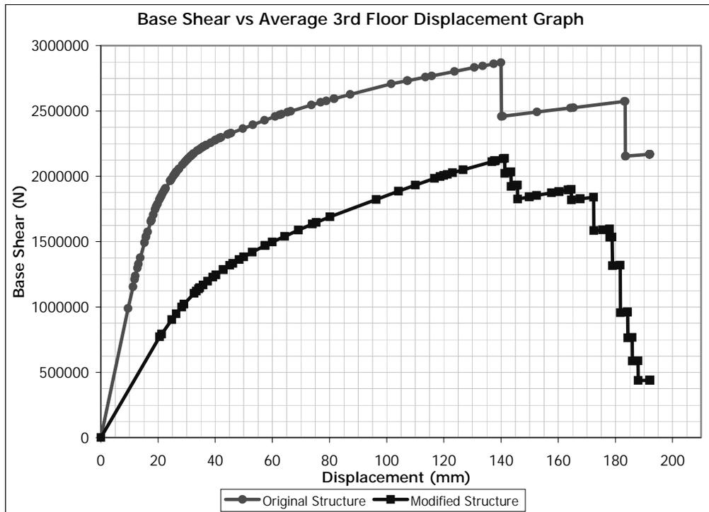
Figure 5.138 (+) Y Direction Pushover for Building 4. All Floor Beams are removed
