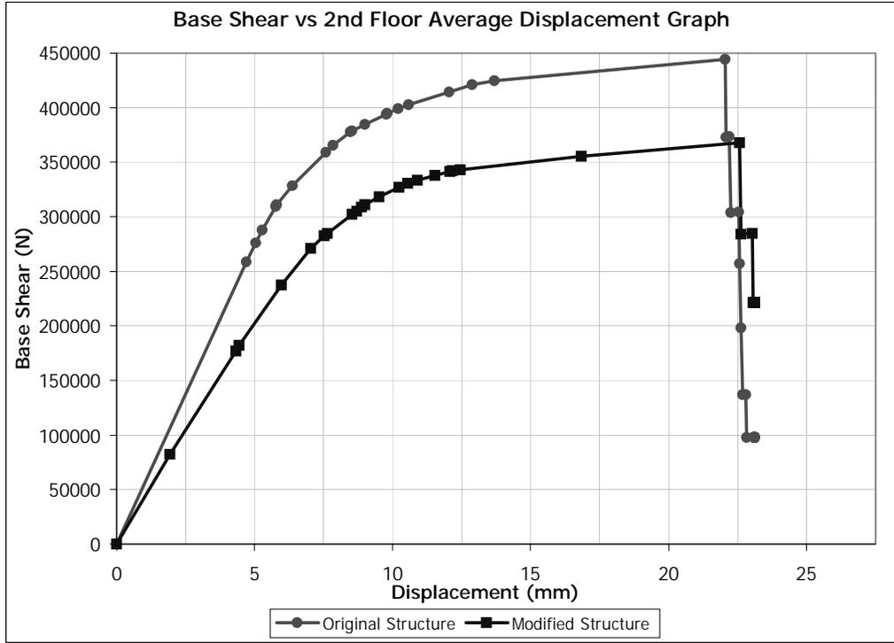
Figure 5.48 (+) X Direction Pushover for Building 2. Removed Member: C0107
