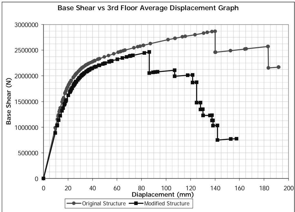
Figure 5.122 (+) Y Direction Pushover for Building 4. Removed Member: C0109
