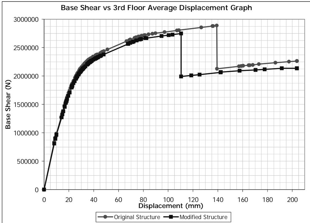
Figure 5.112 (+) X Direction Pushover for Building 4. Removed Member: SW0102
