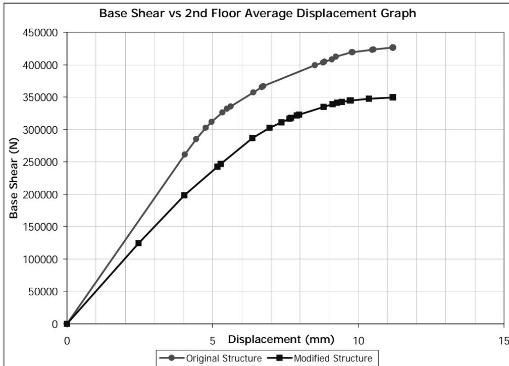
Figure 5.65 (-) X Direction Pushover for Building 3. Removed Member: C0101
