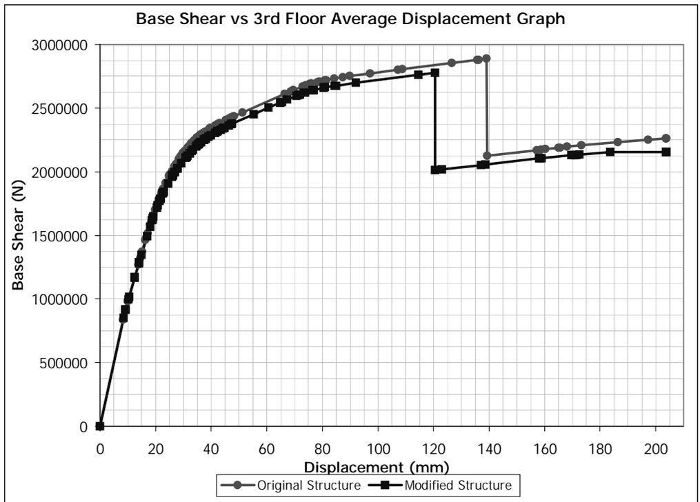
Figure 5.104 (+) X Direction Pushover for Building 4. Removed Member: C0104
