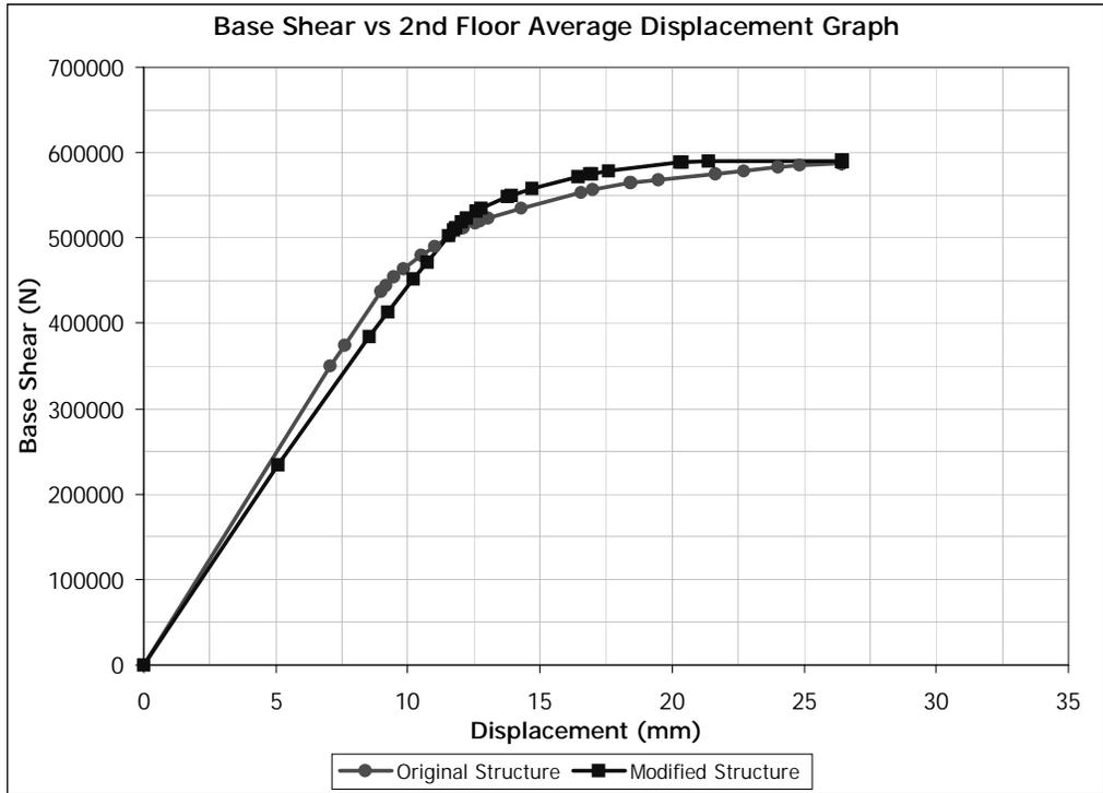
Figure 5.19 (-) X Direction Pushover for Building 1. Removed Member: C0102
