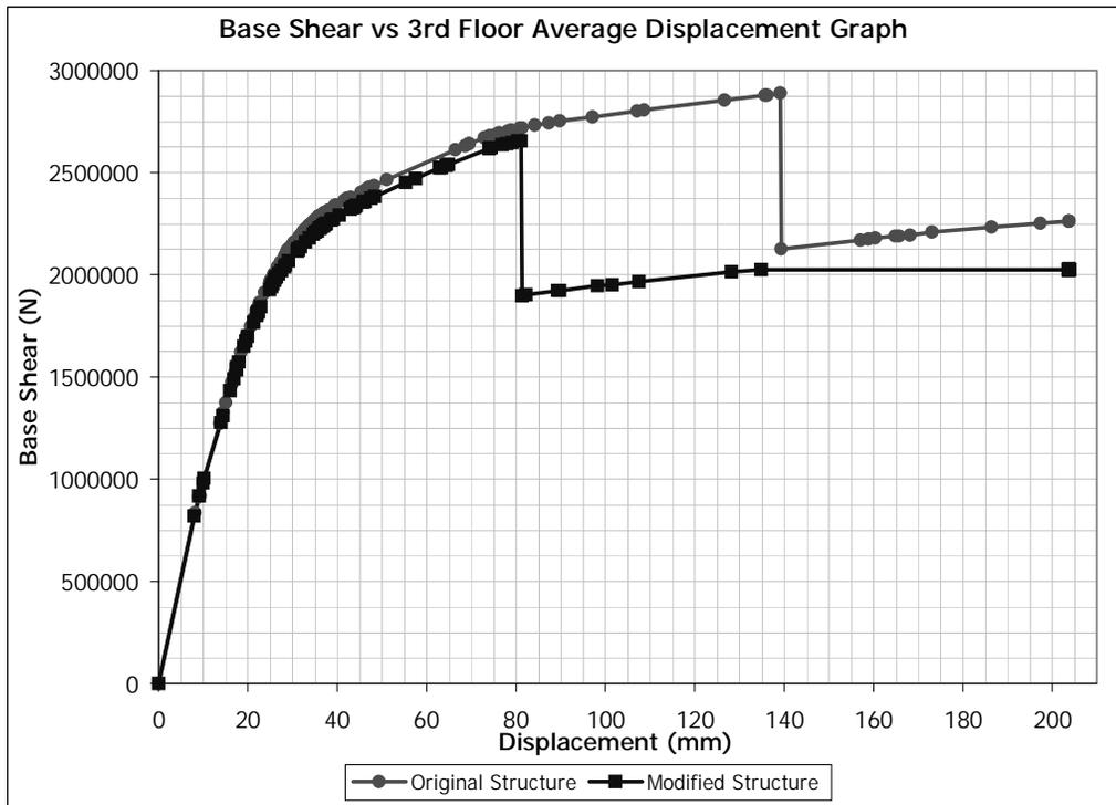
Figure 5.106 (+) X Direction Pushover for Building 4. Removed Member: C0106
