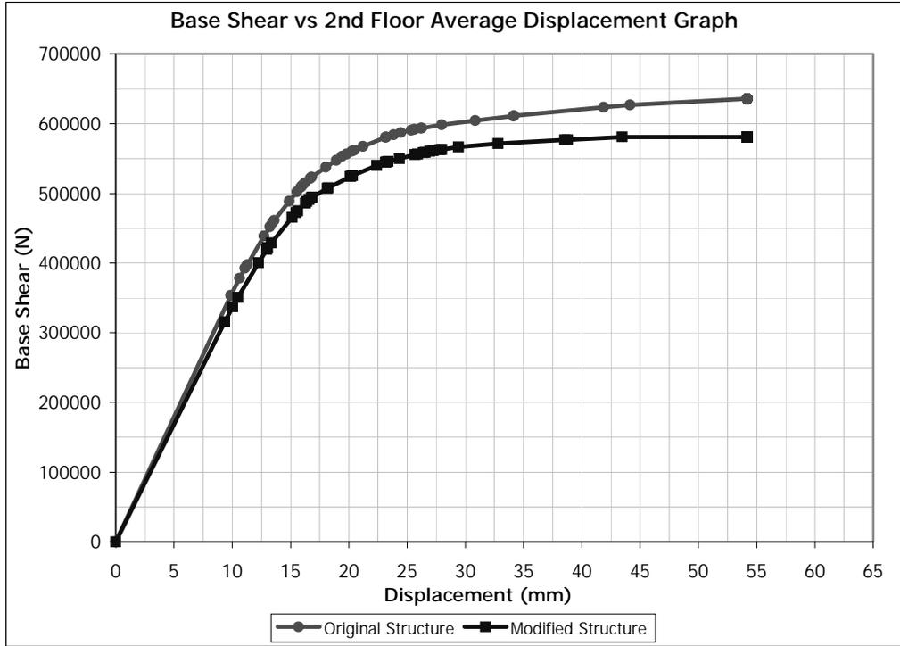
Figure 5.28 (-) Y Direction Pushover for Building 1. Removed Member : C0102
