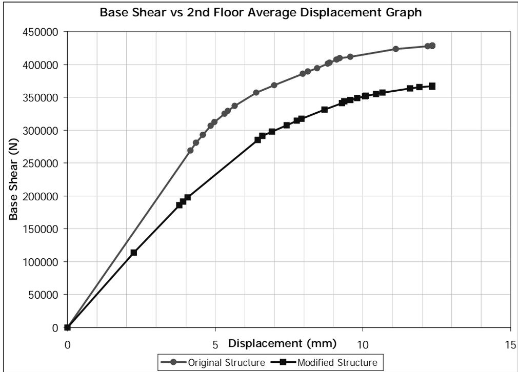
Figure 5.67 (+) X Direction Pushover for Building 3. Removed Member: C0103
