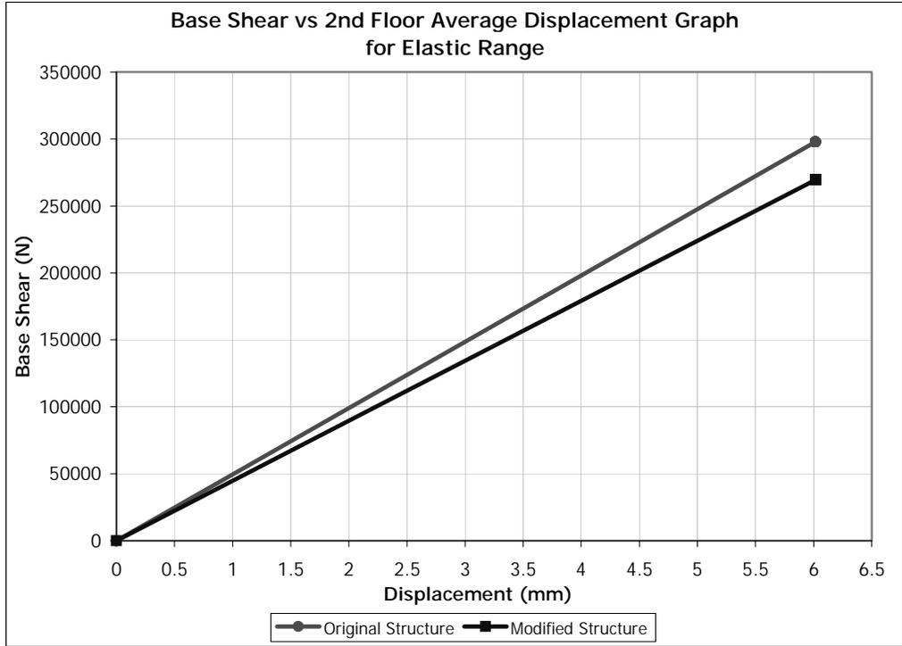
**Figure 5.36** (+) X Direction Pushover for Elastic Range. Removed Member: C0101
