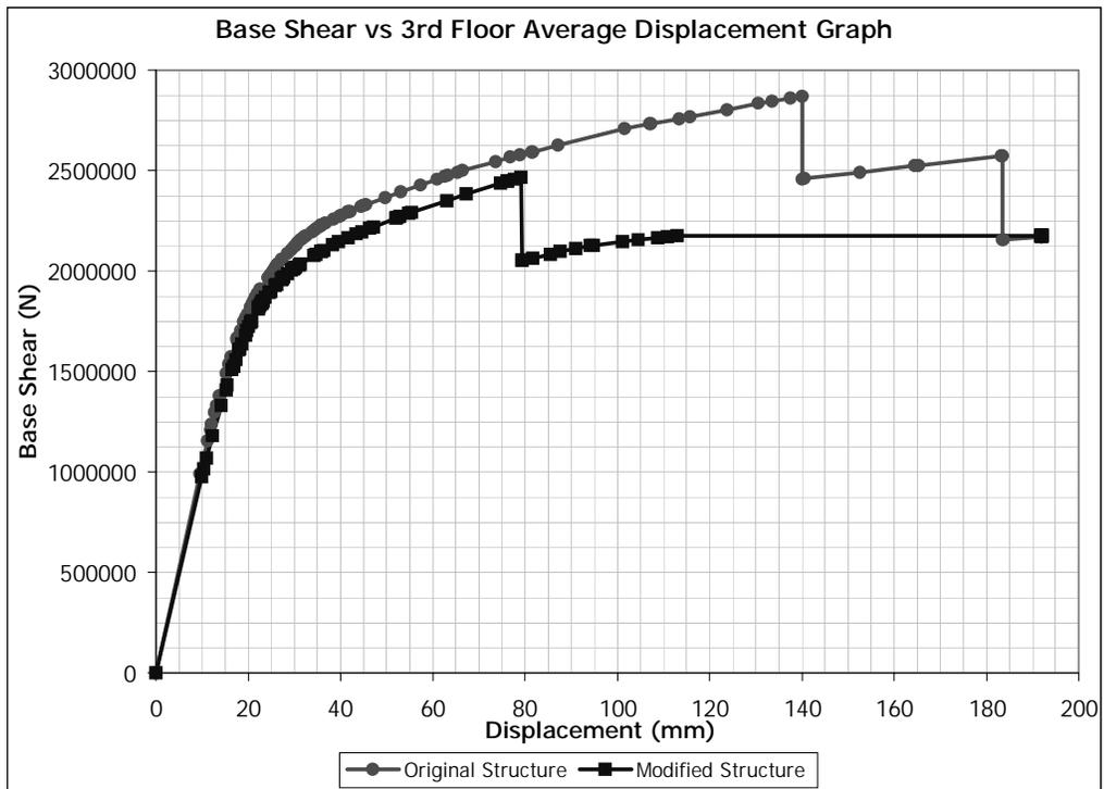
Figure 5.126 (+) Y Direction Pushover for Building 4. Removed Member: SW0103
