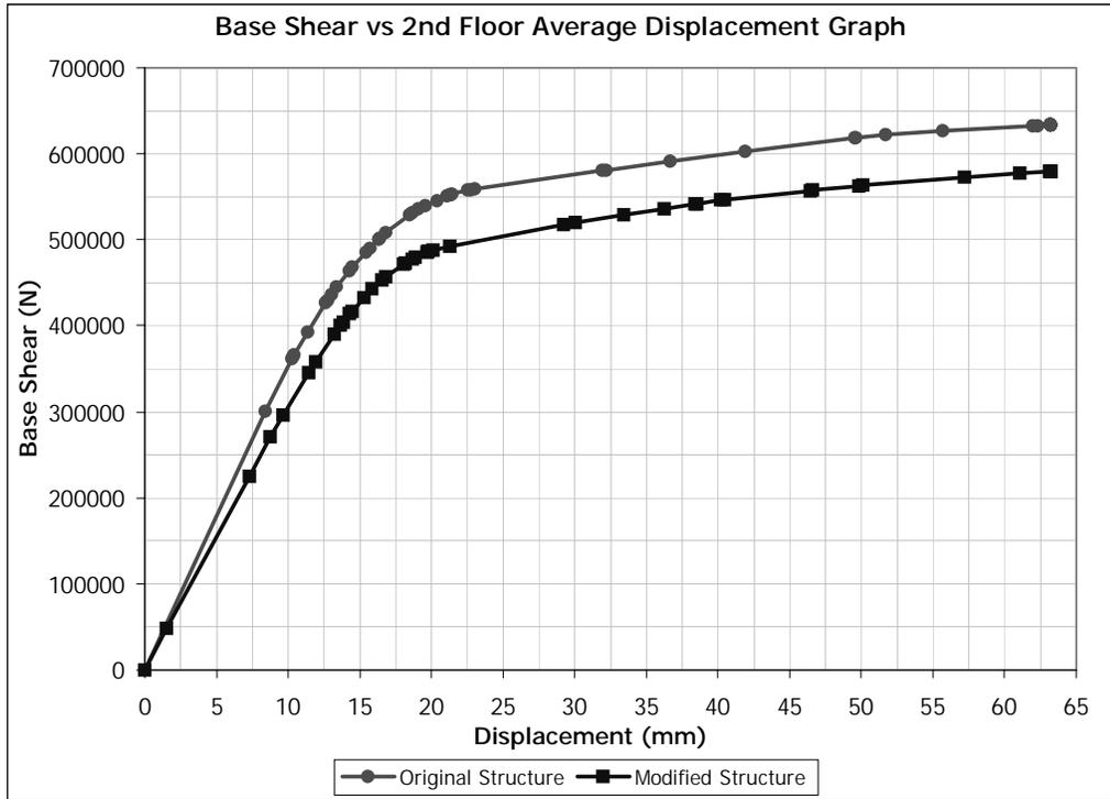
Figure 5.31 (+) Y Direction Pushover for Building 1. Removed Member : C0105
