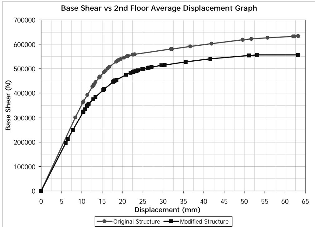
Figure 5.33 (+) Y Direction Pushover for Building 1. Removed Member: C0107
