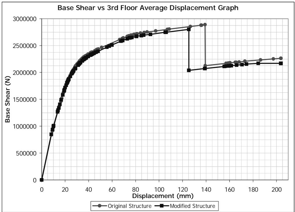
Figure 5.101 (+) X Direction Pushover for Building 4. Removed Member: C0101
