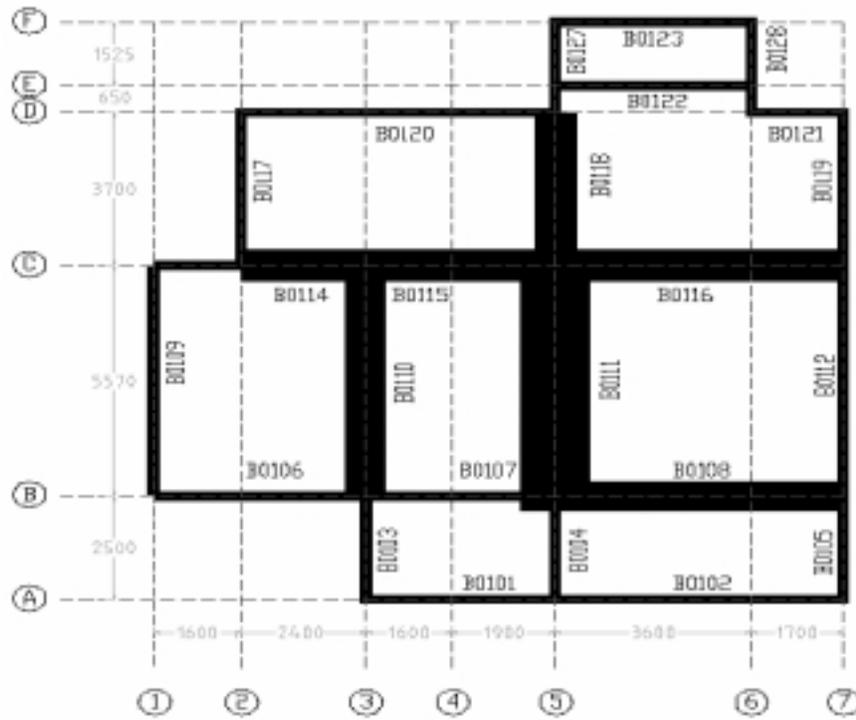
Figure A.4 First Floor Beam Layout of Building
