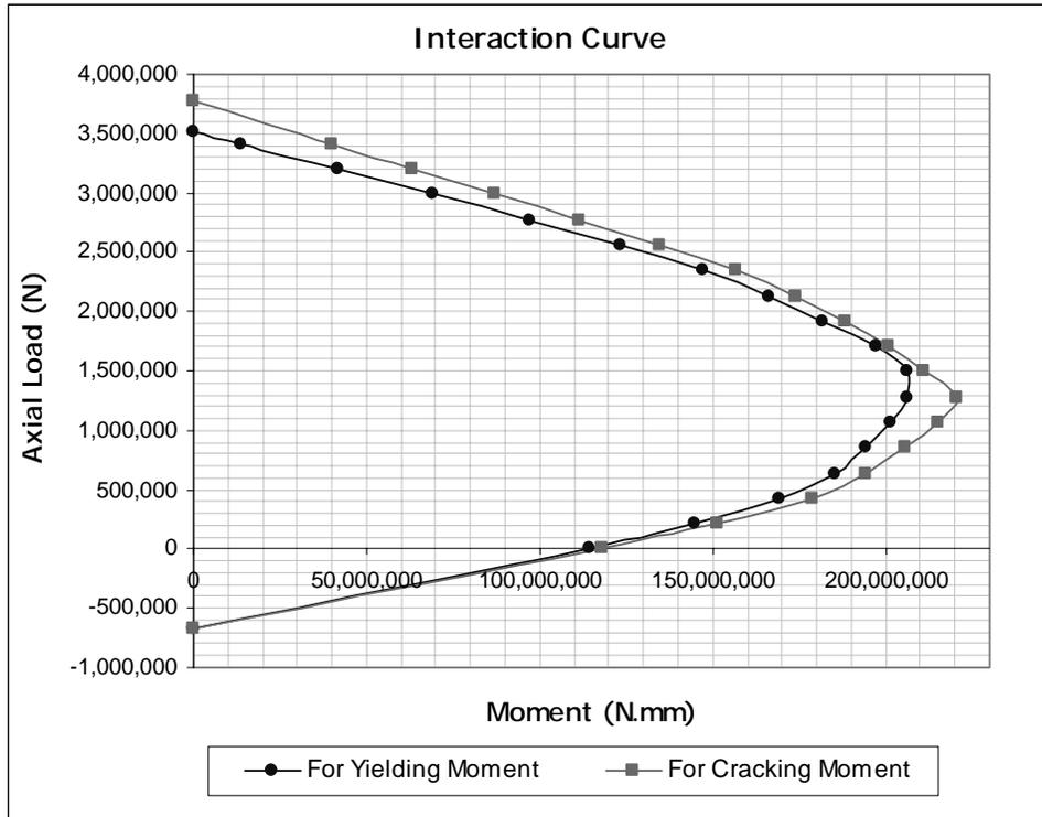
Figure 3.11 Interaction Relation for Cover Concrete Thickness = 30mm
