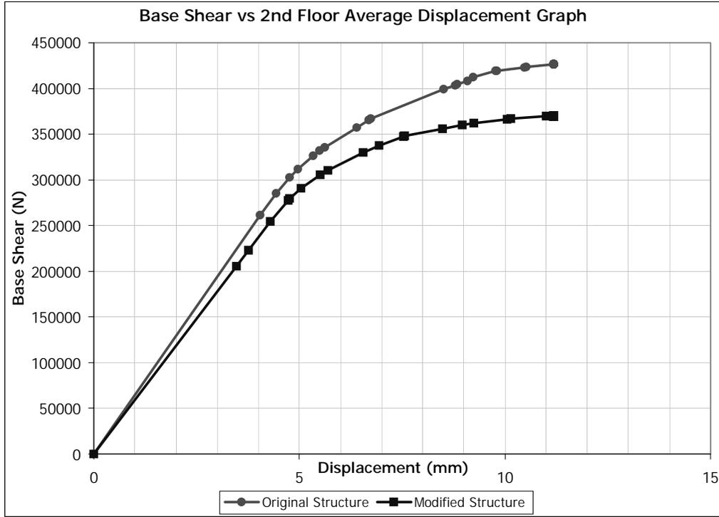
Figure 5.70 (-) X Direction Pushover for Building 3. Removed Member: C0106
