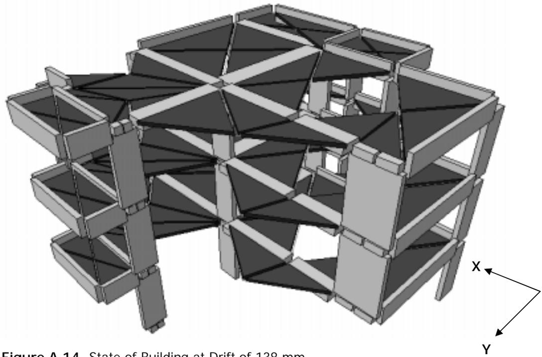
Figure A.14 State of Building at Drift of 138 mm
