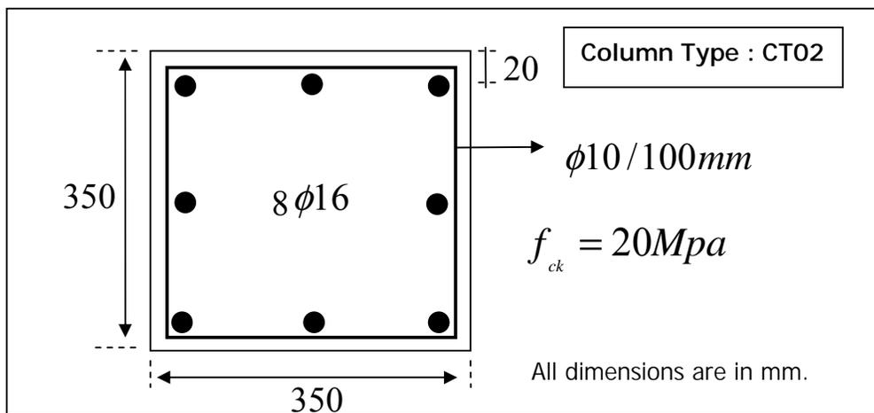
Figure 5.2 Details of Column Type CT02
