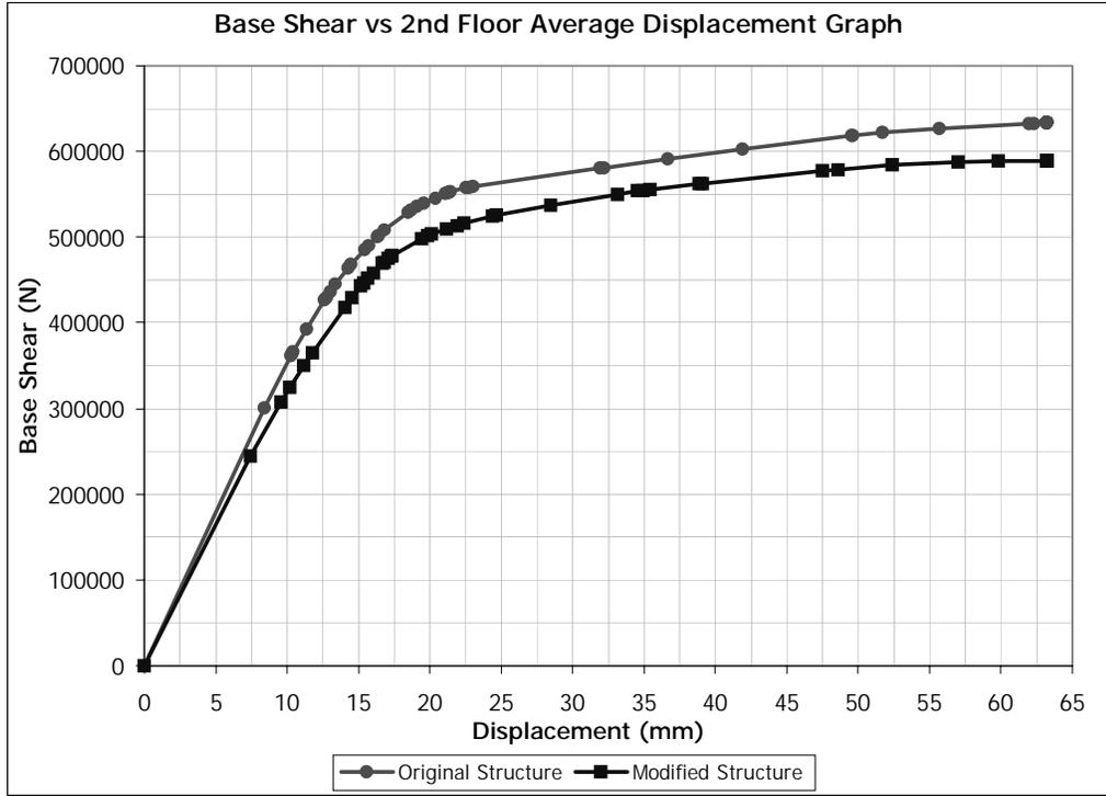
Figure 5.30 (+) Y Direction Pushover for Building 1. Removed Member : C0104
