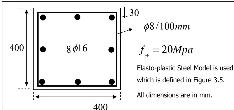
Figure 3.7 Example Cross-Section with Reinforcement Details
