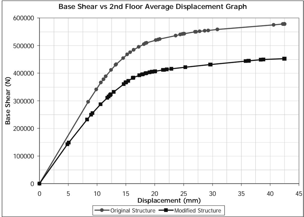
Figure 5.58 (+) Y Direction Pushover for Building 2. Removed Member: C0109
