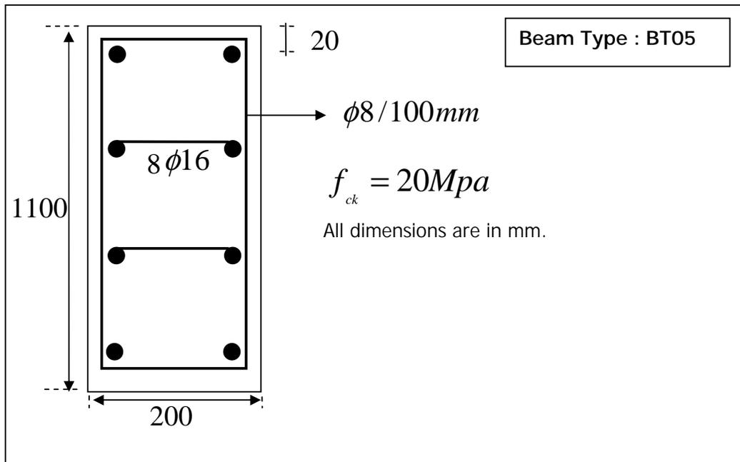
Figure 5.88 Details of Beam Type BT05
