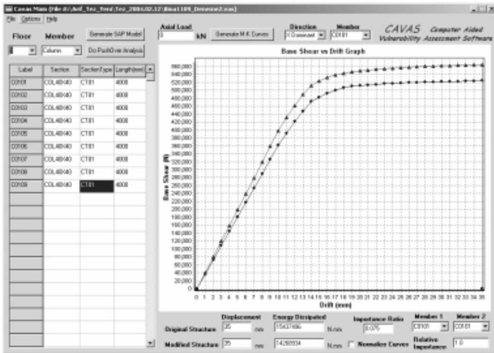
Figure 4.6 Example Pushover Results in X Dominant Direction for the Case Member C0101 is removed.
