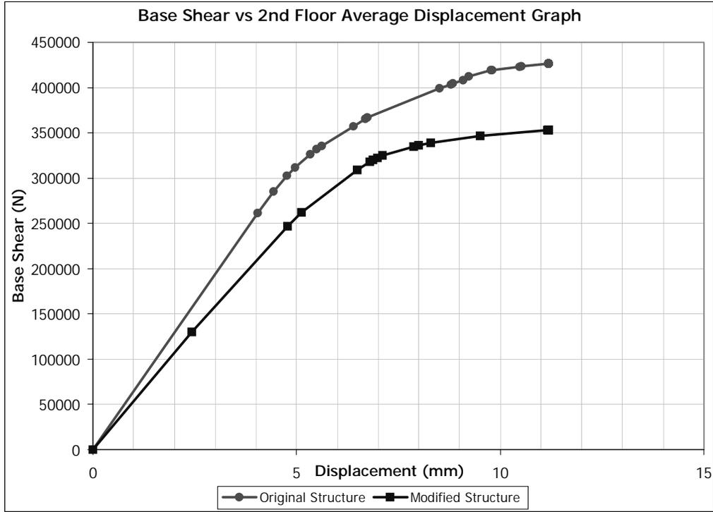
Figure 5.66 (-) X Direction Pushover for Building 3. Removed Member: C0102
