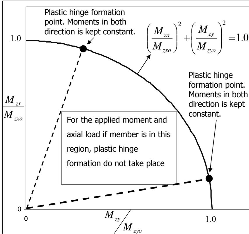
Figure 3.15 Behavior of Section under Axial load and Moment
