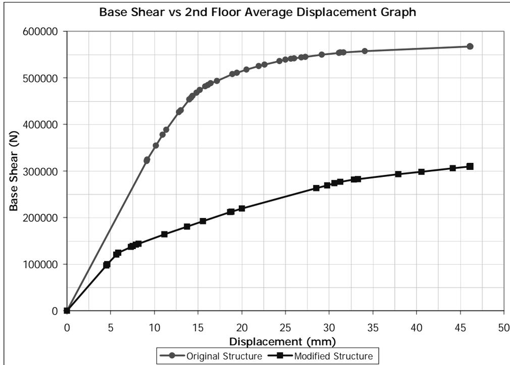
Figure 5.80 (+) Y Direction Pushover for Building 3. Removed Member:SW0102
