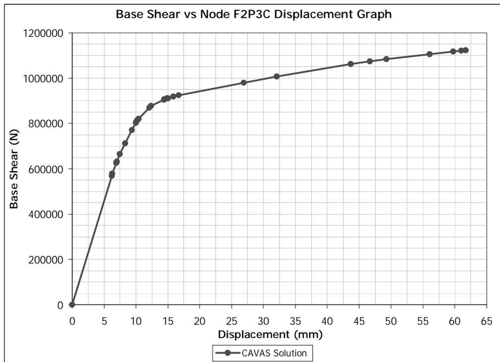
Figure B.4 CAVAS Pushover analysis result conducted in X Direction
