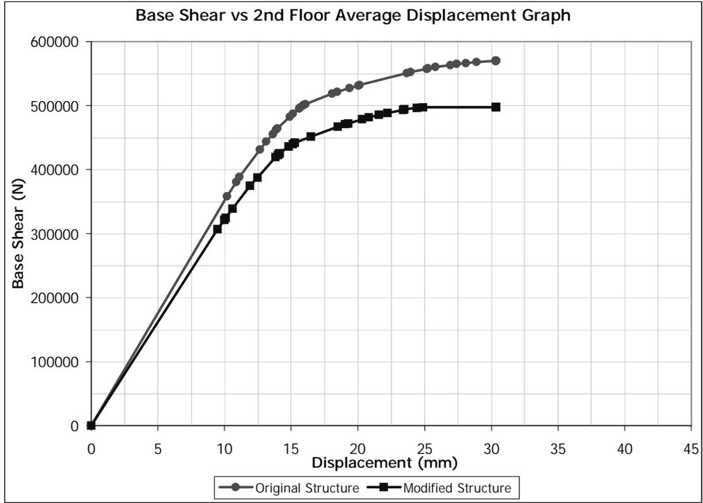
Figure 5.52 (-) Y Direction Pushover for Building 2. Removed Member: C0103
