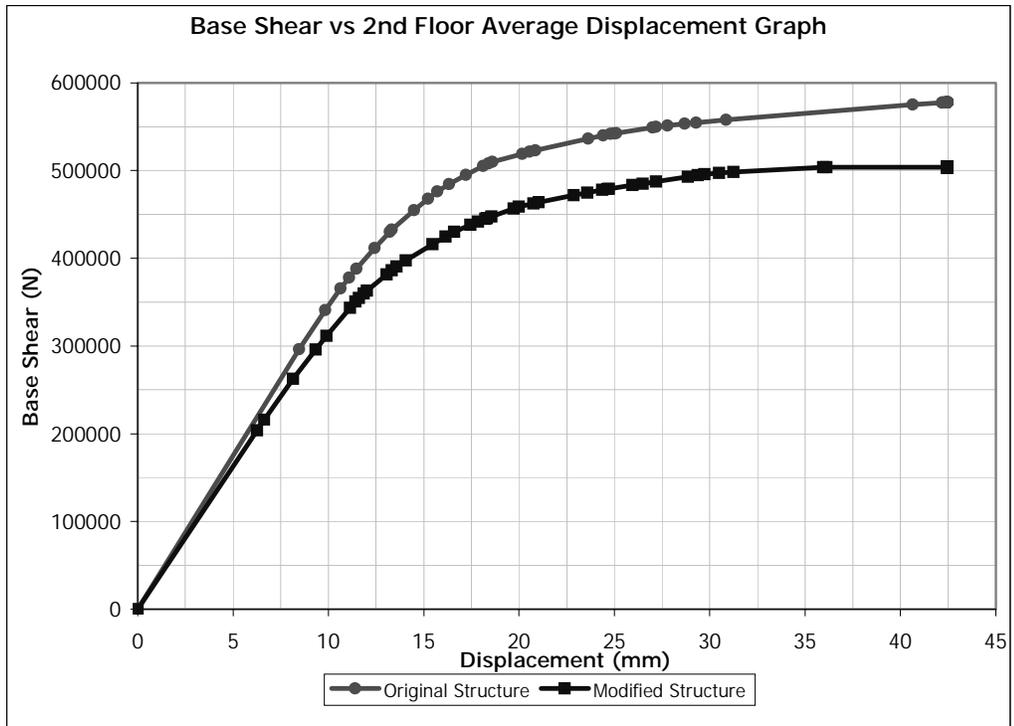
Figure 5.57 (+) Y Direction Pushover for Building 2. Removed Member: C0108
