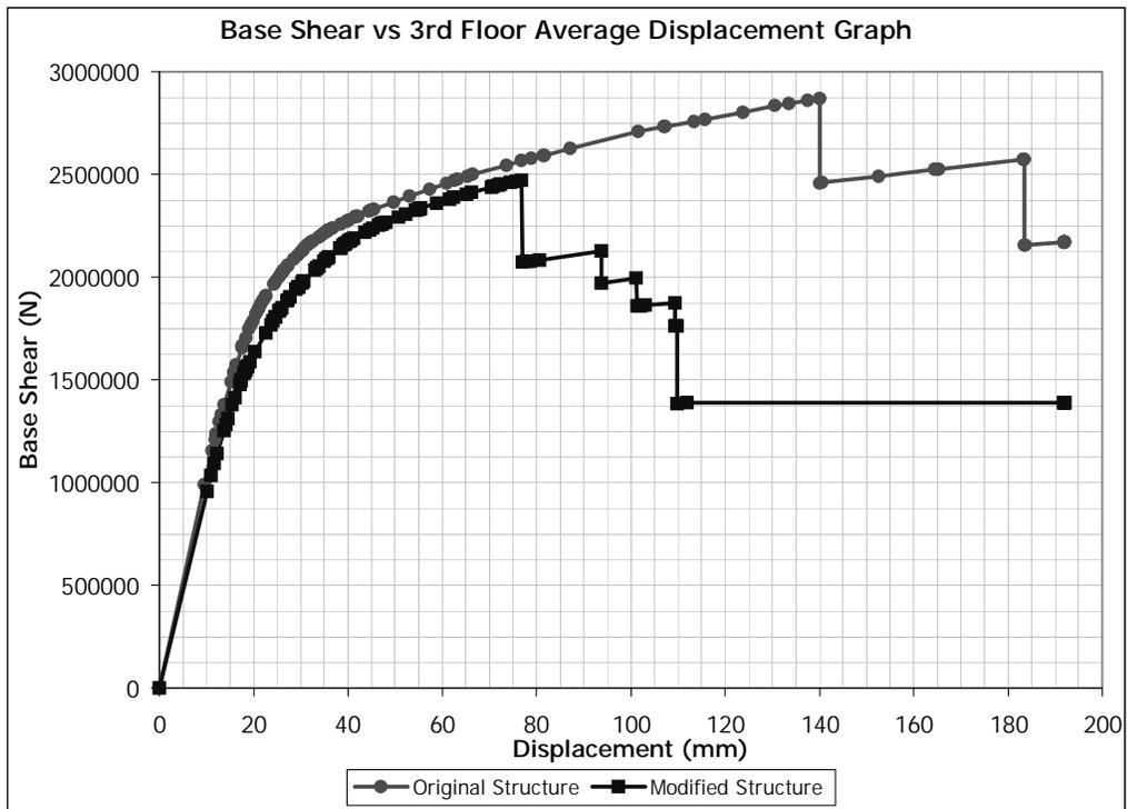
Figure 5.116 (+) Y Direction Pushover for Building 4. Removed Member: C0103
