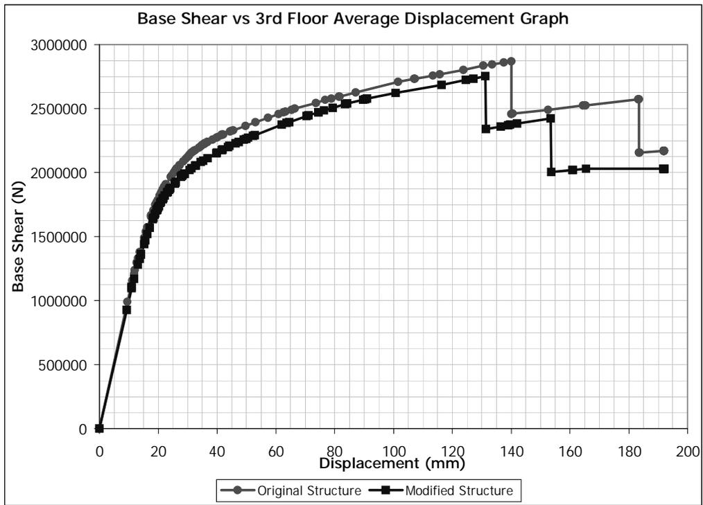
Figure 5.119 (+) Y Direction Pushover for Building 4. Removed Member: C0106
