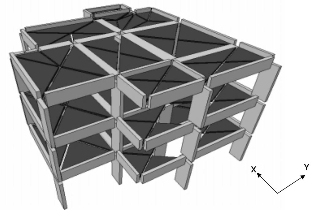
Figure A.9 State of Building (Back Side) at Drift of 90 mm
