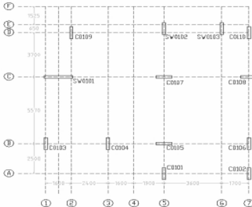
Figure A.5 Base Floor Column & Shear Wall Layout of Building
