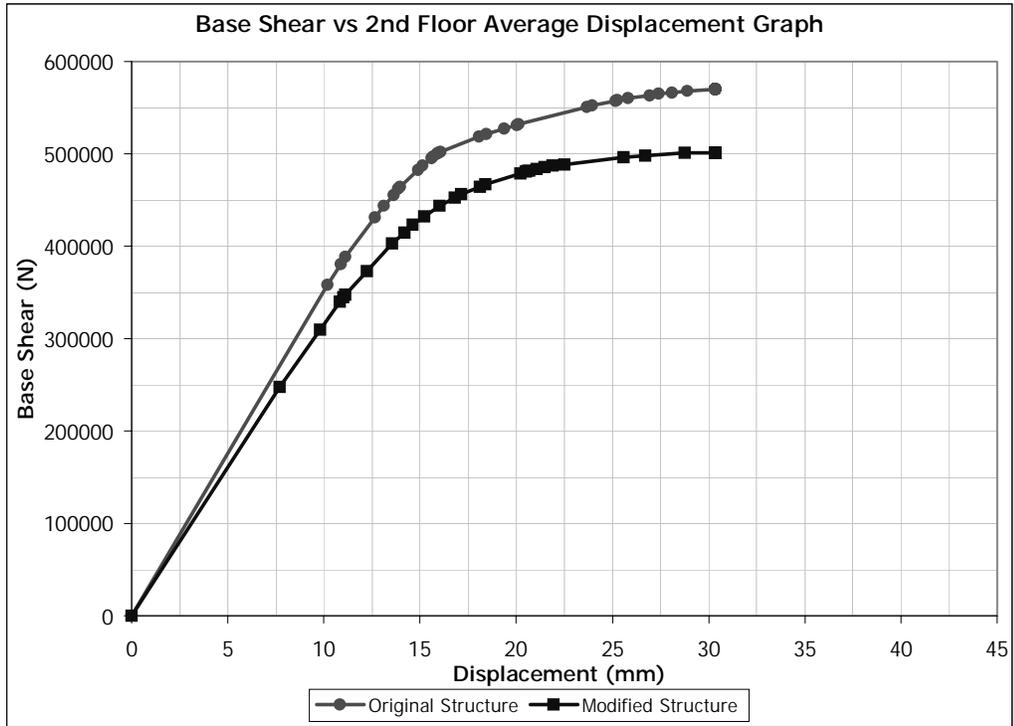
Figure 5.53 (-) Y Direction Pushover for Building 2. Removed Member: C0104
