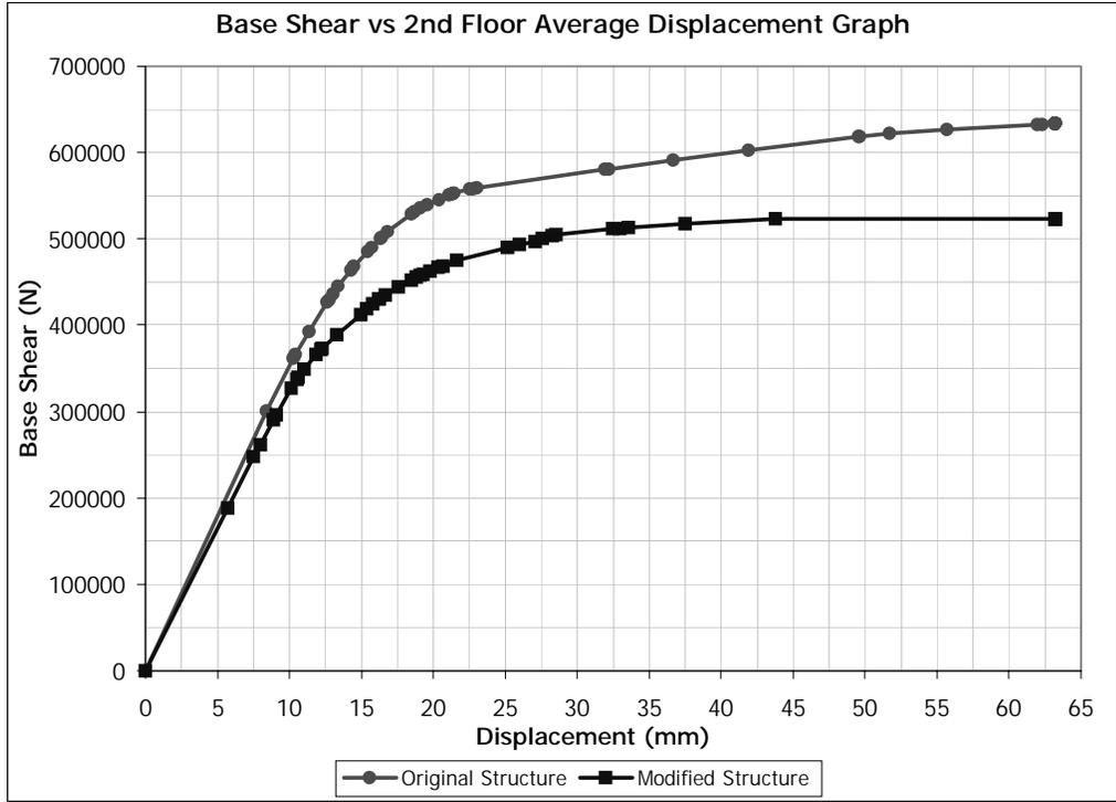
Figure 5.34 (+) Y Direction Pushover for Building 1. Removed Member: C0108
