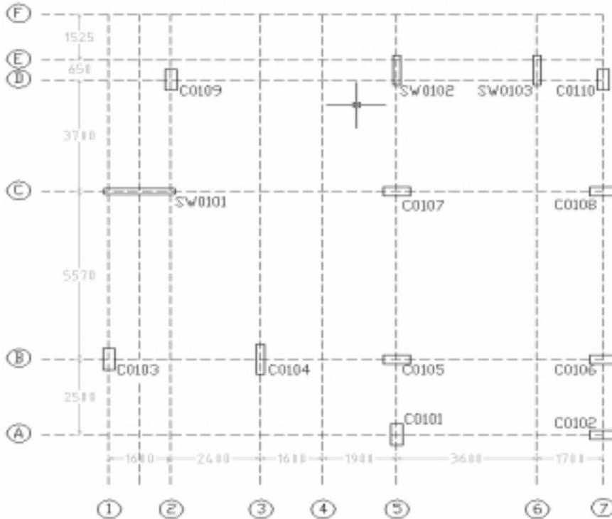
Figure 5.96 Base Floor Column & Shear Wall Layout of Building 4
