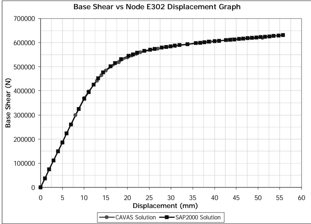
Figure 5.14 Pushover Curves obtained by CAVAS and SAP2000 in X Direction
