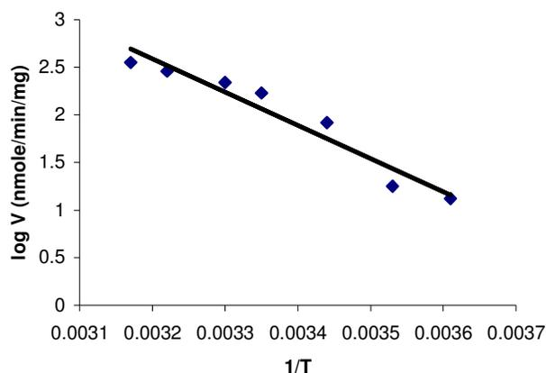
**Figure 16.** The Arrhenius plot for Turkish red pine GST catalyzed reactions. The slope, for calculating the activation energy value, was determined from linear scale. The conditions were identical to those described in the legend of Figure 17.
