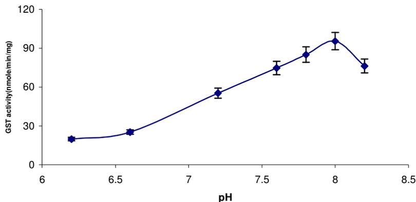
**Figure 14.** Effect of pH on cytosolic GST activity. Reaction mixture contained 1 mM GSH, 1 mM CDNB, 25 mM phosphate buffer and distile water. The reactions were carried out at 25° C for 2 minutes. Each point is the mean of three different sets of experiments done three independent experiments.
