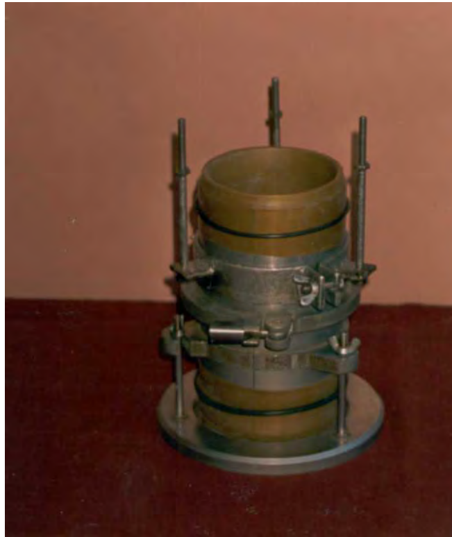
Figure 6.2. Rubber membranes on the three-part split mould with special attachment (after Gökalp, 1994)
