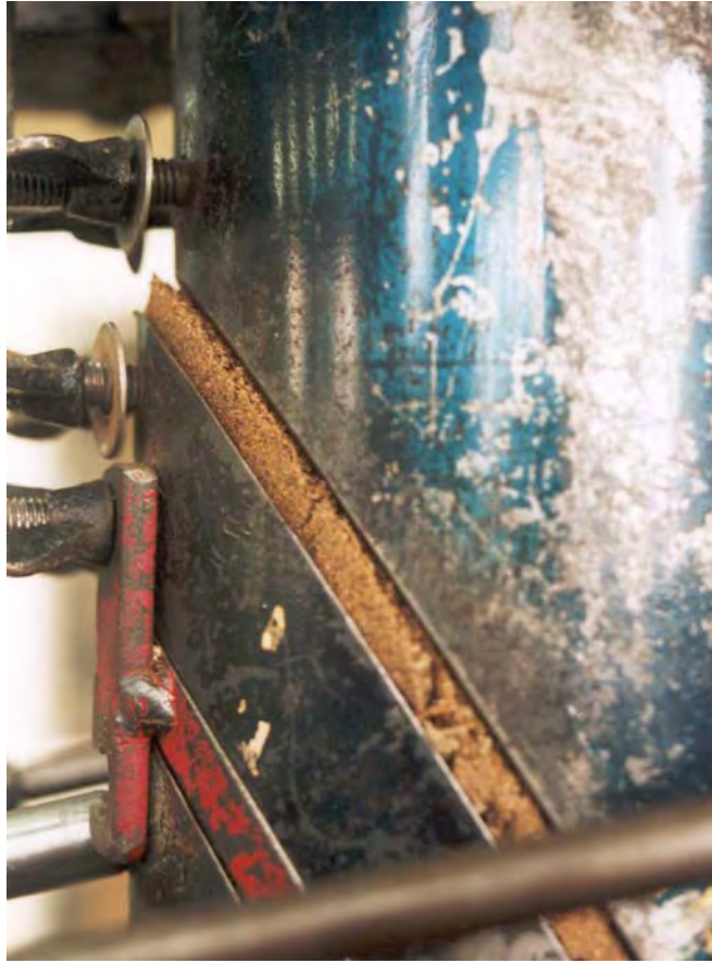
Figure D.1. The sand specimen does not bear on the test mould during shear
