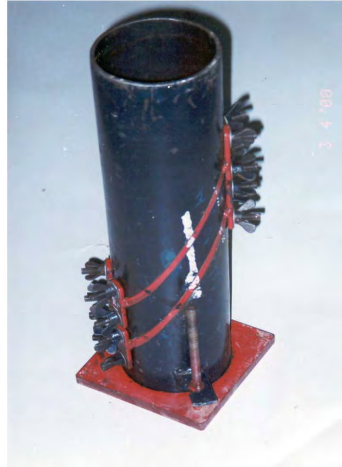
Figure 5.1. Apparatus used for cylwests (a) modified compression machine; (b) double-cut mould (after Gürol, 2000)
