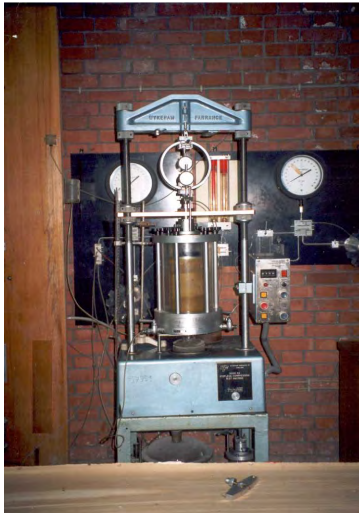
Figure 6.6. Layout of triaxial cell with the anti-friction guide
