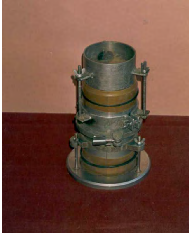
Figure 6.4. Three-part split mould with collar held gently above the rubber membrane (after Gökalp, 1994)
