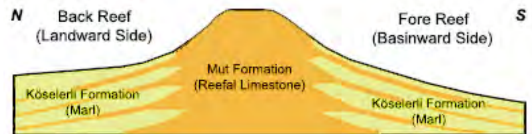
Figure 2.6: Sketch illustrating the relationship between Mut and Köşelerli formations (Not to scale).
