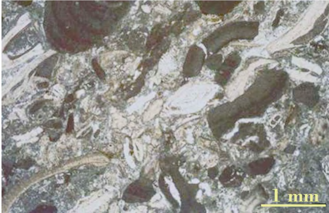
Figure 4.1: On the ramp sequence (Sequence I) little porosity is present. Present pore spaces are filled by calcite cement. There are some leaching. This may be due to low porosity and permeability. Sample number 43 (Plane light x2.5).
