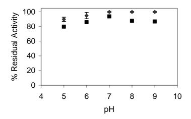
**Figure 3.12** The effect of pH on stability of polyphenol oxidase. The enzyme solutions were incubated at different pHs for 1 h. ( $\blacklozenge$ ) crude extract, ( $\blacksquare$ ) pure enzyme.
