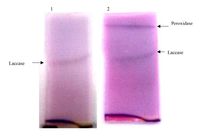
**Figure 3.6** Laccase and peroxidase activities on polyacrylamide gel. (1) gel after the treatment with ADA, (2) gel after the treatment with  $H_2O_2$ .
