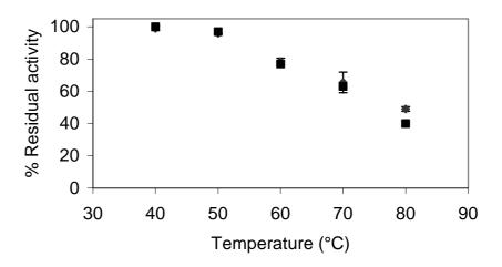
**Figure 3.10** Thermostability of polyphenol oxidase. Relative activity was defined as percentage of residual activity compared to maximum activity remained. (♦) crude extract, (■) pure enzyme.
