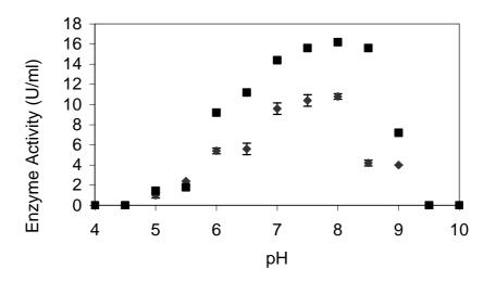
Figure 3.11 Effect of pH on the activity of polyphenol oxidase. (♦) crudeextract, (■) pure enzyme. Enzyme experiments were performed at 50°C.
