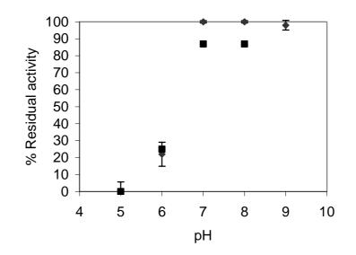
Figure 3.13 Long-term pH stability of the polyphenol oxidase. The enzyme solutions were incubated at different pHs for 18 h at room temperature.
