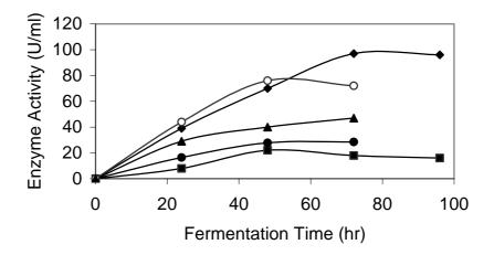
**Figure 3.4** The effect of fermentation pH on PPO production. Fermentation medium: 1.4% yeast extract, 0.3% MgSO<sub>4</sub>, 1% KH<sub>2</sub>PO<sub>4</sub>, 0.003% CuSO<sub>4</sub>, 0.032% gallic acid. Fermentations were performed in a 3 L bioreactor at 50°C, 400 rpm, 80% dissolved oxygen at varying pH levels (pH 7.0 (•), 8.0 (•), 8.5 ( $\circ$ ), 9.0 ( $\blacktriangle$ ) and uncontrolled ( $\blacksquare$ ).
