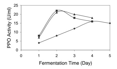
Figure 3.5 The effect of dissolved oxygen on polyphenol oxidase production. Fermentation medium: 1.4% yeast extract, 0.3% MgSO<sub>4</sub>, 1% KH<sub>2</sub>PO<sub>4</sub>, 0.003% CuSO<sub>4</sub>, 0.032% gallic acid. Fermentations were performed in a bioreactor at 50°C, at 400 rpm, pH 7.0, dissolved oxygen [70% ( $\blacklozenge$ ), 80% ( $\blacksquare$ ), 90% ( $\blacktriangle$ )].
