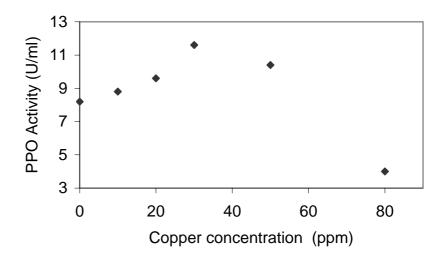
Figure 3.1 The effect of CuSO<sub>4</sub> concentration on polyphenol oxidase production. Fermentation medium: 1.43% yeast extract, 0.3% MgSO<sub>4</sub>, 1% KH<sub>2</sub>PO<sub>4</sub> and 10-80 ppm CuSO<sub>4</sub>. The fermentations were performed at 45°C at 155 rpm in a shaker incubator.
