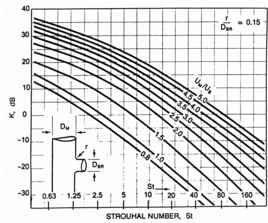
**Figure 3.3** Normalized Spectra for Flow-Generated Noise of Takeoffs and Junctions without Splitter Damper or Scoop [6]
