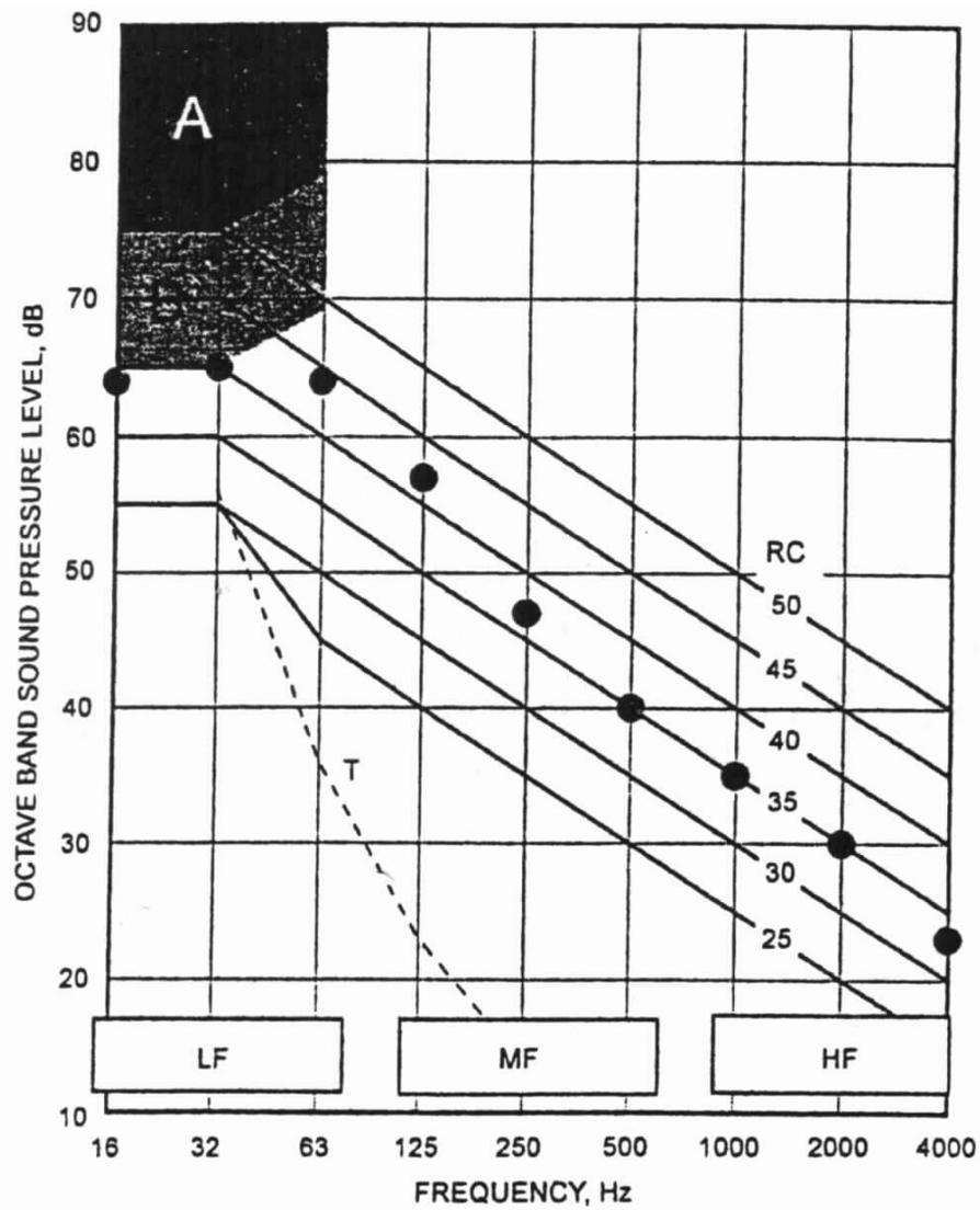
Noise levels in region B are likely to generate perceptible vibration in light walls and ceilings. Rattles are a slight possibility in light fixtures, doors, windows, etc. Noise levels in region A have a high probability of generating easily perceptible noise induced vibration in light walls and ceilings. Audible rattling in light fixtures, doors, windows, etc. is likely. Regions LF, MF, and HF are explained in the text. The solid dots are sound pressure levels for Example 5.
