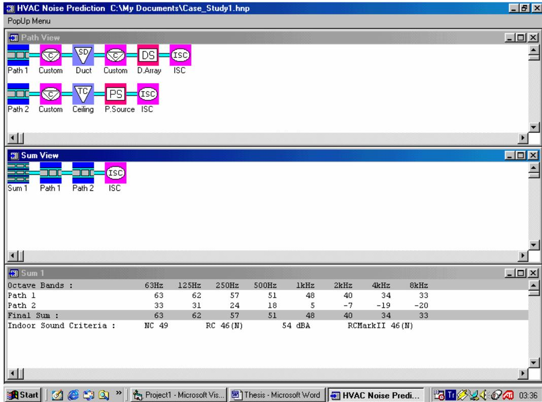
**Figure 6.1** A Snap Shot from the HNP Program with a Completed Sum Showing the Case\_Study1 Rating Results
