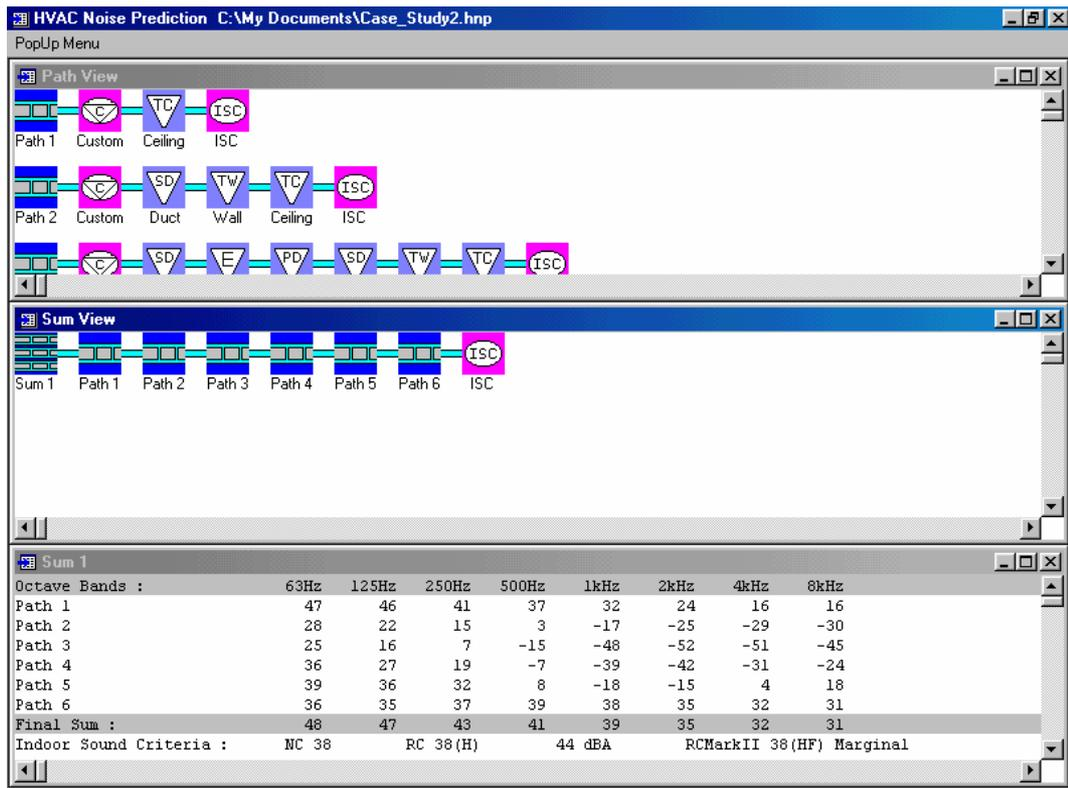
**Figure 6.11** A Snap Shot from the HNP Program with a Completed Sum Showing the Case\_Study2 Rating Results
