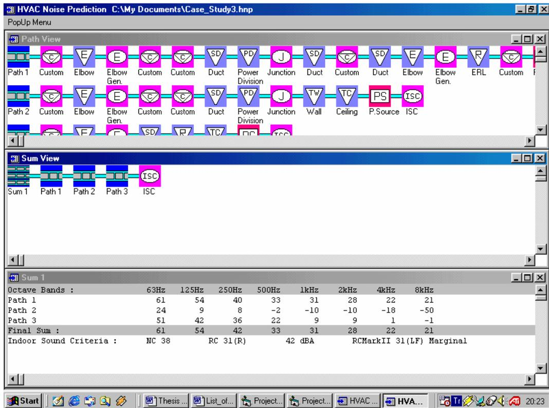
**Figure 6.19** A Snap Shot from the HNP Program with a Completed Sum Showing the Case\_Study3 Rating Results
