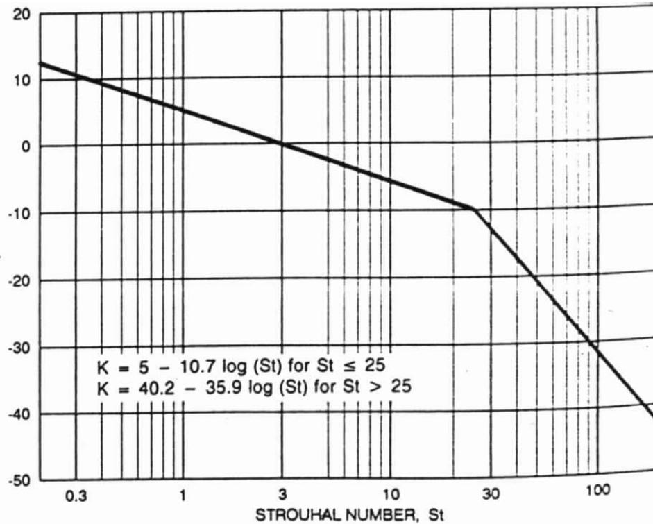
**Figure 3.1** Characteristic Spectrum of K of Flow-Generated Noise of Dampers for use with Equation (3. 3) [6]
