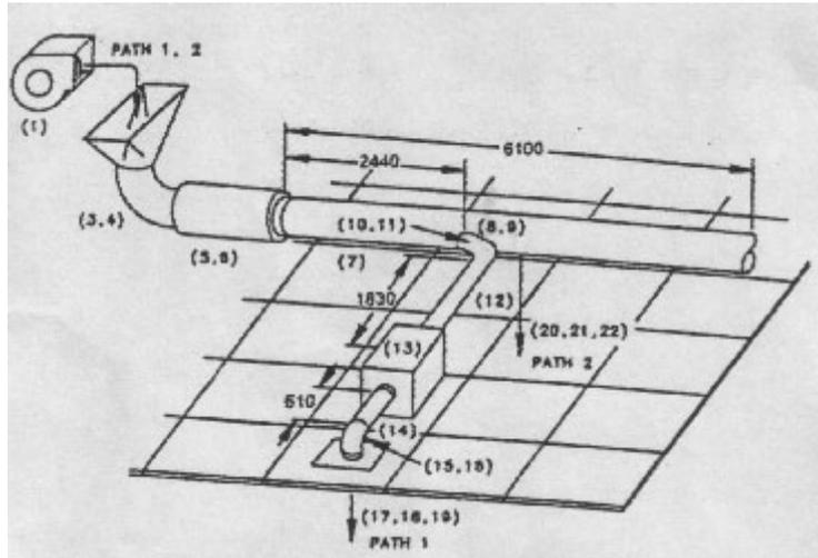
**Figure 6.14** Supply Air Portion Layout for Case\_Study3 [5]
