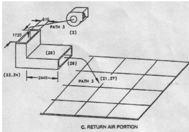
**Figure 6.15** Return Air Portion Layout for Case\_Study3 [5]
