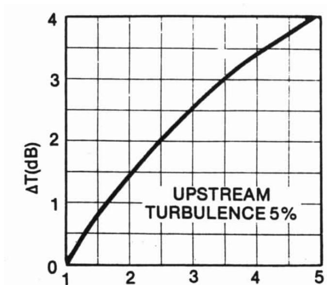
Figure 3.5 Correction for Upstream Turbulence [6]
