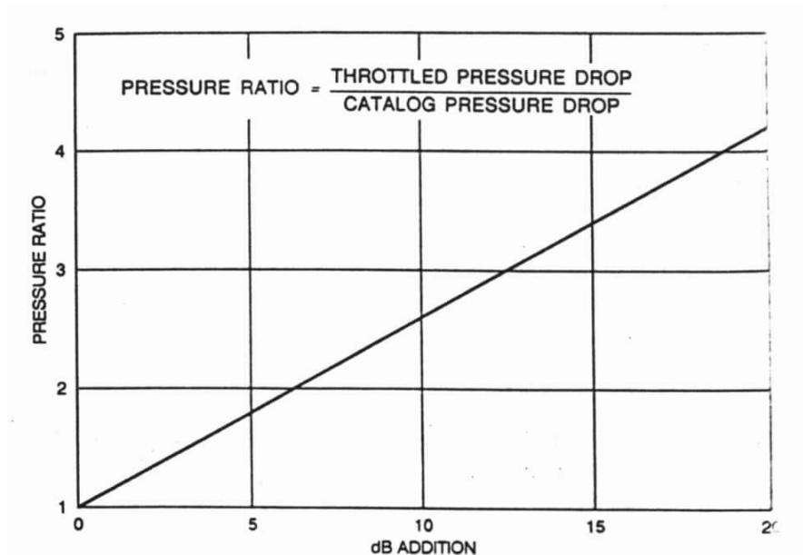
**Figure 3.6** Decibels to be Added to Outlet Sound for Throttled Damper Close to Outlet [6]
