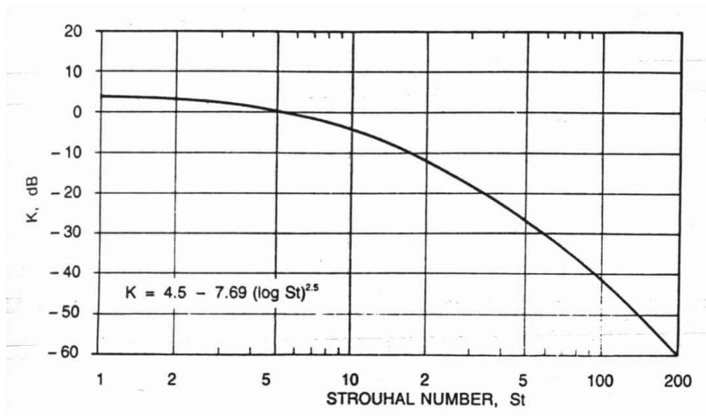
**Figure 3.2** Characteristic Spectrum of K of Flow-Generated Noise for Bends Fitted with Curved-Blade Turning Vanes [6]
