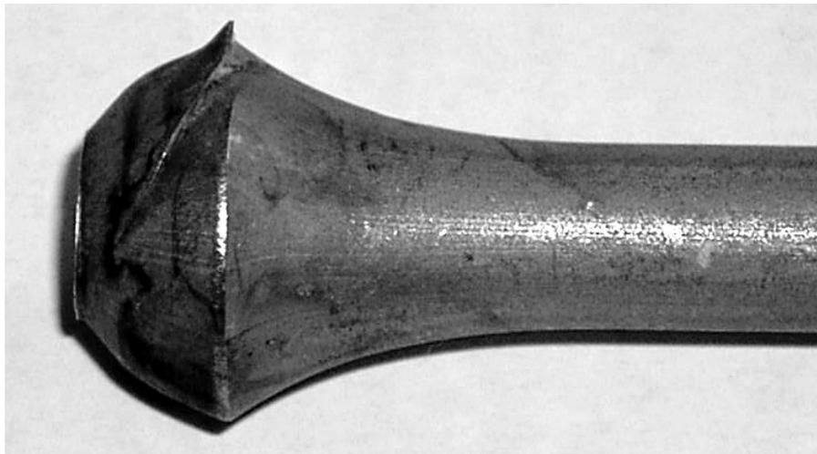
**Figure 4.22** Cracked material in a heading process (HILTI Corp., Liechtenstein)
