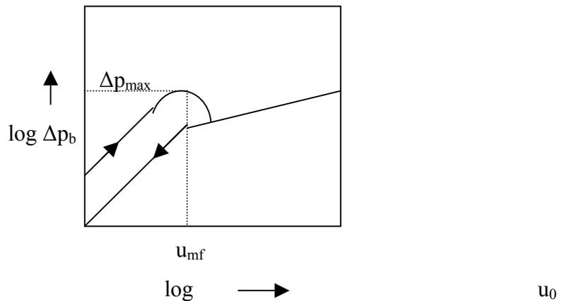
**Figure 1.2** Pressure drop - velocity relationship for an actual bed.
