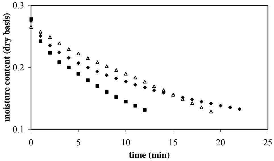
**Figure 3.13** Drying curves for 70°C temperature and 50% power level.
