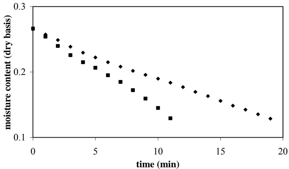
**Figure 3.3** Microwave drying curves at different power levels.
