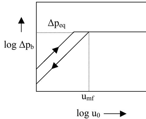
**Figure 1.1** Pressure drop - velocity relationship for an ideal bed.
