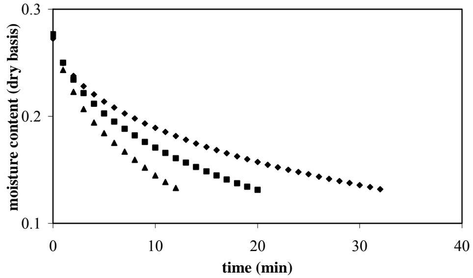
**Figure 3.4** Drying curves for fluidized bed and microwave assisted fluidized bed drying at 50°C temperature.
