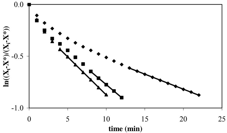
**Figure 3.17** Variation of dimensionless moisture content with time for the fluidized bed and microwave assisted fluidized bed drying at 70°C temperature.
