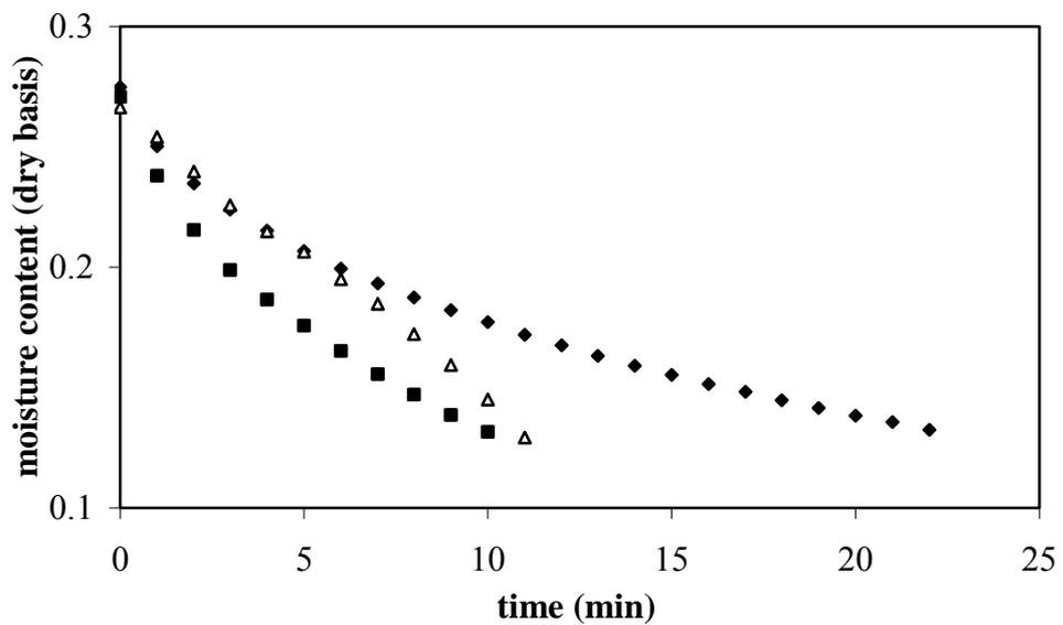
**Figure 3.14** Drying curves for 70°C temperature and 100% power level.
