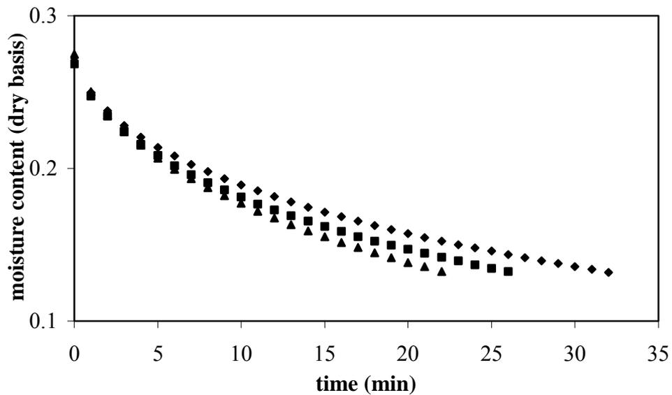
**Figure 3.2** Fluidized bed drying curves at different temperatures.
