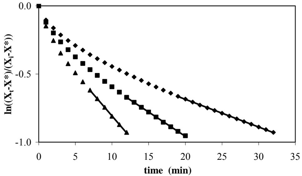
**Figure 3.15** Variation of dimensionless moisture content with time for the fluidized bed and microwave assisted fluidized bed drying at 50°C temperature.
