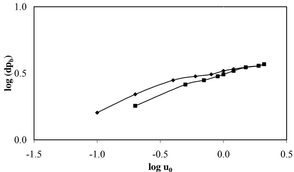
**Figure 3.1** Variation of the pressure drop with the superficial air velocity in the fluidized bed.
