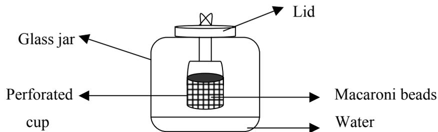
**Figure 2.2** Rehydration apparatus.
