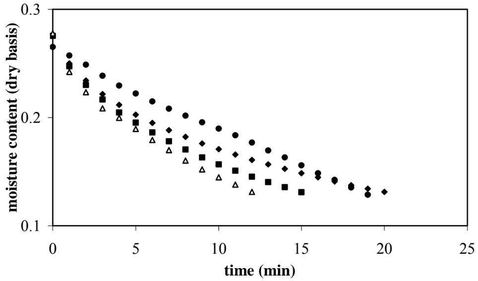
**Figure 3.7** Drying curves for microwave and microwave assisted fluidized bed drying at 50% power level.
