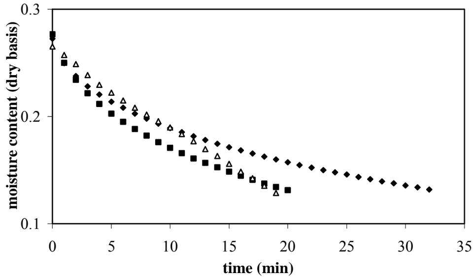
**Figure 3.9** Drying curves for 50°C temperature and 50% power level.
