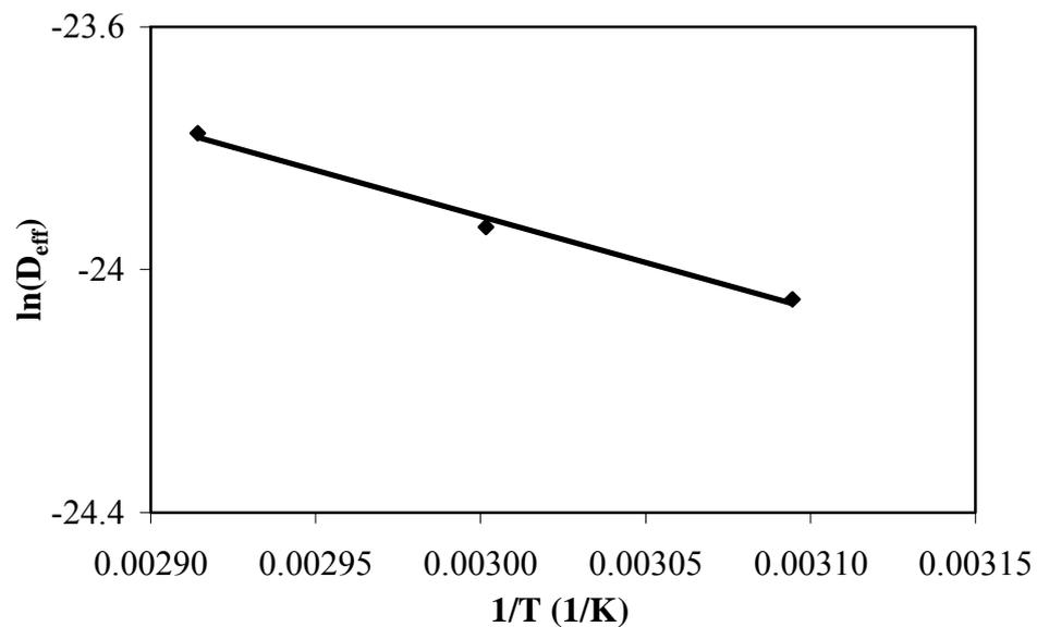
**Figure 3.18** Arrhenius plot for the fluidized bed drying.
