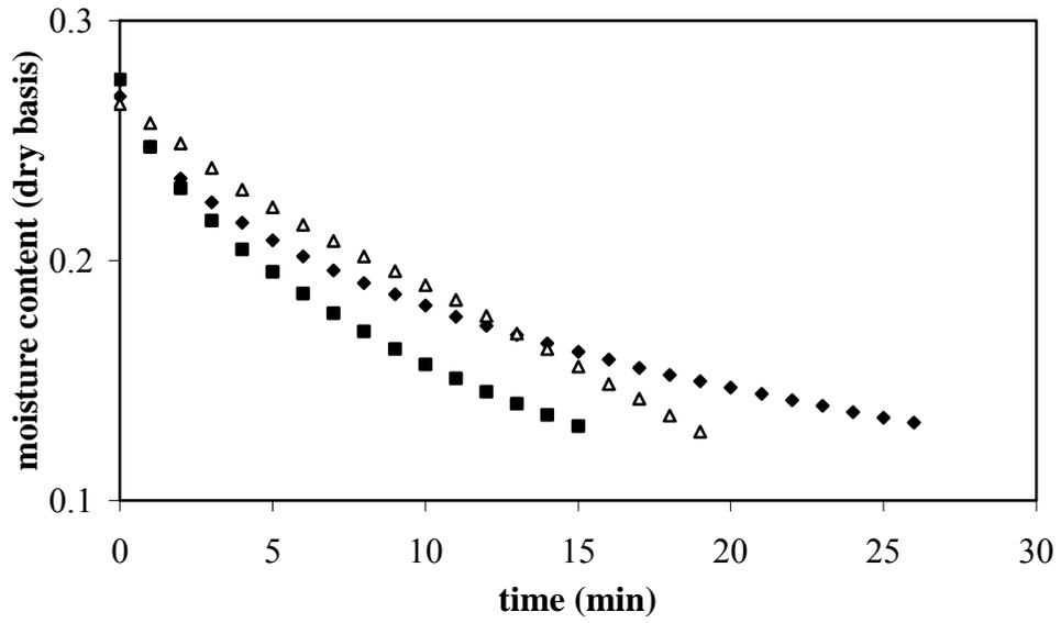
**Figure 3.11** Drying curves for 60°C temperature and 50% power level.
