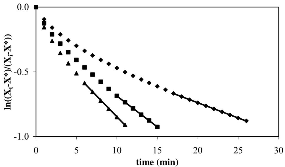
**Figure 3.16** Variation of dimensionless moisture content with time for the fluidized bed and microwave assisted fluidized bed drying at 60°C temperature.
