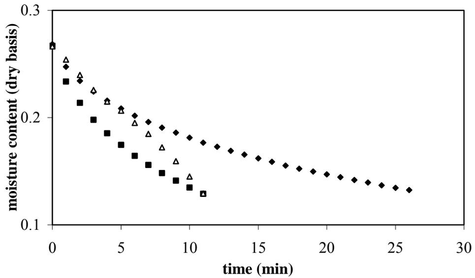
**Figure 3.12** Drying curves for 60°C temperature and 100% power level.
