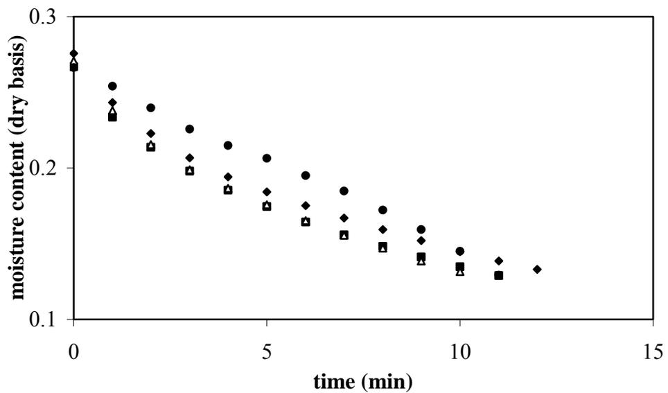
**Figure 3.8** Drying curves for microwave and microwave assisted fluidized bed drying at 100% power level.
