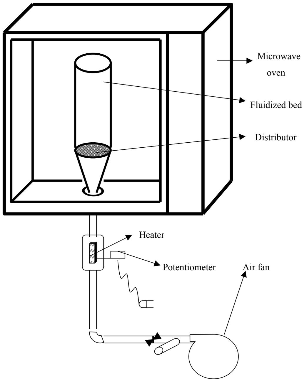
**Figure 2.5** Microwave assisted fluidized bed drying apparatus.
