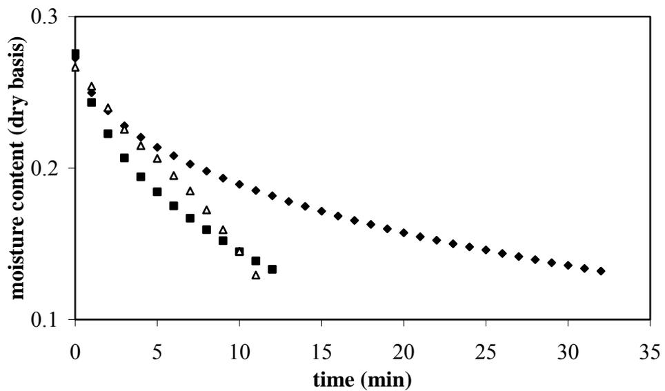
**Figure 3.10** Drying curves for 50°C temperature and 100% power level.
