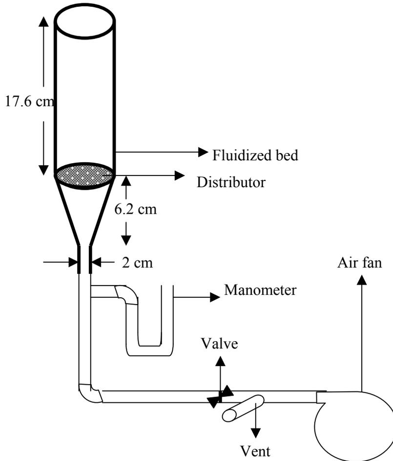
**Figure 2.1** Apparatus for the determination of superficial air velocity.
