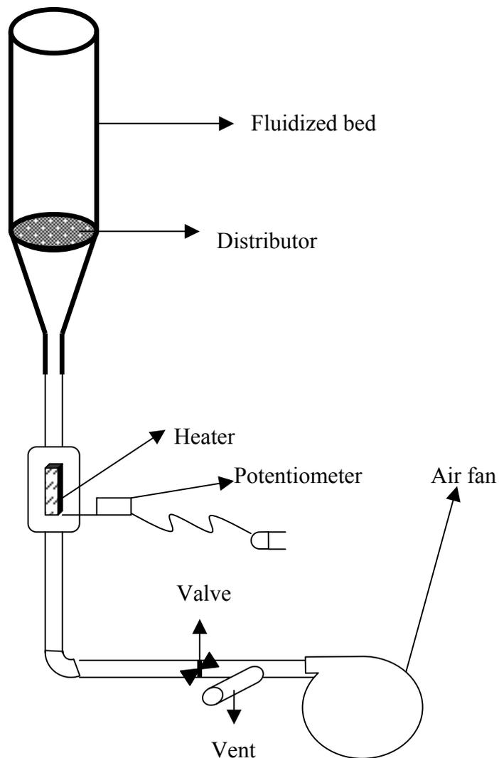
**Figure 2.3** Fluidized bed drying apparatus.
