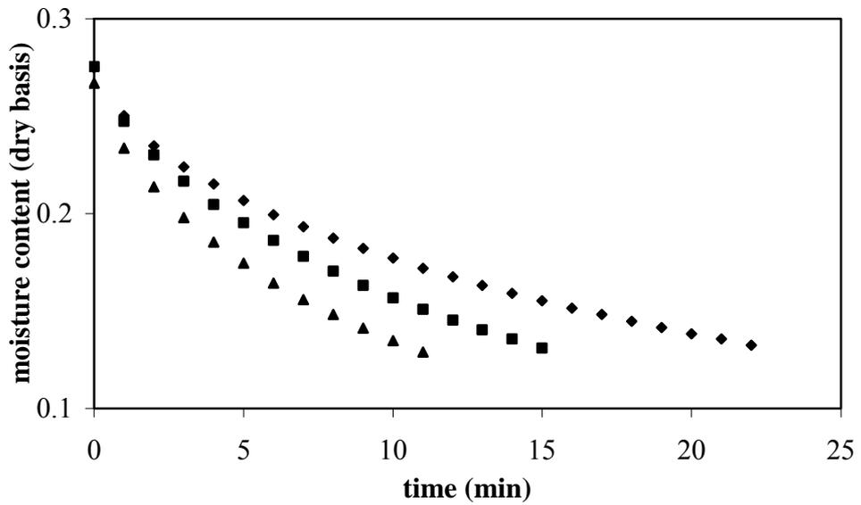
**Figure 3.5** Drying curves for fluidized bed and microwave assisted fluidized bed drying at 60°C temperature.
