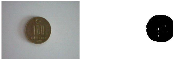
Figure 5.8 Original coin image and binarized coin image (Threshold = 123)
