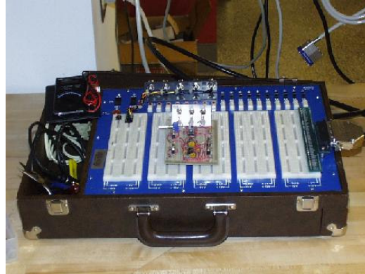
Figure 3.7 Breadboard kit for prototyping and dSpace interfacing used at MIT [7]
